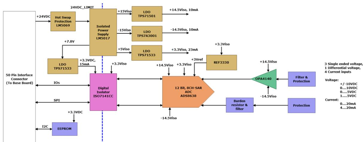
Figure 1 Block Level Design
