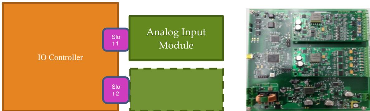
The IO Controller communicates with the Analog Input Module through an isolated SPI interface. A graphical user interface is provided to communicate with the IO Controller.
