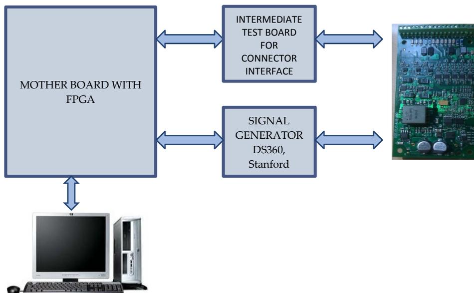
The design verification setup uses FPGA and GUI based Test Setup. The GUI on the PC connects to the FPGA based data capture card through USB communication. The FPGA based data capture card then controls the Analog Input Card via SPI interface. The setup has a precision signal generator (DS360, Stanford Research Systems), which feeds the analog input signal to the Analog Input Module. The Digital Output generated is measured by the data capture card. The GUI does the computation of results.
