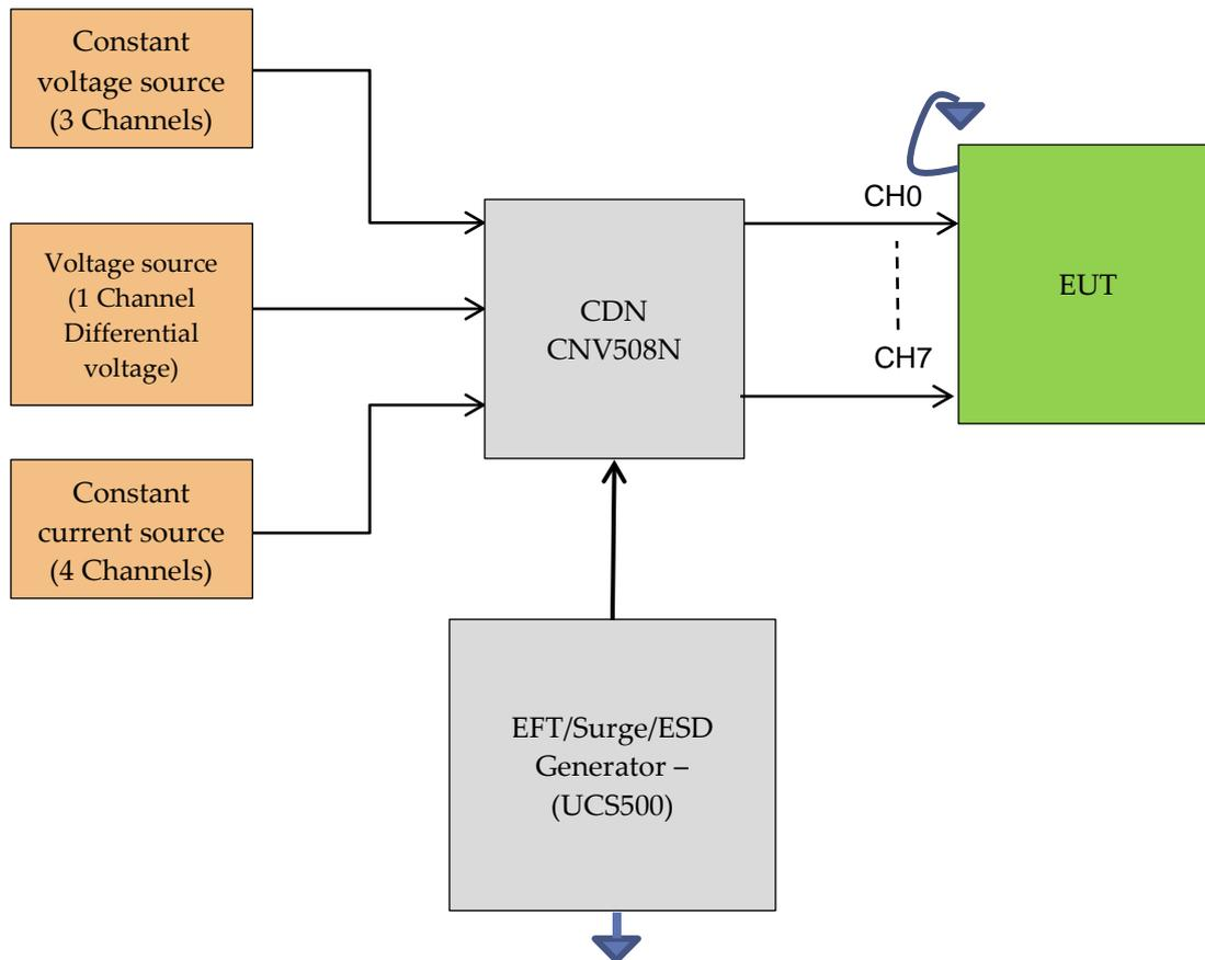
EUT operation monitored after the test. All the eight channels were monitored after the test by the MCU (on IO Controller) and compared with a Set Value (equivalent of the external constant voltage or current source). The Error should be within accuracy as mentioned in Section 6.3.1.
