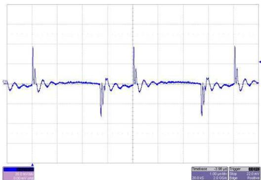
Figure 15. 12-V Ripple (C38), 20 mV/div, 1  $\mu$ s/div
