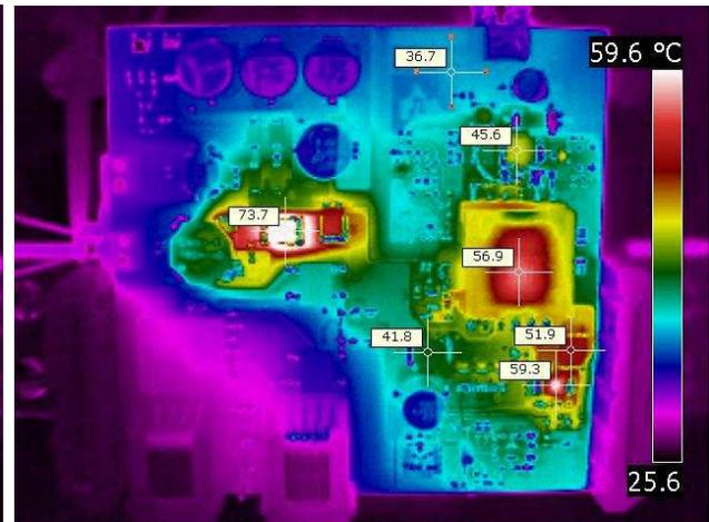
Figure 27. 12-V Input and 1.25-A Load
