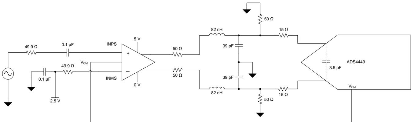
Figure 12. Circuit Used for the DC-Coupled Measurements
