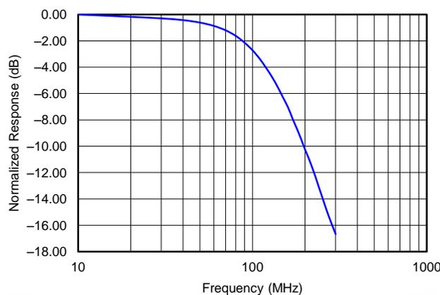
Figure 13. Normalized Gain Response — DC-Coupled First Nyquist Zone
