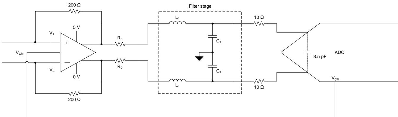
Figure 6. Typical Interface Circuit Driving an ADC
