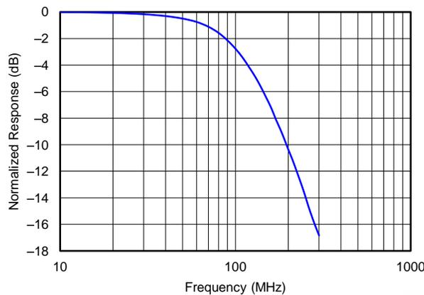
Figure 11. Normalized Gain Response — AC-Coupled
