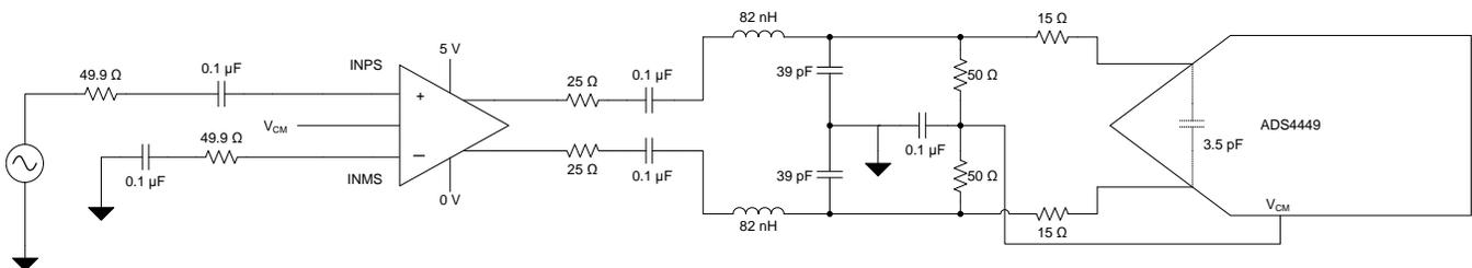
Figure 10. Circuit Used for the AC-coupled Measurements
