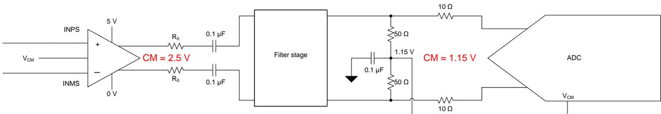
Figure 3. Interfacing With AC-Coupled Configuration
