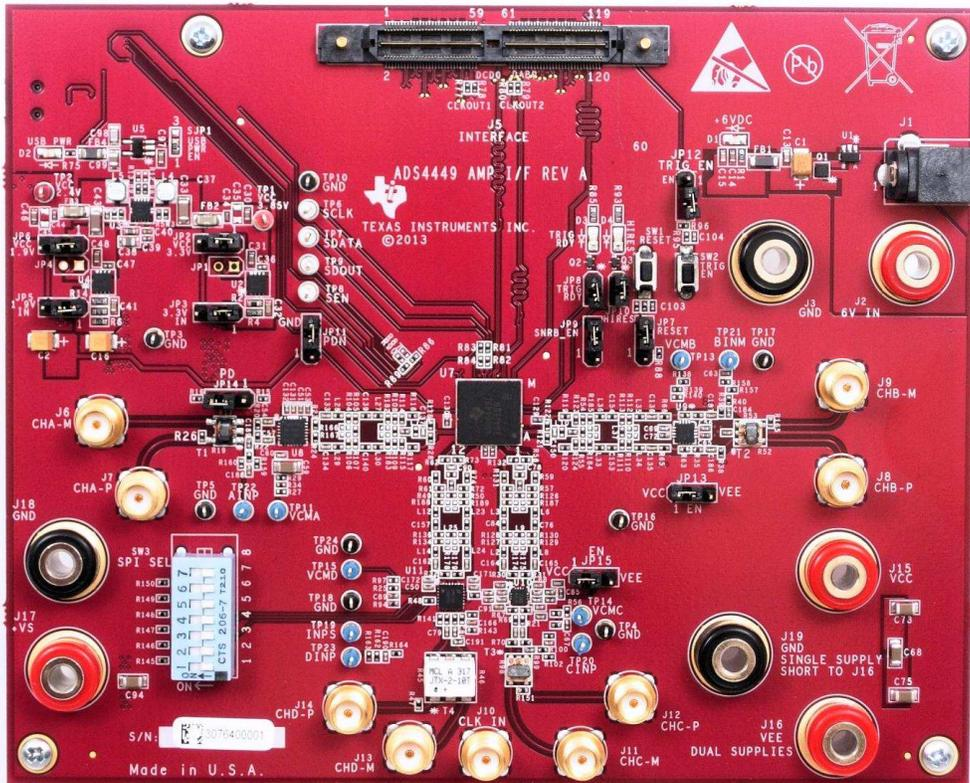
**Figure 7. LMH6881 and ADS4449 Test Board**
