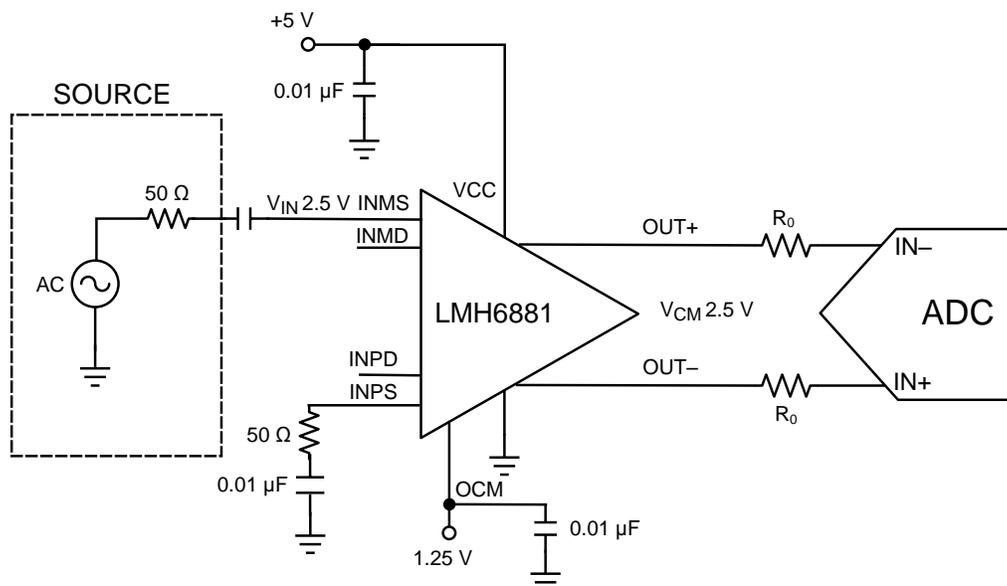
**Figure 1. Single-Ended Input With Differential Output**
