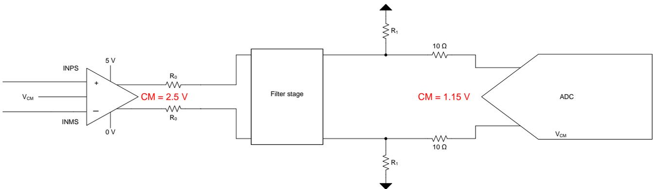
Figure 4. Interfacing With DC-Coupled Configuration
