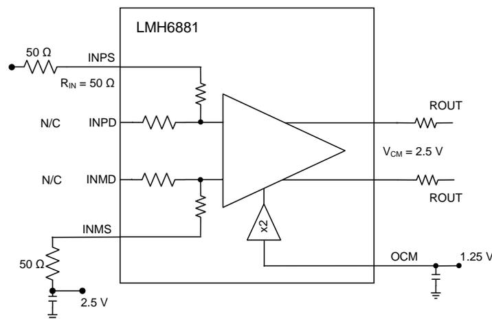
Figure 2. DC-Coupled Configuration
