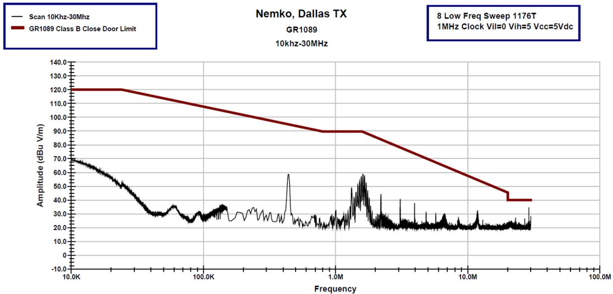
**Figure 3. Radiated Emissions (dBμV/m) from 10 kHz to 30 MHz**
