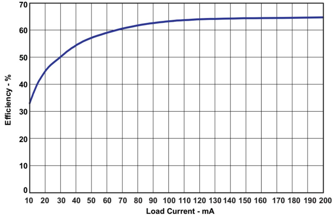
**Figure 4. Efficiency Over Load Current**
