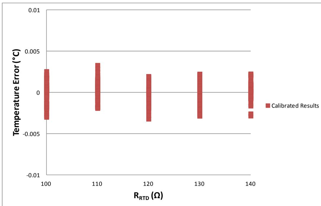
**Figure 1. Measured Temperature Accuracy with Resistive Input Representing 0°C – 100°C**
