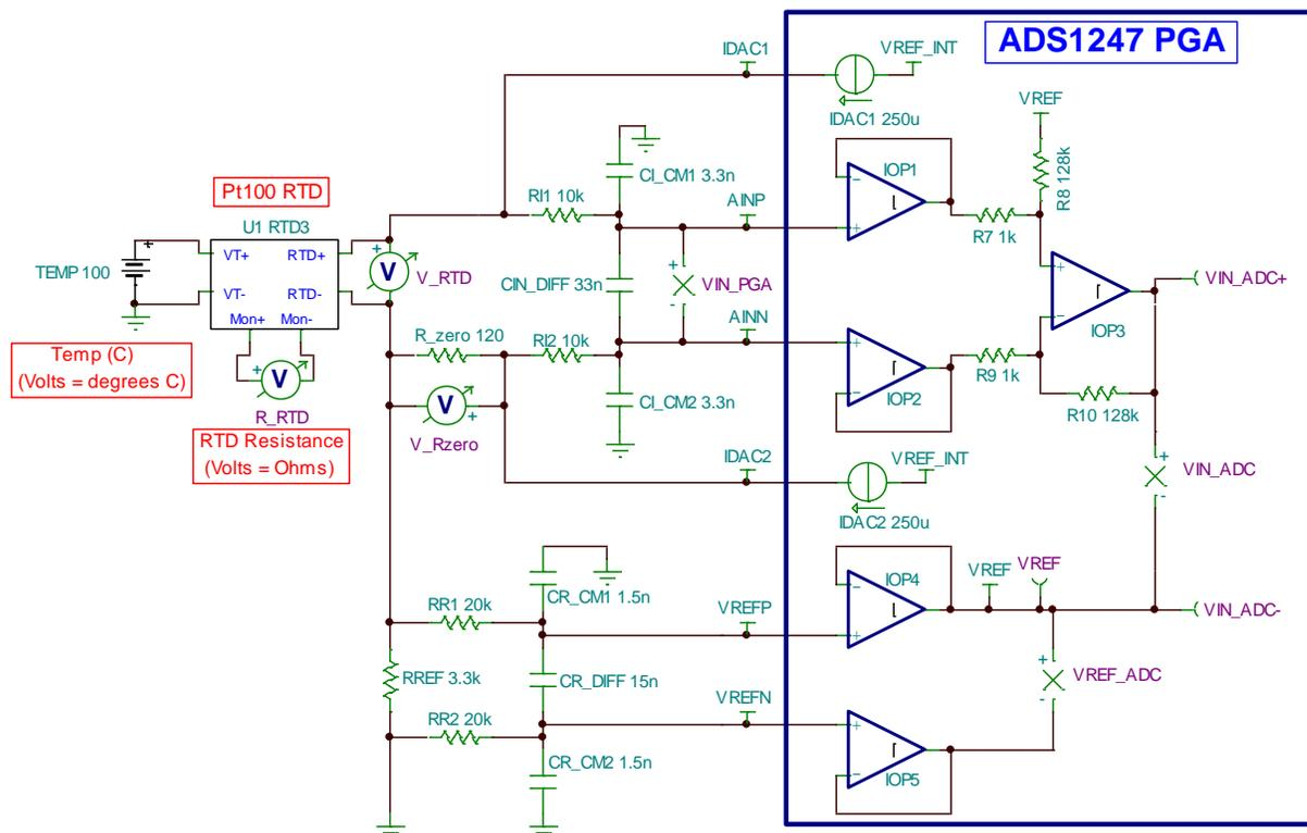
Figure 11. TINA-TI™ Simulation Circuit for the RTD and ADS1247 Inputs
