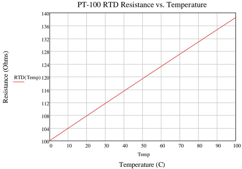
**Figure 25. PT-100 RTD Resistance from 0°C – 100°C**
