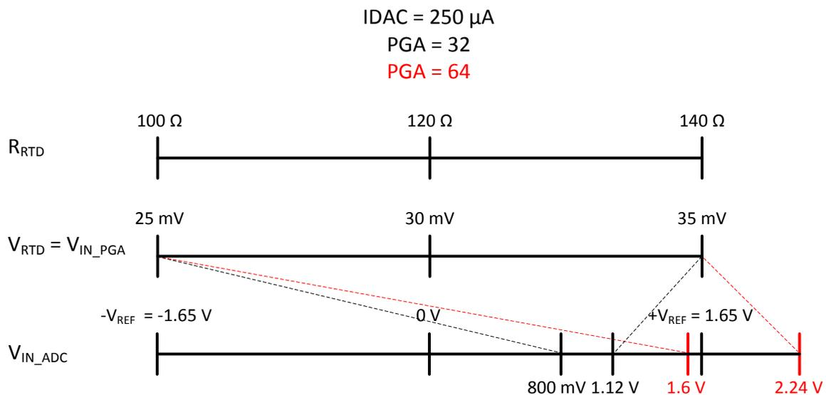
Figure 6: ADC Input Signals in a Traditional RTD System
