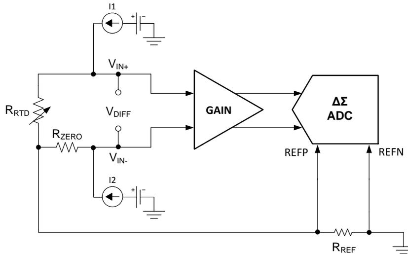
Figure 5. Hardware Compensated 3-Wire RTD System
