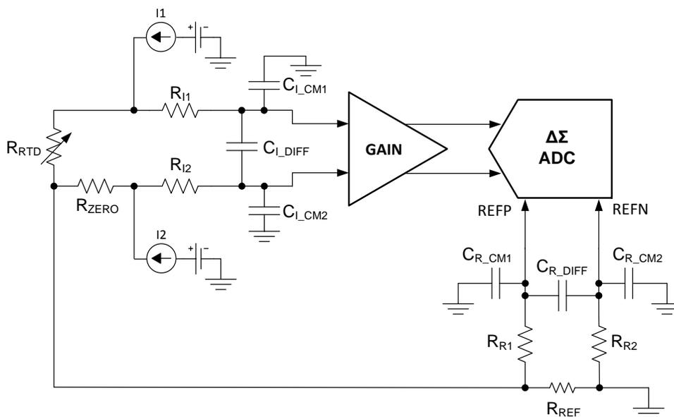
**Figure 8: Input and Reference Low-Pass Filtering**
