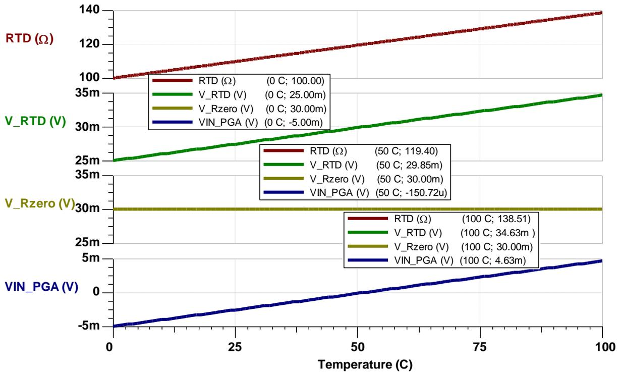
Figure 12. RTD,  $R_{ZERO}$ , and PGA Input from 0°C – 100°C
