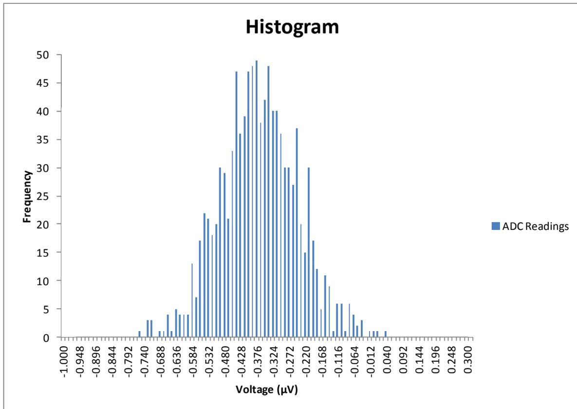
**Figure 22. Histogram with  $R_{RTD} = 120 \Omega, 0.01\%$**
