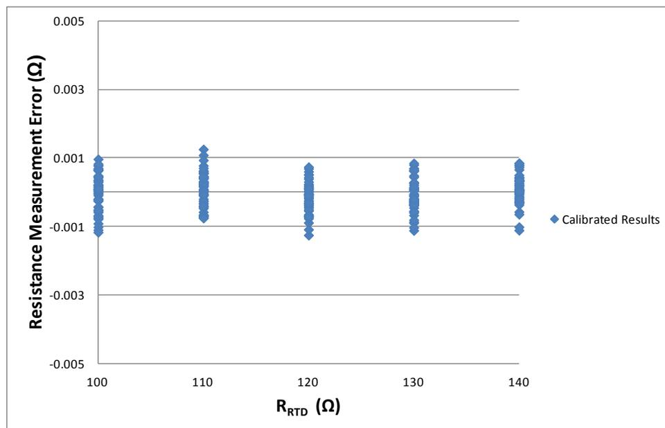
Figure 20. Resistance Measurement Results with Precision Resistors after Calibration
