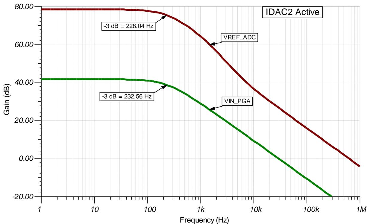
**Figure 28. Input Filter Frequency Response with IDAC2 Active**
