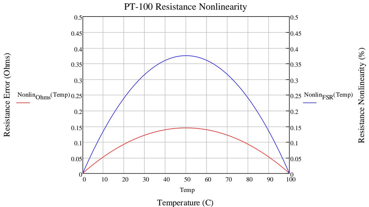
**Figure 26. PT-100 RTD Non-Linearity from 0°C – 100°C**
