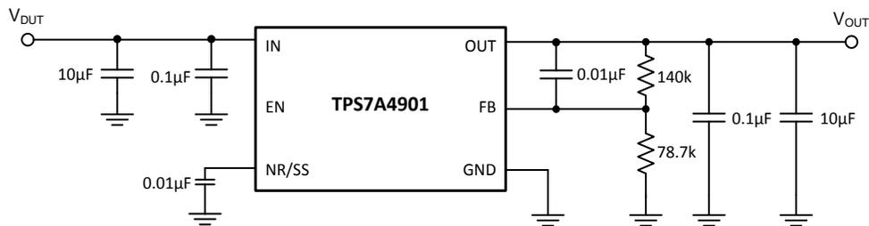
Figure 10. LDO Configuration for +3.3 V Output
