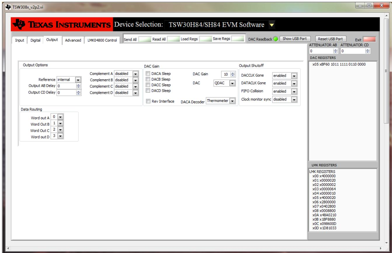
Figure 7. Output Tab Control Options – DAC348x
