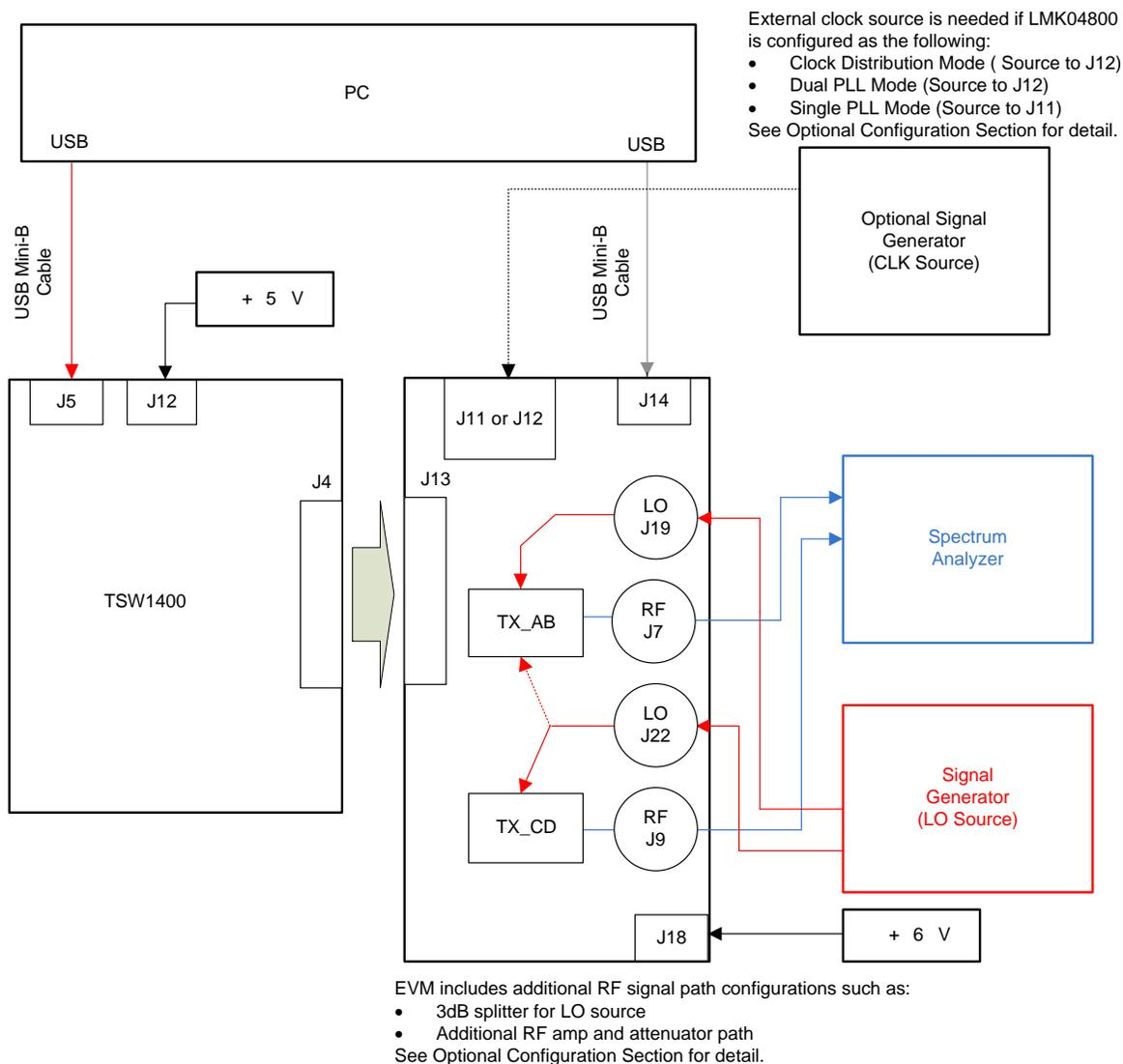
**Figure 12. TSW1400 and TSW3084/TSW30H84 Test Setup Block Diagram**
