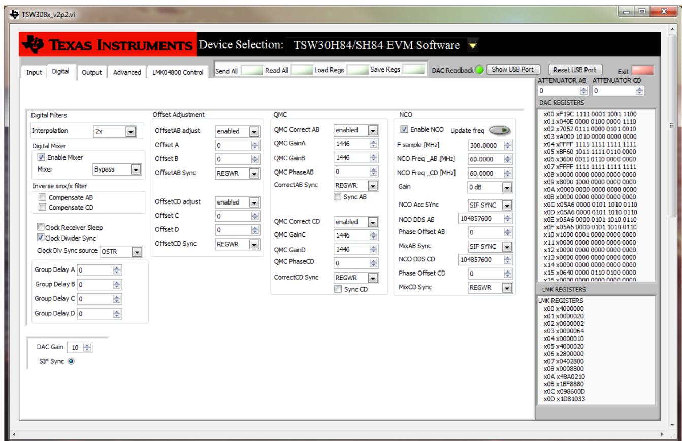
Figure 6. Digital Tab Control Options – DAC348x
