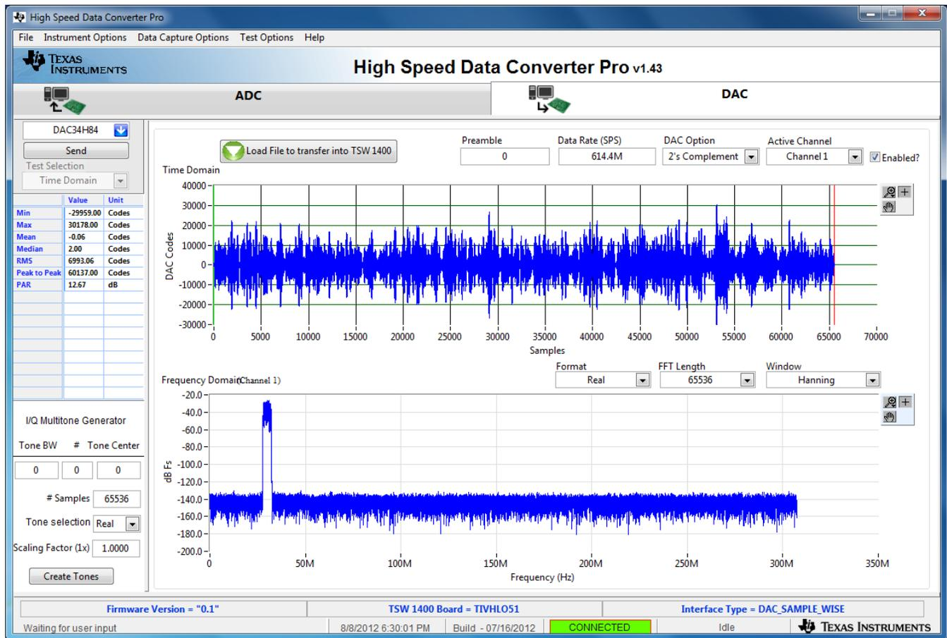
Figure 17. Load File to Transfer into TSW1400
