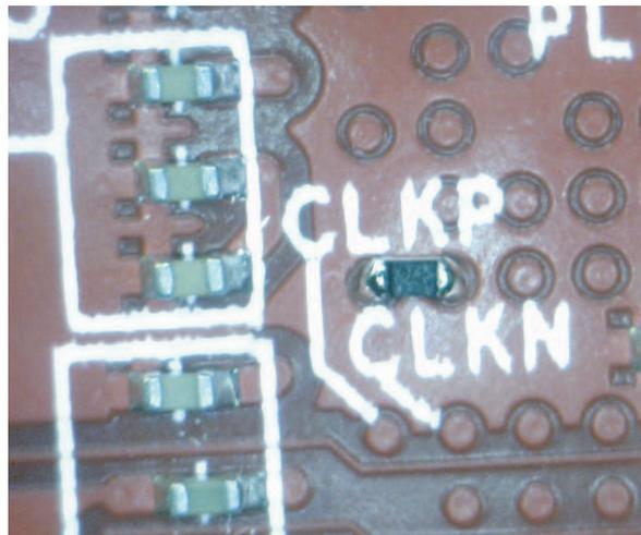
**Figure 20. TSW3100 FPGA Clock 100- $\Omega$  LVDS Termination at Pins T31 and T32 of the FPGA**
