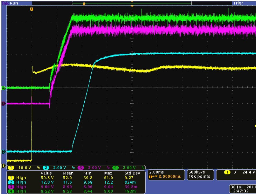
Yellow(channel 1)=Vin, Blue(channel 2)=Vout, Pink(channel 3)=primary bias, Green(channel 4)=secondary bias; **Vin=60V Iout= 15A** External capacitance=150uf
