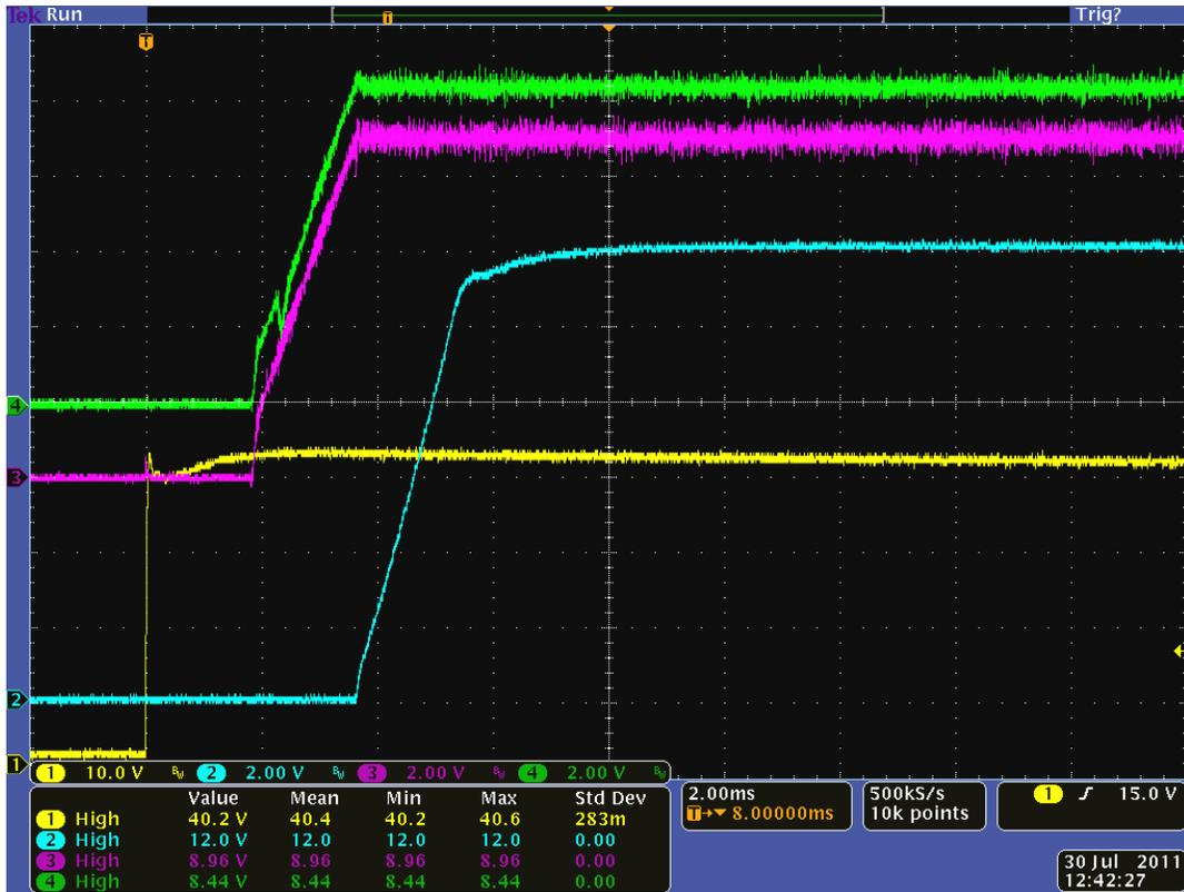
Yellow(channel 1)=Vin, Blue(channel 2)=Vout, Pink(channel 3)=primary bias, Green(channel 4)=secondary bias; **Vin=40V Iout= 0A** External capacitance=150uf
