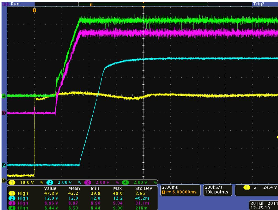
Yellow(channel 1)=Vin, Blue(channel 2)=Vout, Pink(channel 3)=primary bias, Green(channel 4)=secondary bias; **Vin=48V Iout= 15A** External capacitance=150uf
