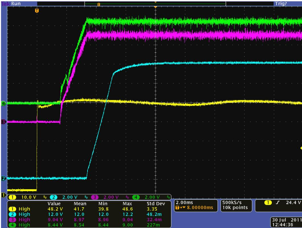
Yellow(channel 1)=Vin, Blue(channel 2)=Vout, Pink(channel 3)=primary bias, Green(channel 4)=secondary bias; **Vin=48V Iout= 5A** External capacitance=150uf
