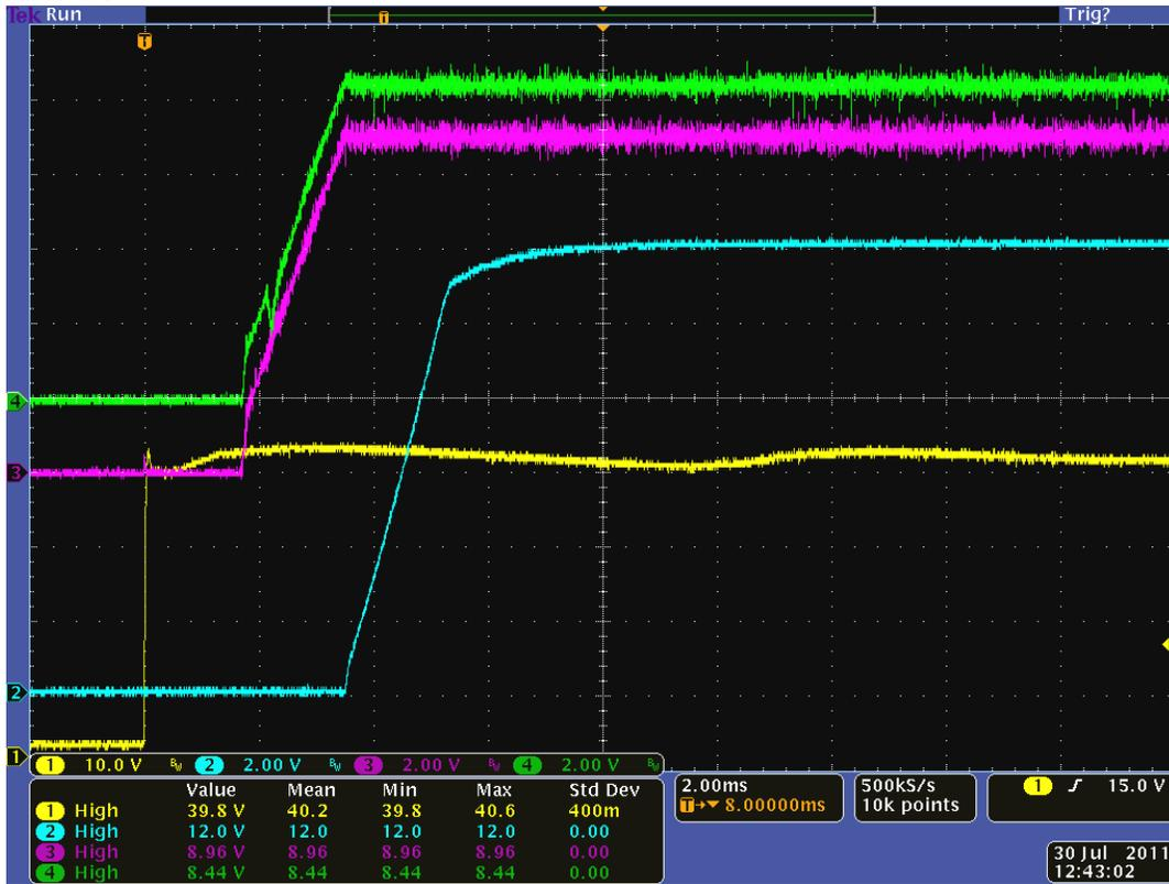
Yellow(channel 1)=Vin, Blue(channel 2)=Vout, Pink(channel 3)=primary bias, Green(channel 4)=secondary bias; **Vin=40V Iout= 5A** External capacitance=150uf
