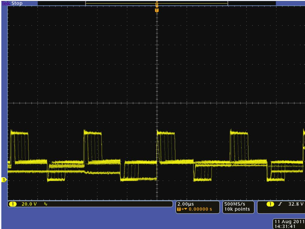
Yellow(channel 1)=Transformer Primary Voltage External capacitance=150uf
