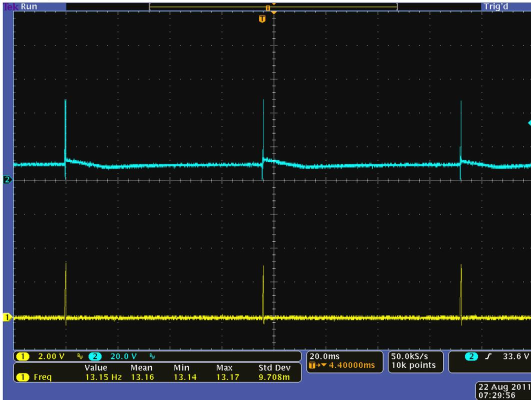
Yellow(channel 1)=  $V_{out}$ , Blue(channel 2)= Transformer Primary Voltage;  $I_{out}=20A$
