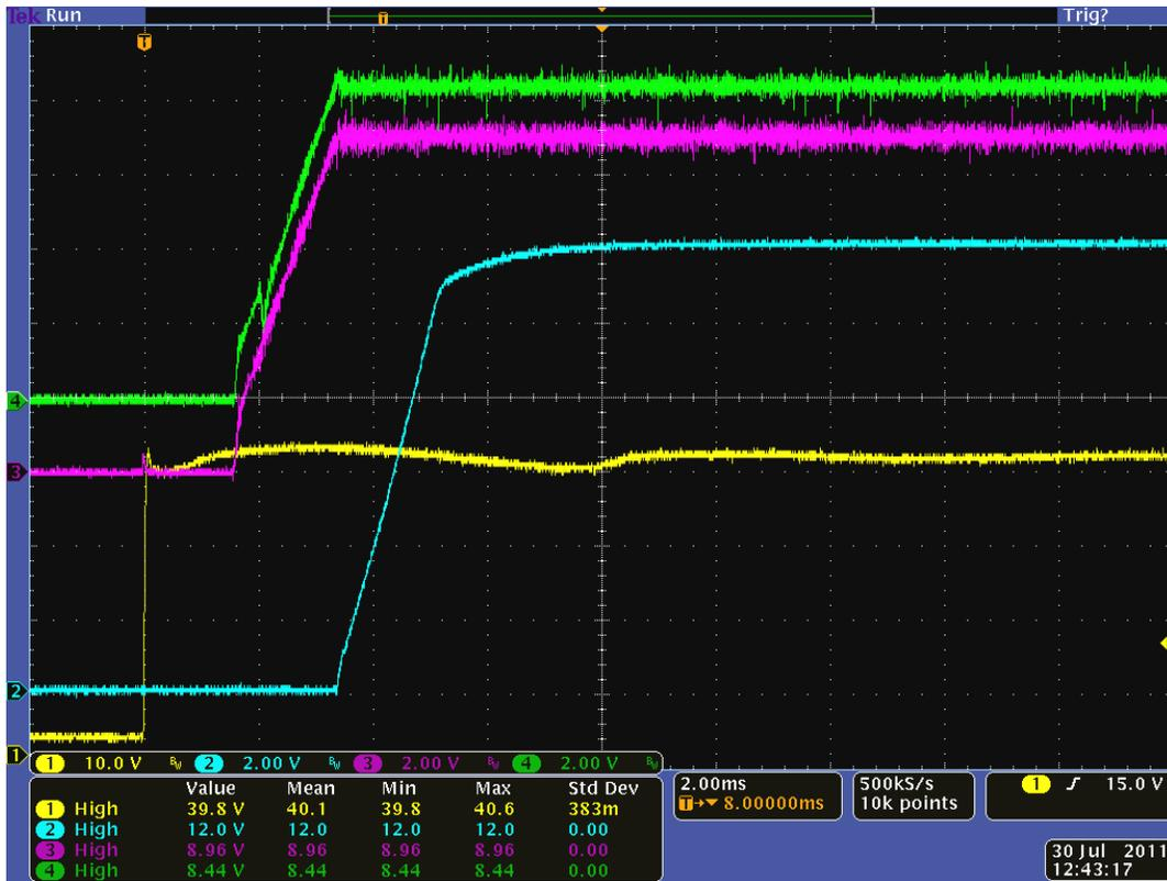
Yellow(channel 1)=Vin, Blue(channel 2)=Vout, Pink(channel 3)=primary bias, Green(channel 4)=secondary bias; **Vin=40V Iout= 10A** External capacitance=150uf
