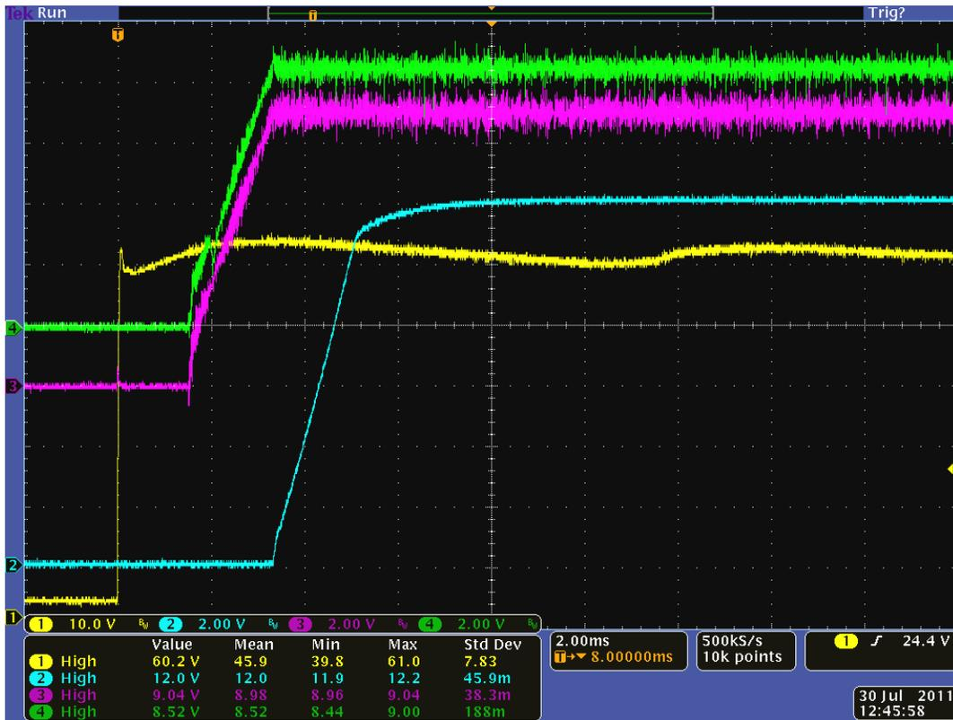
Yellow(channel 1)=Vin, Blue(channel 2)=Vout, Pink(channel 3)=primary bias, Green(channel 4)=secondary bias; **Vin=60V Iout= 10A** External capacitance=150uf
