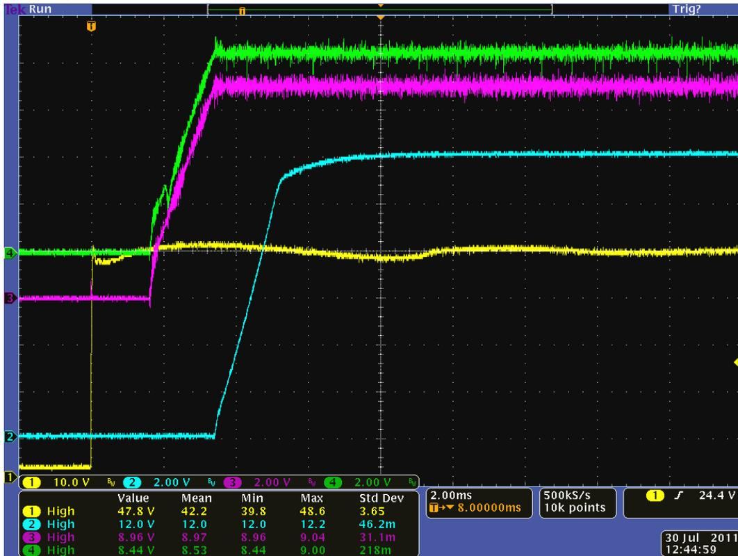
Yellow(channel 1)=Vin, Blue(channel 2)=Vout, Pink(channel 3)=primary bias, Green(channel 4)=secondary bias; **Vin=48V Iout= 10A** External capacitance=150uf
