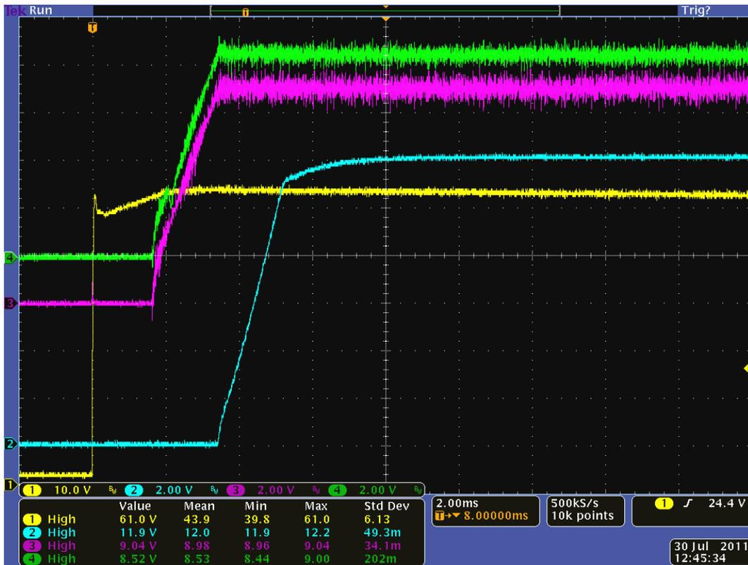
Yellow(channel 1)=Vin, Blue(channel 2)=Vout, Pink(channel 3)=primary bias, Green(channel 4)=secondary bias; **Vin=60V Iout= 0A** External capacitance=150uf
