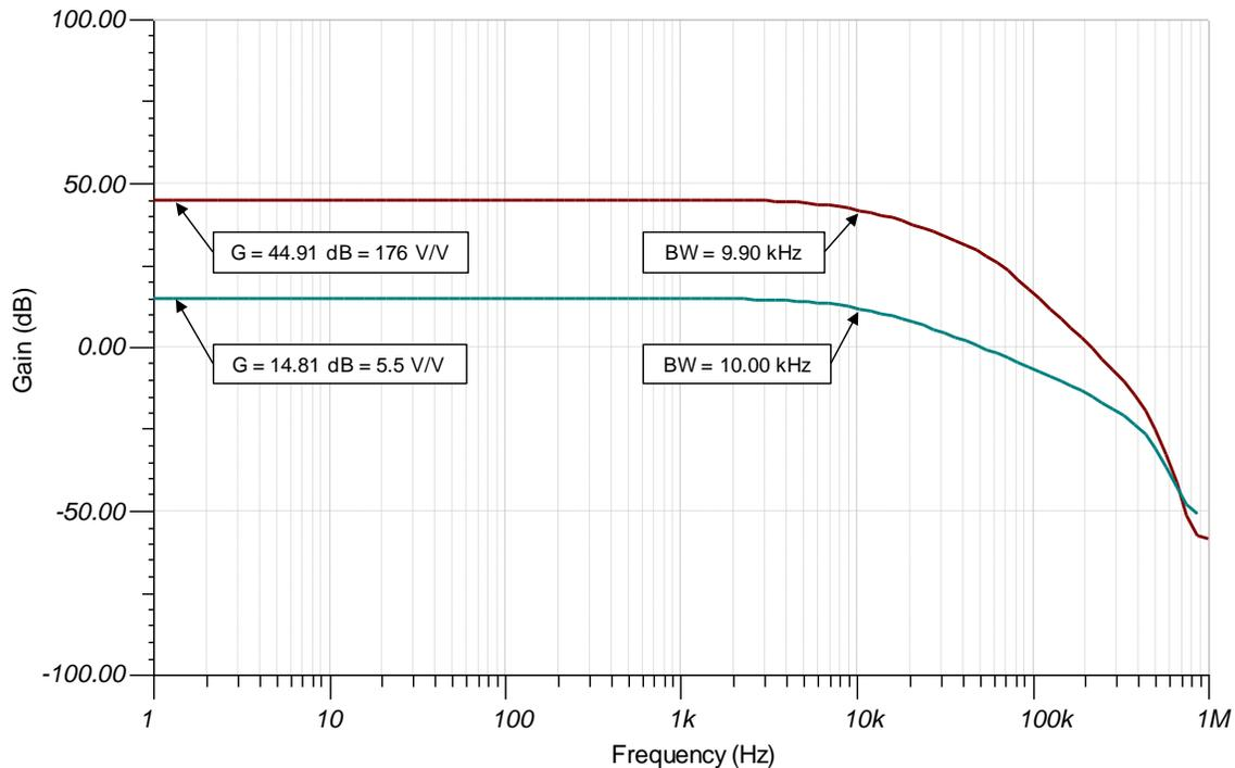
Figure 8: Simulated AC Analysis
