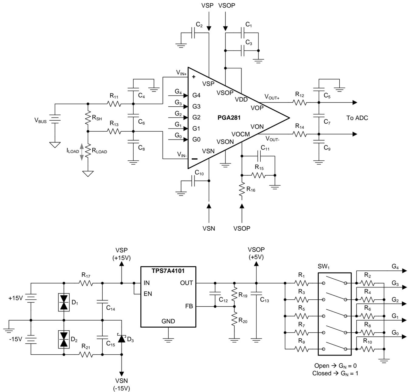
**Figure 2: Complete Circuit Schematic**
