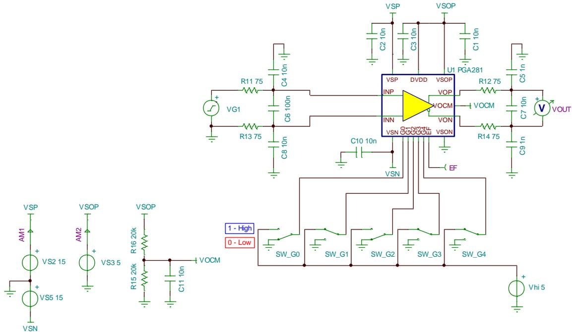
Figure 7: AC Analysis Schematic
