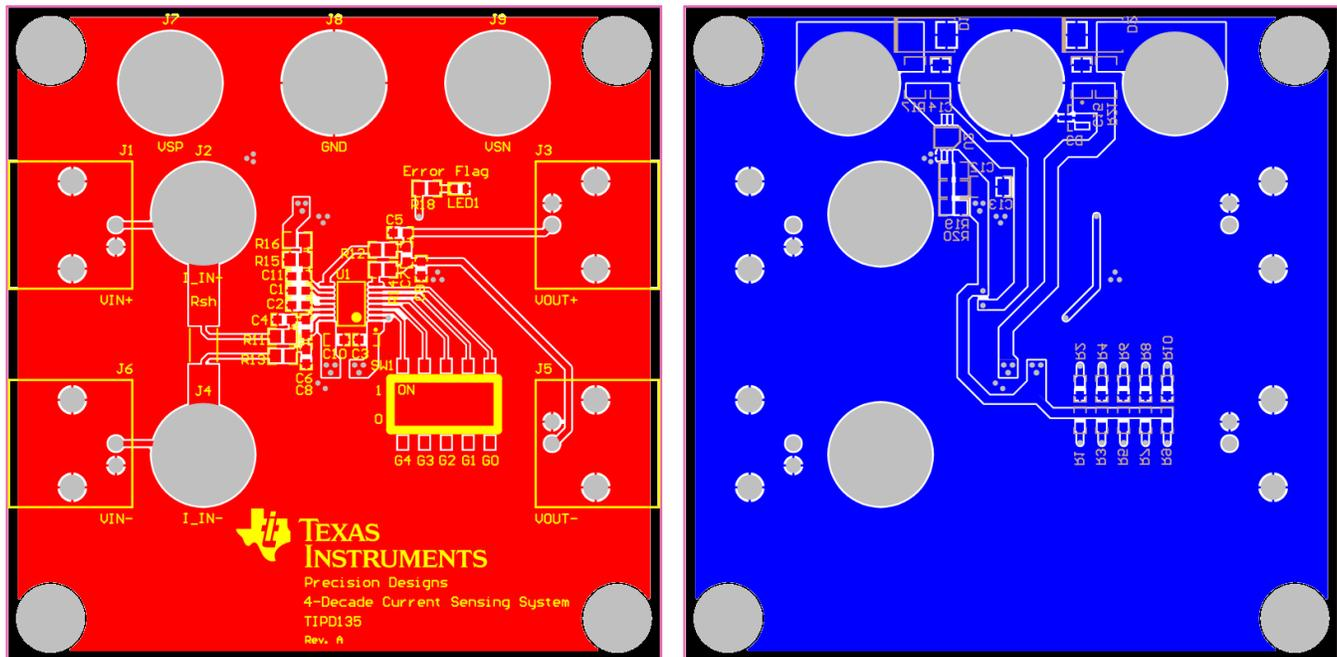
**Figure 10: PCB Layout**
