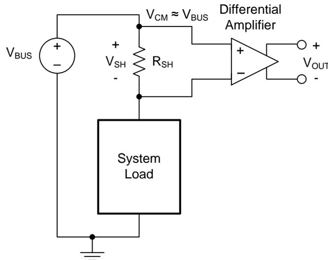
**Figure 3: High-Side Current Sensing Topology**
