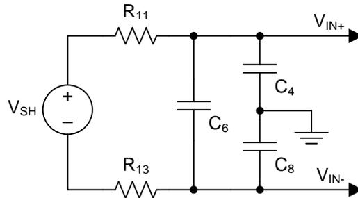
**Figure 4: Input Filter Schematic**
