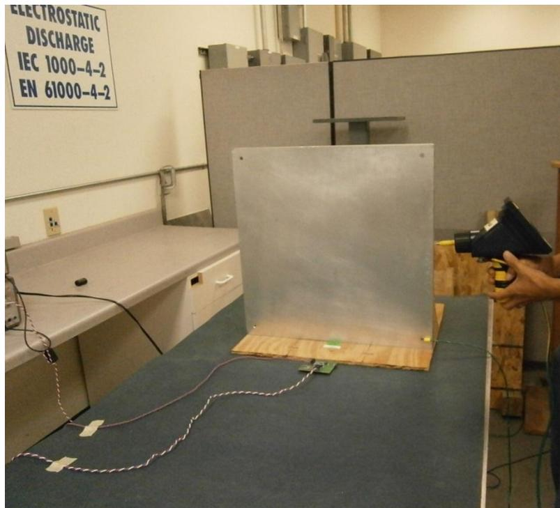
Figure B-2: 8kV ESD Vertical Contact Discharge
