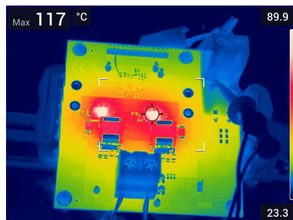
Figure 2-4. 48V IN , 50A Thermal Image With Fan
