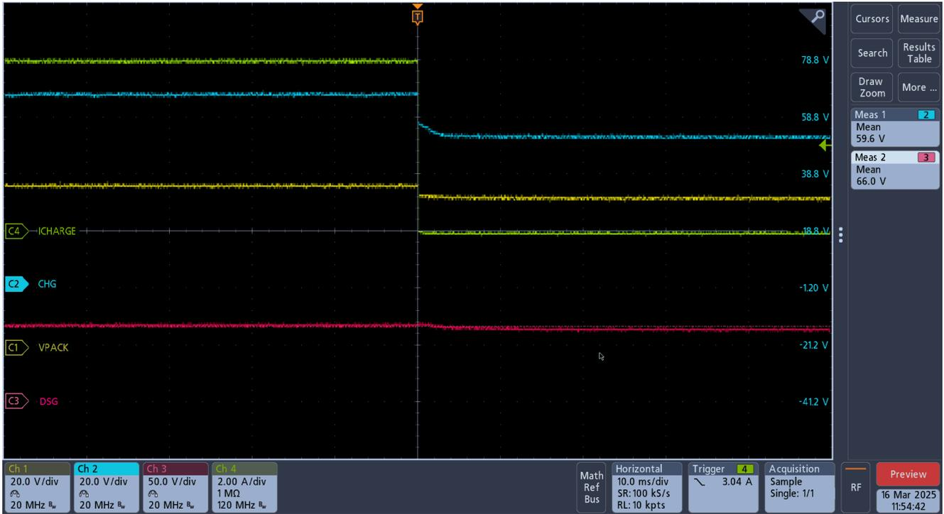
Figure 3-1. Overcurrent Protection at 6A During Charge
