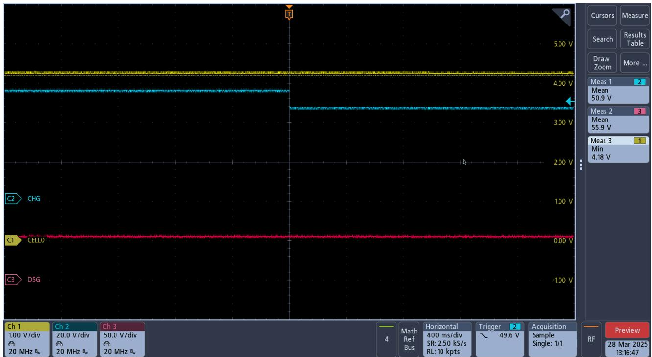
Figure 3-4. Cell Overvoltage Protection at 4.2V
