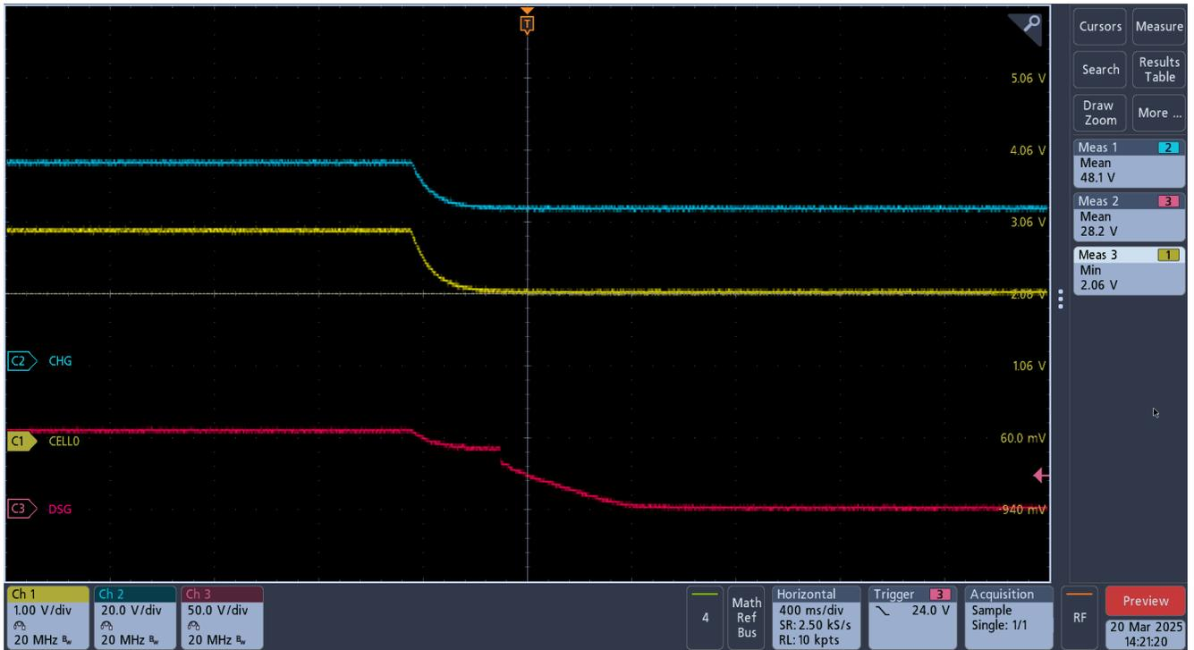
Figure 3-3. Cell Undervoltage Protection at 2.7V
