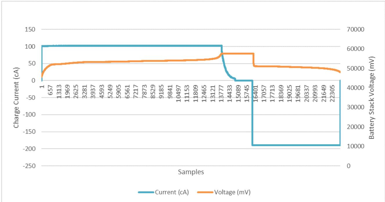
Figure 2-2. Battery Stack Voltage and Charge and Discharge Current
