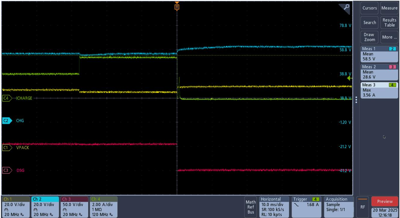
Figure 3-2. Overcurrent Protection at 3.5A During Discharge
