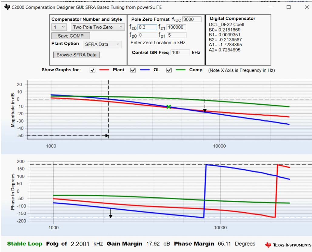
Figure 2-11. Compensator Bode Plot
