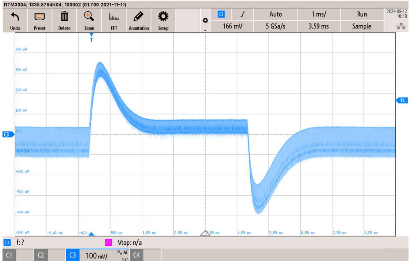
Figure 3-3. AC-Coupled Output Voltage, Output 1 (550mA) [Scale: 100mV-div, 1ms-div, 20MHz BW]
