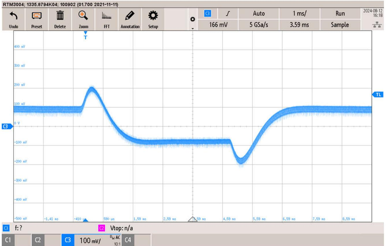
Figure 3-4. AC-Coupled Output Voltage, Output 2 (160mA) [Scale: 100mV-div, 1ms-div, 20MHz BW]
