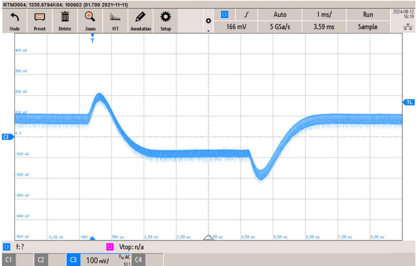
Figure 3-5. AC-Coupled Output Voltage, Output 3 (160mA) [Scale: 100mV/div, 1ms/div, 20MHz BW]
