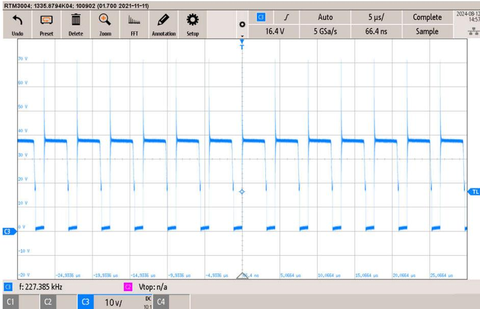
**Figure 3-1. DC-Coupled Switch Node Voltage (Scale: 10V-div, 5µs-div)**
