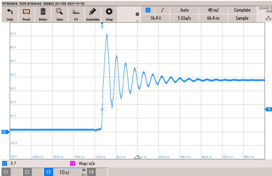
**Figure 3-2. DC-Coupled Switch Node Voltage (Scale: 10V-div, 40ns-div)**
