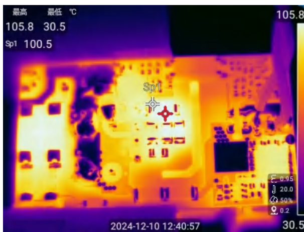
Figure 2-21. 90VAC, Dual Port, 45W (15V, 3A) +20W (9V, 2.25A), Full Load, PCB Bottom Side
