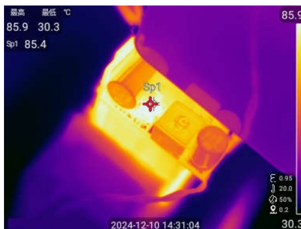
Figure 2-14. 90VAC, Single Port, 20V, Full Load, DCDC Board
