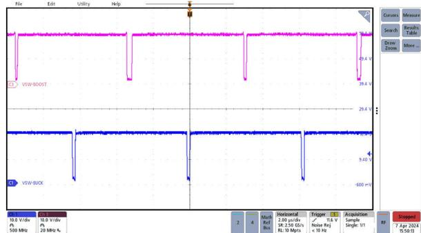
**Figure 3-10. Buck-Boost Mode Switching Node Waveform**
