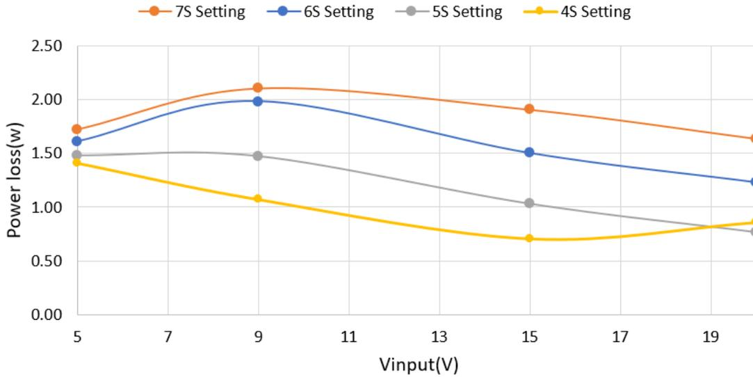
**Figure 2-2. Power Loss Across V<sub>IN</sub> and Battery Voltage**
