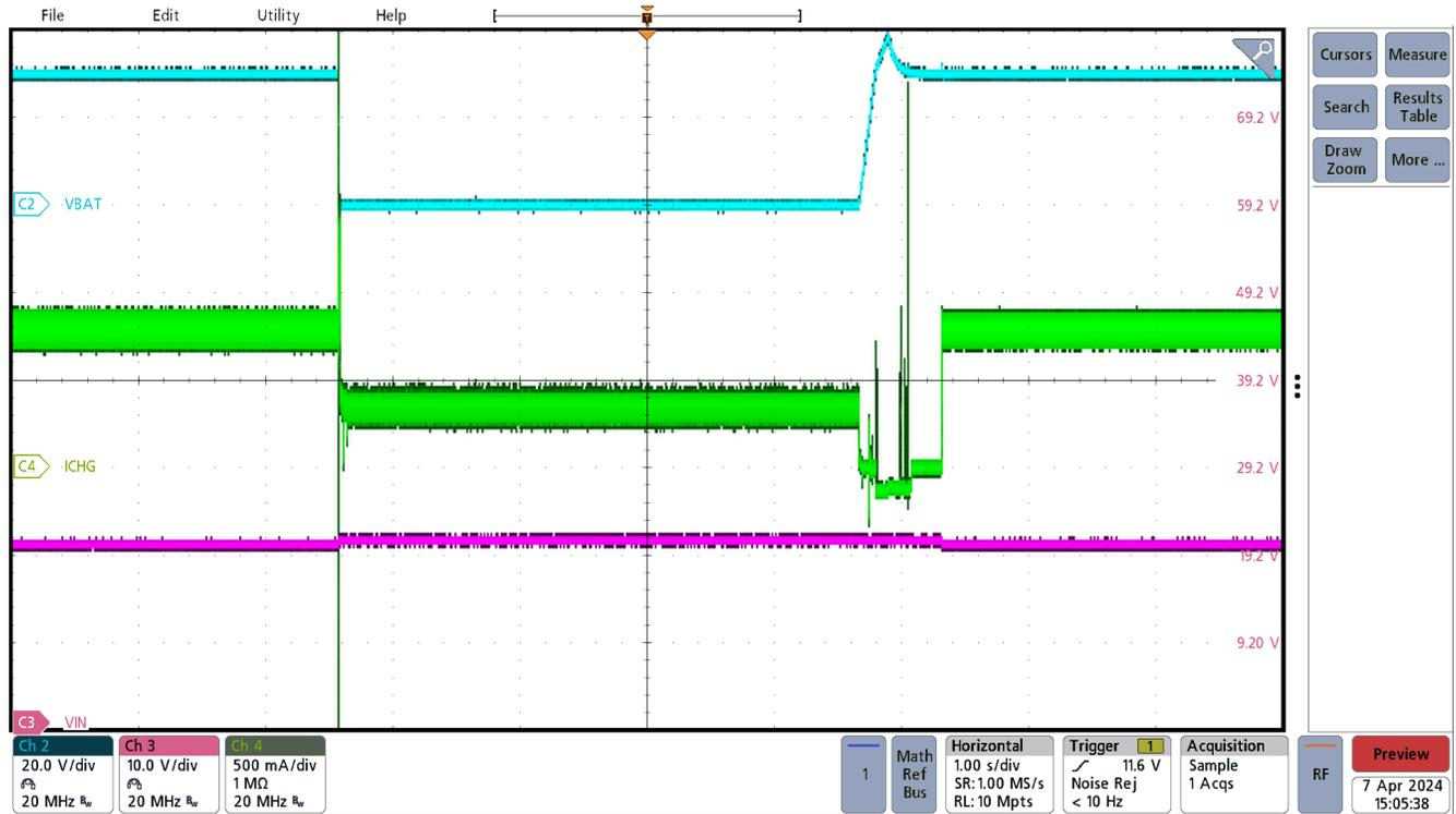
Figure 3-11. Short-Circuit Protection and Recovery at 20V<sub>IN</sub> and 30V Battery Condition
