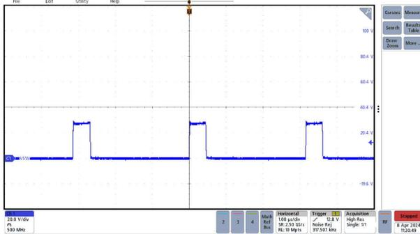
**Figure 3-5. Boost Mode Switching Node Waveform**
