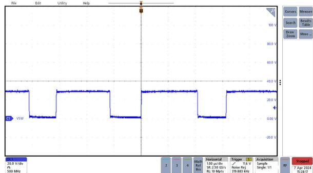
**Figure 3-8. Boost Mode Switching Node Waveform**
