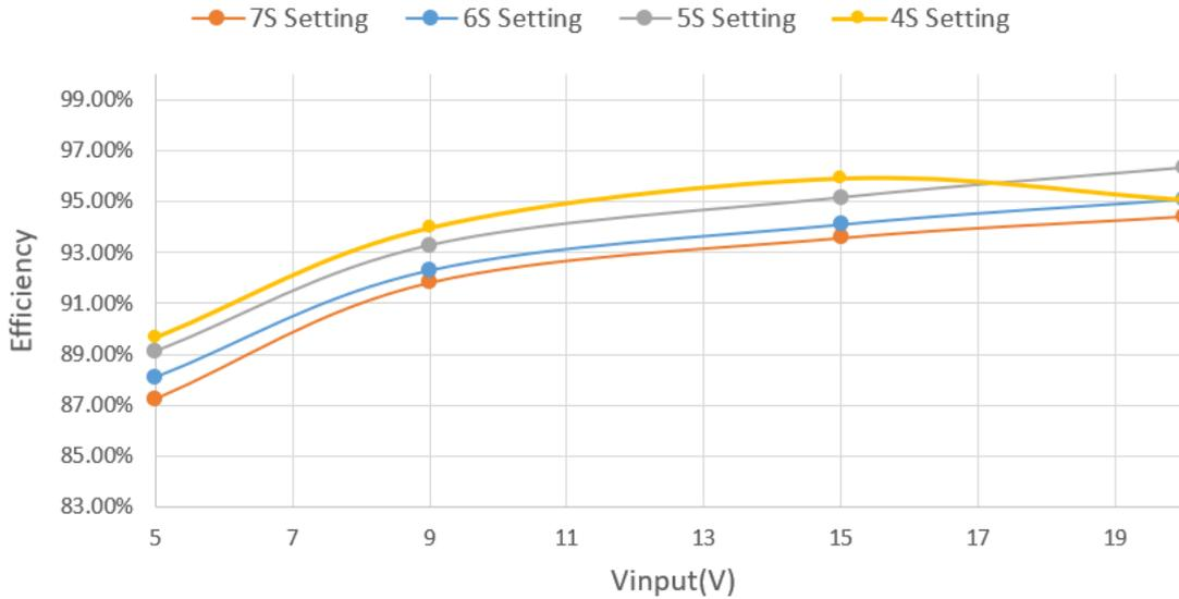
**Figure 2-1. Efficiency Across Input Voltage and Battery Voltage**
