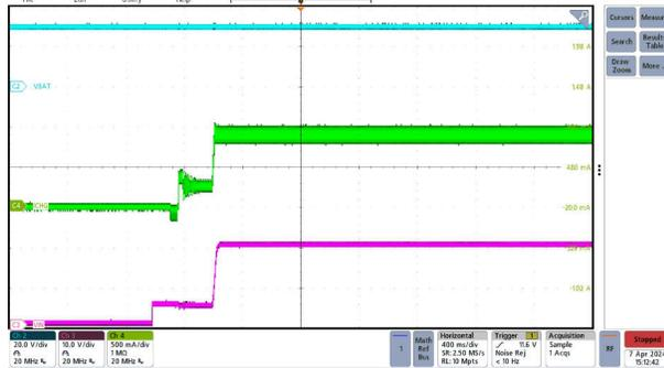
**Figure 3-1. 20V, 3A Input Source to 7S Battery 30V, 900mA Charge**
