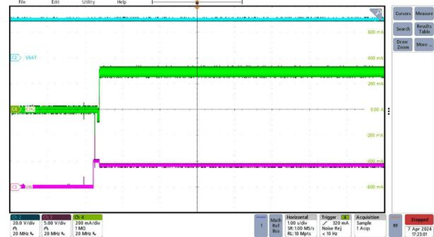
**Figure 3-4. 5V, 2A Non-USB PD Input Source Charge 7S Battery 30V, Input Voltage Dynamic Power Management Works, Charge Current Reduced to 300mA**
