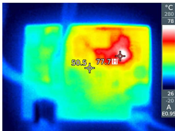
**Figure 2-4. 5V<sub>IN</sub> to 30V Battery Charge Thermal**
