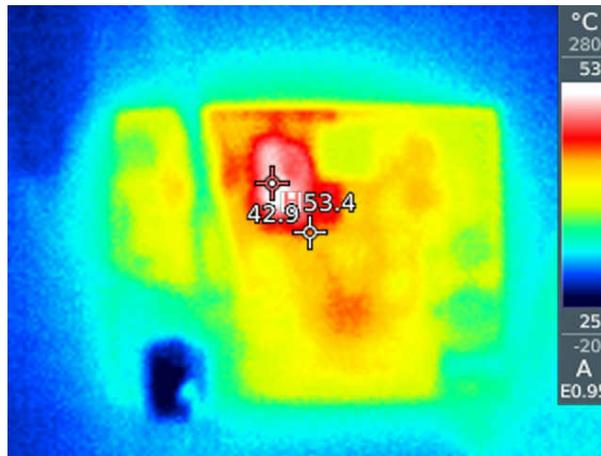
Figure 2-8. 20V<sub>IN</sub> to 30V Battery Short Circuit Thermal Test
