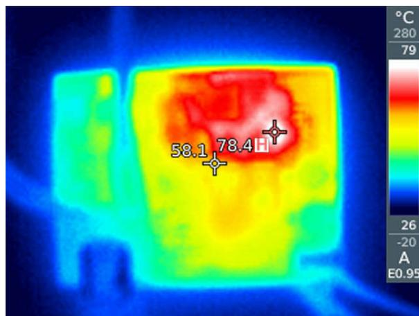
**Figure 2-6. 15V<sub>IN</sub> to 30V Battery Charge Thermal**
