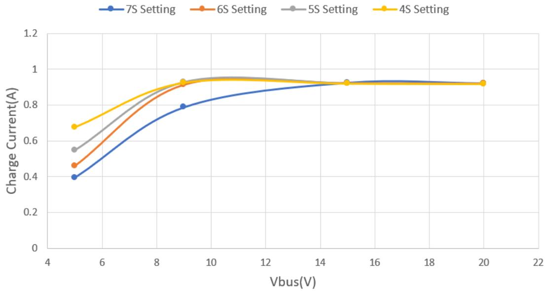
**Figure 2-3. Charge Current Across  $V_{IN}$  and Battery Voltage**
