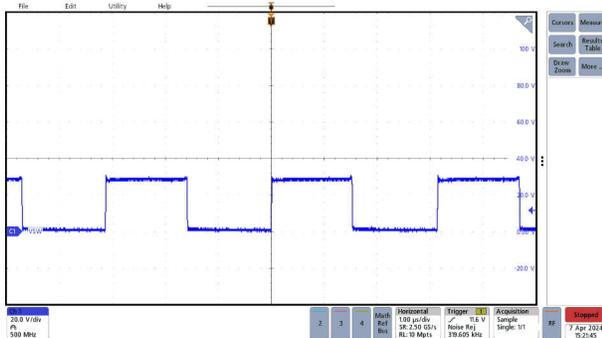
**Figure 3-7. Boost Mode Switching Node Waveform**
