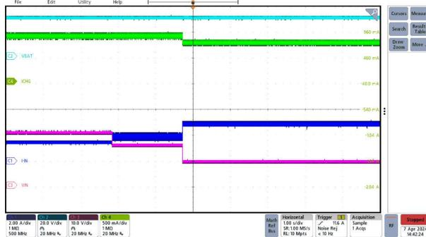
**Figure 3-3. Input Source Voltage Transition Down From 20V to 15V, 9V Charge 7S Battery 30V, 900mA**
