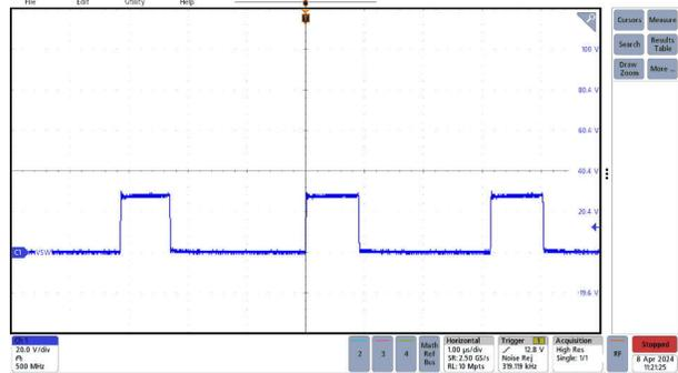
**Figure 3-6. Boost Mode Switching Node Waveform**
