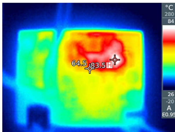
**Figure 2-5. 9V<sub>IN</sub> to 30V Battery Charge Thermal**
