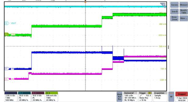
**Figure 3-2. Input Source Voltage Transition up From 5V to 9V, 15V, 20V USB PD Source Charge 7S Battery 30V, 900mA**
