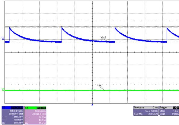
Figure 3-10. Output Voltage Ripple, 24V Input, No Load, PFM Mode
