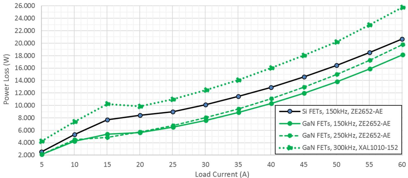
Figure 3-30. Power Loss Comparison Between Silicon and GaN FET Solutions at Varying Switching Frequencies (5A to 60A Load)
