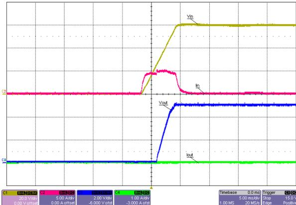
Figure 3-26. Start-Up Into No Load, 60V Input
