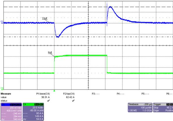
Figure 3-19. Load Transient Response, 24V Input, 30A-to-60A Load Step
