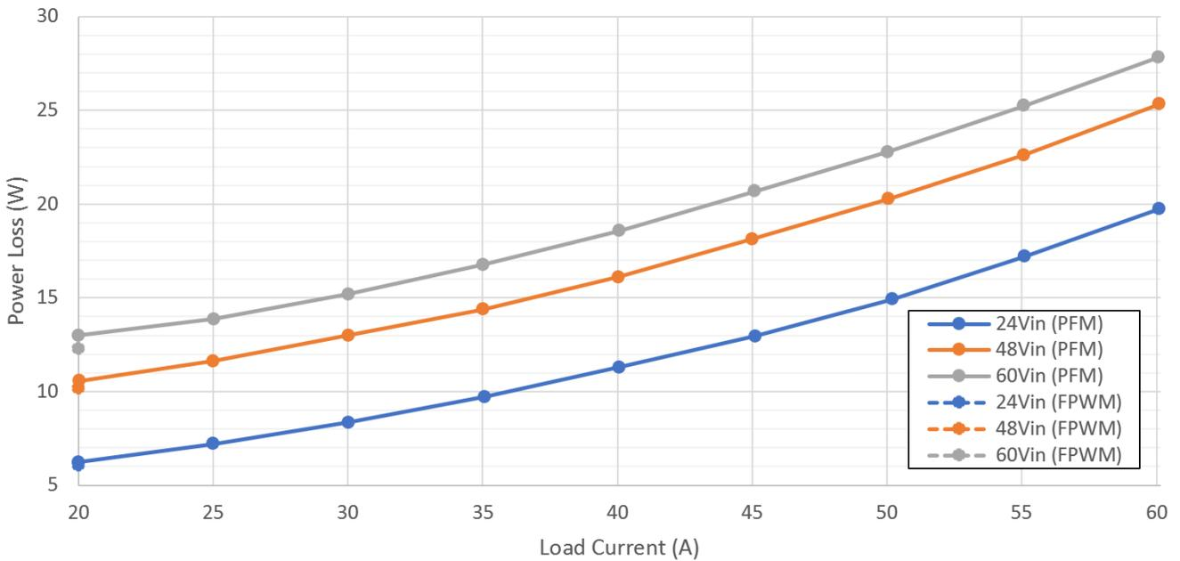
**Figure 2-8. Power Loss (20A to 60A Load)**
