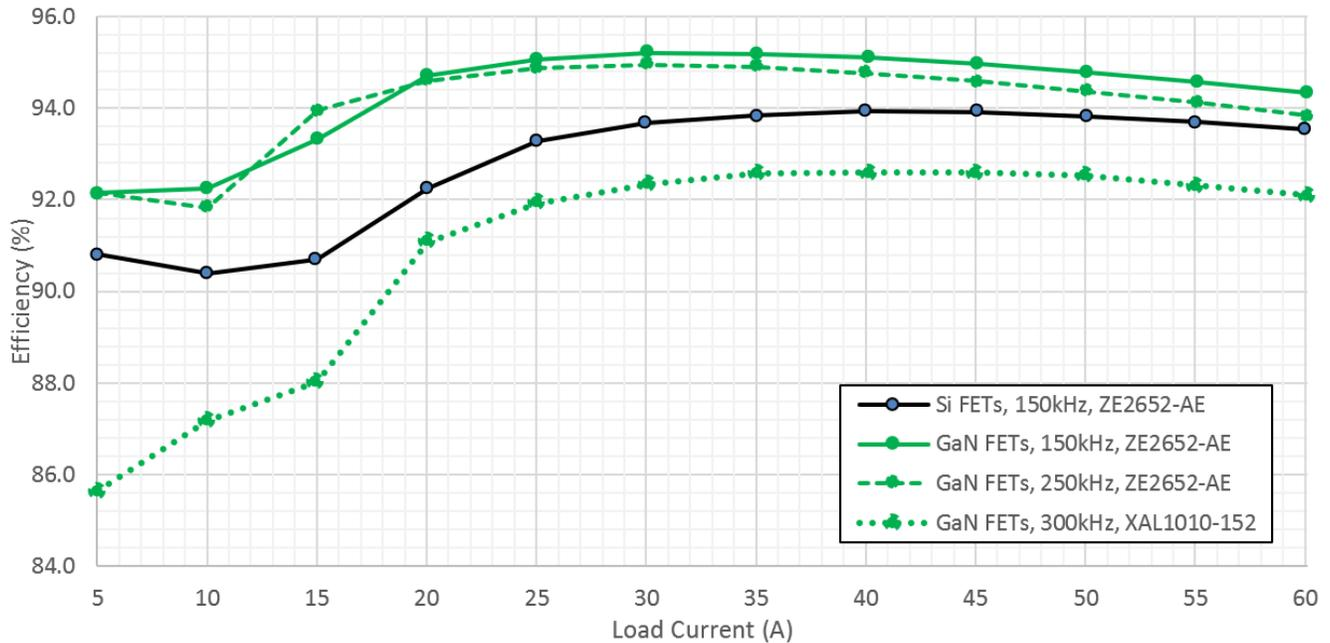
Figure 3-29. Efficiency Comparison Between Silicon and GaN FET Solutions at Varying Switching Frequencies (5A to 60A Load)
