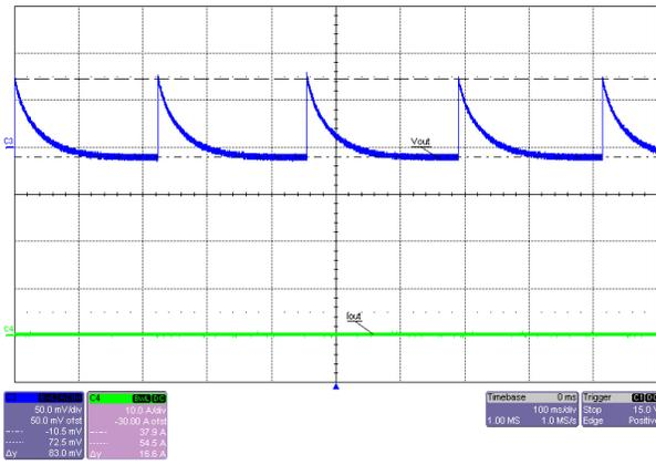
Figure 3-13. Output Voltage Ripple, 48V Input, No Load, PFM Mode
