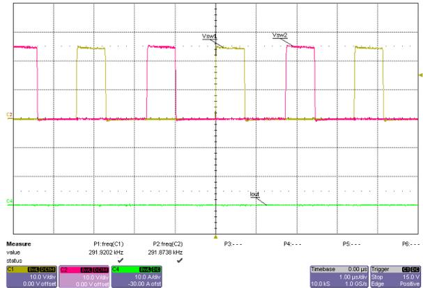
**Figure 3-2. Switch Node Voltages, 24V Input, No Load, FPWM Mode**
