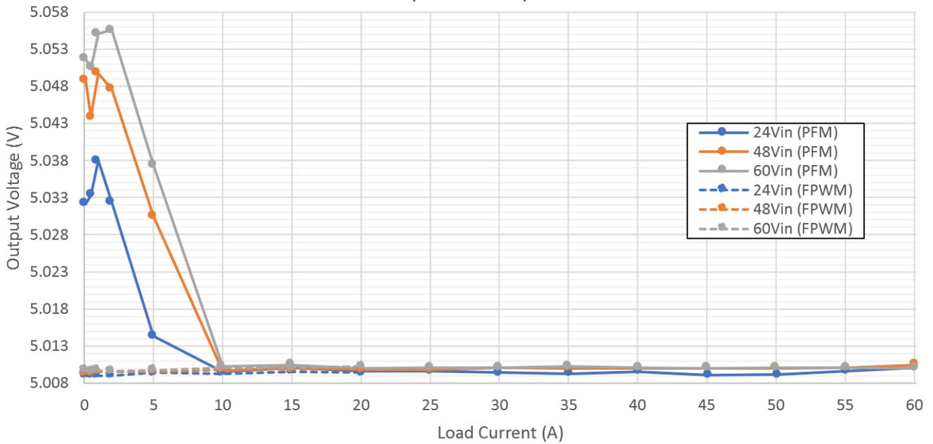
Figure 2-9. Load Regulation (0A to 60A Load)
