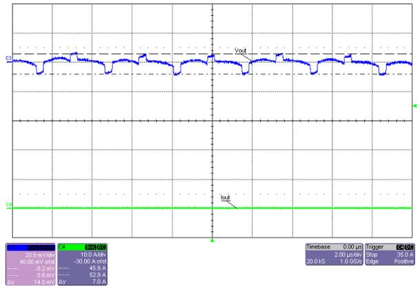
Figure 3-14. Output Voltage Ripple, 48V Input, No Load, FPWM Mode
