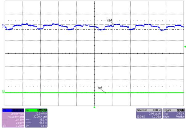
Figure 3-11. Output Voltage Ripple, 24V Input, No Load, FPWM Mode
