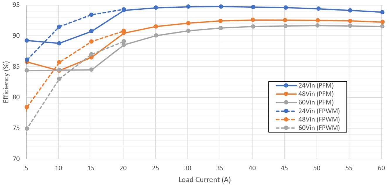
Figure 2-3. Efficiency (5A to 60A)
