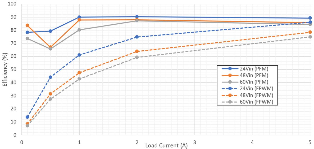
Figure 2-2. Efficiency (0A to 5A)
