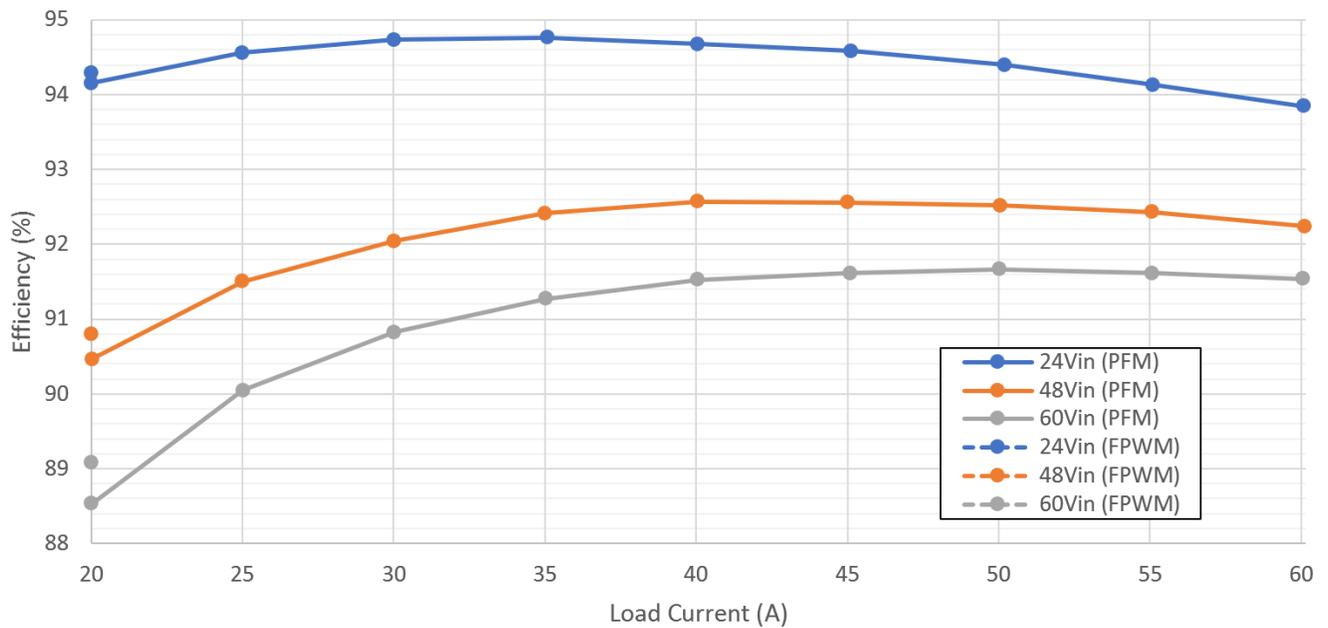
Figure 2-4. Efficiency (20A to 60A)
