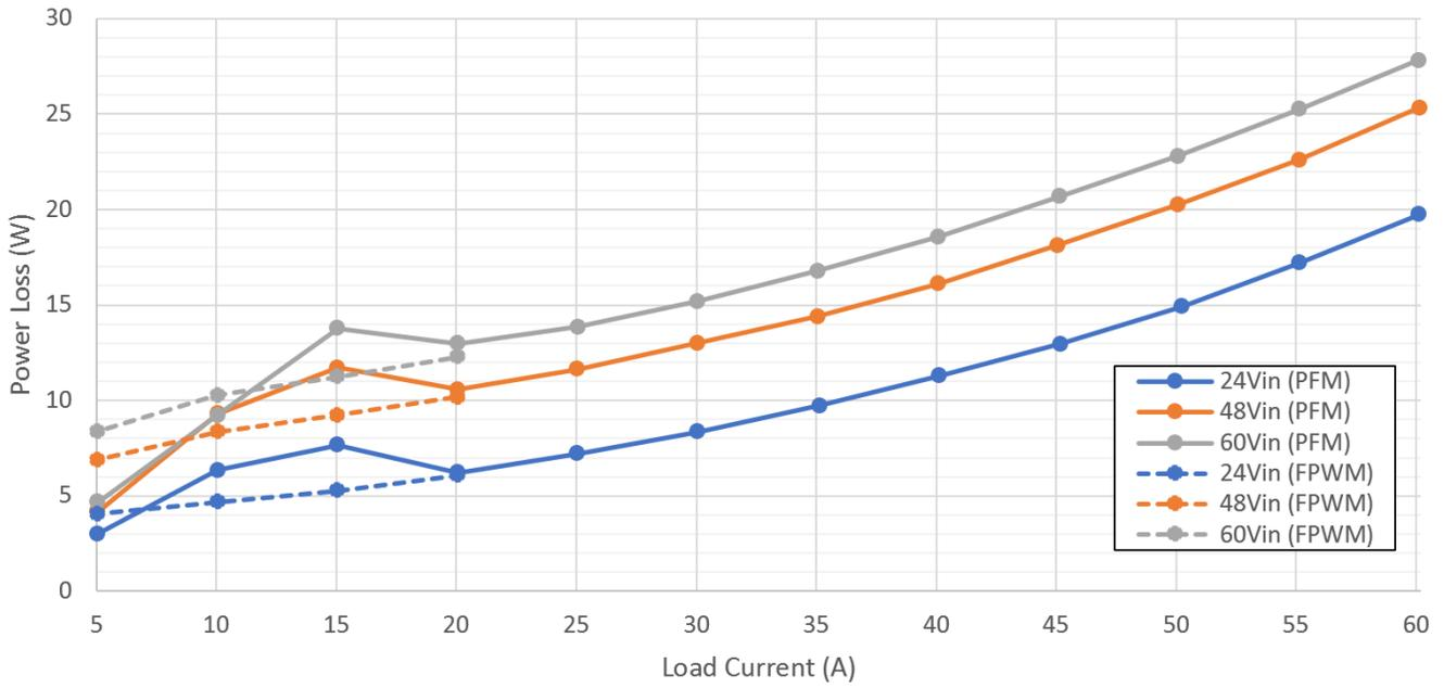
**Figure 2-7. Power Loss (5A to 60A Load)**
