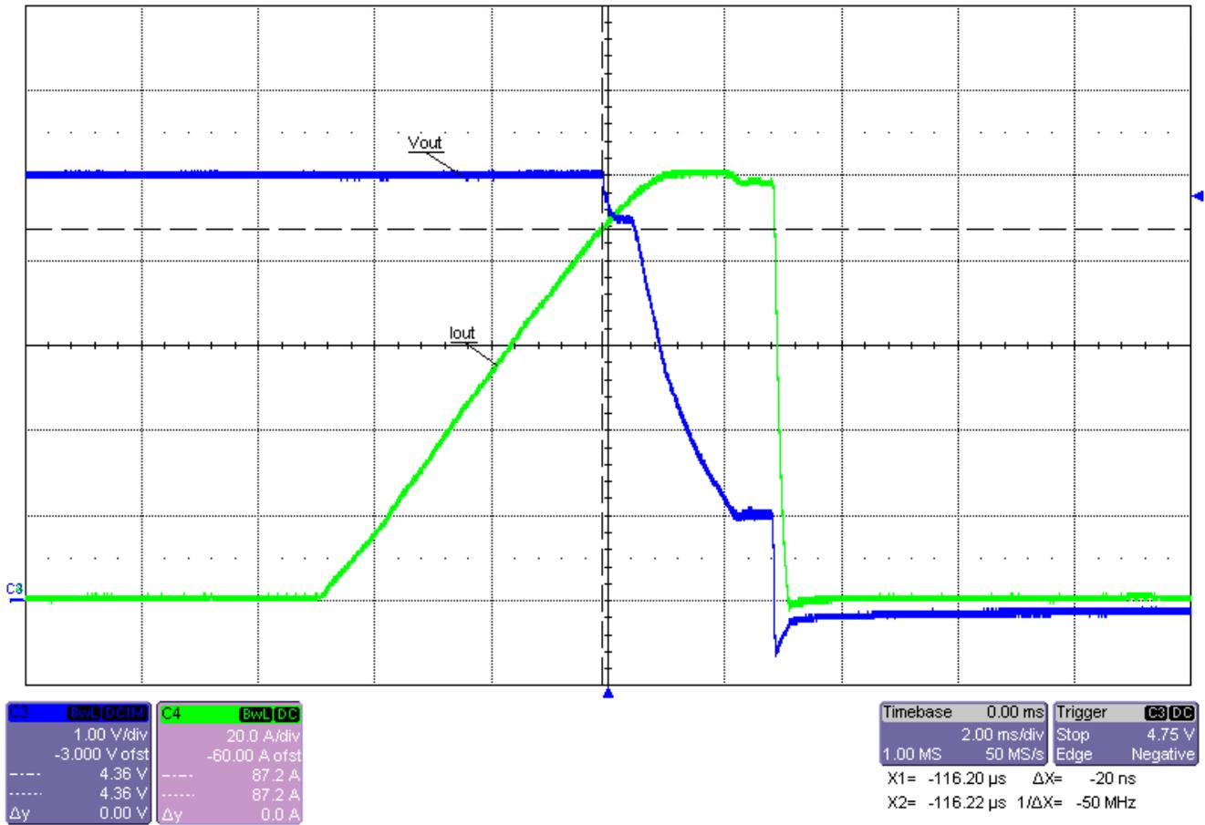
Figure 3-28. Overcurrent Protection at 48V Input
