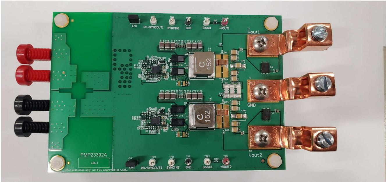
Figure 2-14. Top of PMP23392 Board
