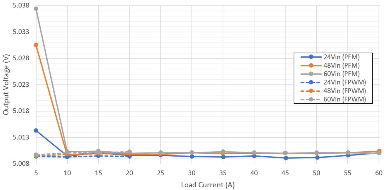
Figure 2-11. Load Regulation (5A to 60A Load)
