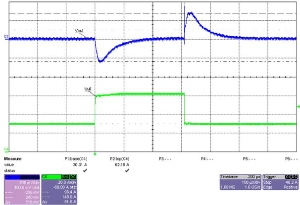
Figure 3-20. Load Transient Response, 48V Input, 30A-to-60A Load Step
