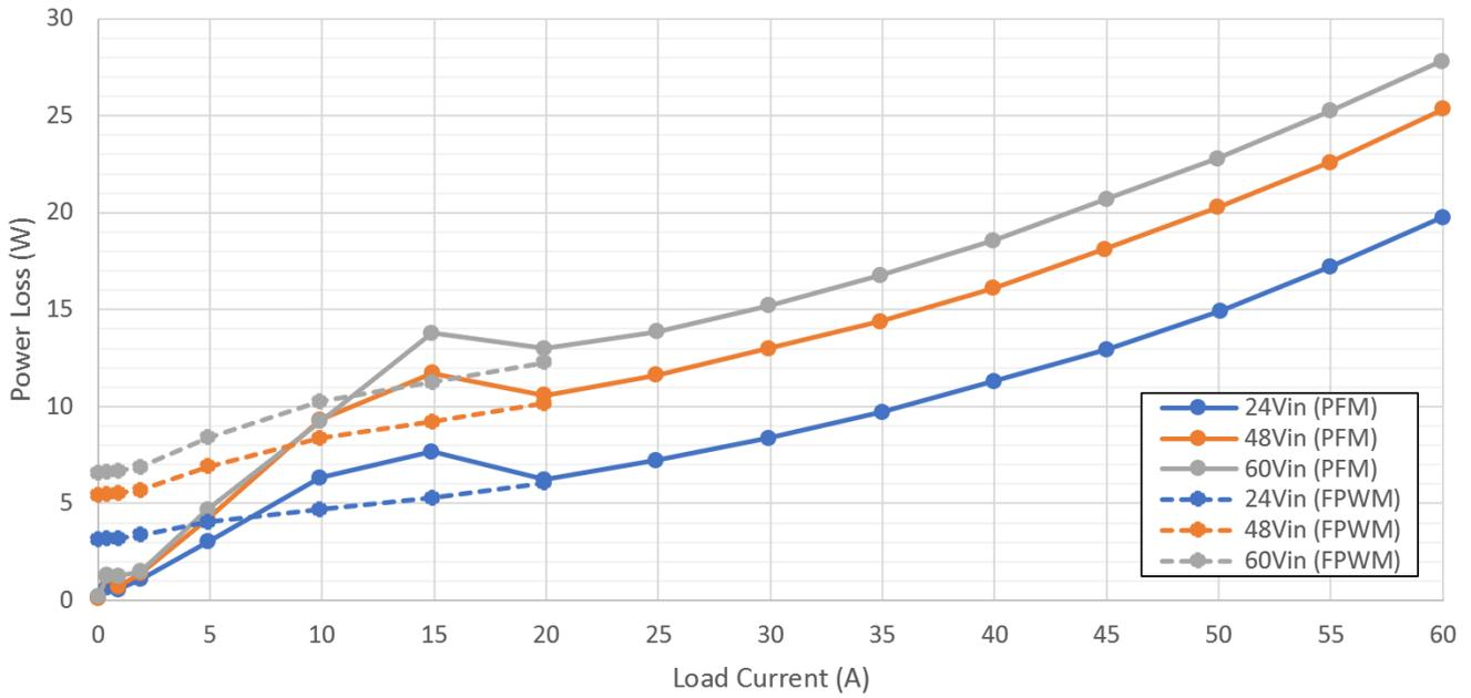
Figure 2-5. Power Loss (0A to 60A Load)
