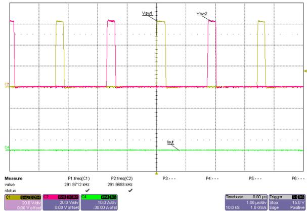
Figure 3-8. Switch Node Voltages, 60V Input, No Load, FPWM Mode
