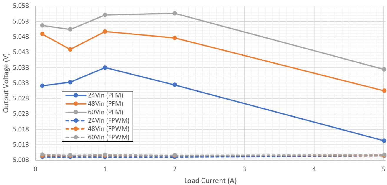
Figure 2-10. Load Regulation (0A to 5A Load)
