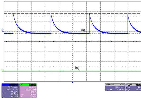
Figure 3-16. Output Voltage Ripple, 60V Input, No Load, PFM Mode
