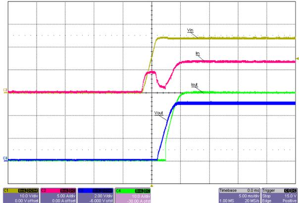
Figure 3-23. Start-Up Into 30A Constant-Resistance Load, 24V Input
