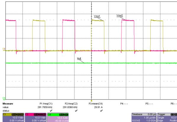
**Figure 3-3. Switch Node Voltages, 24V Input, 30A Load**
