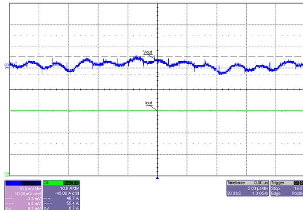
Figure 3-12. Output Voltage Ripple, 24V Input, 30A Load
