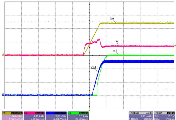
Figure 3-25. Start-Up Into 30A Constant-Resistance Load, 48V Input
