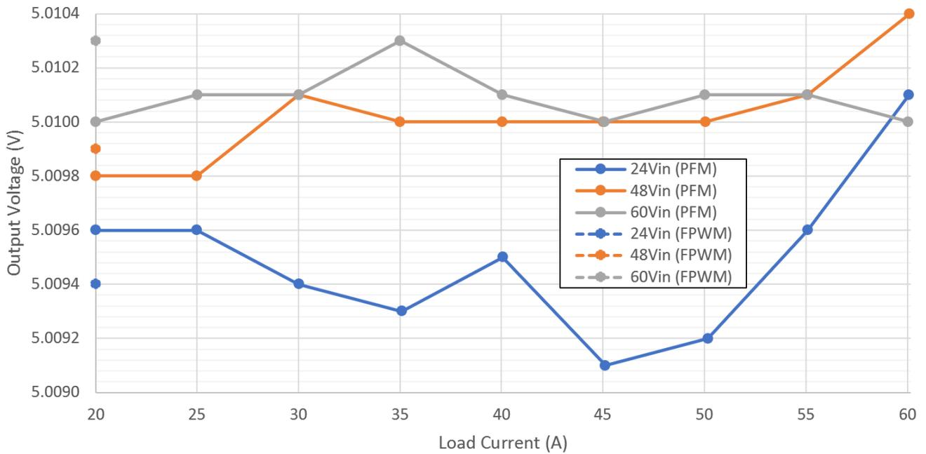
Figure 2-12. Load Regulation (20A to 60A Load)
