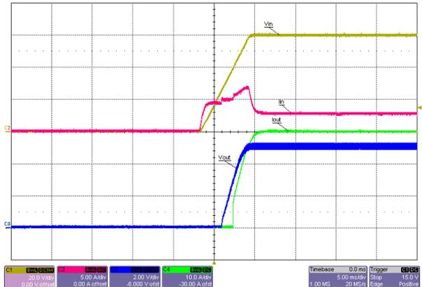
Figure 3-27. Start-Up Into 30A Constant-Resistance Load, 60V Input
