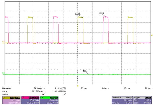
Figure 3-5. Switch Node Voltages, 48V Input, No Load, FPWM Mode
