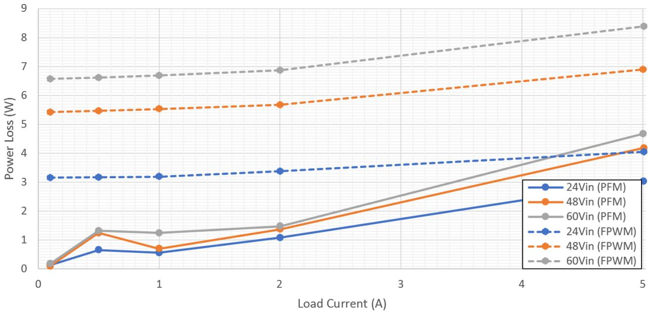
Figure 2-6. Power Loss (0A to 5A Load)
