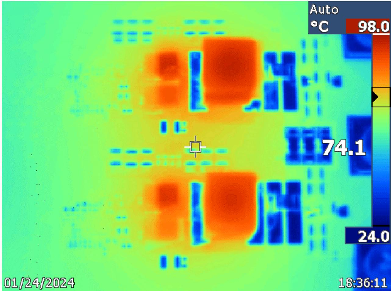
Natural convection (that is, no airflow); ambient at room temperature; thermal equilibrium reached
