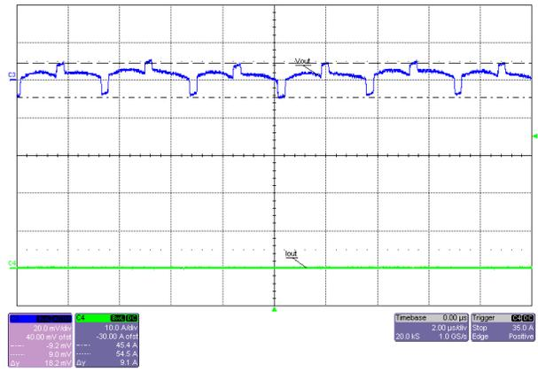
Figure 3-17. Output Voltage Ripple, 60V Input, No Load, FPWM Mode
