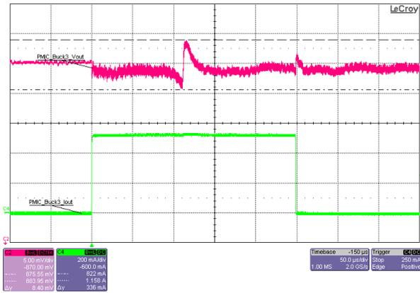
**Figure 3-32. GTAVCC Rail Load Transient Response (PMIC\_Buck3), at 5V<sub>IN</sub>, 0.88V<sub>OUT</sub>, 0A-to-0.49A (that is, 0%-to-70%) Load Step, PFM Mode**
