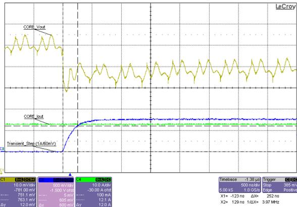
**Figure 3-26. VCCINT - Core Rail Buck Converter Load Transient Response, Load Step Rising Slew Rate, at 5V<sub>IN</sub>, 12.8A-to-25.6A (that is, 33%-to-66%) Load Step (Slew Rate  $\approx$  40A/ $\mu$ s)**
