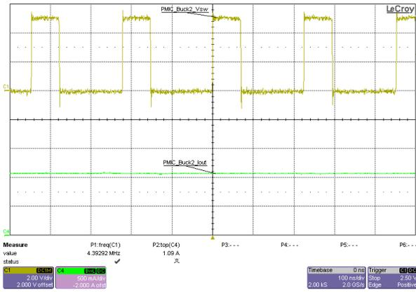
Figure 3-7. VCCAUX Rail Switch Node Voltage (PMIC\_Buck2), 5V Input, 1.5V<sub>OUT</sub>, 1.1A Load
