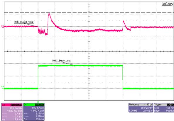
**Figure 3-34. GTAVTT Rail Load Transient Response (PMIC\_Buck4), at 5V<sub>IN</sub>, 1.2V<sub>OUT</sub>, 0A-to-0.91A (that is, 0%-to-70%) Load Step, PFM Mode**
