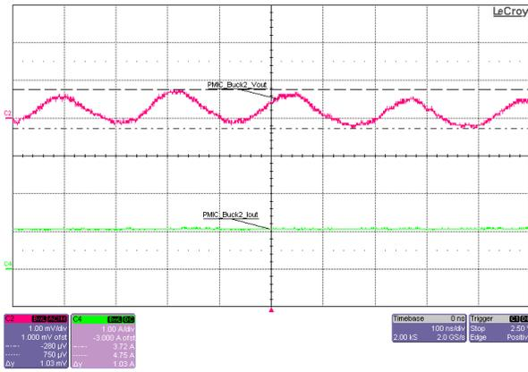
Figure 3-18. VCCAUX Output Voltage Ripple (PMIC\_Buck2), 5V Input, 1.5V Output, 1.1A Load
