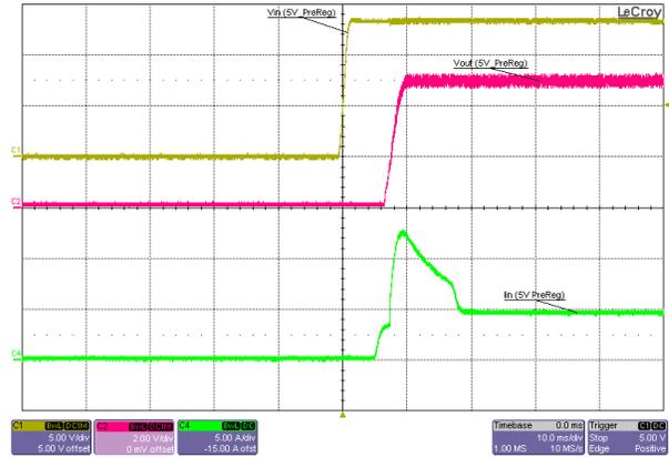
Figure 3-41. 5V Pre-Regulator Start-Up, 13.5V Input, 12A Constant-Current eLoad
