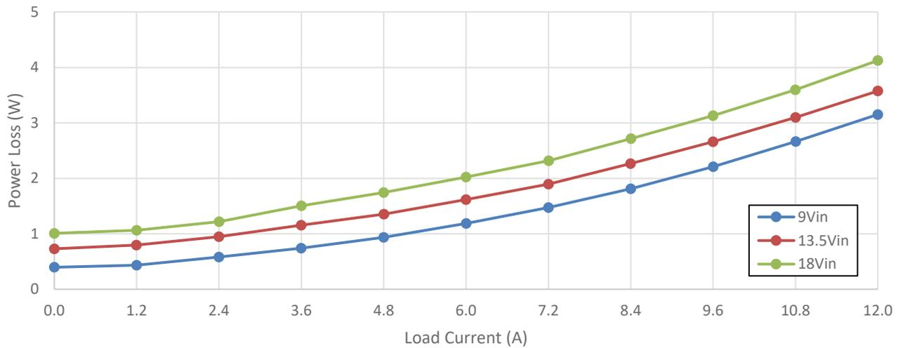
Figure 2-2. 5V Pre-Regulator Buck Power Loss
