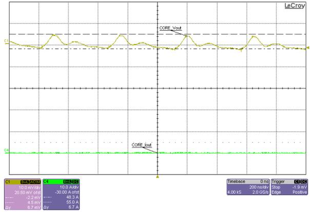
Figure 3-13. VCCINT Rail Output Voltage Ripple, 5V Input, 0.8V Output, No Load
