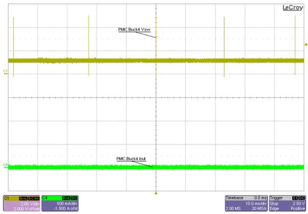
Figure 3-10. GTAVTT Rail Switch Node Voltage (PMIC\_Buck4), 5V Input, 1.2V<sub>OUT</sub>, No Load, PFM Mode
