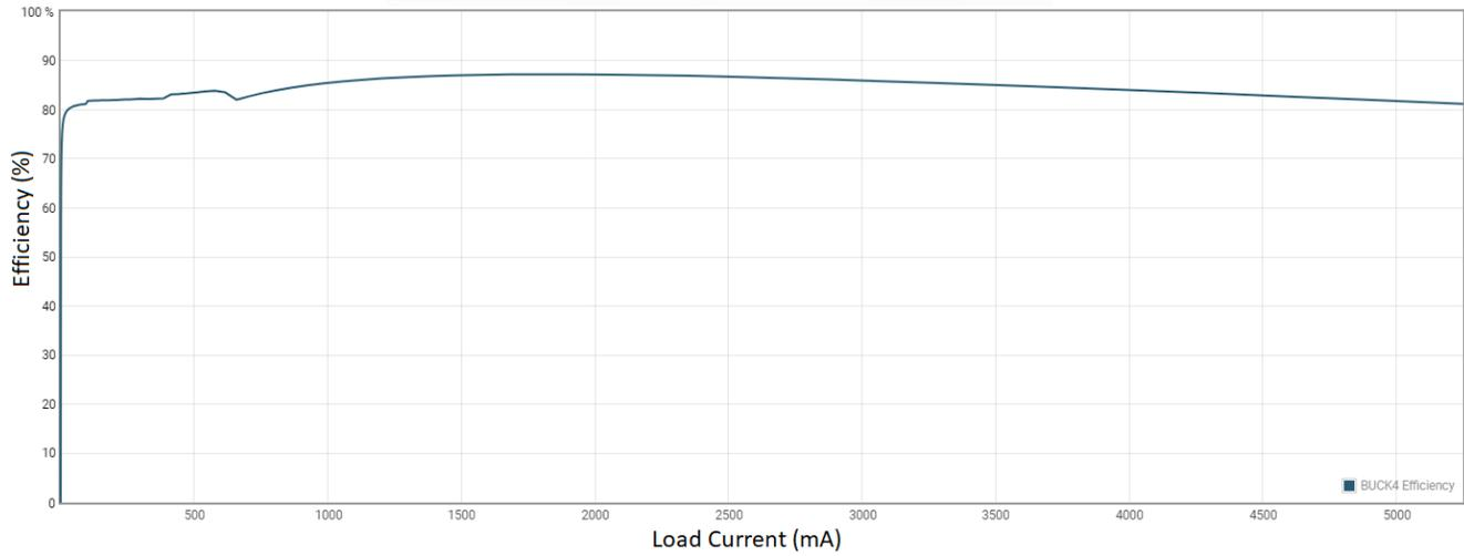
Figure 2-11. GTAVTT/MGTYAVTT Rail Efficiency (PMIC Buck 4),PFM Mode Operation
