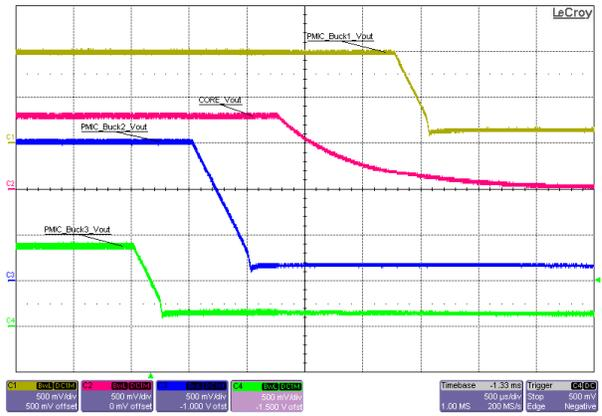
**Figure 3-53. Sequence Power-Down, Sequence Rails 4, 3, 2, and 1, PMIC nRSTOUT, No Load**
