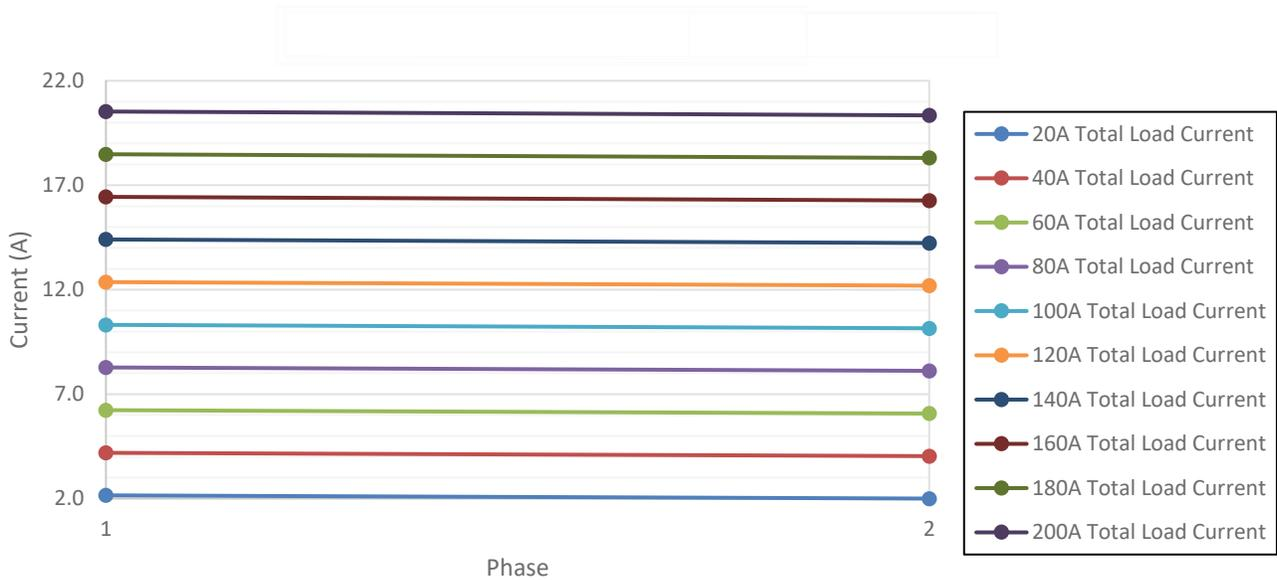
Figure 2-14. VCCINT- Core Rail Current Sharing Distribution
