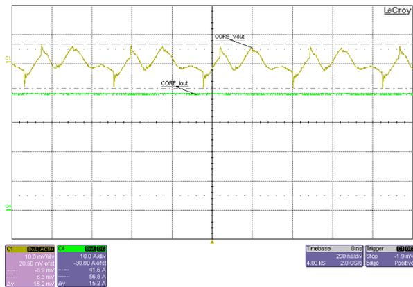
Figure 3-14. VCCINT Rail Output Voltage Ripple, 5V Input, 0.8V Output, 39A Load
