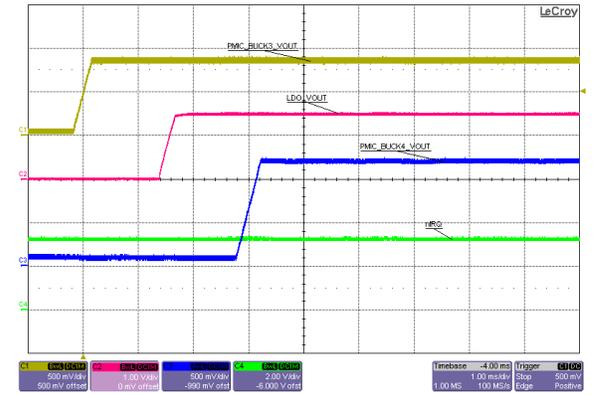
**Figure 3-55. Sequence Power-Up, Sequence Rails 4, 5, and 6, Discrete Vsupervisor nIRQ, No Load**
