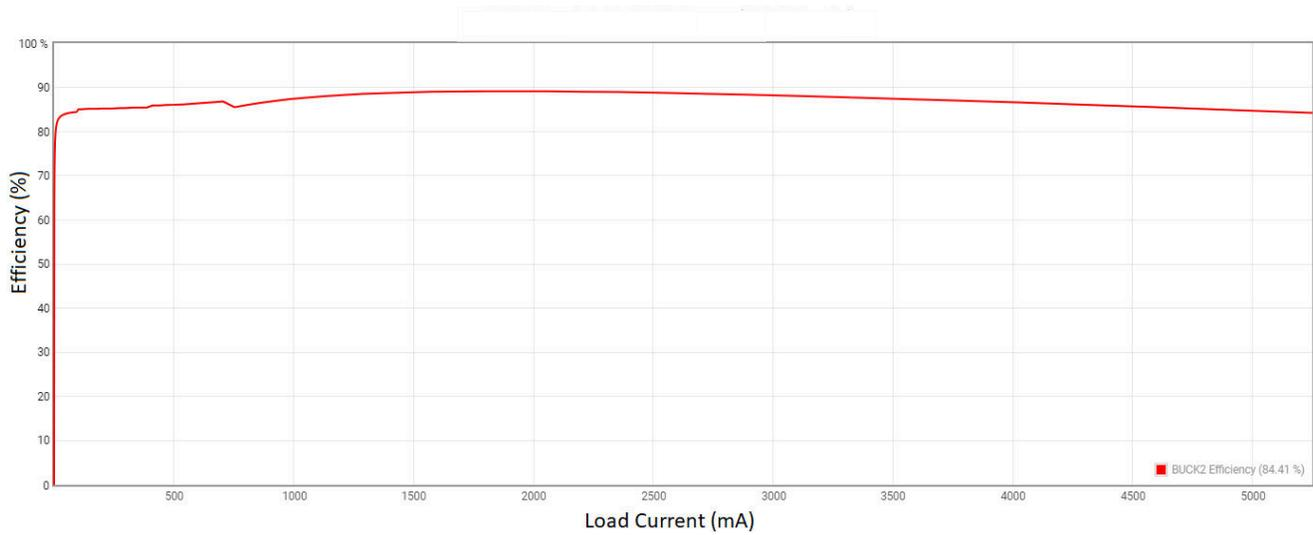
**Figure 2-7. VCCAUX Rail Efficiency (PMIC Buck 2), PFM Mode Operation**
