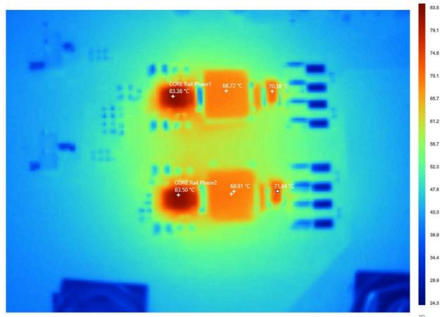
**Figure 2-16. VCCINT - Thermal Image, Core Rail, 5V Input, 0.8V Output at 39A Load**
