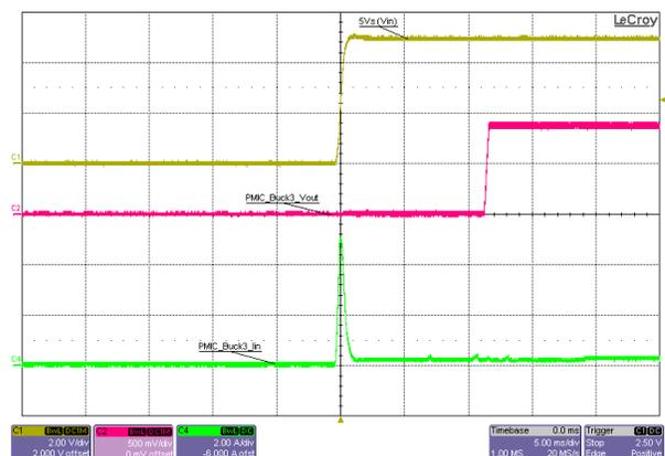
Figure 3-45. GTAVCC Rail Start-Up (PMIC\_Buck3), 5V Input, 0.7A Constant-Resistance eLoad
