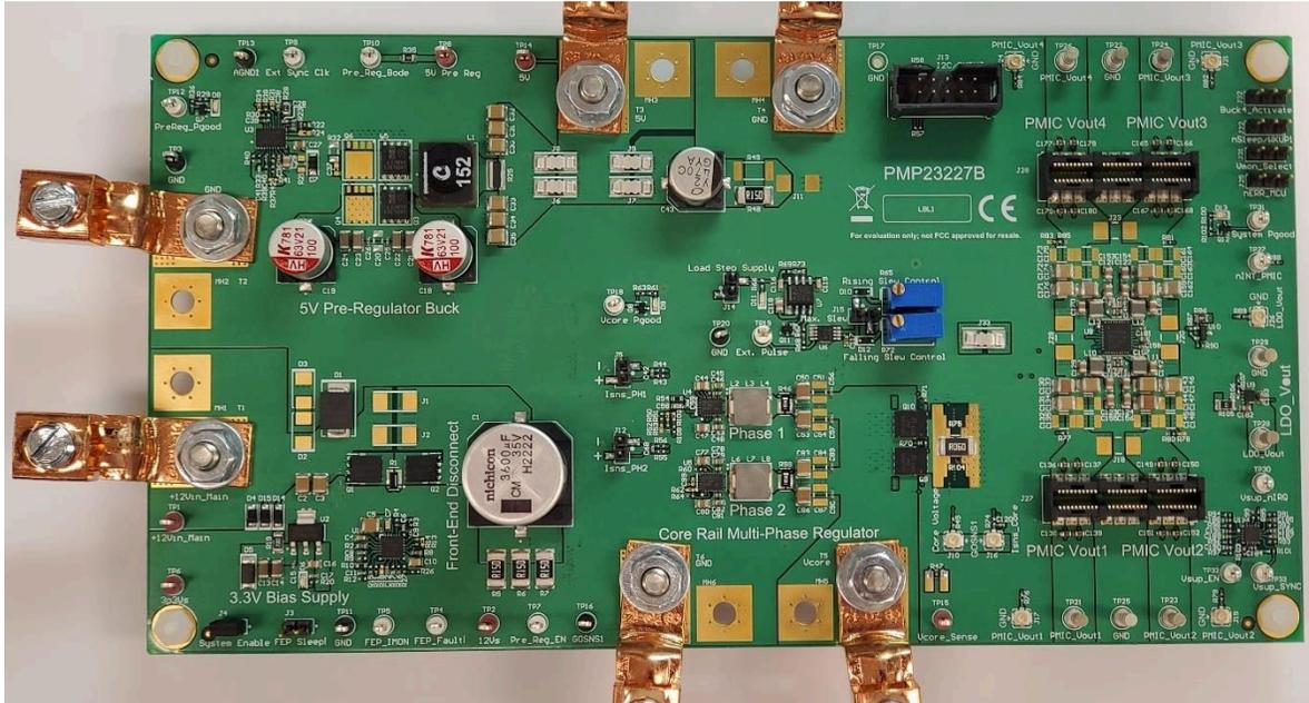
Figure 2-19. Top of PMP23227 Board
