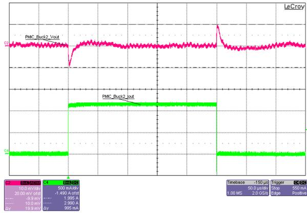
**Figure 3-31. VCCAUX Rail Load Transient Response (PMIC\_Buck2), at 5V<sub>IN</sub>, 1.5V<sub>OUT</sub>, 0A-to-1.1A (that is, 0%-to-100%) Load Step, FPWM Mode**
