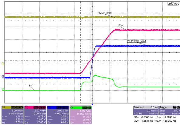
**Figure 3-61. Front-End Protection, OVLO Falling Enable, 5V Pre-Regulator Buck Output Loaded at 5A Load (FEP OVLO Enable Threshold  $\approx$  18.8V; 5V Pre-Regulator UVLO Enable Threshold  $\approx$  6.75V)**
