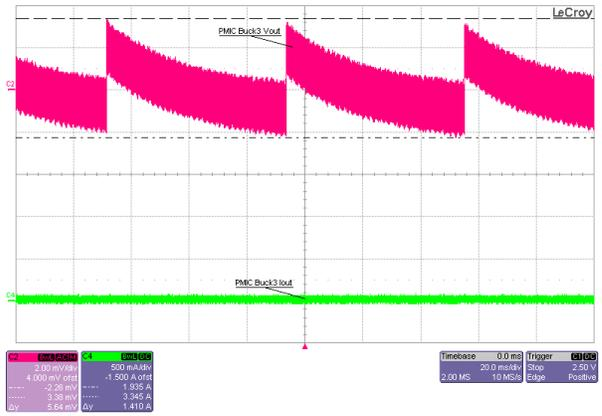
Figure 3-19. GTAVCC Output Voltage Ripple (PMIC\_Buck3), 5V Input, 0.88V Output, No Load, PFM Mode
