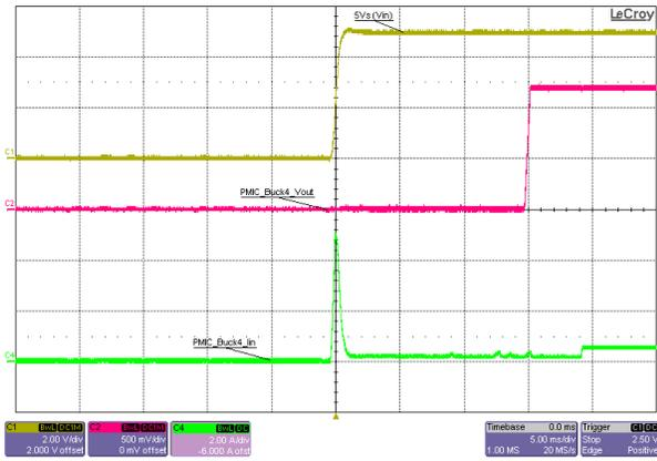
**Figure 3-46. GTAVTT Rail Start-Up (PMIC\_Buck4), 5V Input, 1.3A Constant-Resistance eLoad**
