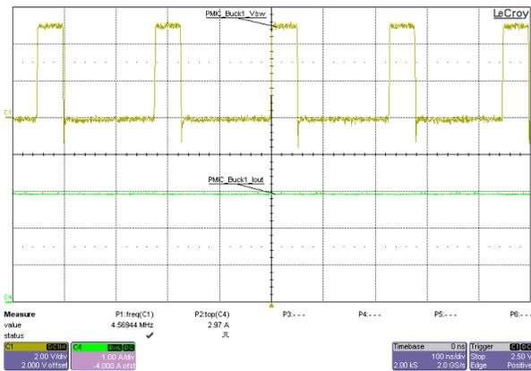
Figure 3-5. VCCO Rail Switch Node Voltage (PMIC\_Buck1), 5V Input, 1.0V<sub>OUT</sub>, 3A Load
