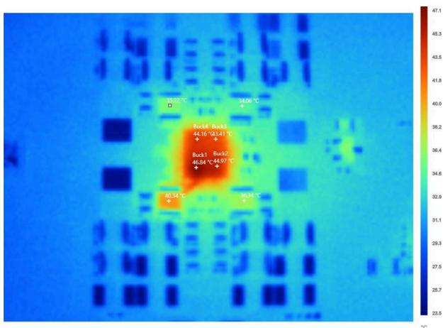
**Figure 2-17. VCCO, VCCAUX, GTAVCC, GTAVTT - Thermal Image, PMIC, 5V Input**
