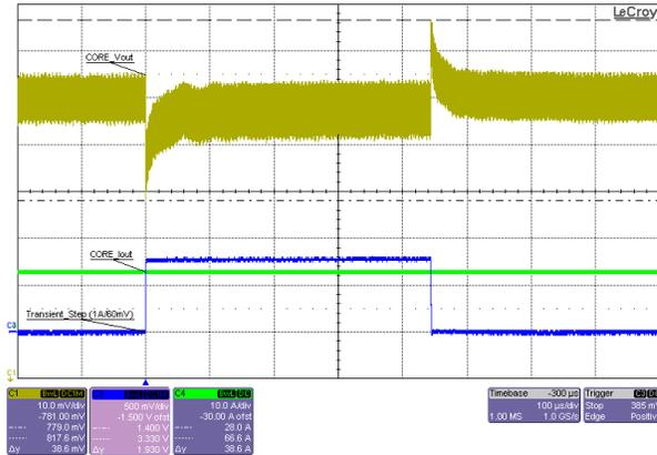
**Figure 3-25. VCCINT - Core Rail Buck Converter Load Transient Response, at 5V<sub>IN</sub>, 12.8A-to-25.6A (that is, 33%-to-66%) Load Step**
