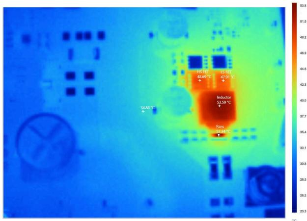
**Figure 2-15. Thermal Image, Pre-Regulator Buck and FEP, 13.5V Input, 5V Output at 12A Load**
