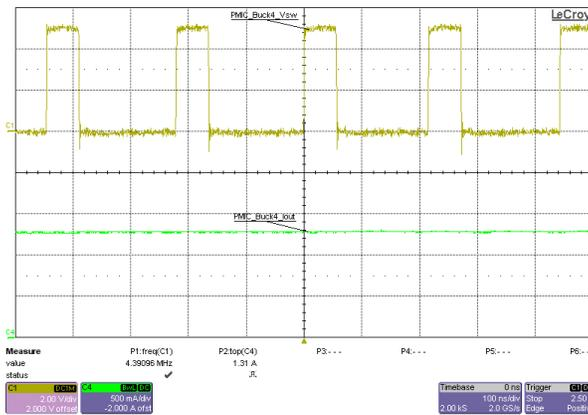
Figure 3-11. GTAVTT Rail Switch Node Voltage (PMIC\_Buck4), 5V Input, 1.2V<sub>OUT</sub>, 1.3A Load
