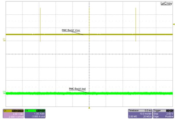
Figure 3-4. VCCO Rail Switch Node Voltage (PMIC Buck1), 5V Input, 1.0V<sub>OUT</sub>, No Load, PFM Mode
