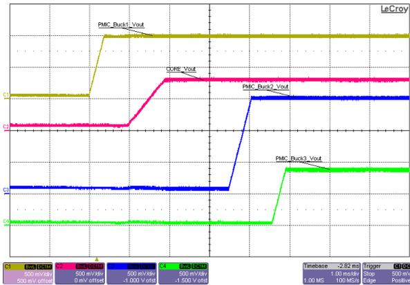
**Figure 3-50. Sequence Power-Up, Sequence Rails 1, 2, 3, and 4, PMIC nRSTOUT, No Load**
