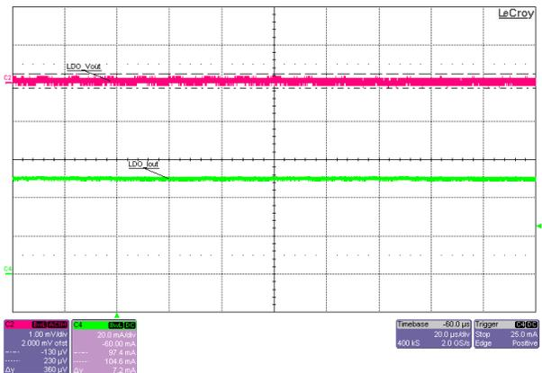
Figure 3-23. GTAVCCAUX Output Voltage Ripple (LDO), 5V Input, 1.5V Output, 0.05A Load
