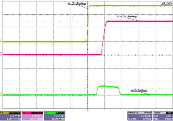
Figure 3-40. 5V Pre-Regulator Start-Up, 13.5V Input, No Load
