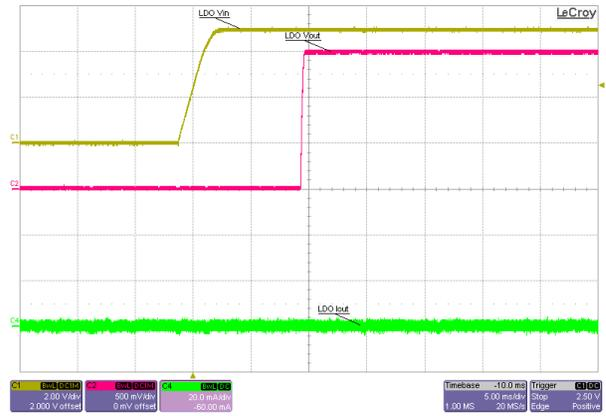
**Figure 3-47. GTAVCCAUX Rail Start-Up (LDO), 5V Input, No Load**
