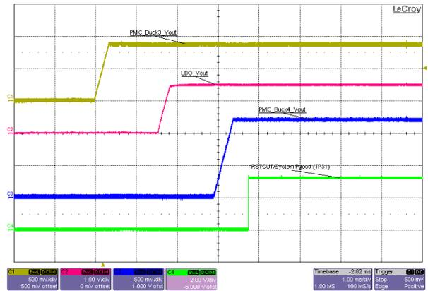
**Figure 3-51. Sequence Power-Up, Sequence Rails 4, 5, and 6, PMIC nRSTOUT, No Load**
