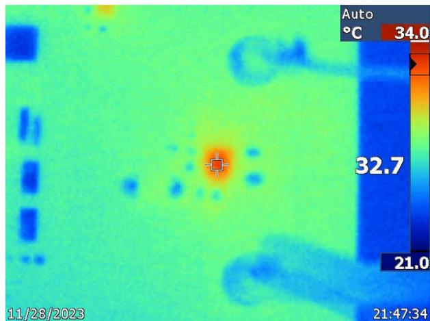
**Figure 2-18. GTAVCCAUX - Thermal Image, LDO Linear Regulator, 5V Input, 1.5V Output at 0.05A Load**
