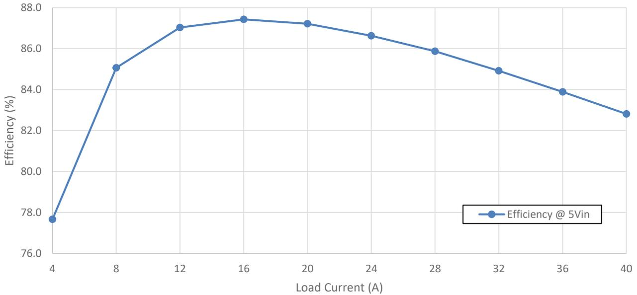
Figure 2-3. VCCINT/VCC SOC Efficiency
