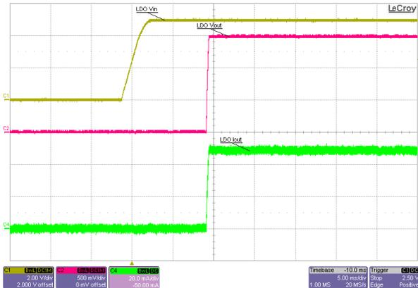
**Figure 3-48. GTAVCCAUX Rail Start-Up (LDO), 5V Input, 0.05A Resistor Load**
