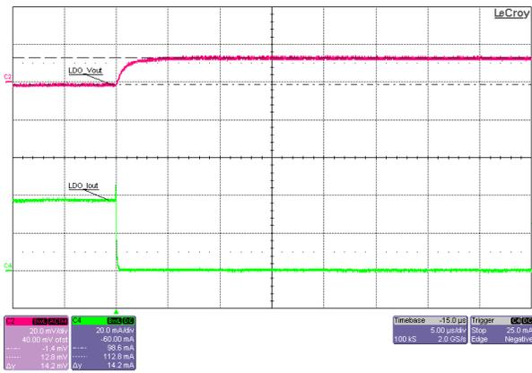
Figure 3-38. GTAVCCAUX Rail Load Transient Response (LDO), at 5V<sub>IN</sub>, 1.5V<sub>OUT</sub>, 0A-to-0.035A (that is, 0%-to-70%) Load Step, Overshoot
