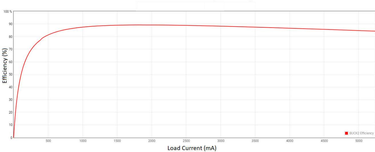
**Figure 2-8. VCCAUX Rail Efficiency (PMIC Buck 2), FPWM Mode Operation**
