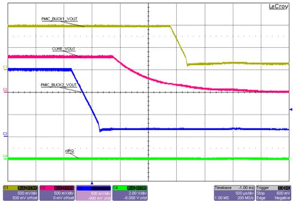
**Figure 3-57. Sequence Power-Down, Sequence Rails 4, 3, 2, and 1, Discrete Vsupervisor nIRQ, No Load**
