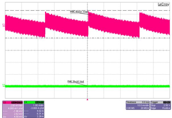
Figure 3-15. VCCO Output Voltage Ripple (PMIC\_Buck1), 5V Input, 1.0V Output, No Load, PFM Mode
