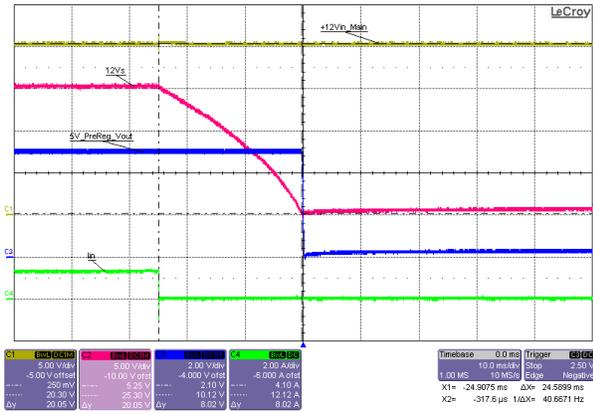
**Figure 3-60. Front-End Protection, OVLO Rising Disable, 5V Pre-Regulator Buck Output Loaded at 5A Load (FEP OVLO Disable Threshold  $\approx$  20.3V; 5V Pre-Regulator UVLO Disable Threshold  $\approx$  5.2V)**
