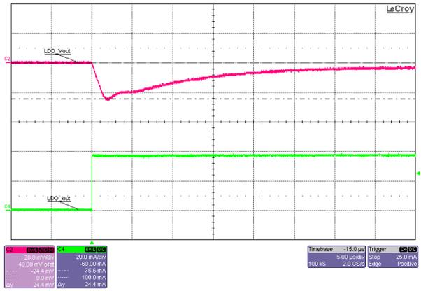
Figure 3-37. GTAVCCAUX Rail Load Transient Response (LDO), at 5V<sub>IN</sub>, 1.5V<sub>OUT</sub>, 0A-to-0.035A (that is, 0%-to-70%) Load Step, Undershoot
