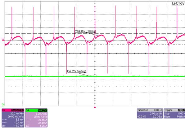
Figure 3-12. 5V Pre-Regulator Buck Output Voltage Ripple, 13.5V Input, 12A Load
