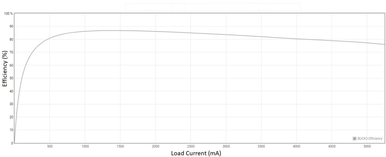
**Figure 2-10. GTAVCC/MGTYAVCC Rail Efficiency (PMIC Buck 3), FPWM Mode Operation**
