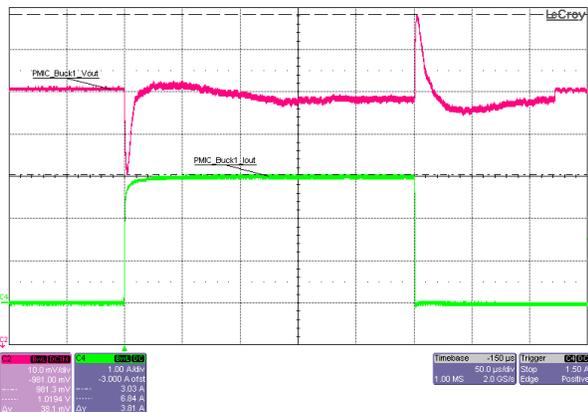
**Figure 3-28. VCCO - PMC\_Buck1 Rail Converter Load Transient Response, at 5V<sub>IN</sub>, 1.0V<sub>OUT</sub>, 0A-to-3A (that is, 0%-to-100%) Load Step, PFM Mode**
