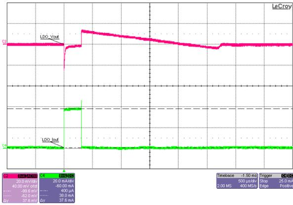
Figure 3-36. GTAVCCAUX Rail Load Transient Response (LDO), at 5V<sub>IN</sub>, 1.5V<sub>OUT</sub>, 0mA-to-35mA (that is, 0%-to-70%) Load Step, Full Step
