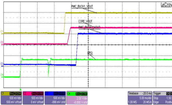
**Figure 3-54. Sequence Power-Up, Sequence Rails 1, 2, 3, and 4, Discrete Vsupervisor nIRQ, No Load**
