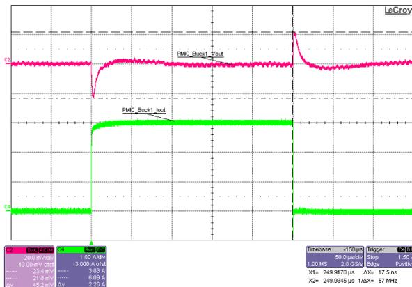
**Figure 3-29. VCCO Rail Load Transient Response (PMC\_Buck1), at 5V<sub>IN</sub>, 1.0V<sub>OUT</sub>, 0A-to-3A (that is, 0%-to-100%) Load Step, FPWM Mode**
