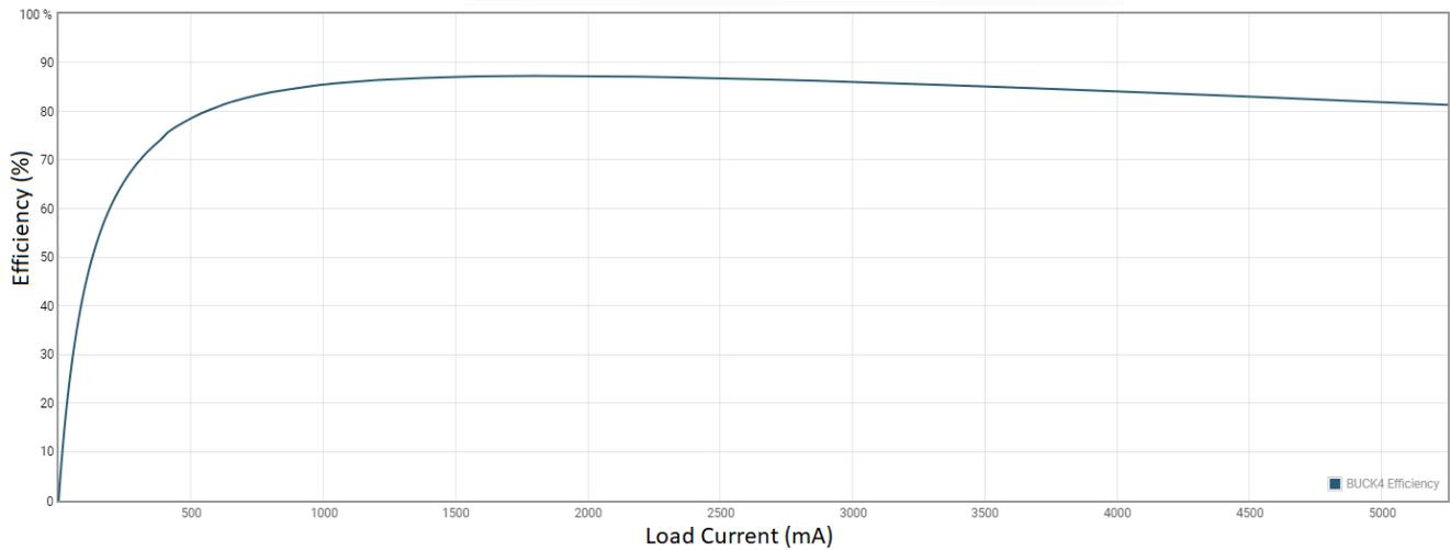
Figure 2-12. GTAVTT, MGTYAVTT Rail Efficiency (PMIC Buck 4), FPWM Mode Operation
