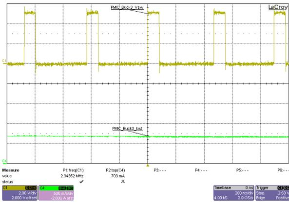
Figure 3-9. GTAVCC Rail Switch Node Voltage (PMIC\_Buck3), 5V Input, 0.88V<sub>OUT</sub>, 0.7A Load
