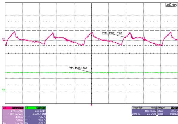
Figure 3-16. VCCO Output Voltage Ripple (PMIC\_Buck1), 5V Input, 1.0V Output, 3A Load
