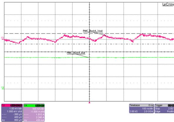
Figure 3-22. GTAVTT Output Voltage Ripple (PMIC\_Buck4), 5V Input, 1.2V Output, 1.3A Load
