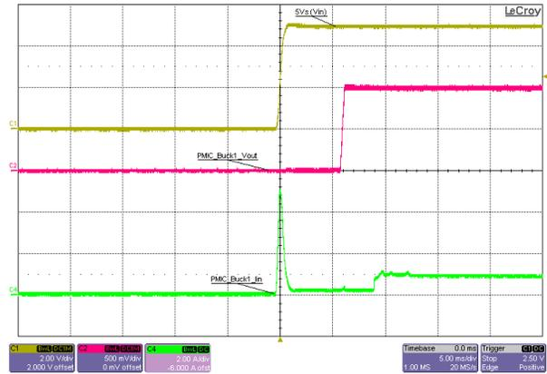
Figure 3-43. VCCO Rail Start-Up (PMIC\_Buck1), 5V Input, 3A Constant-Resistance eLoad
