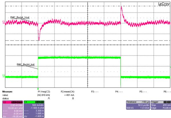
**Figure 3-35. GTAVTT Rail Load Transient Response (PMIC\_Buck4), at 5V<sub>IN</sub>, 1.2V<sub>OUT</sub>, 0A-to-0.91A (that is, 0%-to-70%) Load Step, FPWM Mode**
