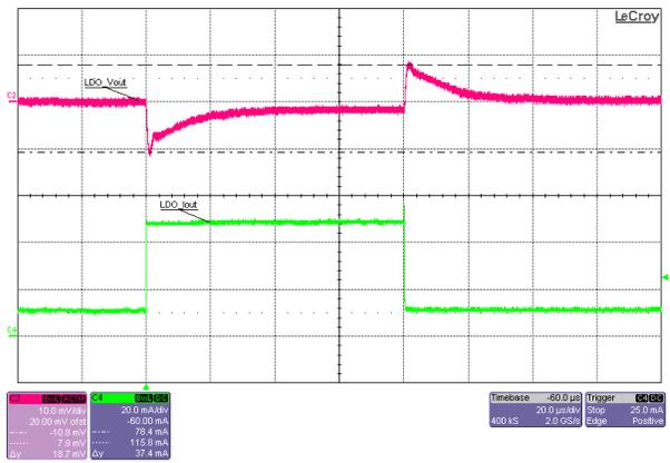
Figure 3-39. GTAVCCAUX Rail Load Transient Response (LDO), at 5V<sub>IN</sub>, 1.5V<sub>OUT</sub>, 11mA-to-48mA Load Step, Full Step
