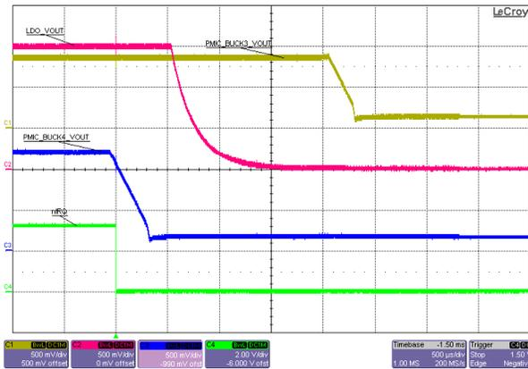
**Figure 3-56. Sequence Power-Down, Sequence Rails 6, 5, and 4, Discrete Vsupervisor nIRQ, No Load**
