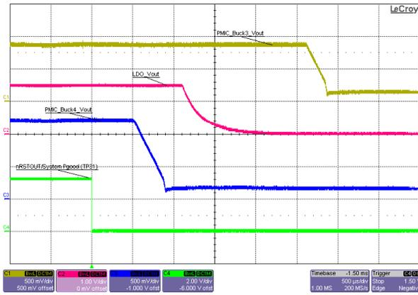
**Figure 3-52. Sequence Power-Down, Sequence Rails 6, 5, and 4, PMIC nRSTOUT, No Load**
