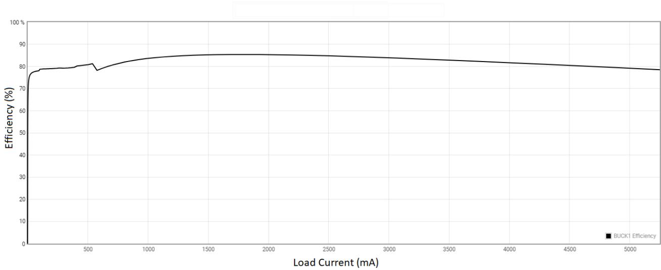
**Figure 2-5. VCCO Rail Efficiency (PMIC Buck 1), PFM Mode Operation**
