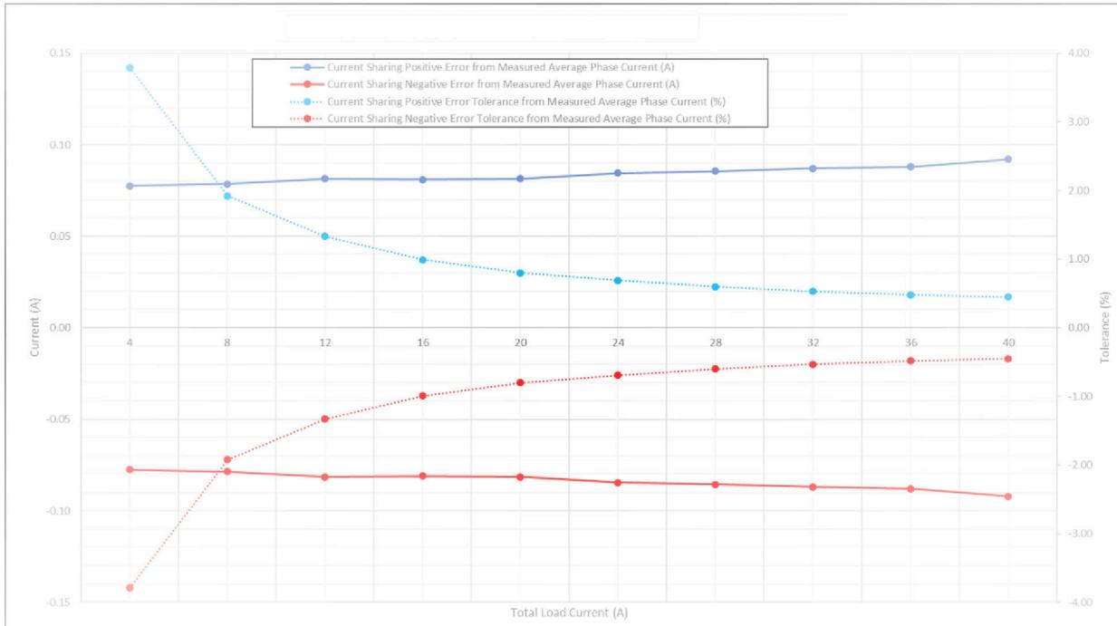
Figure 2-13. VCCINT- Core Rail Current Sharing Variance and Tolerance
