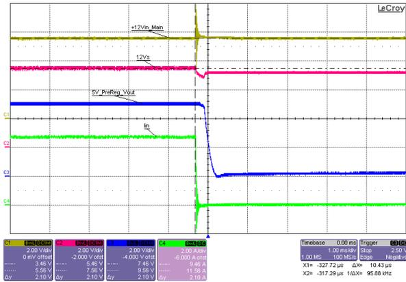
**Figure 3-59. Front-End Protection, UVLO Falling Disable, 5V Pre-Regulator Buck Output Loaded at 5A Load (FEP UVLO Disable Threshold  $\approx$  5.6V; 5V Pre-Regulator UVLO Disable Threshold  $\approx$  5.2V)**
