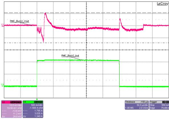
**Figure 3-30. VCCAUX Rail Load Transient Response (PMIC\_Buck2), at 5V<sub>IN</sub>, 1.5V<sub>OUT</sub>, 0A-to-1.1A (that is, 0%-to-100%) Load Step, PFM Mode**
