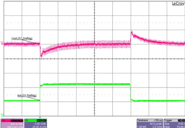
**Figure 3-24. 5V Pre-Regulator Buck Converter Load Transient Response, 13.5V Input,  $\approx$  6A-to-12A Load Step**
