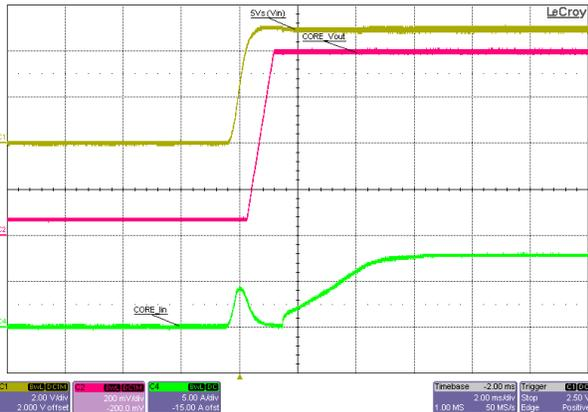
Figure 3-42. VCCINT - Core Rail Start-Up, 5V Input, 40A Constant-Resistance eLoad
