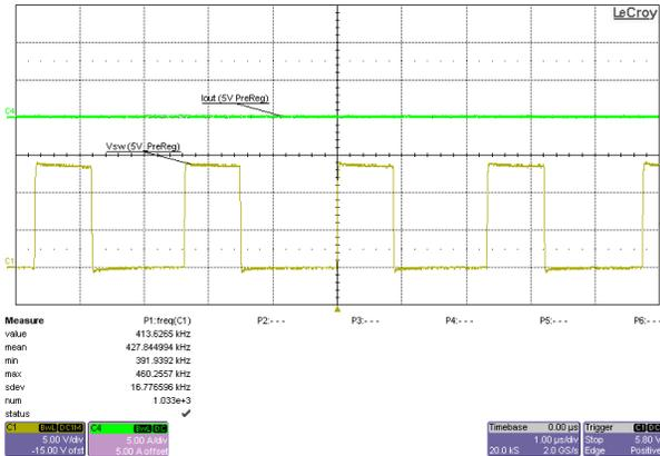
Figure 3-1. 5V Pre-Regulator, Switching 1
