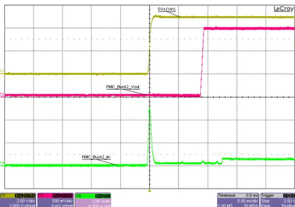
Figure 3-44. VCCAUX Rail Start-Up (PMIC\_Buck2), 5V Input, 1.1A Constant-Resistance eLoad
