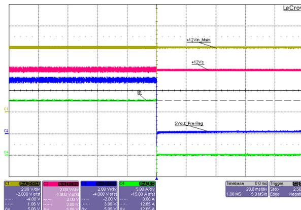
**Figure 3-62. Front-End Protection, OCP Threshold Test, 5V Pre-Regulator Buck at 6V<sub>IN</sub> With the Load Progressively Increasing; 100k $\Omega$  “TMR” Resistor Installed for this Test (FEP OCP Threshold  $\approx$  12.65A)**
