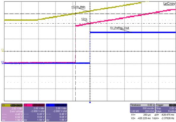
**Figure 3-58. Front-End Protection, UVLO Rising Enable, 5V Pre-Regulator Buck Output No Load (FEP UVLO Enable Threshold  $\approx$  6.0V; 5V Pre-Regulator UVLO Enable Threshold  $\approx$  6.5V)**
