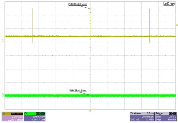
Figure 3-8. GTAVCC Rail Switch Node Voltage (PMIC\_Buck3), 5V Input, 0.88V<sub>OUT</sub>, No Load, PFM Mode
