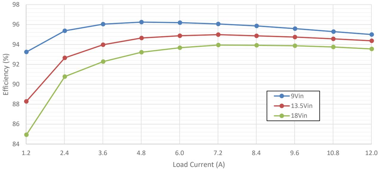
Figure 2-1. 5V Pre-Regulator Buck Efficiency
