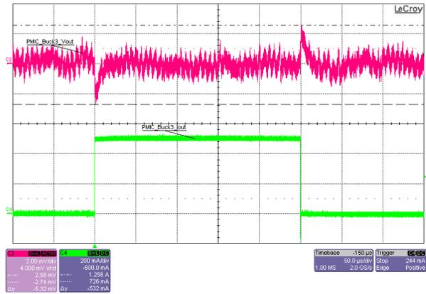
**Figure 3-33. GTAVCC Rail Load Transient Response (PMIC\_Buck3), at 5V<sub>IN</sub>, 0.88V<sub>OUT</sub>, 0A-to-0.49A (that is, 0%-to-70%) Load Step, FPWM Mode**
