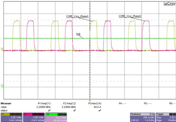
Figure 3-3. VCCINT Rail Switch Node Voltage (Core Rail Buck), 5V Input, 40A Load
