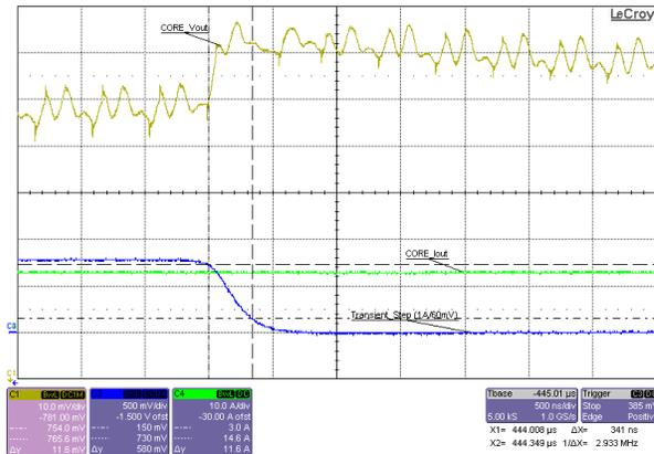
**Figure 3-27. VCCINT - Core Rail Buck Converter Load Transient Response, Load Step Falling Slew Rate, at 5V<sub>IN</sub>, 25.6A-to-12.8A (that is, 66%-to-33%) Load Step (Slew Rate  $\approx$  28A/ $\mu$ s)**
