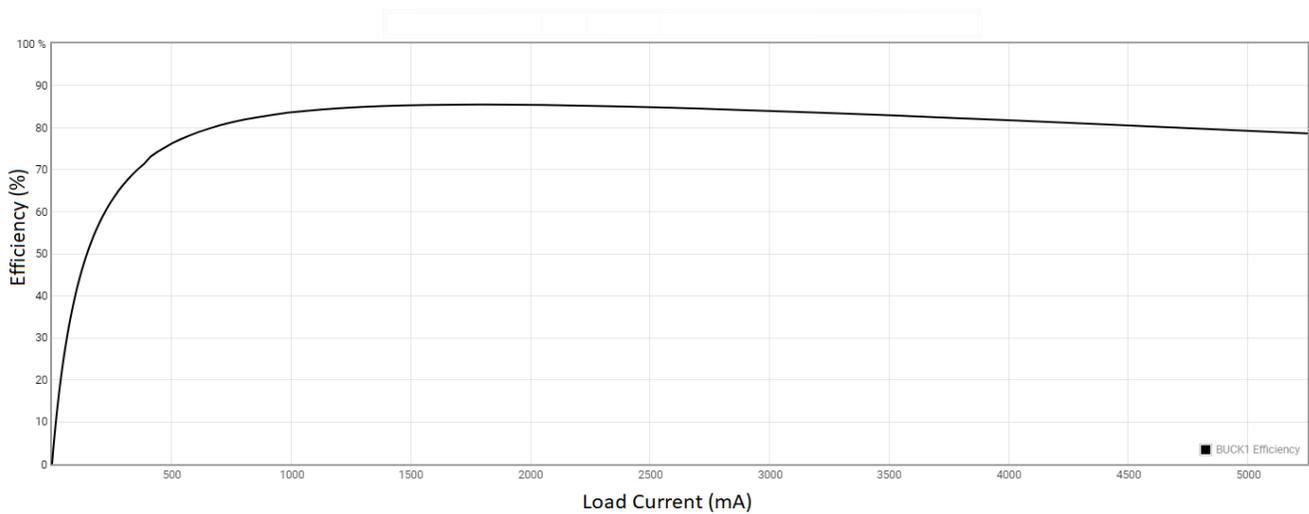
**Figure 2-6. VCCO Rail Efficiency (PMIC Buck 1), FPWM Mode Operation**
