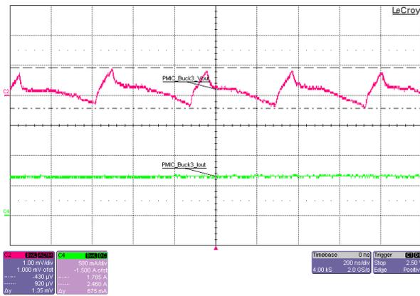
Figure 3-20. GTAVCC Output Voltage Ripple (PMIC\_Buck3), 5V Input, 0.88V Output, 0.7A Load
