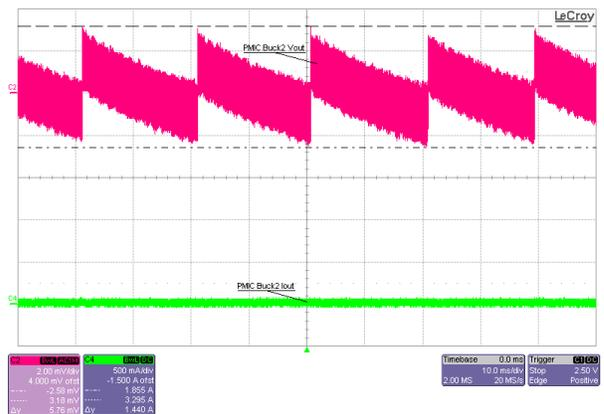
Figure 3-17. VCCAUX Output Voltage Ripple (PMIC\_Buck2), 5V Input, 1.5V Output, No Load, PFM Mode
