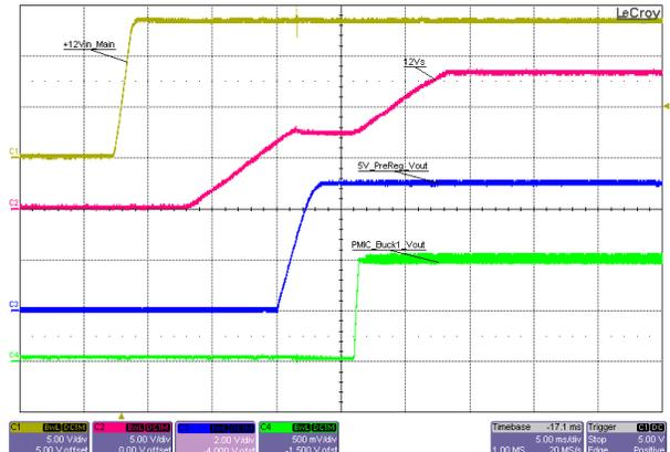
**Figure 3-49. System Start-Up Into No Load, 13.5V Input, +12Vin\_Main, 12Vs, 5V Pre-Regulator, VCCO (PMIC Buck 1)**
