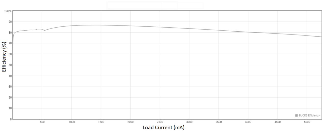
**Figure 2-9. GTAVCC/MGTYAVCC Rail Efficiency (PMIC Buck 3), PFM Mode Operation**
