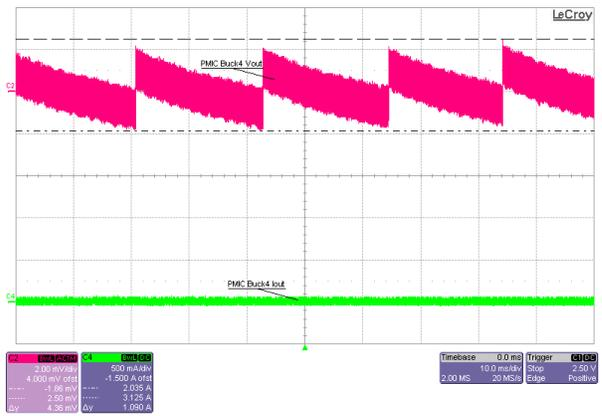
Figure 3-21. GTAVTT Output Voltage Ripple (PMIC\_Buck4), 5V Input, 1.2V Output, No Load, PFM Mode
