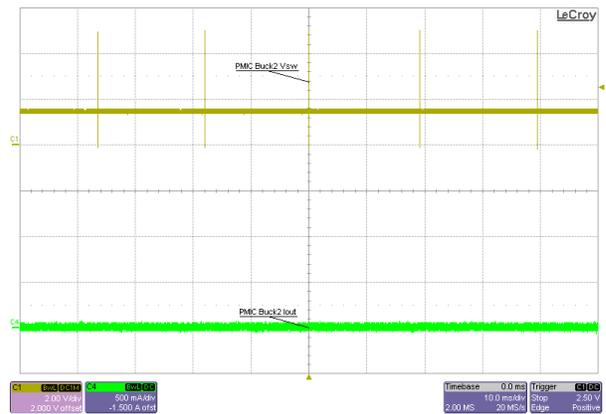
Figure 3-6. VCCAUX Switch Node Voltage (PMIC\_Buck2), 5V Input, 1.5V<sub>OUT</sub>, No Load, PFM Mode
