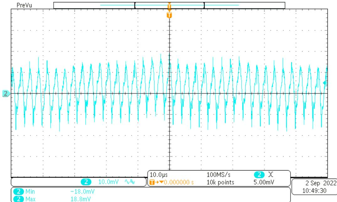
Channel 2: AC coupled input voltage ripple at 15 V<sub>OUT</sub> and 100mA load current, bandwidth limited (20MHz), [scale: 10mV/div, 10.0µs/div]. The input voltage ripple was measured at input capacitor C35.
