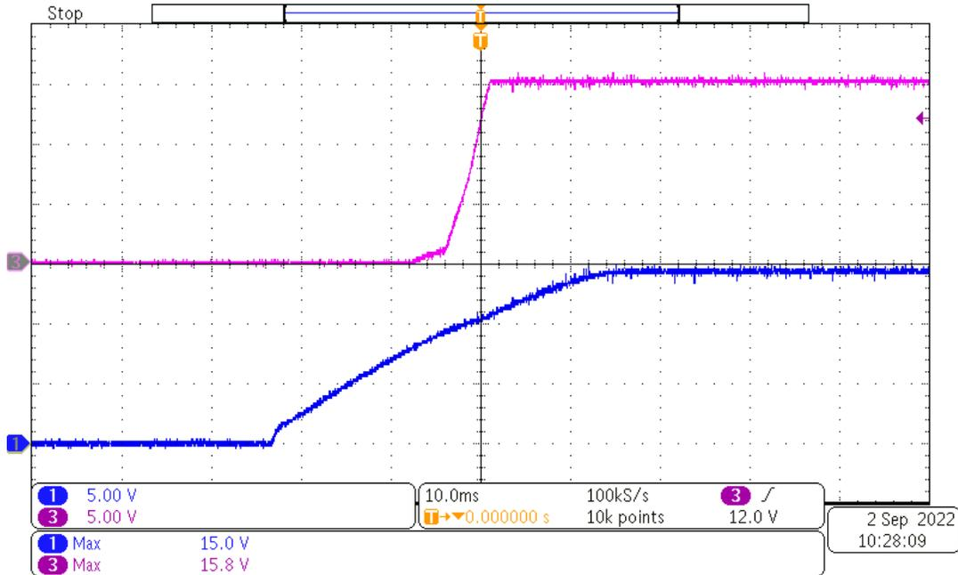
Channel 1: Start-up with input voltage of 15V at full load of 100mA, [scale: 5V/div, 10ms/div]
