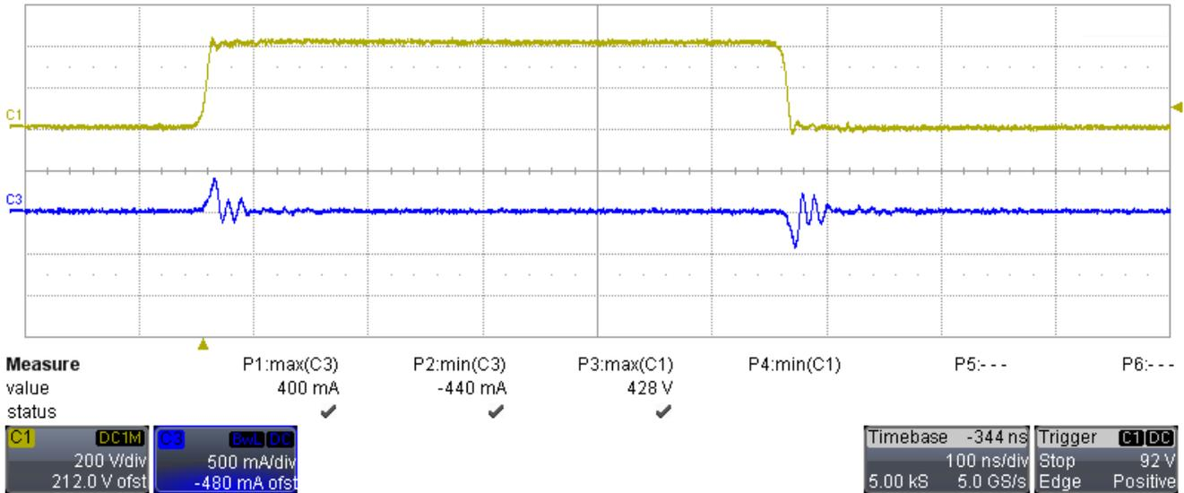
Channel 1: HV switch node, [scale: 200V/div, 100ns/div]
