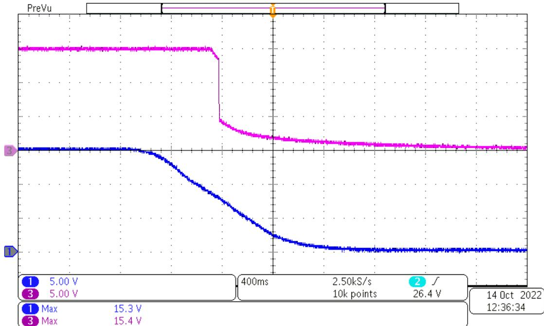
Channel 1: Input voltage at shutoff with UVLO protection at no load, [scale: 5V/div, 400ms/div]
