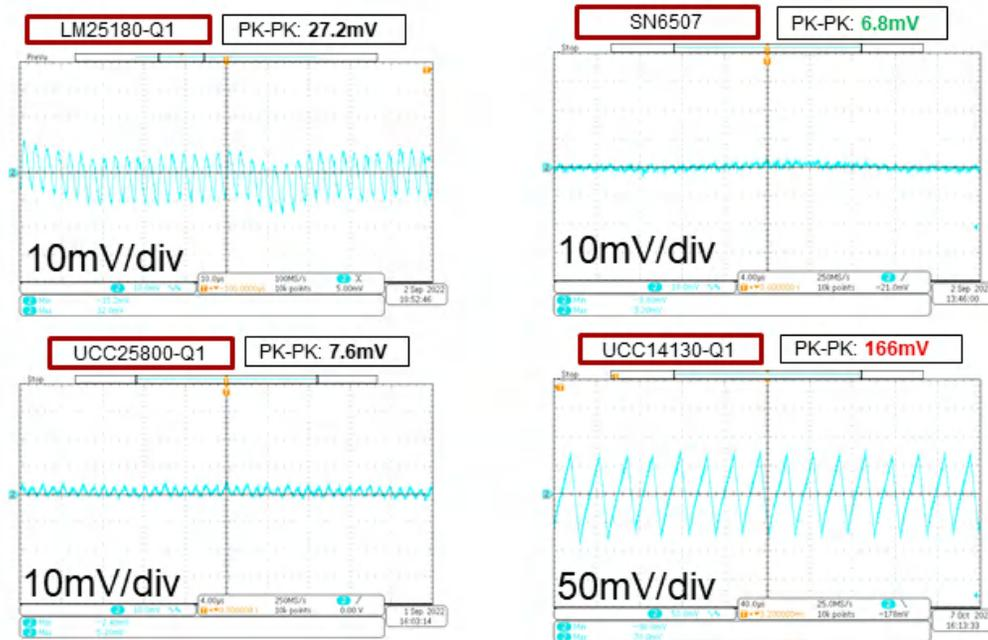
The isolated DCDC module uses an ON-OFF control scheme that results in larger input ripple and output ripple.
