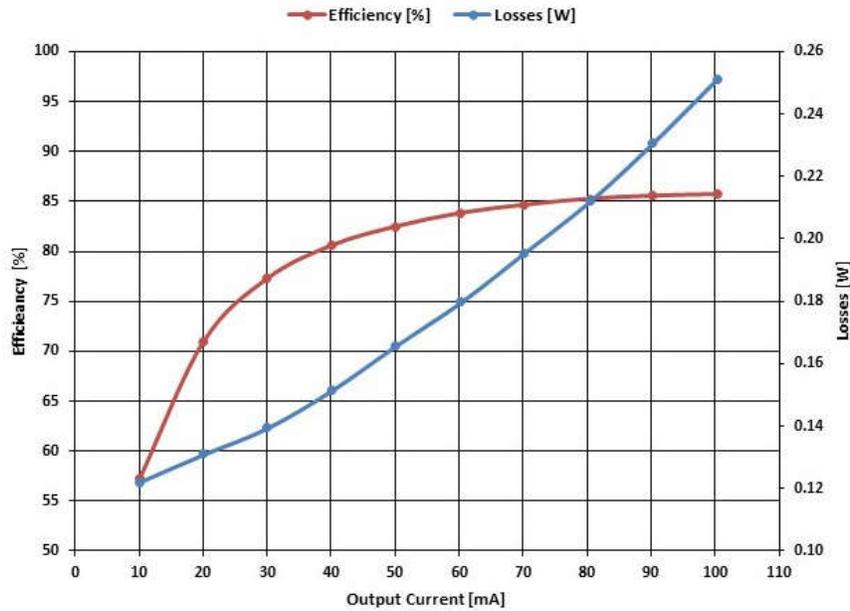
Figure 2-4. UCC25800-Q1 Efficiency at 15 V<sub>IN</sub>
