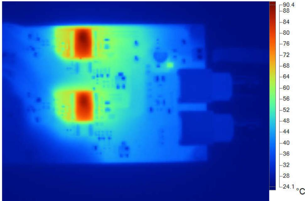
Figure 2-13. Thermal Image – Top Side of PCB at 15 V<sub>IN</sub> and 100mA Full Load Current
