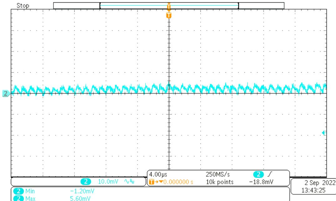
Channel 2: AC coupled Input Voltage Ripple at 15 V<sub>OUT</sub> and 100mA load current, bandwidth limited (20MHz), [scale: 10mV/div, 4.0µs/div]. The input voltage ripple was measured at input capacitor C31.
