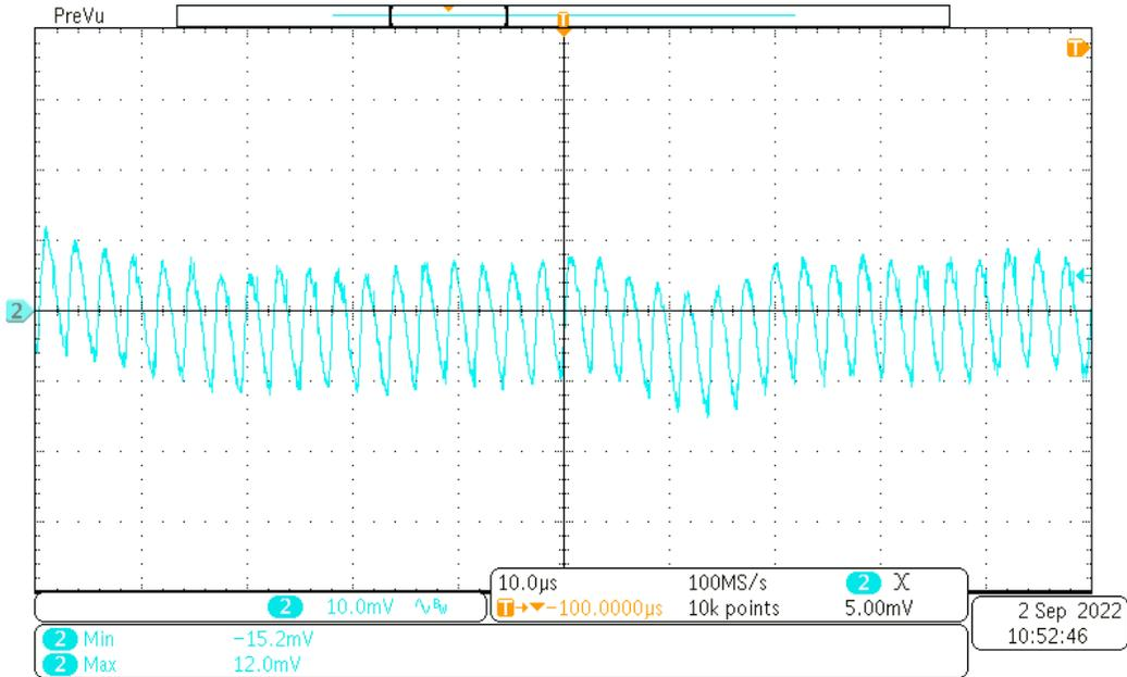
**Figure 3-4. LM25180-Q1 Output Voltage Ripple**
