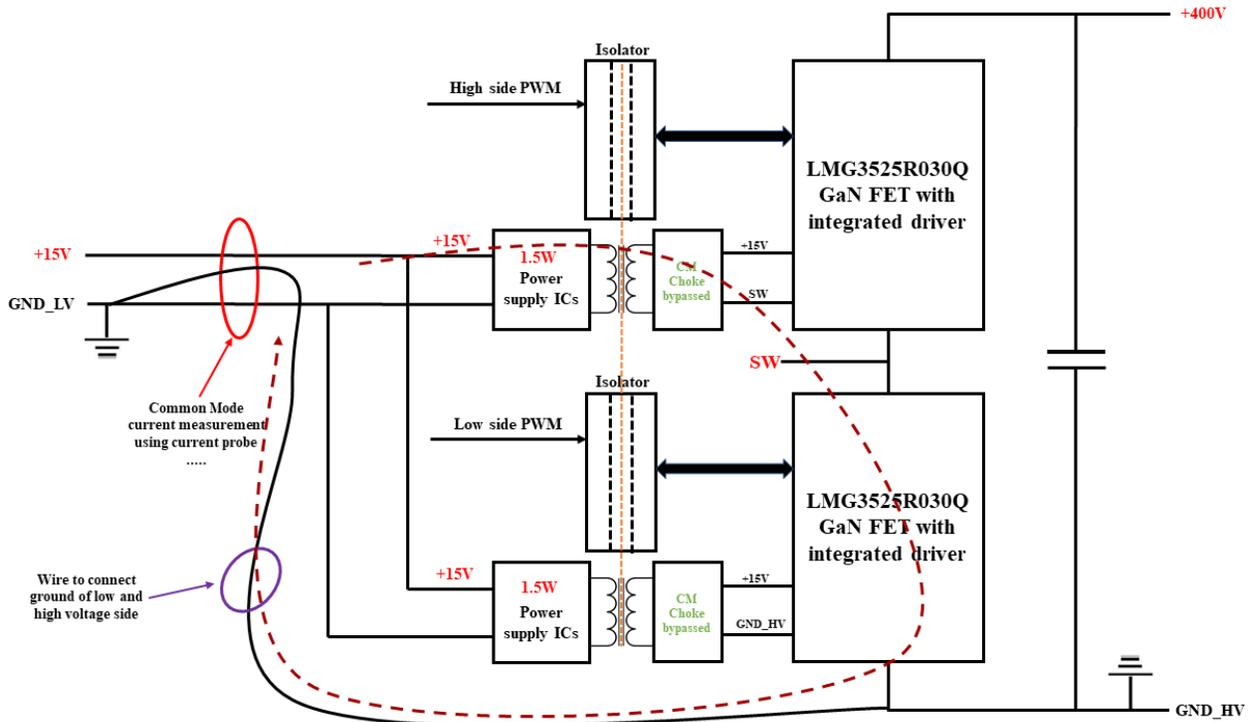
Figure 2-15. Common-Mode Current (CMI) Test Setup
