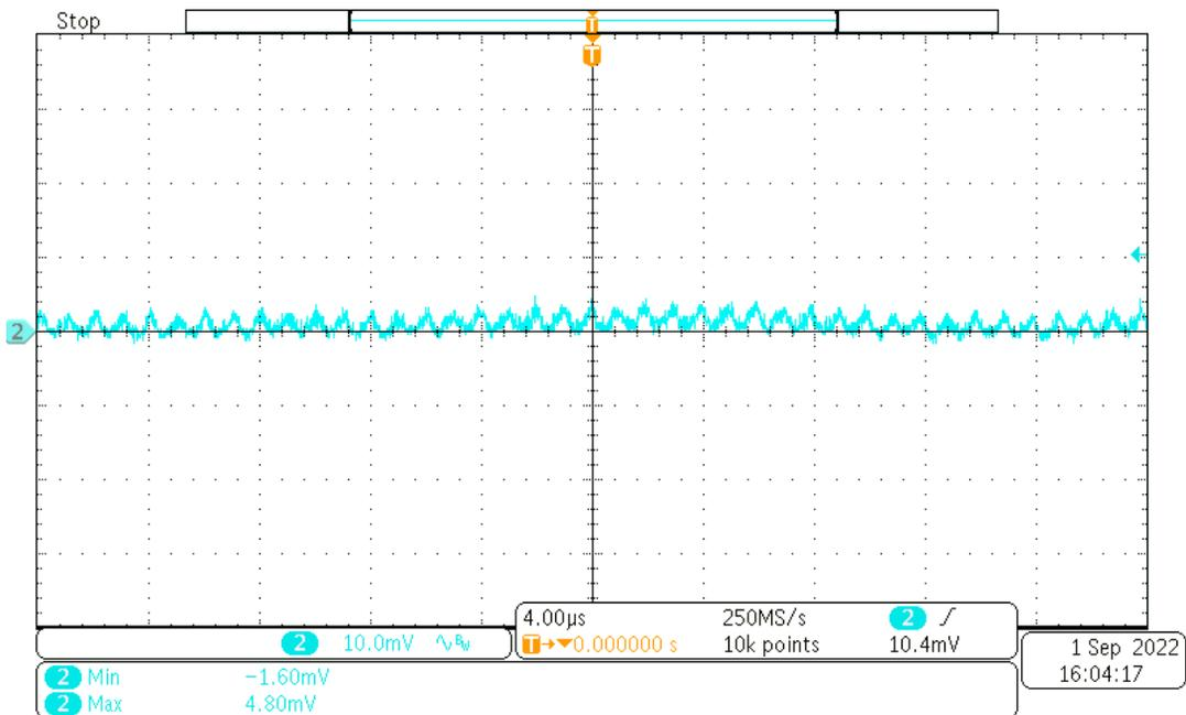
Channel 2: AC coupled input voltage ripple at 15 V<sub>OUT</sub> and 100mA load current, bandwidth limited (20MHz), [scale: 10mV/div, 4.0µs/div]. The input voltage ripple was measured at input capacitor C61.
