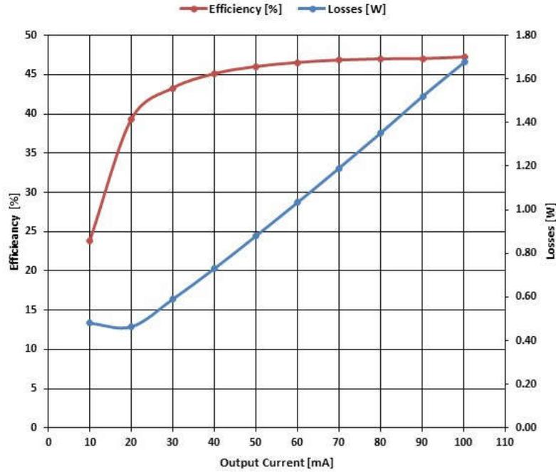
Figure 2-3. UCC14130-Q1 Efficiency at 15 V<sub>IN</sub>
