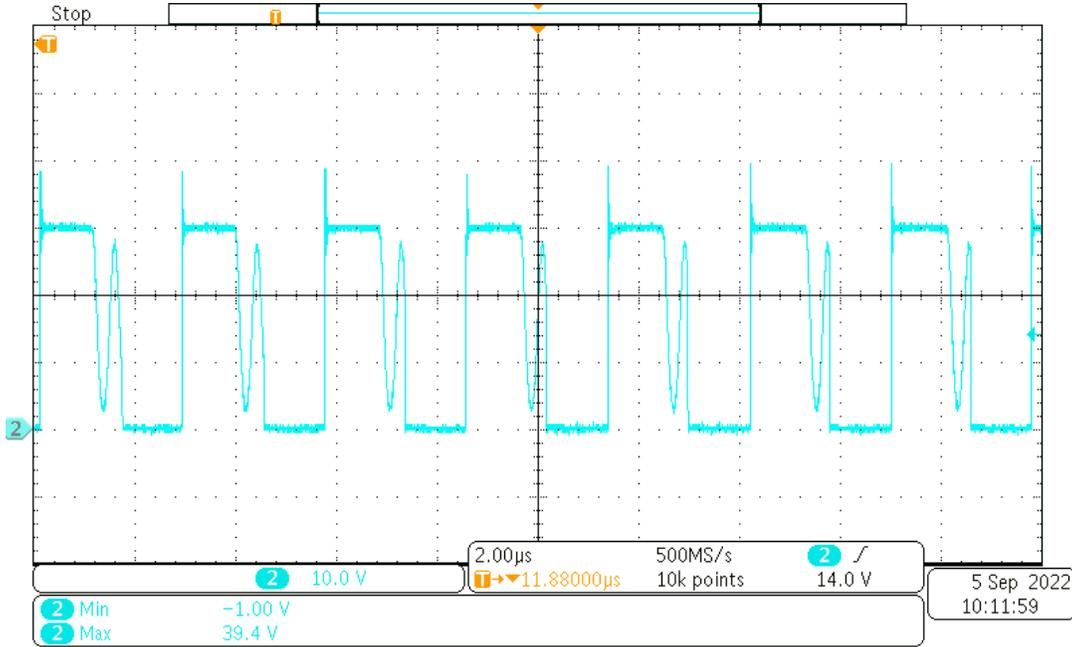
Channel 2: Switching node at 15 V<sub>OUT</sub> and 100mA load current [scale: 10.0V/div, 2.0µs/div]
