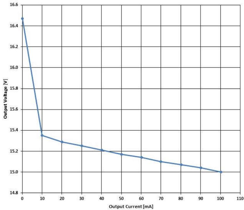
An 18V Zener diode is used to clamp the output voltage in case of no load condition.
