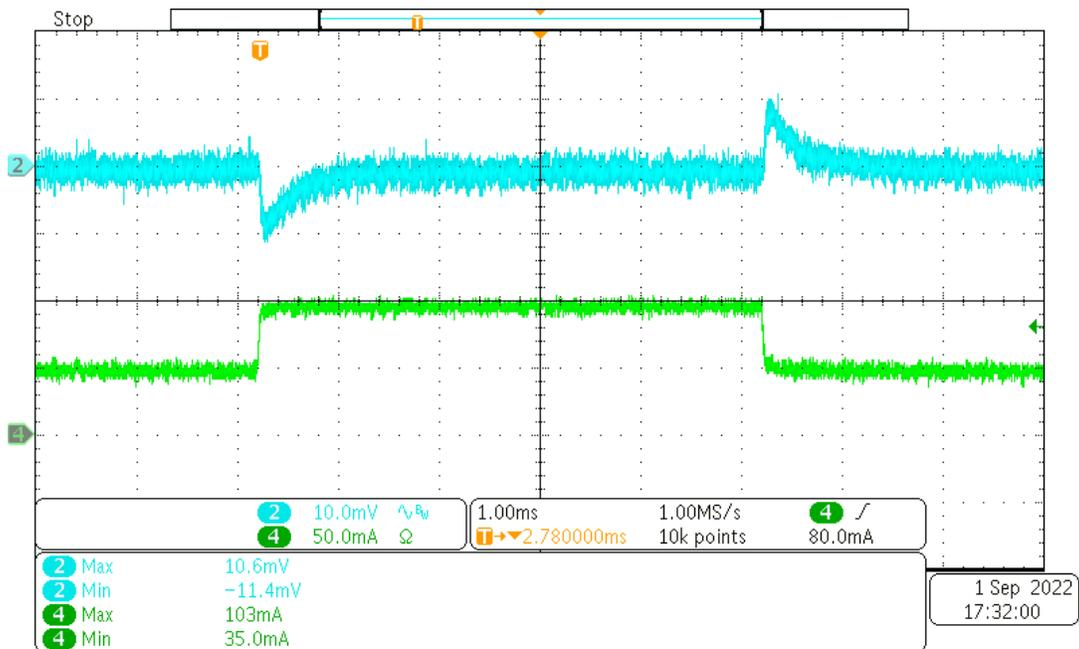
Channel 2: AC-coupled output voltage at 15 V<sub>OUT</sub>, bandwidth limited (20MHz), [scale: 10mV/div, 1ms/div]
