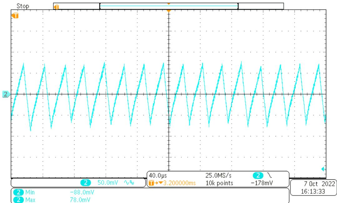
Channel 2: AC coupled output voltage ripple at 15 V<sub>OUT</sub> and 100mA load current, bandwidth limited (20MHz), [scale: 50mV/div, 40.0µs/div]. The output voltage ripple was measured at output capacitor C36.
