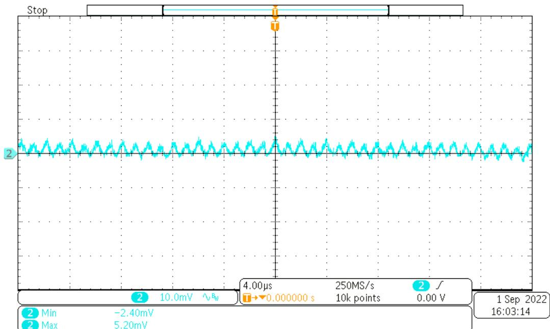
Channel 2: AC coupled output voltage Ripple at 15 V<sub>OUT</sub> and 100mA load current, bandwidth limited (20MHz), [scale: 10mV/div, 4.0µs/div]. The output voltage ripple was measured at output capacitor C64.
