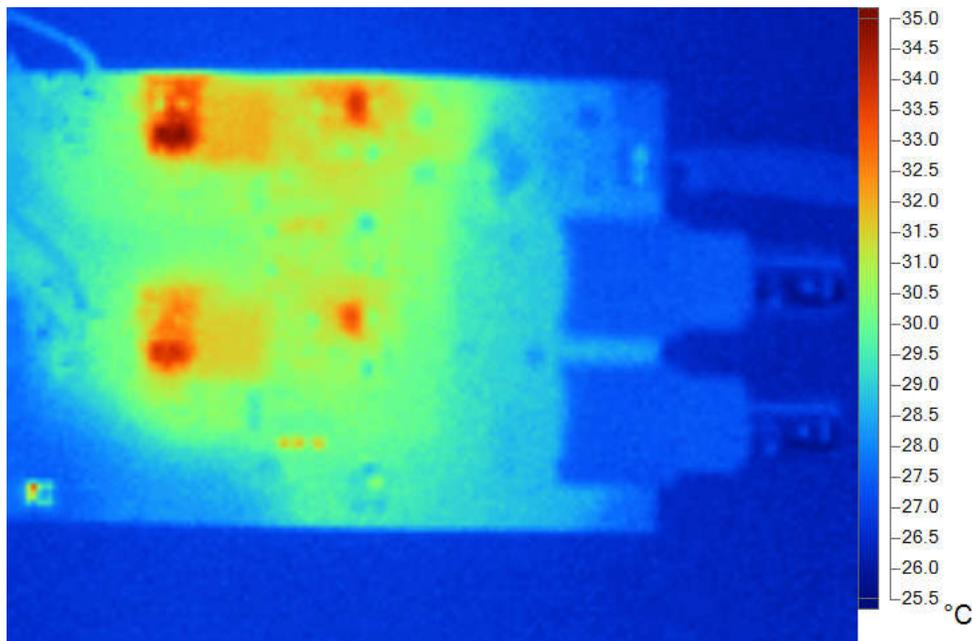
Figure 2-14. Thermal Image – Top Side of PCB at 15 V<sub>IN</sub> and 100mA Full Load Current
