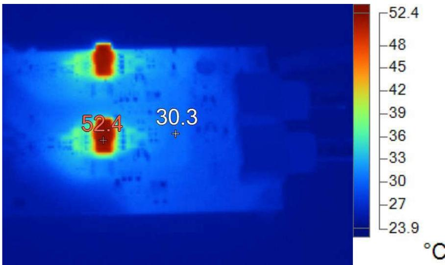
Figure 2-12. Thermal Image – Top Side of PCB at 15 V<sub>IN</sub> and 100mA Full Load Current
