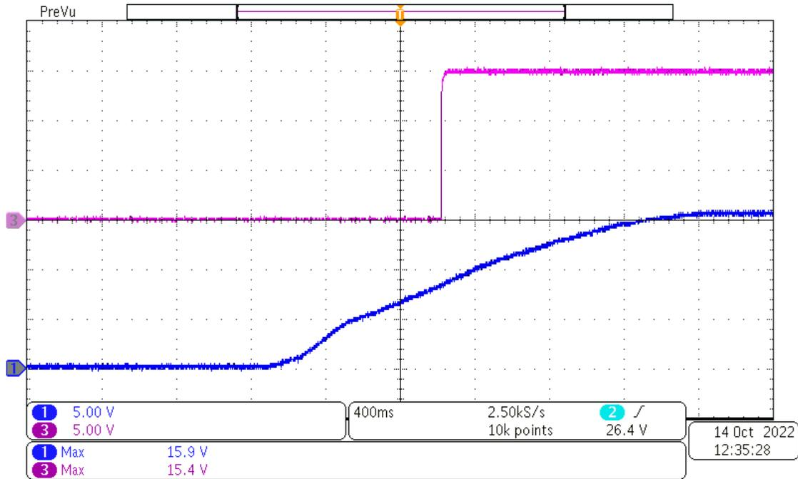
Channel 1: Input voltage at start-up with UVLO protection at no load, [scale: 5V/div, 400ms/div]
