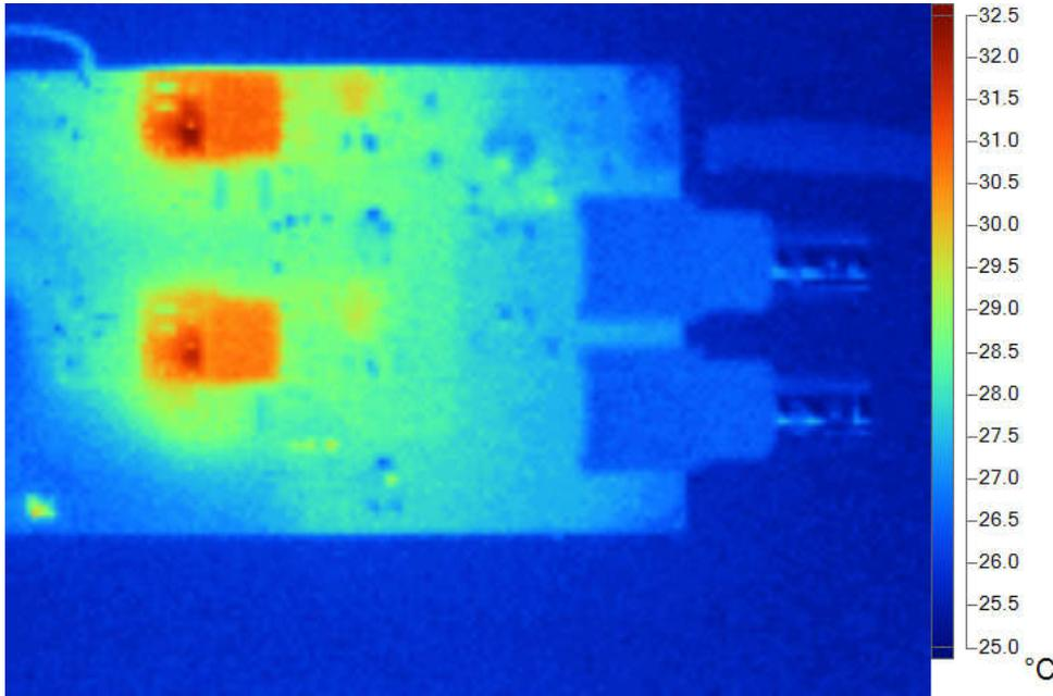
Figure 2-11. Thermal Image – Top Side of PCB at 15 V<sub>IN</sub> and 100mA Full Load Current
