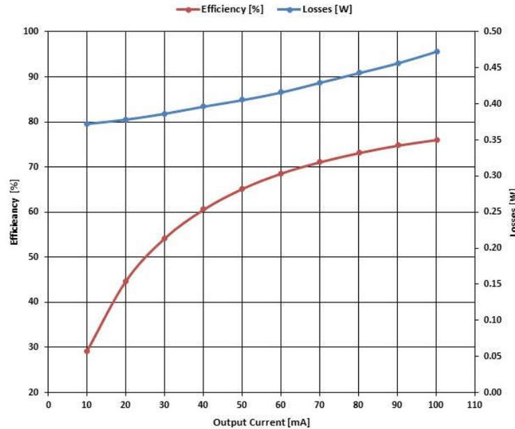
Figure 2-2. SN6507-Q1 Efficiency at 15 V<sub>IN</sub>
