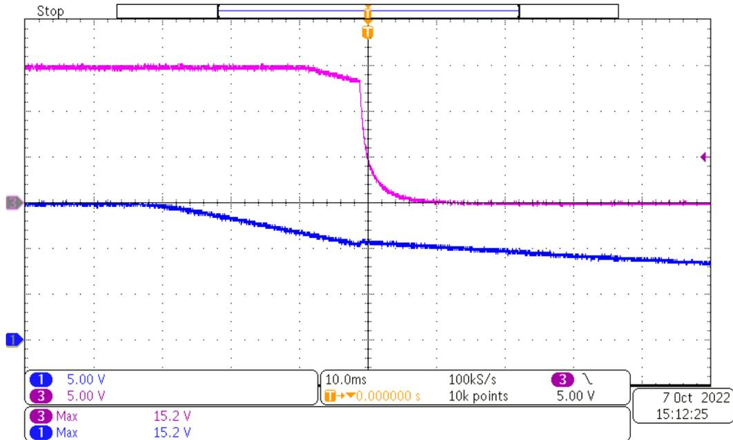
Channel 1: Shutoff with input voltage of 15V at full load of 100mA, [scale: 5V/div, 10ms/div]
