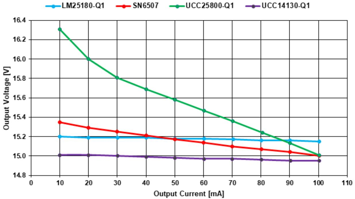
Figure 2-10. Load Regulation Comparison
