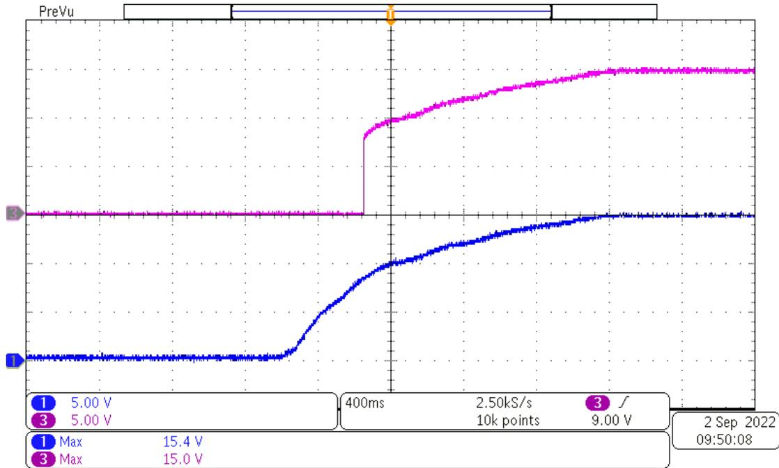
Channel 1: Input voltage at start-up with UVLO protection at full load, [scale: 5V/div, 400ms/div]
