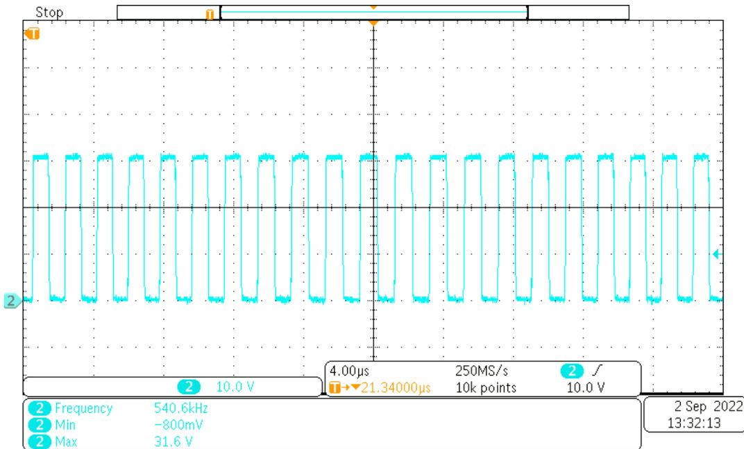
Channel 2: Switching node at 15 V<sub>OUT</sub> and 100mA load current [scale: 10.0V/div, 4.0µs/div]
