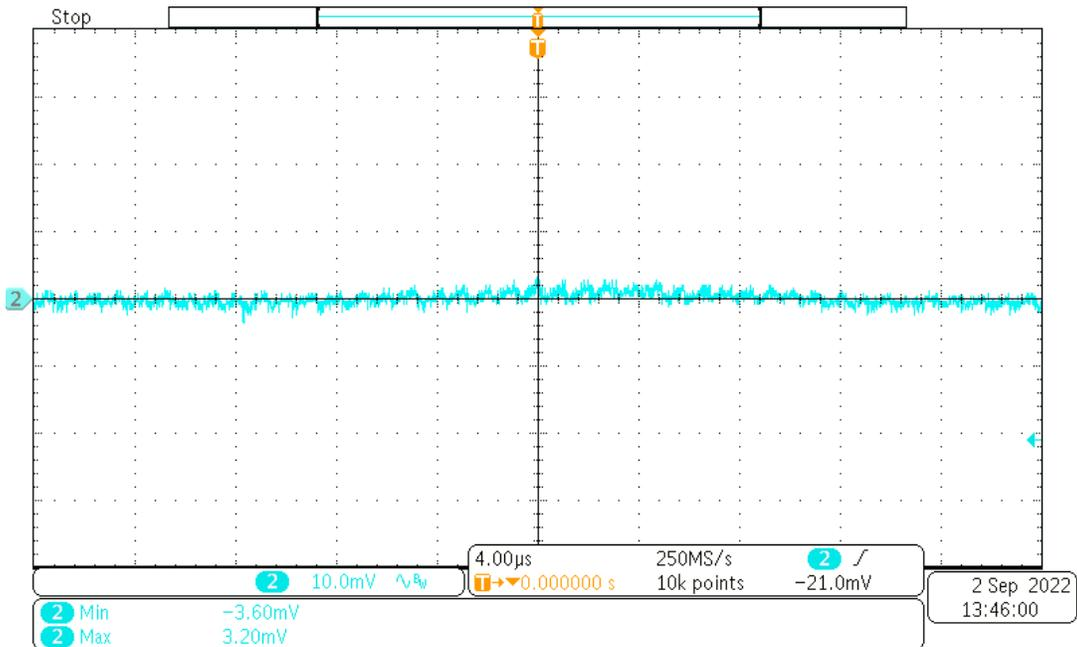
**Figure 3-5. SN6507-Q1 Output Voltage Ripple**
