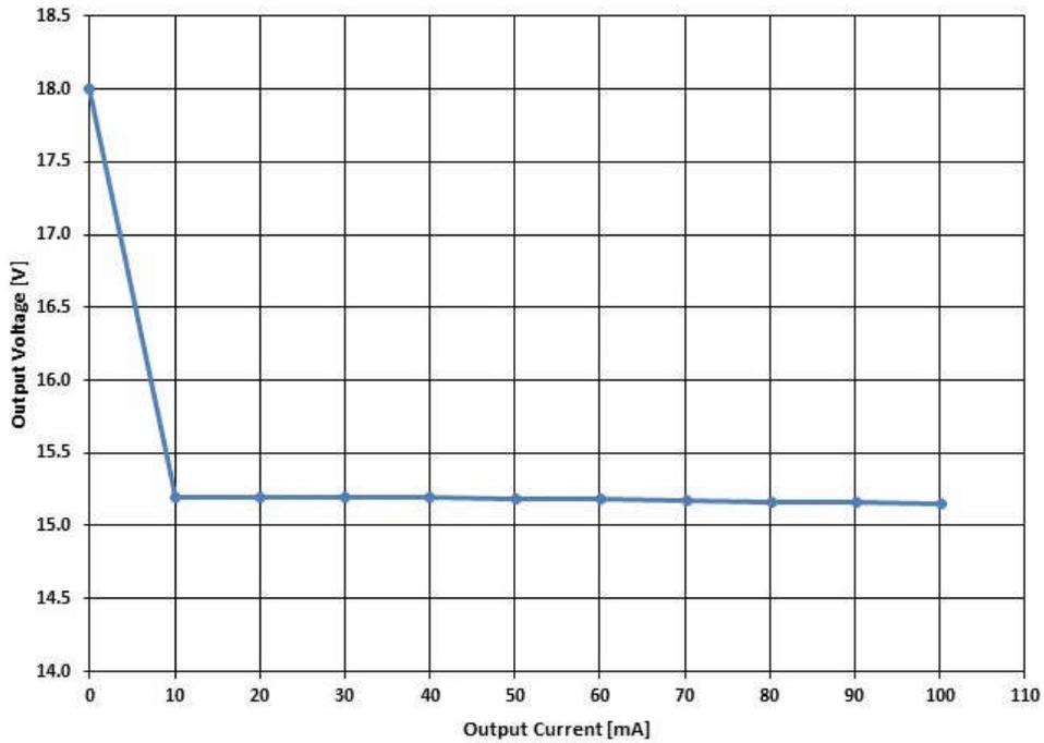
An 18V Zener diode is used to clamp the output voltage in case of no load condition.
