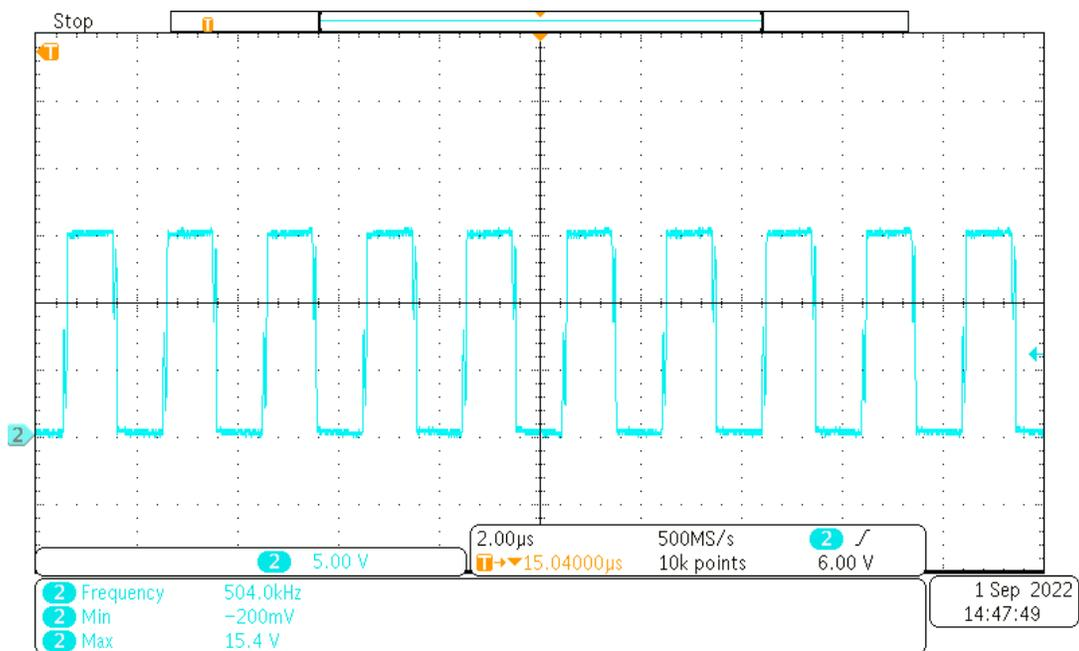
Channel 2: Switching node at 15 V<sub>OUT</sub> and 100mA load current [scale: 5.0V/div, 2.0µs/div]
