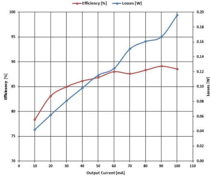
Figure 2-1. LM25180-Q1 Efficiency at 15 V<sub>IN</sub>
