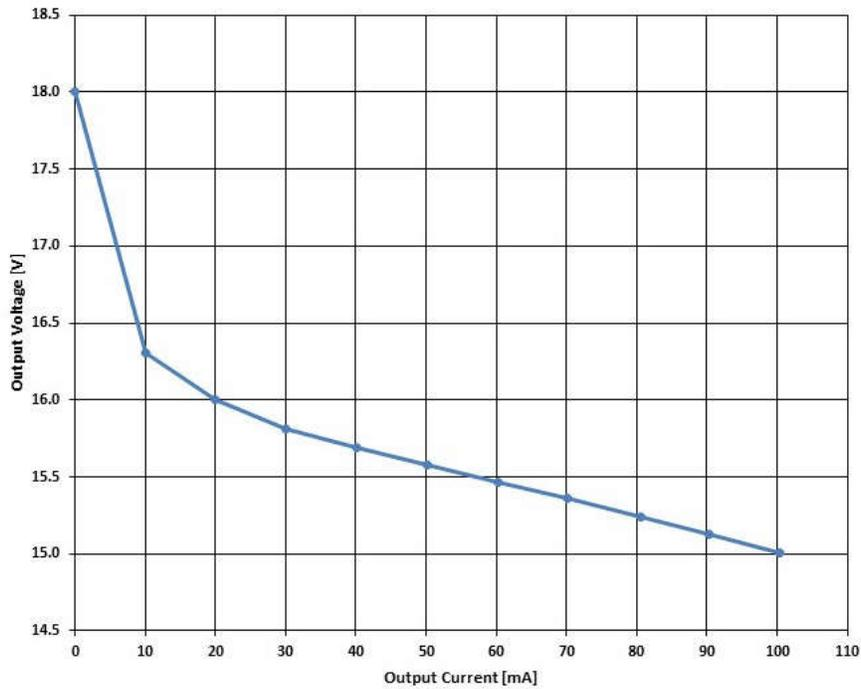
An 18V Zener diode is used to clamp the output voltage in case of no load condition.
