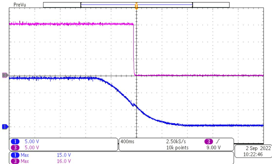
Channel 1: Input voltage at shutoff with UVLO protection at full Load, [scale: 5V/div, 400ms/div]
