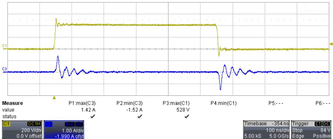
Channel 1: HV switch node, [scale: 200V/div, 100ns/div]
