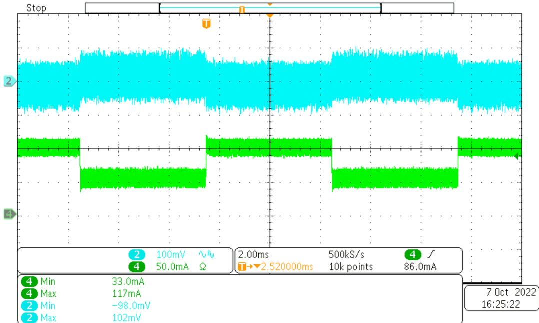
Channel 2: AC-coupled output voltage at 15 V<sub>OUT</sub>, bandwidth limited (20MHz), [scale: 100mV/div, 2ms/div]
