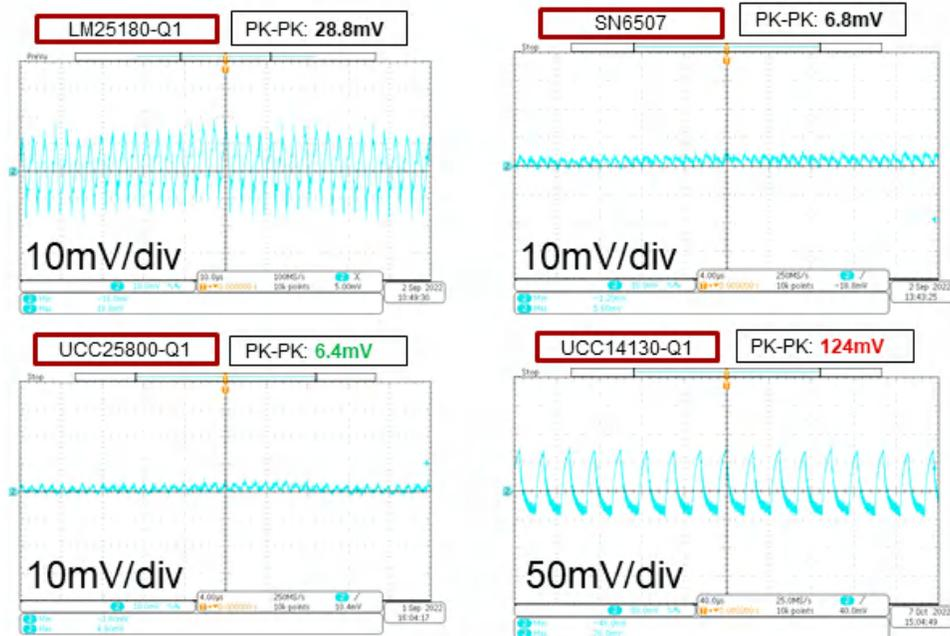
The isolated DCDC module uses an ON-OFF control scheme that results in larger input ripple and output ripple.
