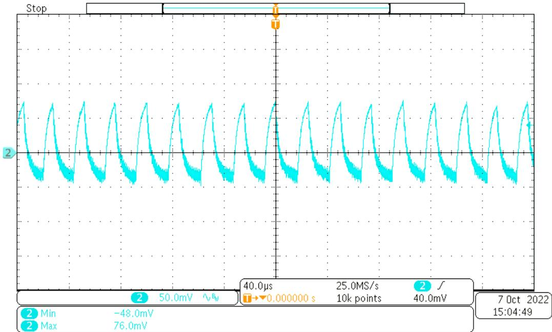
Channel 2: AC coupled Input Voltage Ripple at 15 V<sub>OUT</sub> and 100mA load current, bandwidth limited (20MHz), [scale: 50mV/div, 40.0µs/div]. The input voltage ripple was measured at input capacitor C33.
