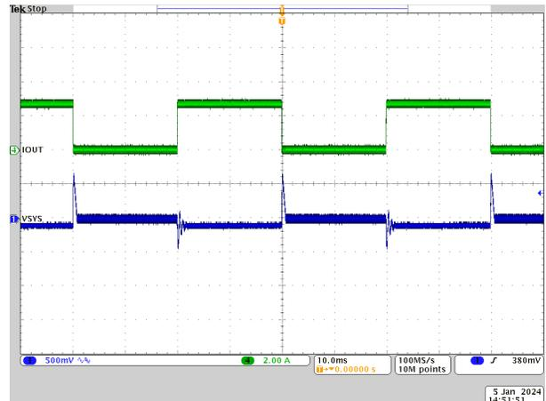
**Figure 3-20. OTG Mode, 5V, 10% to 100% Load Dynamic**
