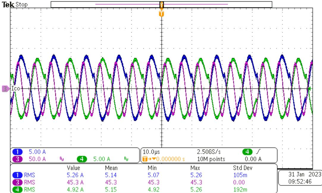
Figure 3-1. Waveform With 0 Degree Shift at 133-A Load
