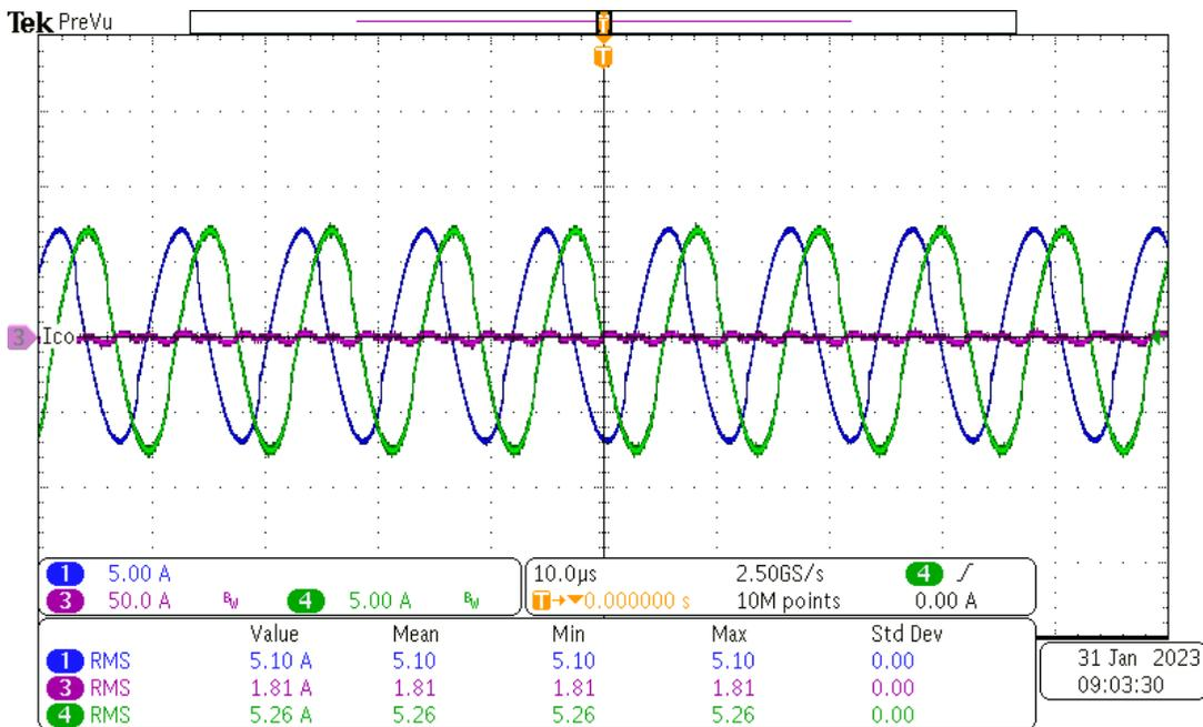
Figure 3-2. Waveform With 90 Degree Shift at 133-A Load
