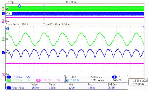
**Figure 3-10. Output Voltage Ripple Under 380-V, 84-A Load**
