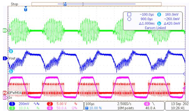
**Figure 3-7. Load Transient of 420-V, 0%-100%,
