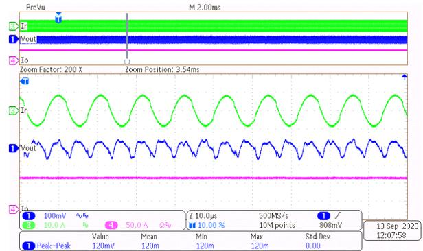
**Figure 3-13. Output Voltage Ripple Under 400-V, 84-A Load**
