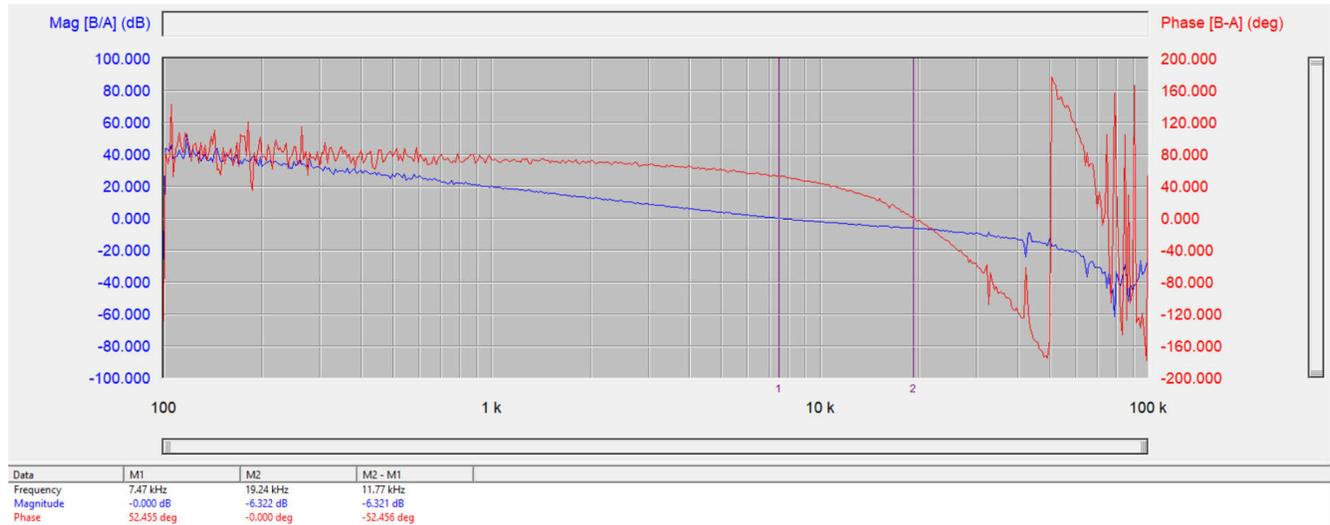
**Figure 2-1. Bode Plot Under 380-V, 20-A Load;  $f_c$ : 4.47 kHz; Phase Margin: 52.455 deg; Magnitude Margin: 6.322 dB**
