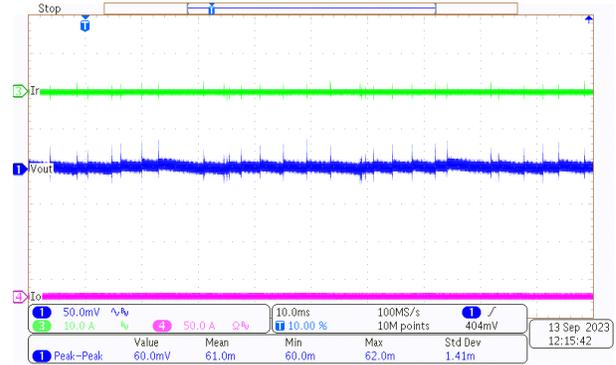
**Figure 3-11. Output Voltage Ripple Under 400-V, 0-A Load**
