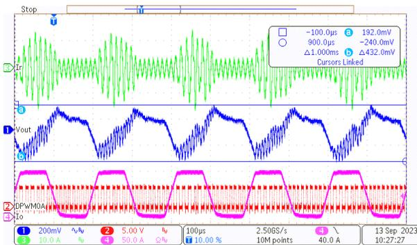
**Figure 3-5. Load Transient of 380-V, 0%-100%, 0.1 ms-0.1 ms, 2.5-A/μs Slew Rate**
