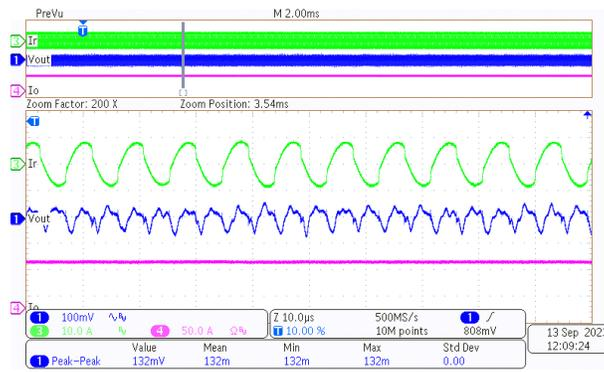
**Figure 3-16. Output Voltage Ripple Under 420-V, 84-A Load**
