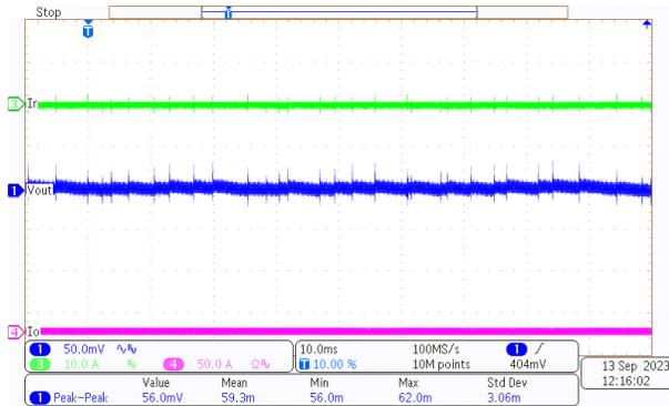
**Figure 3-8. Output Voltage Ripple Under 380-V, 0-A Load**
