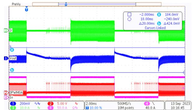
**Figure 3-6. Load Transient of 420-V, 0%-100%, 5 ms-5 ms, 2.5-A/μs Slew Rate**
