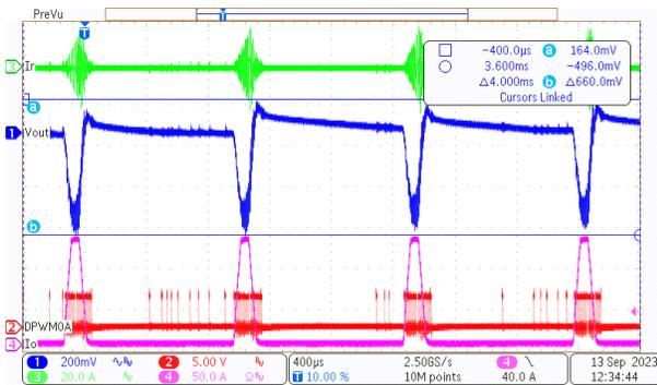
**Figure 3-3. Load Transient of 400-V, 0%-150%, 1 ms-0.1 ms, 2.5-A/μs Slew Rate**
