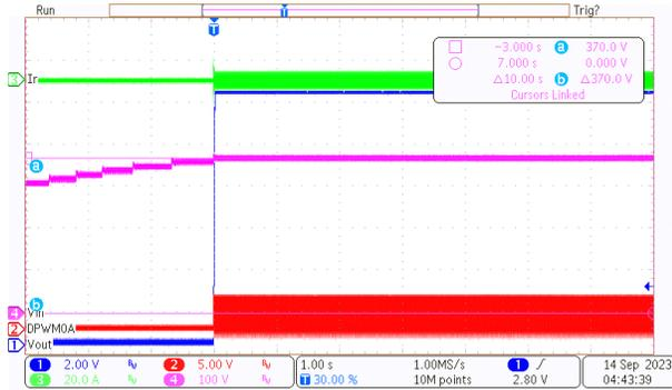
Figure 3-22. Start to Work When V<sub>IN</sub> Above 360 V
