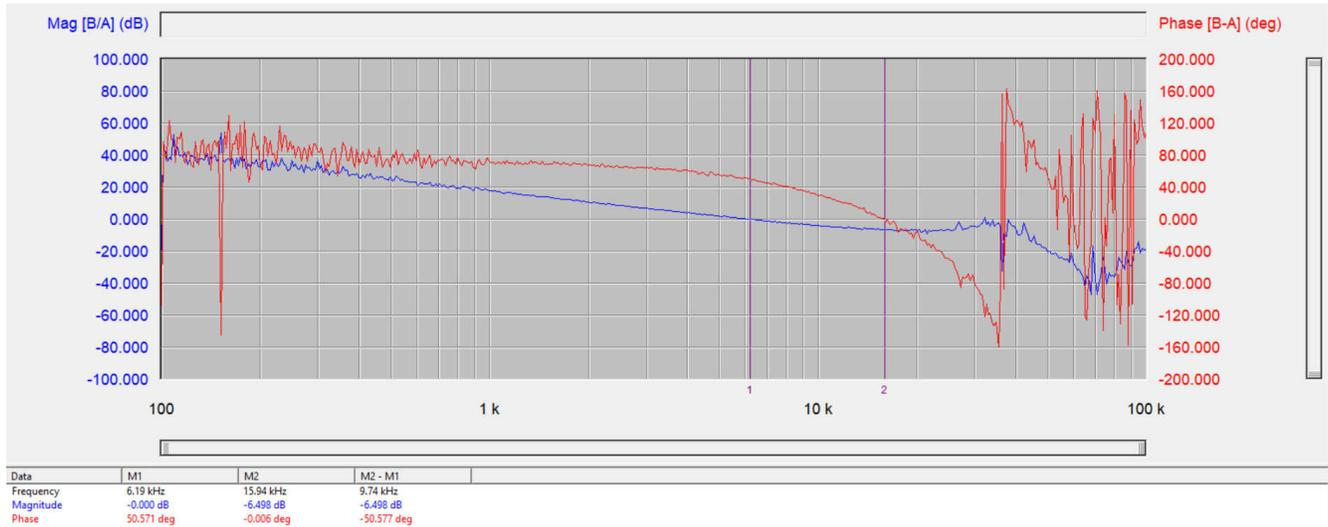
**Figure 2-3. Bode Plot Under 380-V 84-A Load;  $f_c$ : 6.19 kHz; Phase Margin: 50.571 deg; Magnitude Margin: 6.49 dB**
