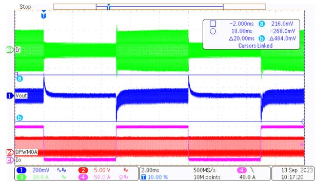
**Figure 3-4. Load Transient of 380-V, 0%-100%, 5 ms-5 ms, 2.5-A/μs Slew Rate**
