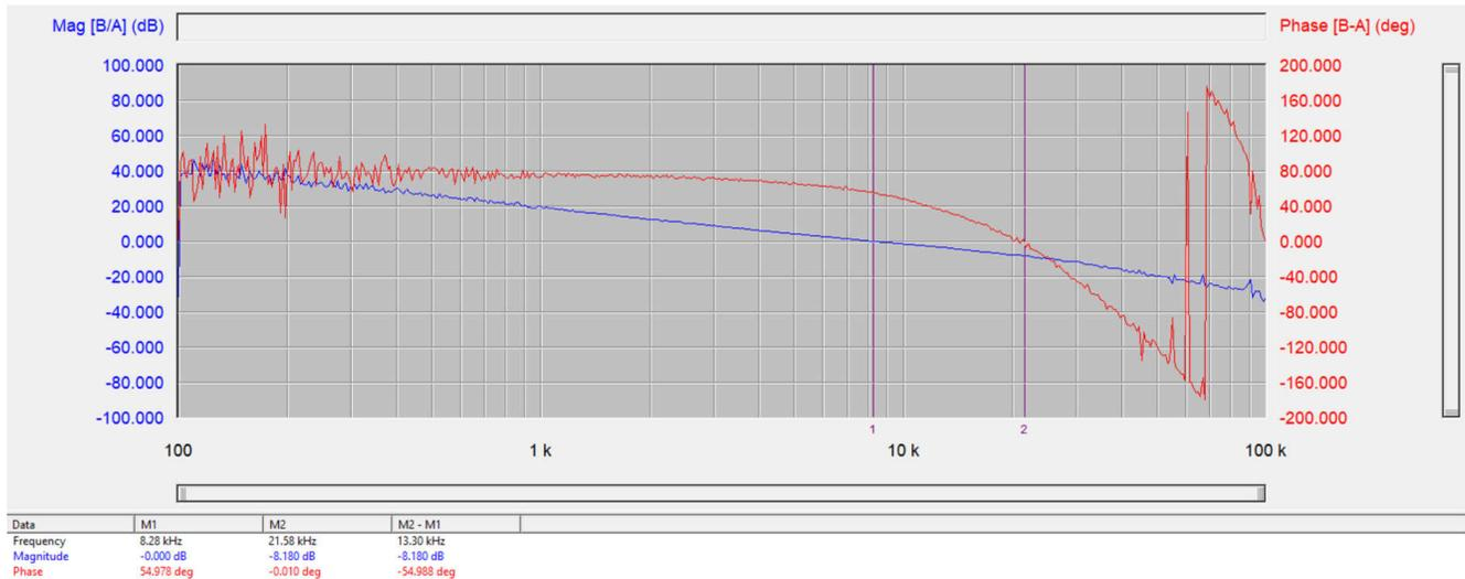
**Figure 2-4. Bode Plot Under 400-V 20-A Load;  $f_c$ : 8.28 kHz; Phase Margin: 54.978 deg; Magnitude Margin: 8.180 dB**
