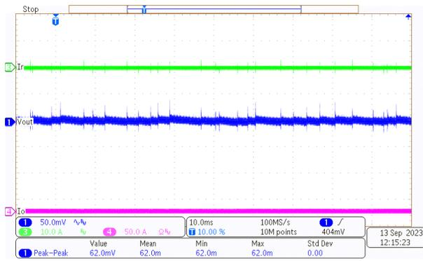
**Figure 3-14. Output Voltage Ripple Under 420-V, 0-A Load**
