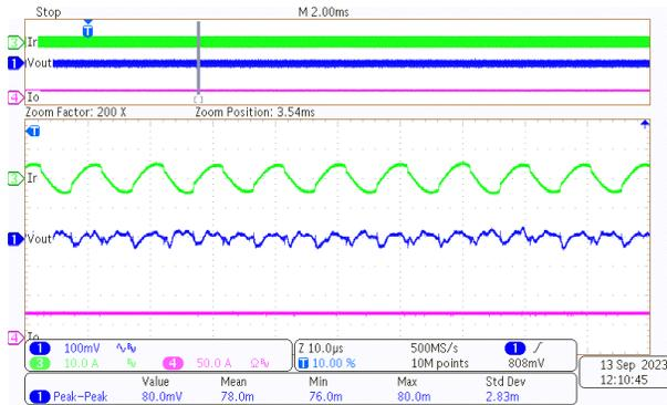
**Figure 3-12. Output Voltage Ripple Under 400-V, 40-A Load**
