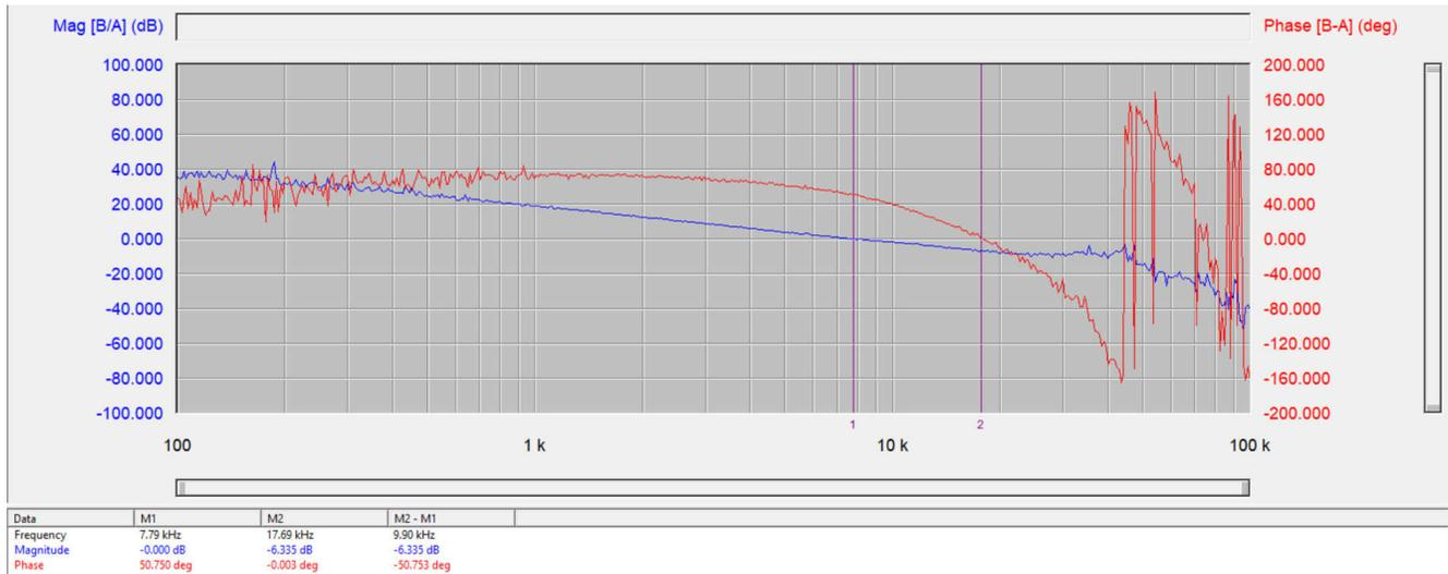
**Figure 2-6. Bode Plot Under 400-V 84-A Load;  $f_c$ : 7.79 kHz; Phase Margin: 50.750 deg; Magnitude Margin: 6.335 dB**
