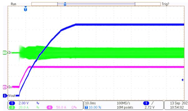
Figure 3-19. Start-Up With 400-V Input and 84-A Load
