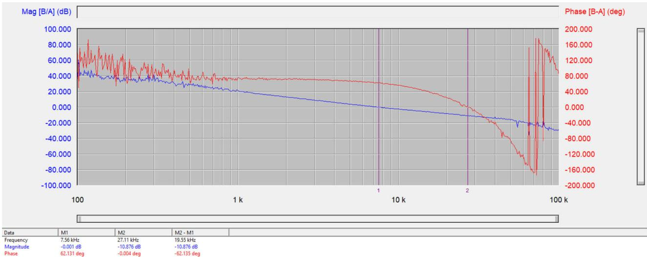
**Figure 2-8. Bode Plot Under 420-V 40-A Load;  $f_c$ : 7.56 kHz; Phase Margin: 62.131 deg; Magnitude Margin: 10.876 dB**
