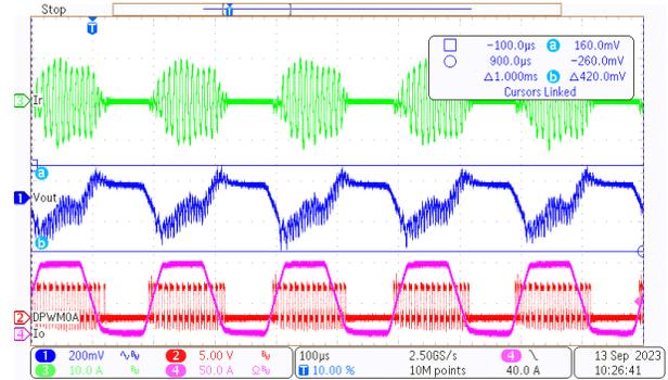
**Figure 3-2. Load Transient of 400-V, 0%-100%, 0.1 ms-0.1 ms, 2.5-A/μs Slew Rate**
