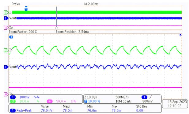
**Figure 3-15. Output Voltage Ripple Under 420-V, 40-A Load**
