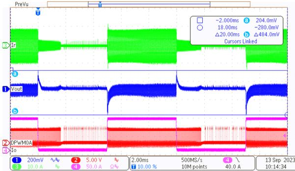
**Figure 3-1. Load Transient of 400-V, 0% -100%, 5 ms-5 ms, 2.5-A/μs Slew Rate**
