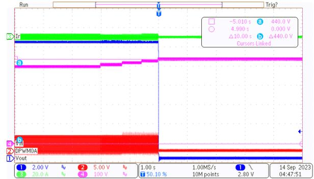
Figure 3-23. Shutdown When V<sub>IN</sub> is Above 440 V
