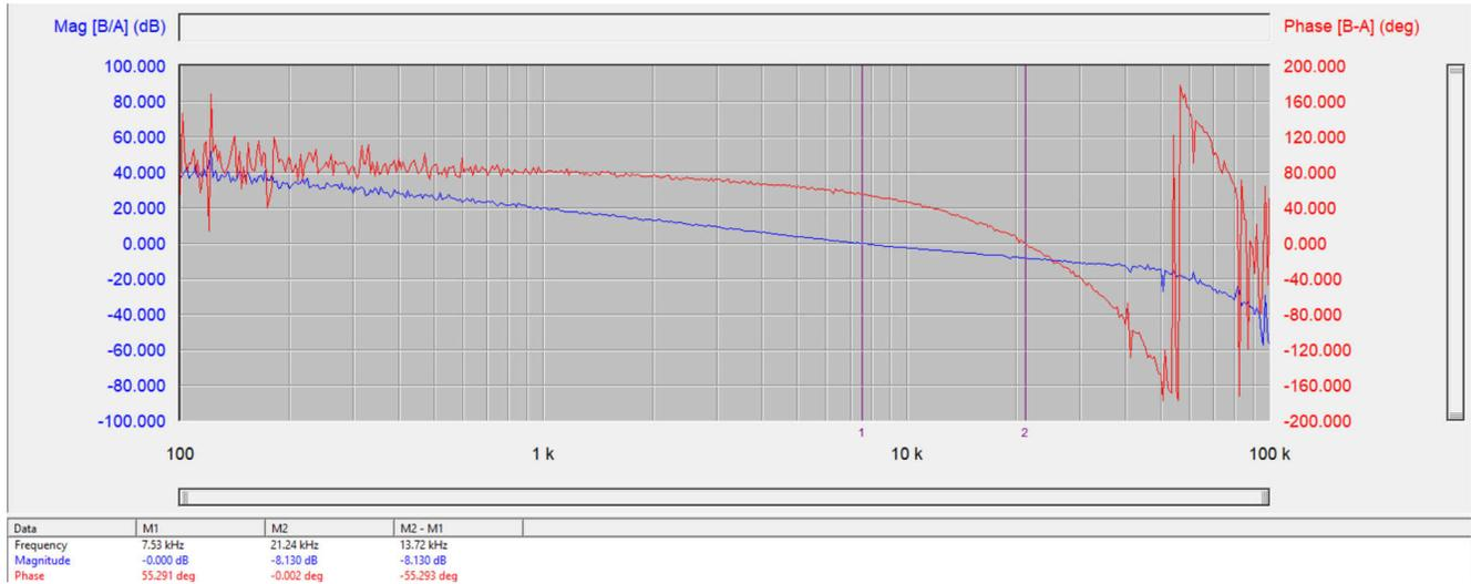
**Figure 2-5. Bode Plot Under 400-V 40-A Load;  $f_c$ : 7.53 kHz; Phase Margin: 55.291 deg; Magnitude Margin: 8.13 dB**
