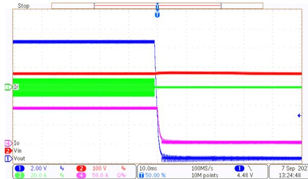
**Figure 3-20. Overcurrent Protection (90 A)**
