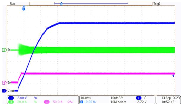
Figure 3-18. Start-Up With 400-V Input and 40-A Load
