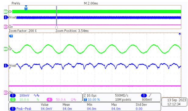
**Figure 3-9. Output Voltage Ripple Under 380-V, 40-A Load**
