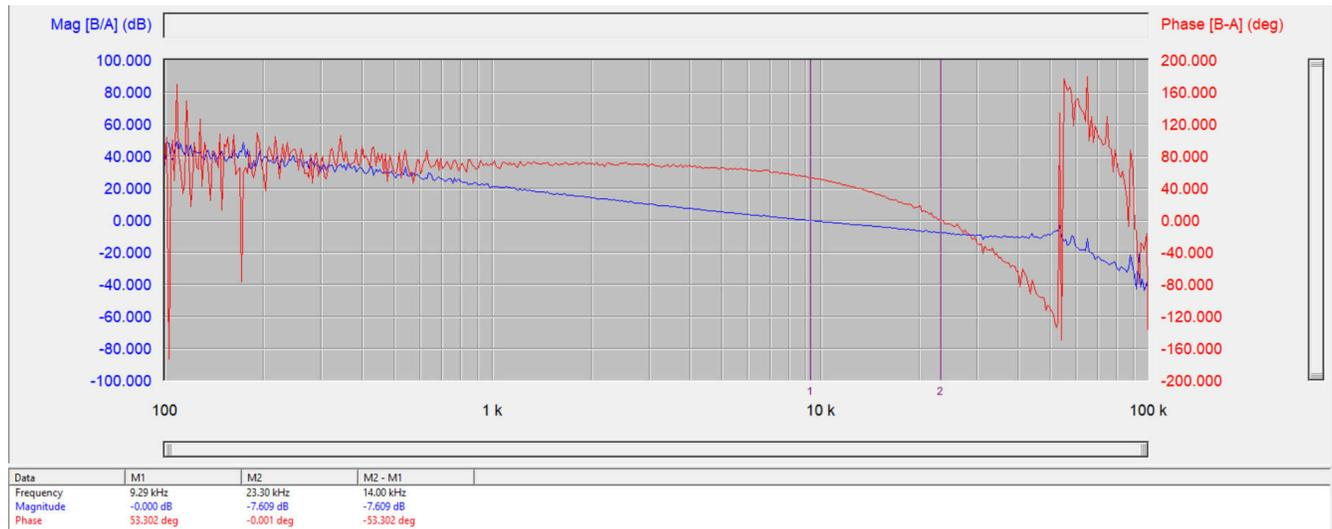
**Figure 2-9. Bode Plot Under 420-V 84-A Load;  $f_c$ : 9.19 kHz; Phase Margin: 51.353 deg; Magnitude Margin: 7.207 dB**
