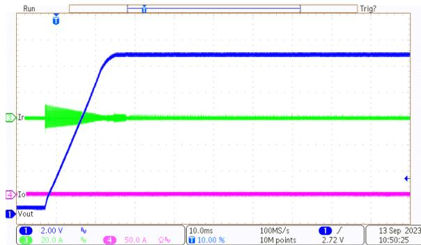
Figure 3-17. Start-Up With 400-V Input and 0-A Load
