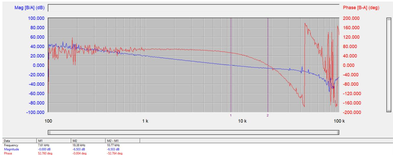
**Figure 2-2. Bode Plot Under 380-V 40-A Load;  $f_c$ : 7.61 kHz; Phase Margin: 52.760 deg; Magnitude Margin: 6.503dB**
