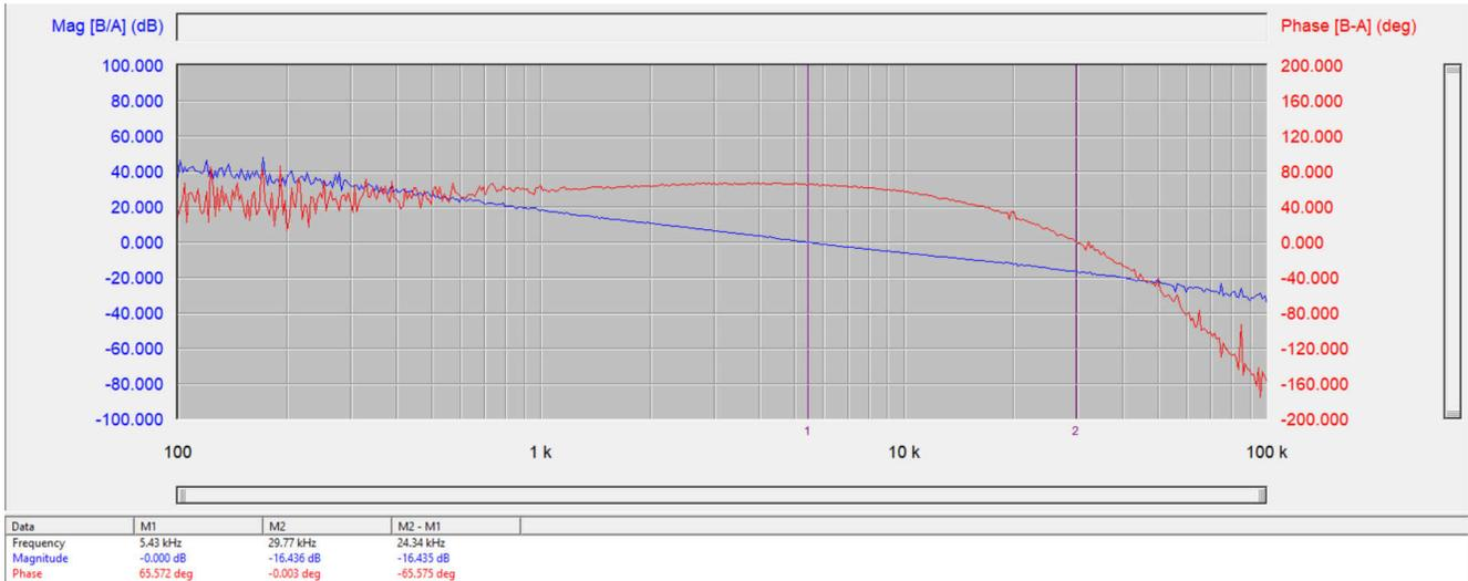
**Figure 2-7. Bode Plot Under 420-V 20-A Load;  $f_c$ : 5.43 kHz; Phase Margin: 65.572 deg; Magnitude Margin: 16.436 dB**
