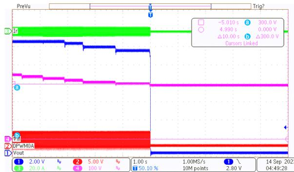
Figure 3-24. Shutdown When V<sub>IN</sub> is Below 300 V
