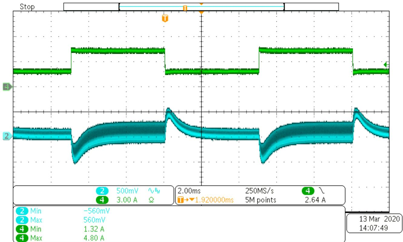
**Figure 3-6. Load Transient From 2 A to 4.5 A**
