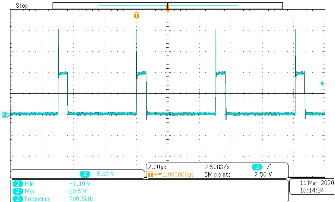
Figure 3-3. Switching Node at 1.5 V<sub>IN</sub> and 4.5-A Load Current [Scale: 5.0 V / div, 2.0 μs / div]
