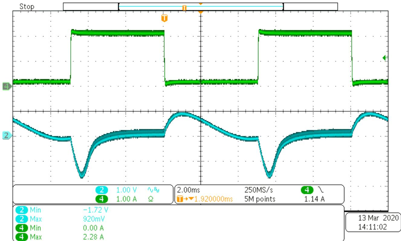
**Figure 3-5. Load Transient From 0.2 A to 2.2 A**
