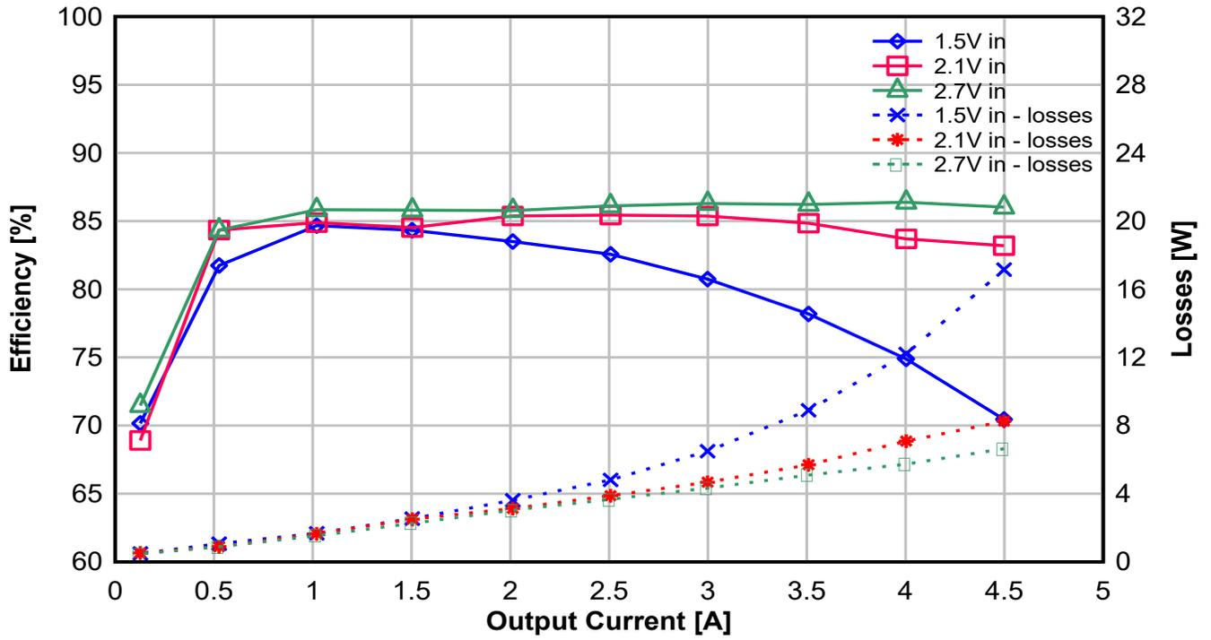
Figure 2-1. Efficiency Graph
