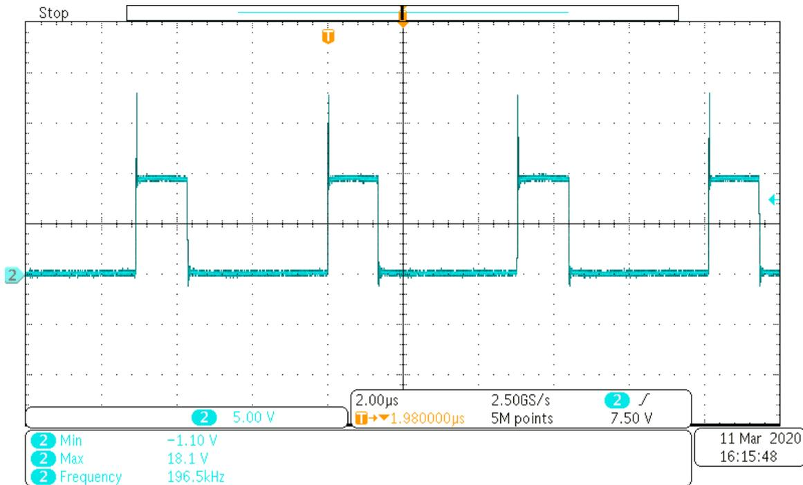
Figure 3-1. Switching Node at 2.7 V<sub>IN</sub> and 4.5-A Load Current [Scale: 5.0 V / div, 2.0 μs / div]
