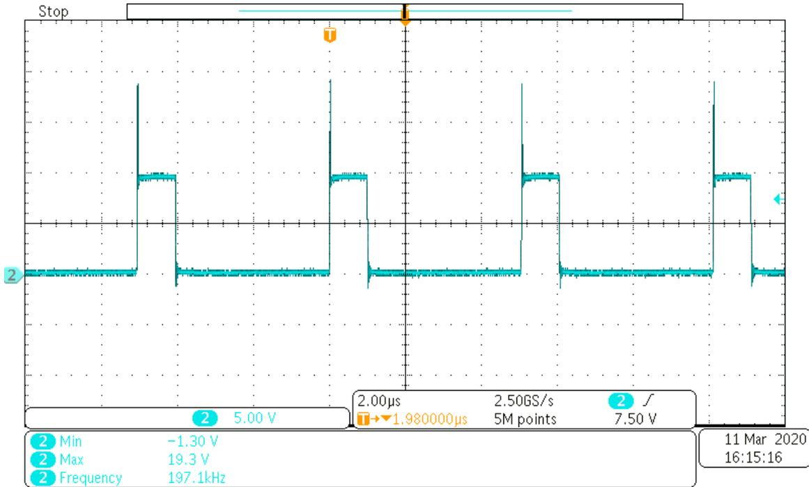
Figure 3-2. Switching Node at 2.1 V<sub>IN</sub> and 4.5-A Load Current [Scale: 5.0 V / div, 2.0 μs / div]
