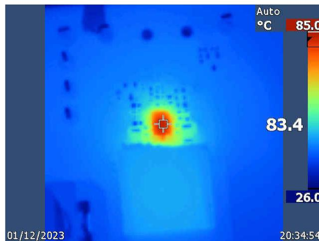
**Figure 2-3. Bottom Side of Board, 12-V Input, –8-V Output at 4-A Load;  $T_{\text{ambient}} \approx 26^{\circ}\text{C}$**
