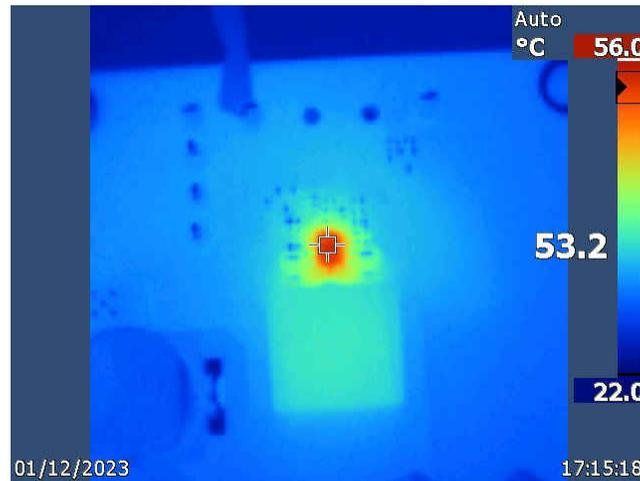
**Figure 2-2. Top Side of Board, 12-V Input, –8-V Output at 2.7-A Load;  $T_{\text{ambient}} \approx 22^{\circ}\text{C}$**
