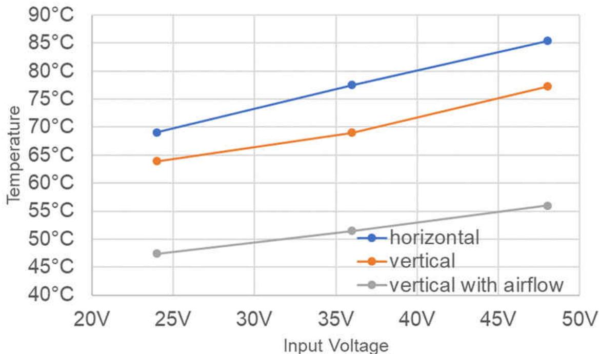
**Figure 2-5. Temperature of Hottest Spot vs Input Voltage at 110% Load 55 A**
