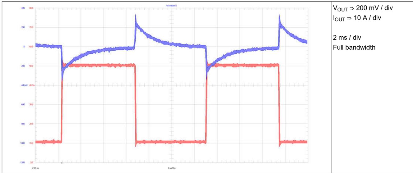
Figure 3-15. Load Transient 10 A to 50 A, Transient Response 350 mV<sub>PK</sub>
