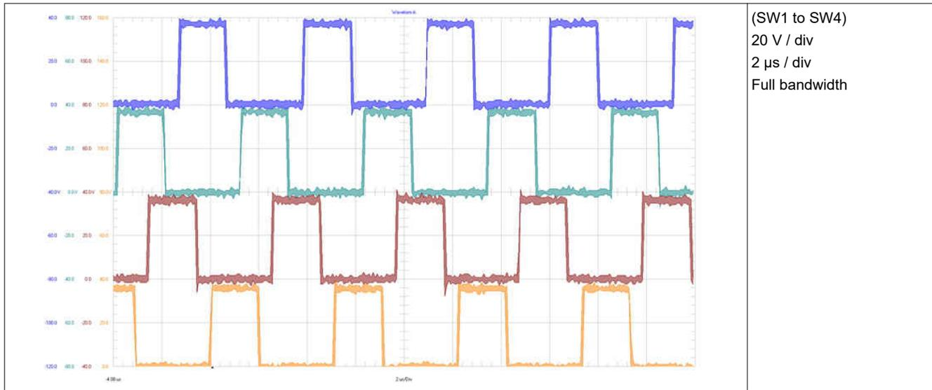
**Figure 3-2. Four Switching Phases at 0, 90, 180, 270 Degrees Phase Shift at 36 V<sub>IN</sub>**
