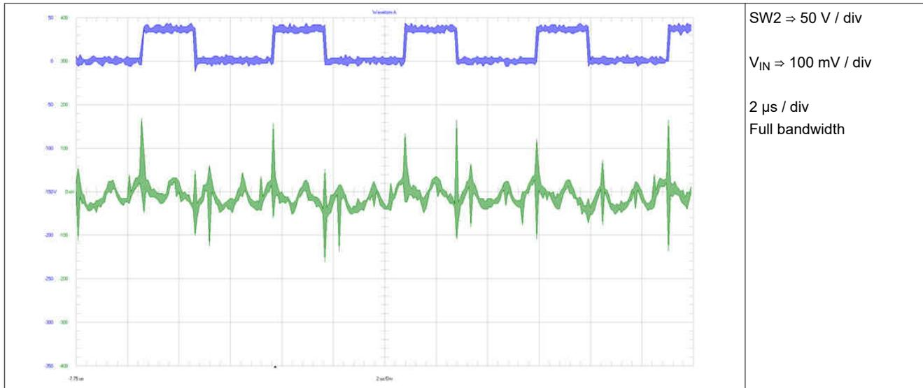
Figure 3-13. Voltage Ripple: Power Stage Input (AC Coupled) at 36-V Input Voltage
