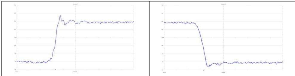
Figure B-3. Waveform at the Switch-Node Q7 Drain to GND
