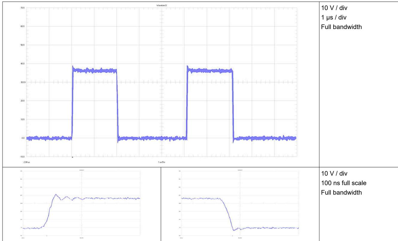
**Figure 3-4. Waveform Switch Node to GND**
