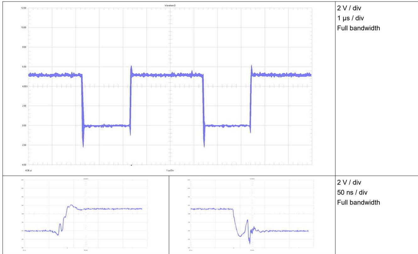
**Figure 3-5. Waveform Low-Side FET to GND**
