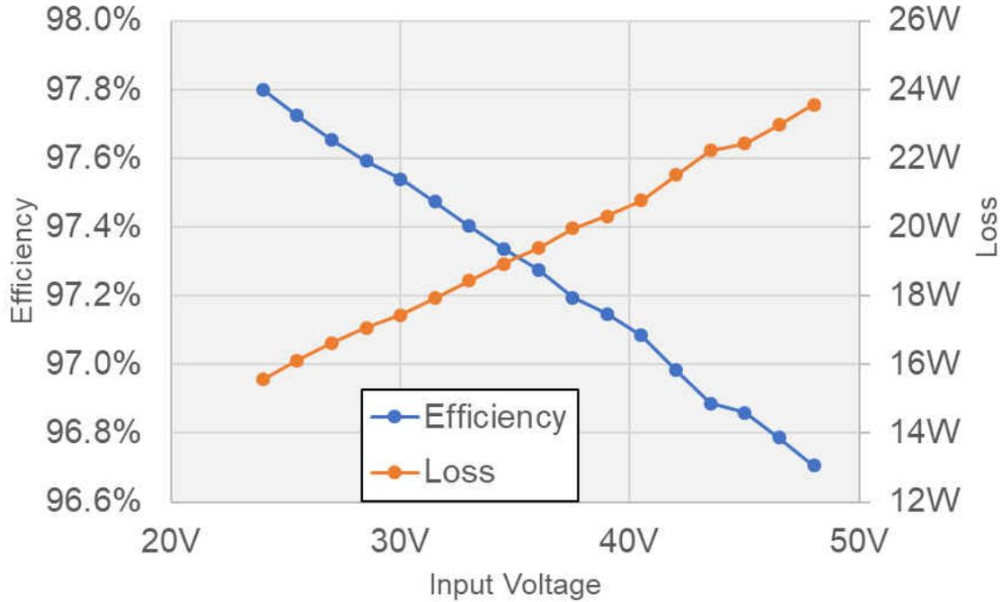
Figure 2-3. Efficiency and Loss vs Input Voltage at Full Load 50 A
