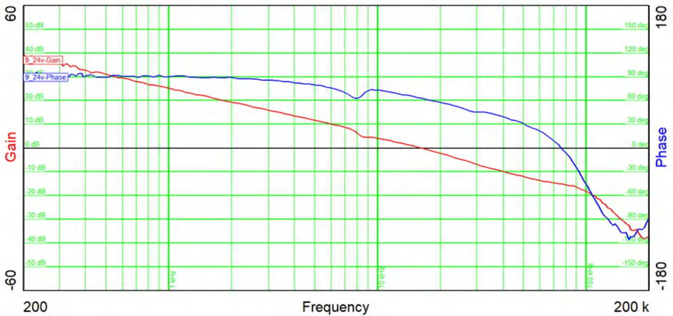
Figure 2-6. Bode Plot at 24-V Input Voltage
