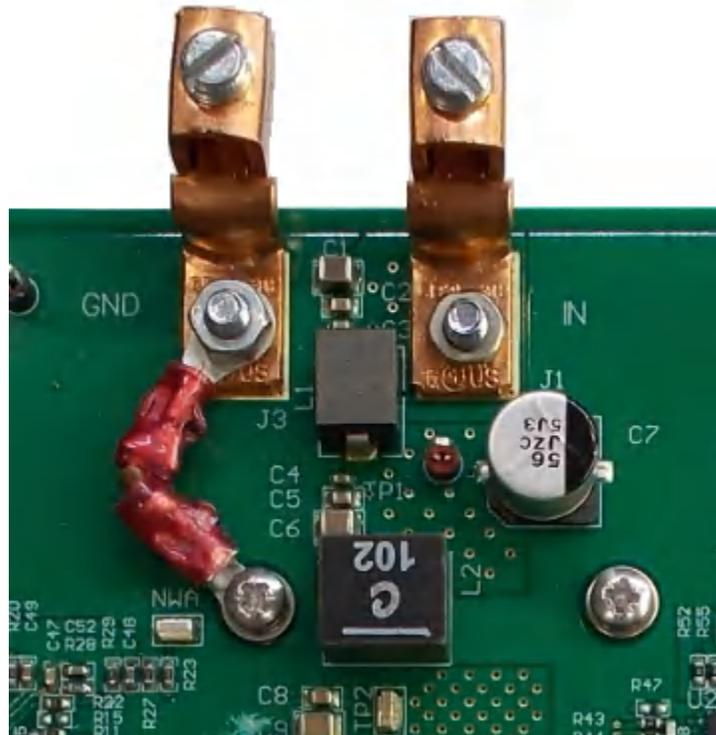
**Figure C-2. GND Connection**
