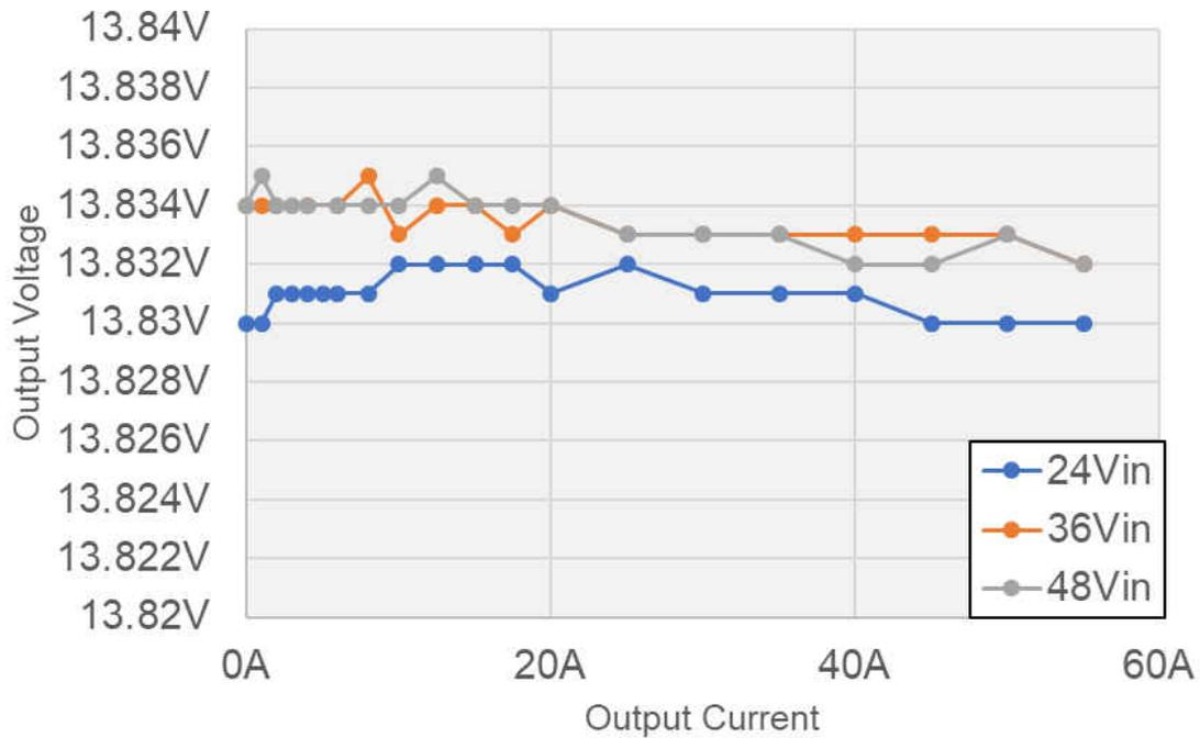
Figure 2-4. Output Voltage vs Output Current
