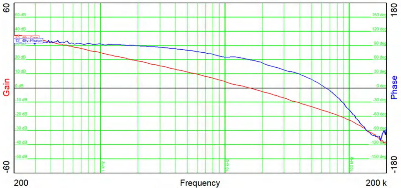
Figure 2-8. Bode Plot at 48-V Input Voltage
