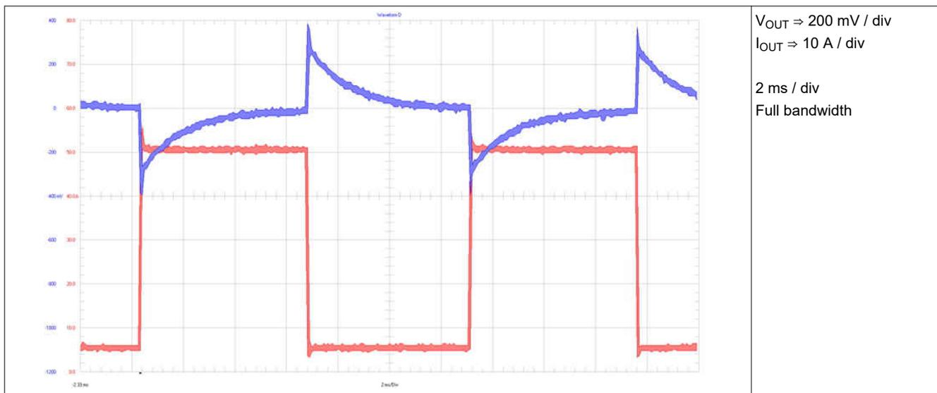
Figure 3-16. Load Transient 5 A to 50 A, Transient Response 400 mV<sub>PK</sub>, Less Than 3%
