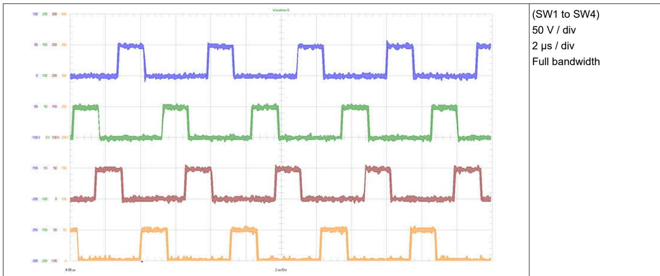
**Figure 3-3. Four Switching Phases at 0, 90, 180, 270 Degrees Phase Shift at 48 V<sub>IN</sub>**
