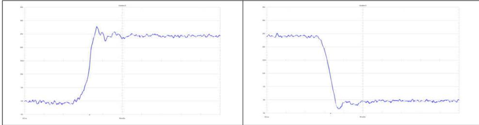
Figure B-1. Waveform at the Switch-Node Q3 Drain to GND
