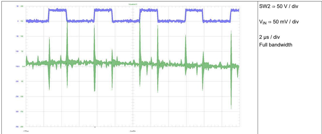
Figure 3-10. Voltage Ripple: Board Input (AC Coupled) at 36-V Input Voltage
