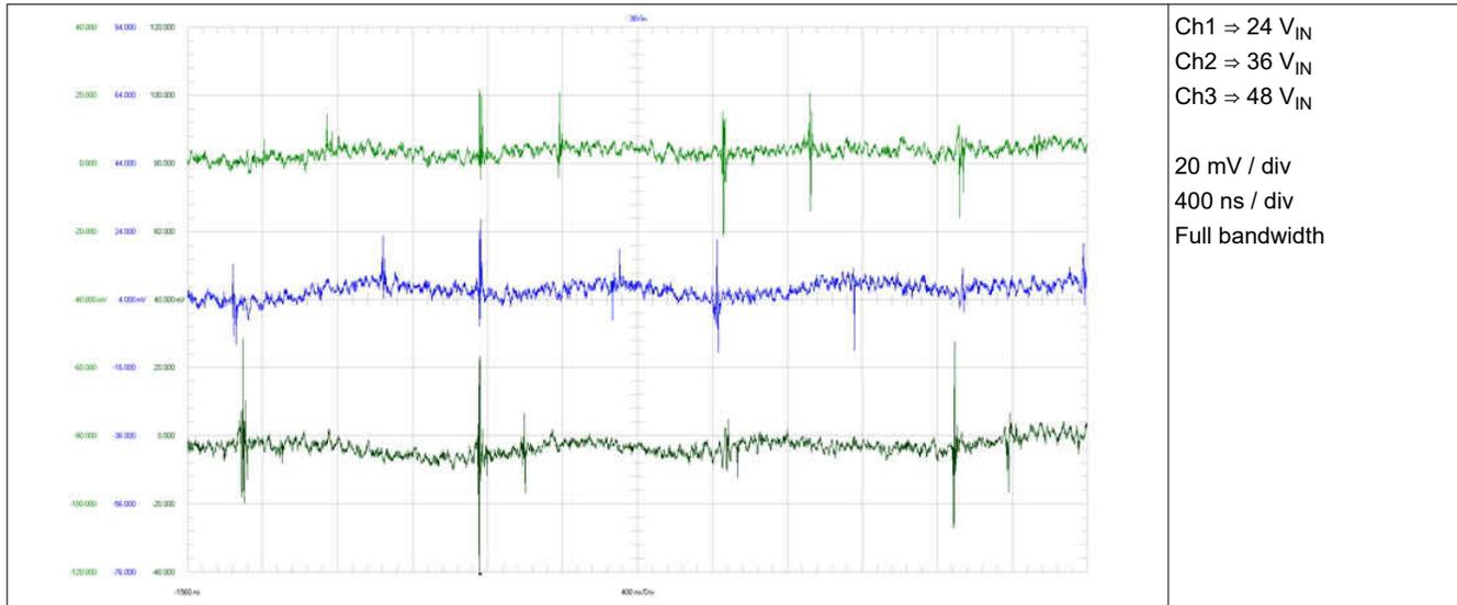
Figure 3-8. Output Voltage Ripple < 10 mV<sub>PP</sub> (AC Coupled), Noise < 30 mV<sub>PK</sub>
