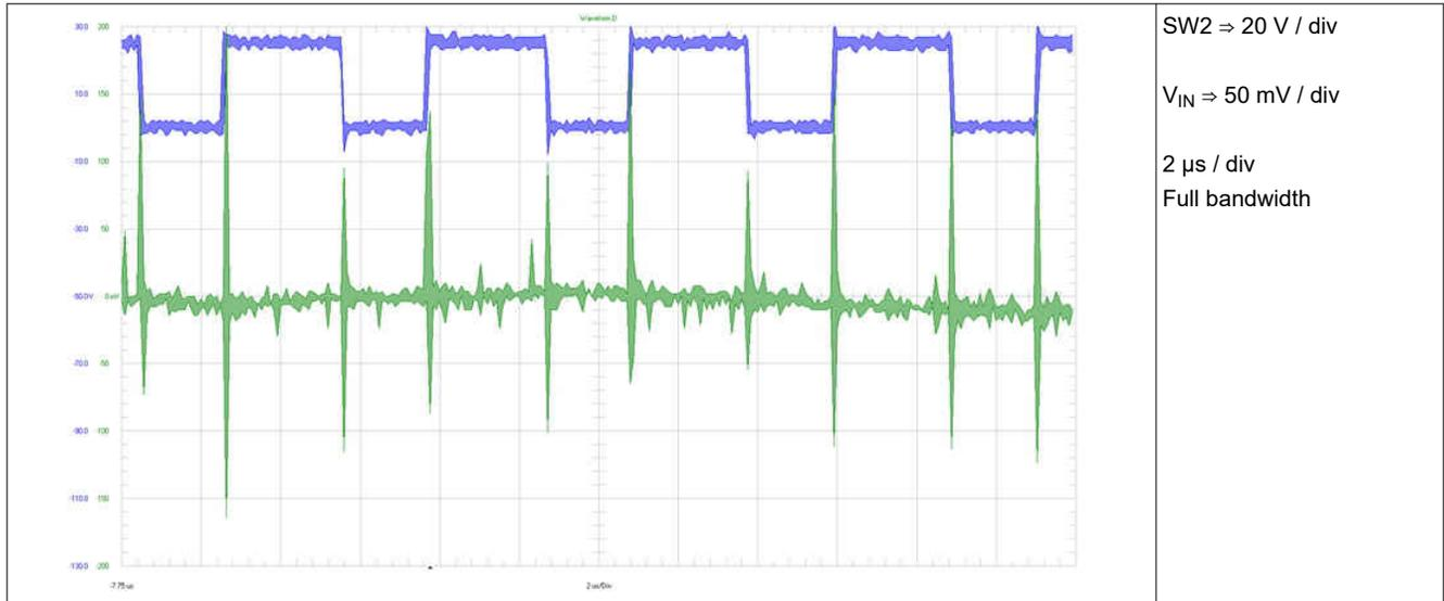
Figure 3-9. Voltage Ripple: Board Input (AC Coupled) at 24-V Input Voltage
