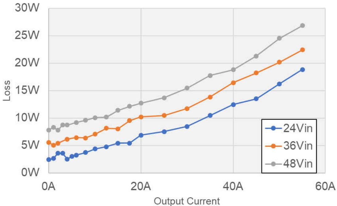
**Figure 2-2. Loss vs Output Current**
