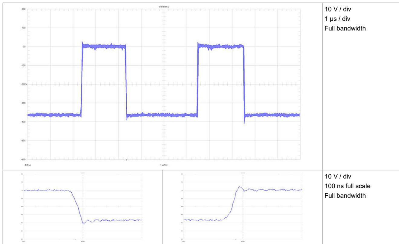
**Figure 3-6. Waveform Switch Node to  $V_{IN}$**
