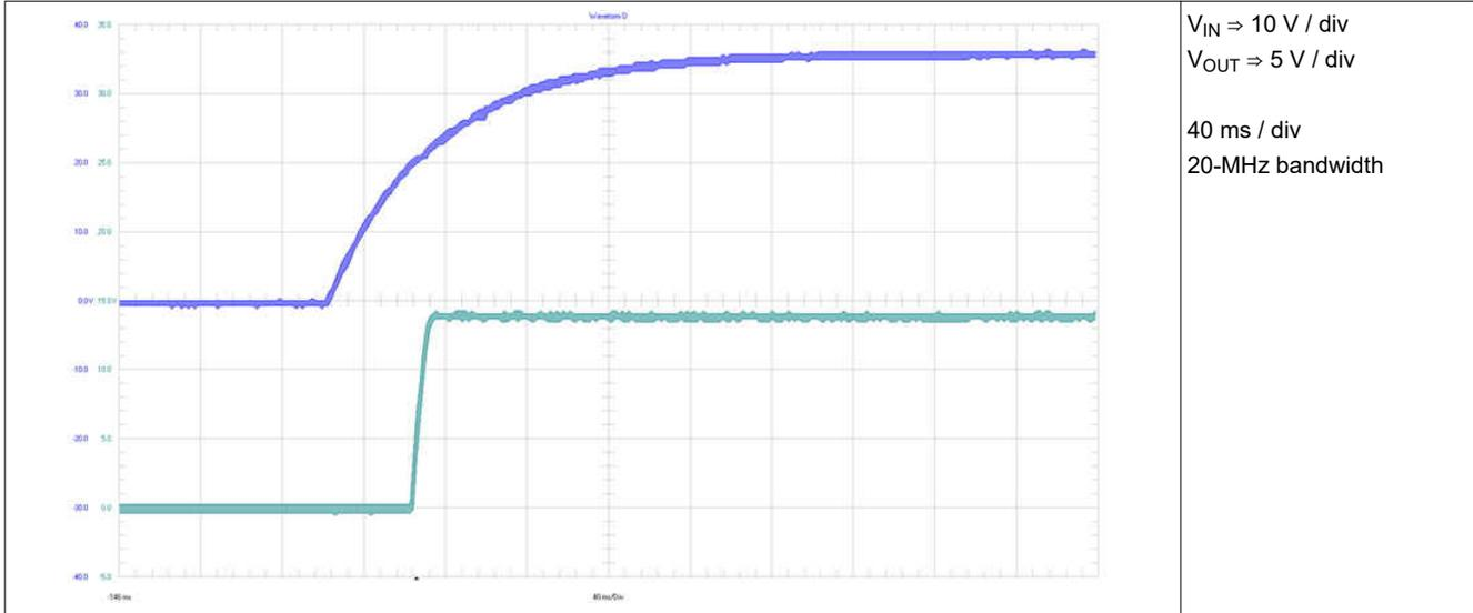
Figure 3-17. Start-Up (Soft Start 10 ms, set via Capacitor C49 = 330 nF)
