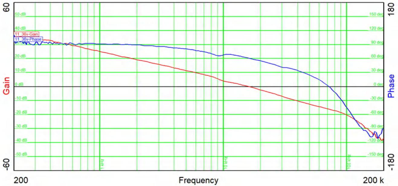
Figure 2-7. Bode Plot at 36-V Input Voltage
