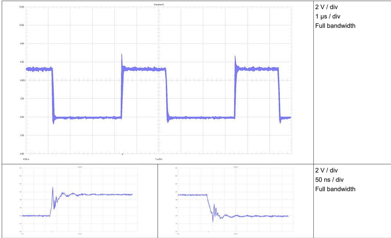
Figure 3-7. Waveform Low-Side FET Gate to Switch Node
