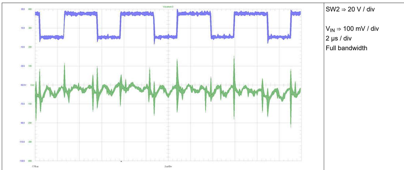
**Figure 3-12. Voltage Ripple: Power Stage Input (AC Coupled) at 24-V Input Voltage**
