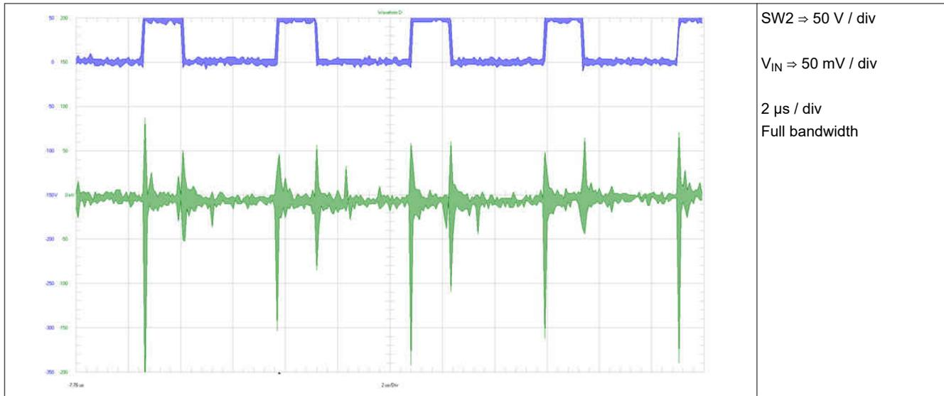
**Figure 3-11. Voltage Ripple: Board Input (AC Coupled) at 36-V Input Voltage**
