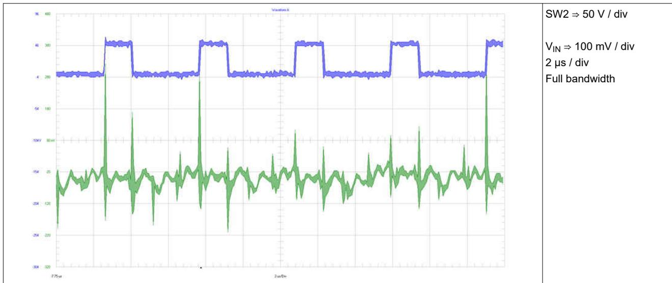
Figure 3-14. Voltage Ripple: Power Stage Input (AC Coupled) at 48-V Input Voltage
