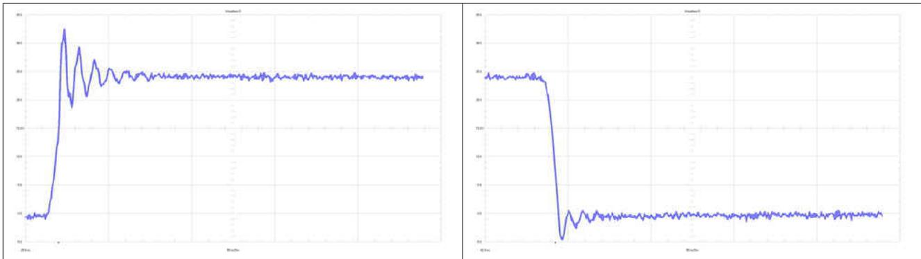
**Figure A-1. Waveform at the Switch Node With 2.21-Ω and 4.75-Ω Resistor**
