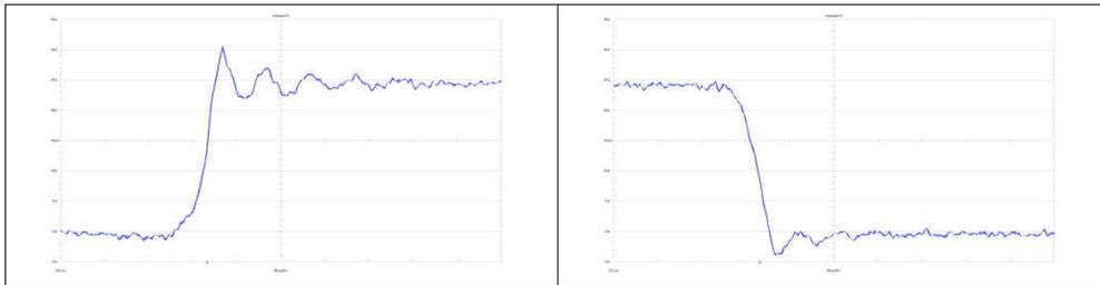
Figure B-2. Waveform at the Switch-Node Q4 Drain to GND
