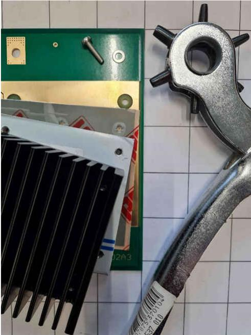
**Figure C-1. Stack: PCB – Thermal Foil – Adapter - Heat Sink**
