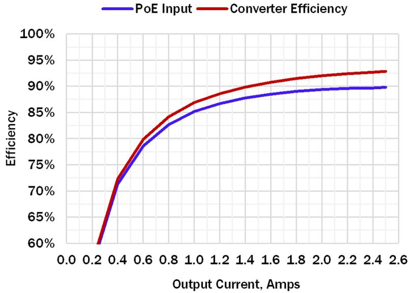
Figure 2-1. PMP23287 Rev. A Efficiency Graph, PoE Diode Bridge
