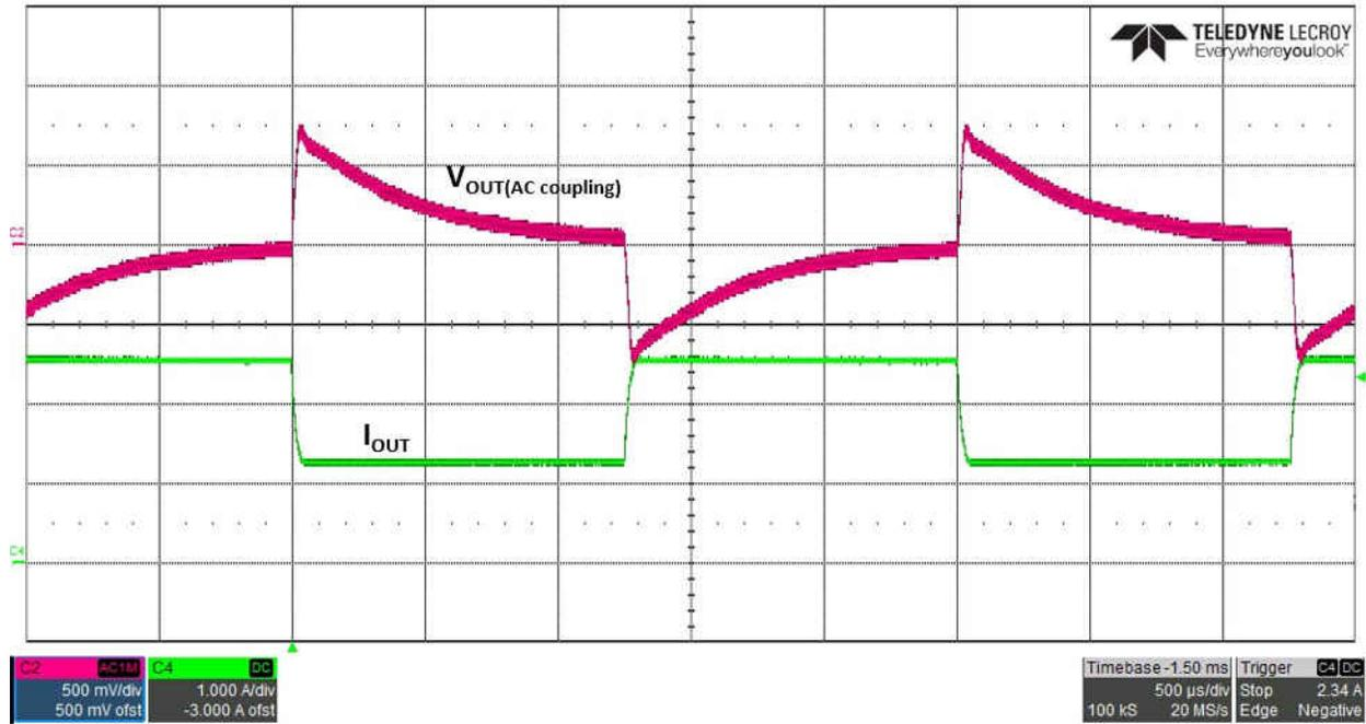
Figure 3-9. Output Load Step Response, 1.25-A to 2.50-A Load Step
