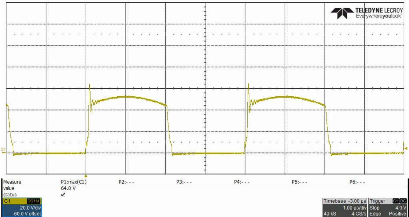
Figure 3-4. Voltage Drain-to-Source, Q8, 57-V Input, 2.5-A Load, Measured 64.0-V  $V_{peak}$
