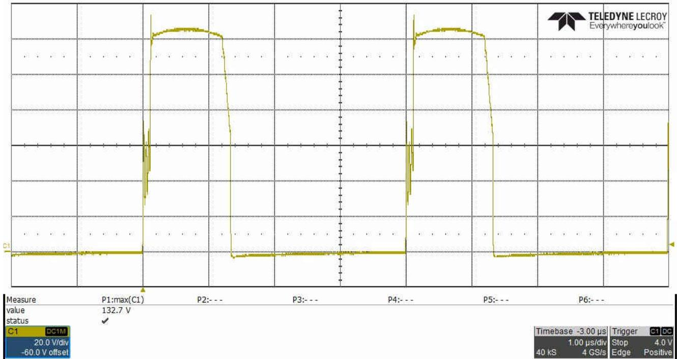
Figure 3-5. Voltage Drain-to-Source, Q10, 37-V Input, 2.5-A Load, Measured 132.7-V  $V_{peak}$
