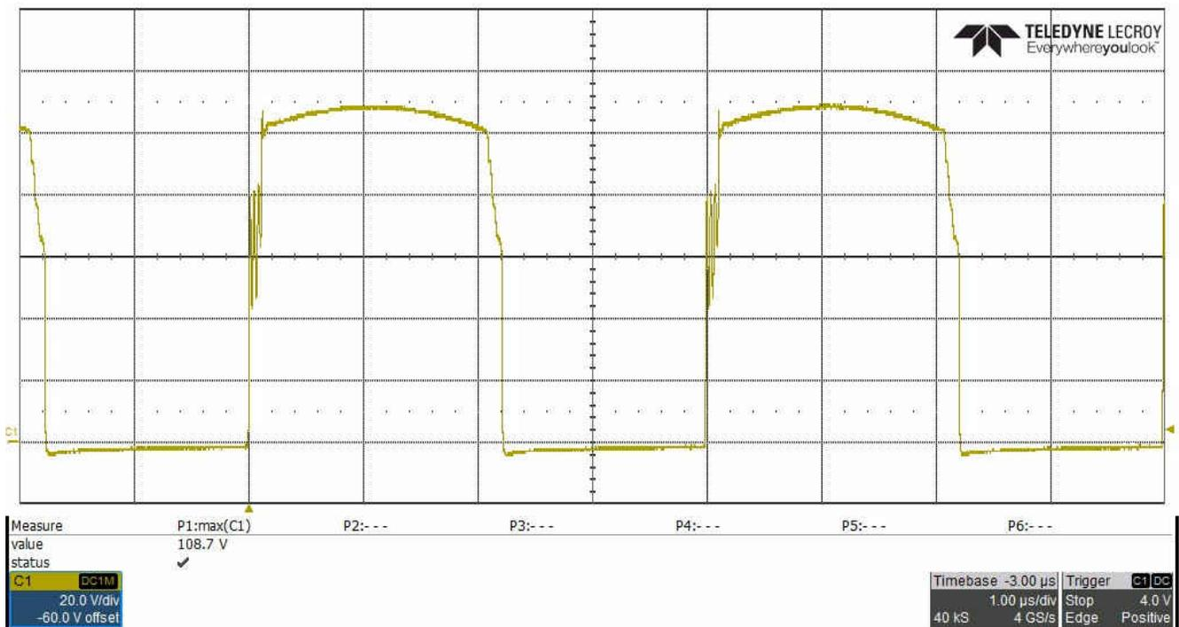
Figure 3-6. Voltage Drain-to-Source, Q10, 57-V Input, 2.5-A Load, Measured 108.7-V  $V_{peak}$
