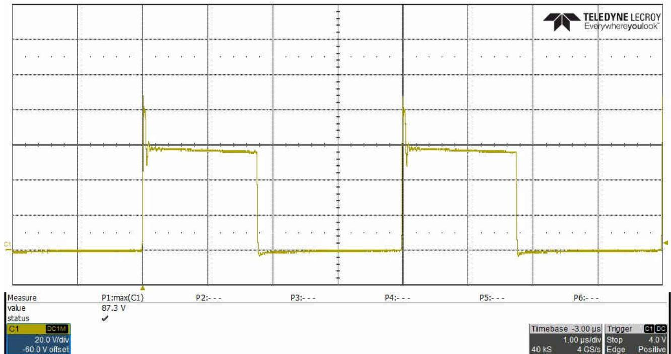
Figure 3-2. Voltage Drain-to-Source, Q6, 57-V Input, 2.5-A Load, Measured 87.3-V  $V_{peak}$
