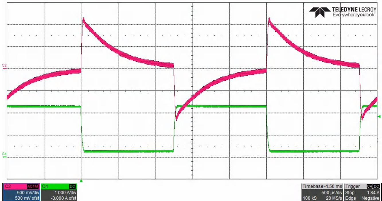
Figure 3-10. Output Load Step Response, 0.25-A to 2.25-A Load Step
