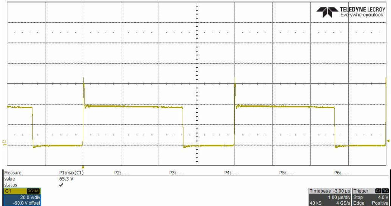
Figure 3-1. Voltage Drain-to-Source, Q6, 37-V Input, 2.5-A Load, Measured 65.3-V  $V_{peak}$
