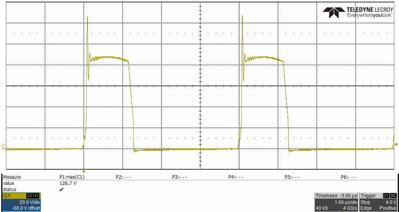
Figure 3-3. Voltage Drain-to-Source, Q8, 37-V Input, 2.5-A Load, Measured 126.7-V  $V_{peak}$
