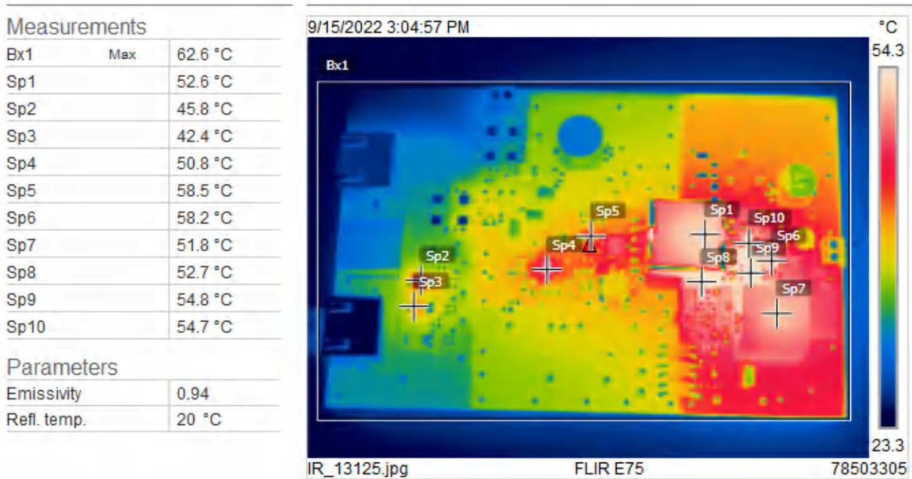
Figure 2-3. Top Thermal Image, 48-V Input, 2-A Load
