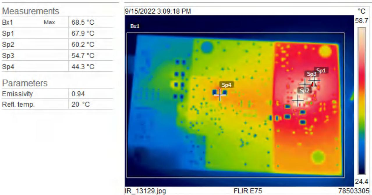
Figure 2-4. Bottom Thermal Image, 48-V Input, 2-A Load
