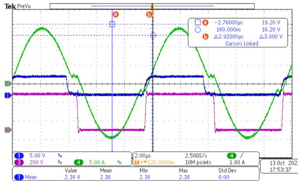
CH1: SR VGS, CH3: PRI MOS VDS, CH4: Resonant Tank Current
