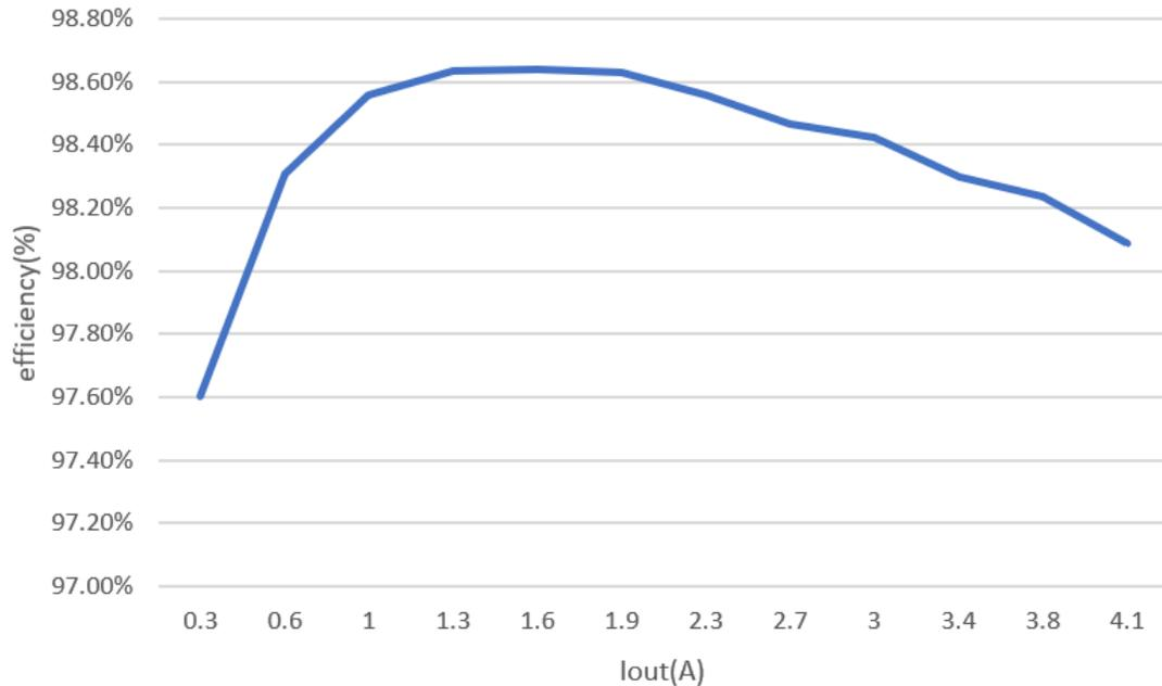
Figure 2-1. PFC Efficiency Graph
