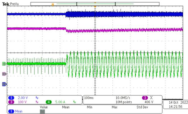
CH1: Output Voltage, CH3: VBUS, CH4: Input Current
