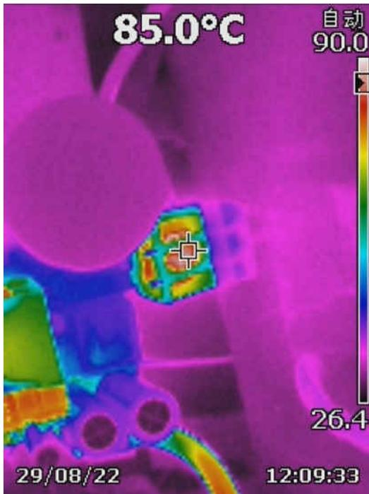
Figure 2-5. Resonant Inductor
