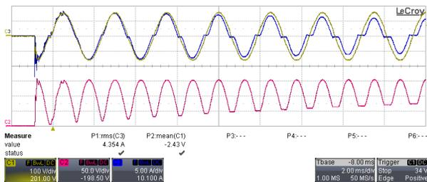
Figure 3-14. Time Division: 2 ms/div, (C2:  $V_{PFC}$ , C1:  $V_{IN}$ , C3:  $I_{IN}$ )
