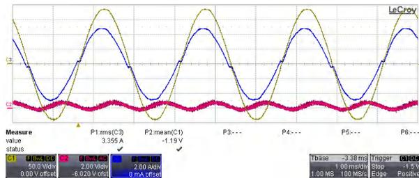
**Figure 3-8.  $V_{IN} = 134$  VAC,  $F = 400$  Hz**
