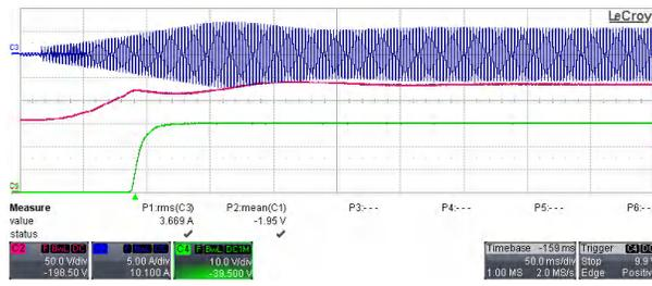
Figure 3-18. 13-A Load (C2:  $V_{PFC}$ , C4:  $V_{OUT}$ , C3:  $I_{IN}$ )
