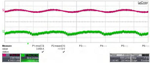
**Figure 3-5. PFC and  $V_{OUT}$  Voltage Ripple at Timebase = 500  $\mu$ s/div**
