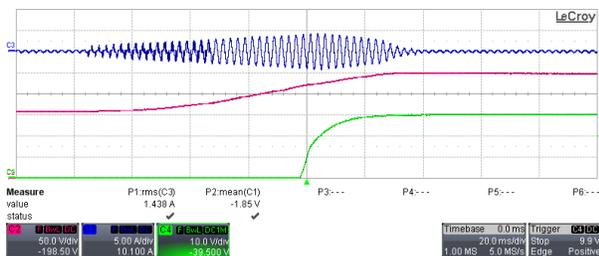
Figure 3-16. No Load (C2:  $V_{PFC}$ , C4:  $V_{OUT}$ , C3:  $I_{IN}$ )
