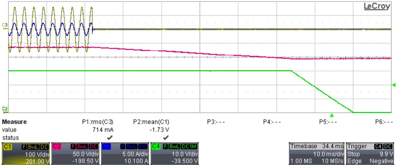
Figure 3-19. Behavior of V<sub>PFC</sub> and V<sub>OUT</sub> During Shutdown (C1: V<sub>IN</sub>, C2: V<sub>PFC</sub>, C3: I<sub>IN</sub>, C4: V<sub>OUT</sub>)
