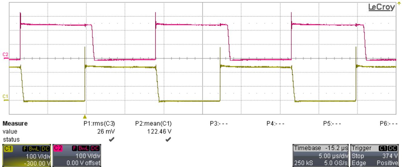
Figure 3-1. Drain-Source Voltages on Q1 and Q12 (C1: Q12-Vds, C2: Q1-Vds) at 96 VAC
