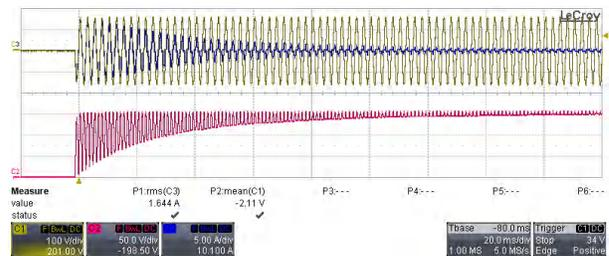
Figure 3-15. Time Division: 20 ms/div, (C2:  $V_{PFC}$ , C1:  $V_{IN}$ , C3:  $I_{IN}$ )
