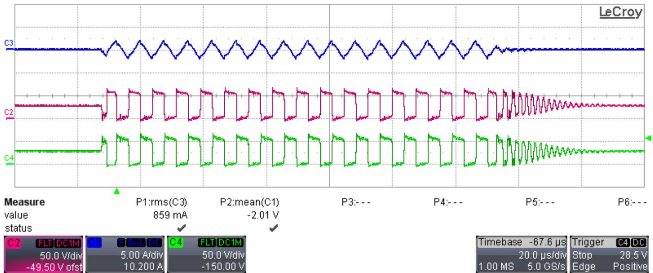
Figure 3-3. Burst Mode Waveforms (C4: Q7-Vds, C3: I(L7), C2: Q5-Vds) at 115 VAC and 200-mA Load
