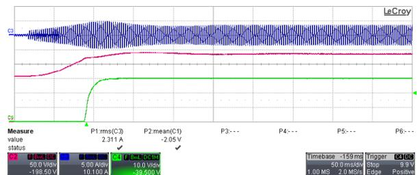
Figure 3-17. 8-A Load (C2:  $V_{PFC}$ , C4:  $V_{OUT}$ , C3:  $I_{IN}$ )
