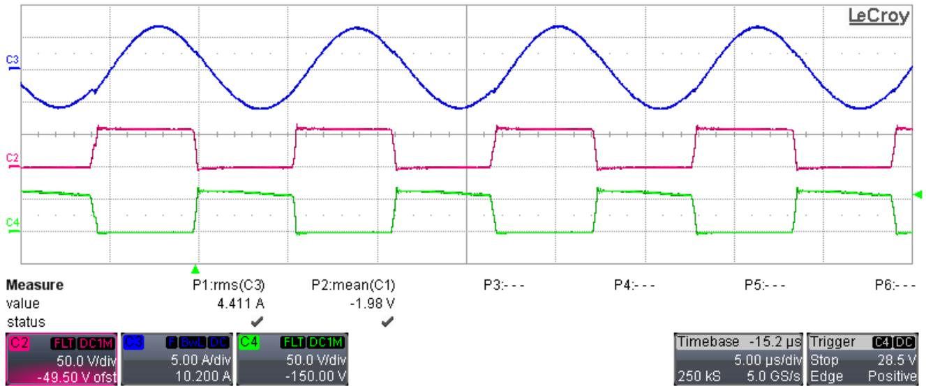
Figure 3-2. Drain-Source Voltages and Resonant Current at 115 VAC (C4: Q7-Vds, C3: I(L7), C2: Q5-Vds)
