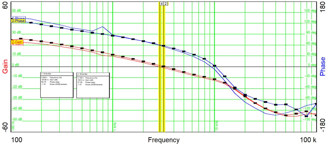
Figure 2-7. Bode Plot at 5 A and 13 A Load Current
