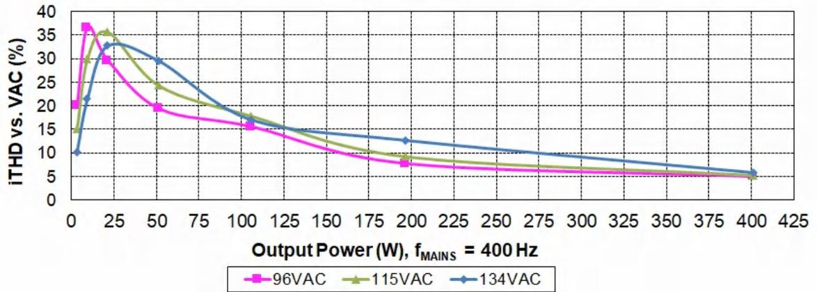
Figure 2-4. iTHD Versus Output Power at 400 Hz
