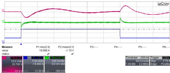
Figure 3-12.  $V_{IN} = 96$  VAC (C2:  $V_{PFC}$ , C3:  $I_{OUT}$ , C4:  $V_{OUT}$ )
