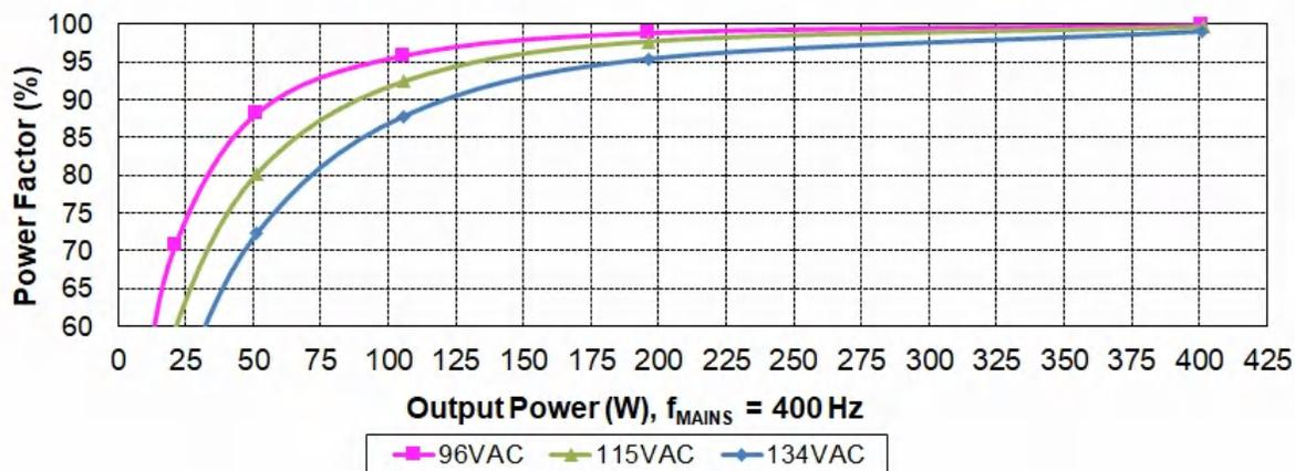
**Figure 2-2. Power Factor Versus Output Power at 400 Hz**
