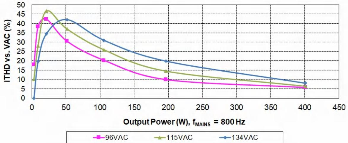
Figure 2-5. iTHD Versus Output Power at 800 Hz
