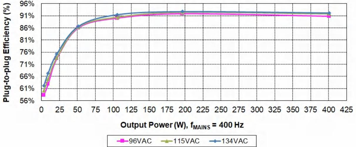
Figure 2-1. Efficiency Graph for Three Different VAC Input Voltages, Versus Output Power
