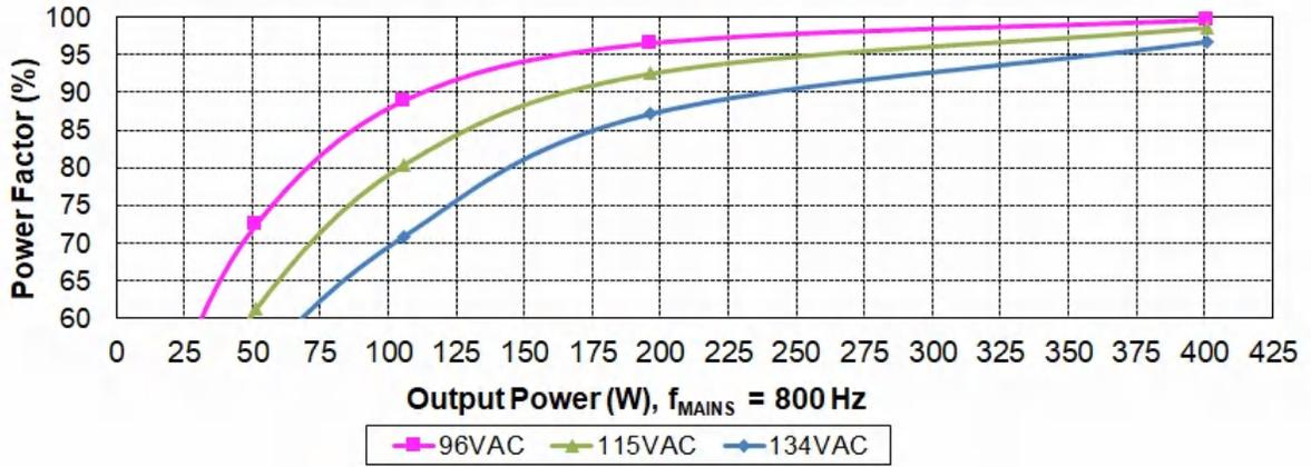
Figure 2-3. Power Factor Versus Output Power at 800 Hz
