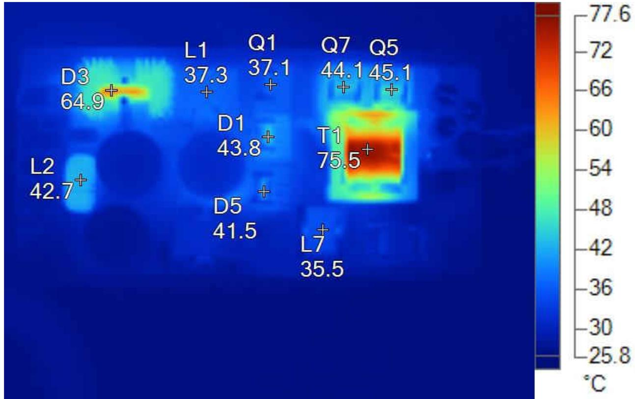
Figure 2-6. Thermal Image, 30 Minutes, Full Load
