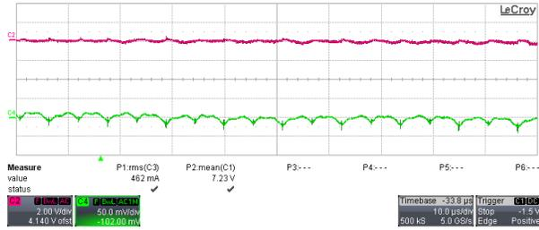
**Figure 3-4. PFC and  $V_{OUT}$  Voltage Ripple (C2:  $V_{PFC}$ , C4:  $V_{OUT}$ )**
