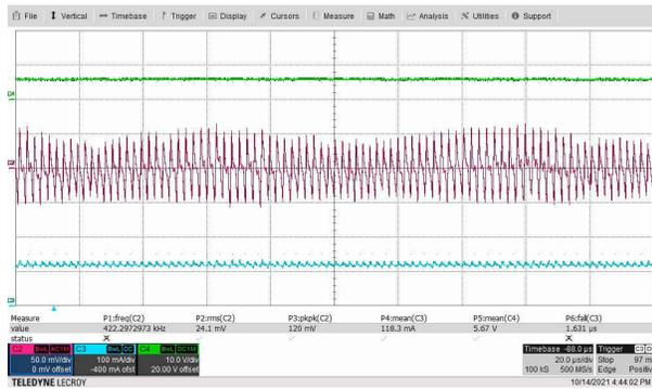
**Figure 3-5. Output Voltage Ripple With 445-kHz Switching Frequency**
