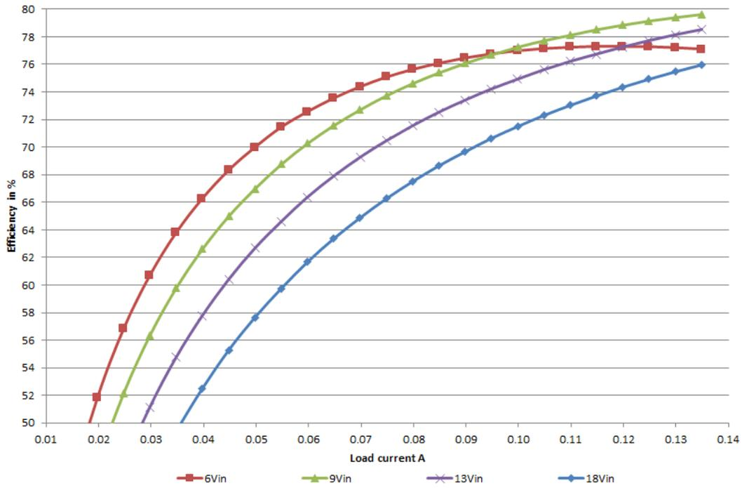
Figure 2-3. Efficiency of the PMP22817 SEPIC at 2 MHz
