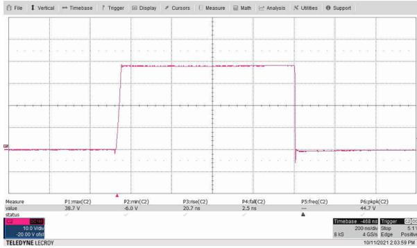
**Figure 3-1. Switching at 18-V<sub>IN</sub> Q1 Drain Full Load at 445 kHz Showing Only 1 Pulse**
