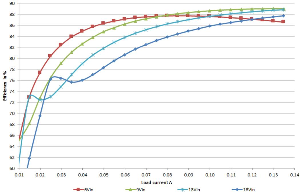
Figure 2-1. Efficiency of the PMP22817 SEPIC at 445 kHz
