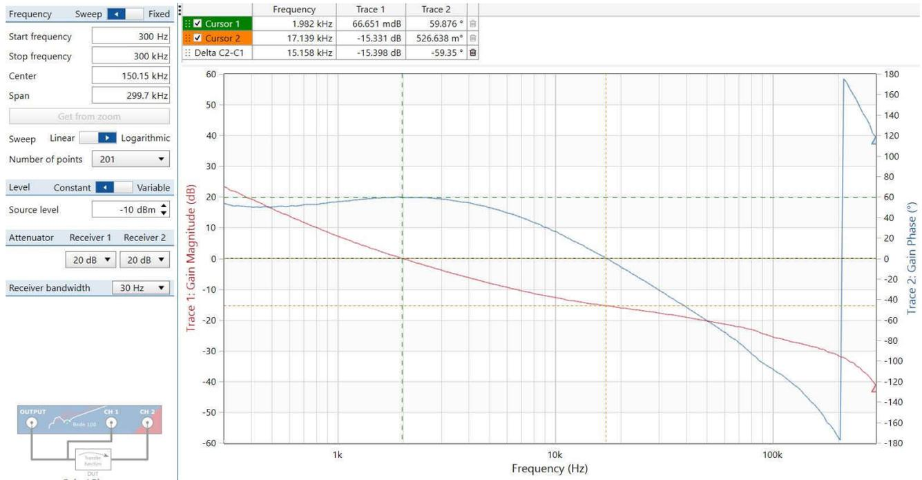
Figure 2-5. Bode Plot at 445-kHz Switching Frequency
