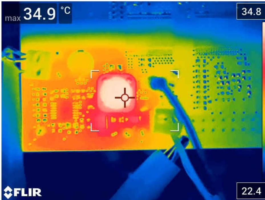
$V_{IN} = 18\text{ V}_{IN}$ ,  $V_{OUT} = 24\text{ V}_{OUT}$  at 130 mA
