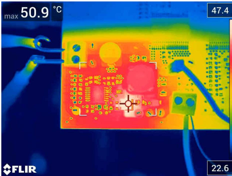
$V_{IN} = 18\text{ V}$ ,  $V_{OUT} = 24\text{ V}_{OUT}$  at 130 mA
