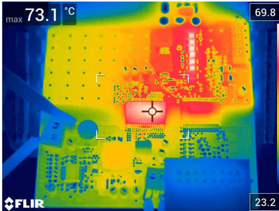
12  $V_{IN}$  to SEPIC, 24 V from SEPIC, +15 V, -5 V from isolated DC/DC. Isolated driver run at 40 kHz, 50% duty into 0.1- $\mu$ F load for 2  $\mu$ C per cycle or 80 mA, 1.6-W average current, power draw from isolated DC/DC. Ambient 21°C to 23°C with no fan. Isolated DC/DC at 73°C, gate driver at 56°C and gate drive resistors up to 76°C
