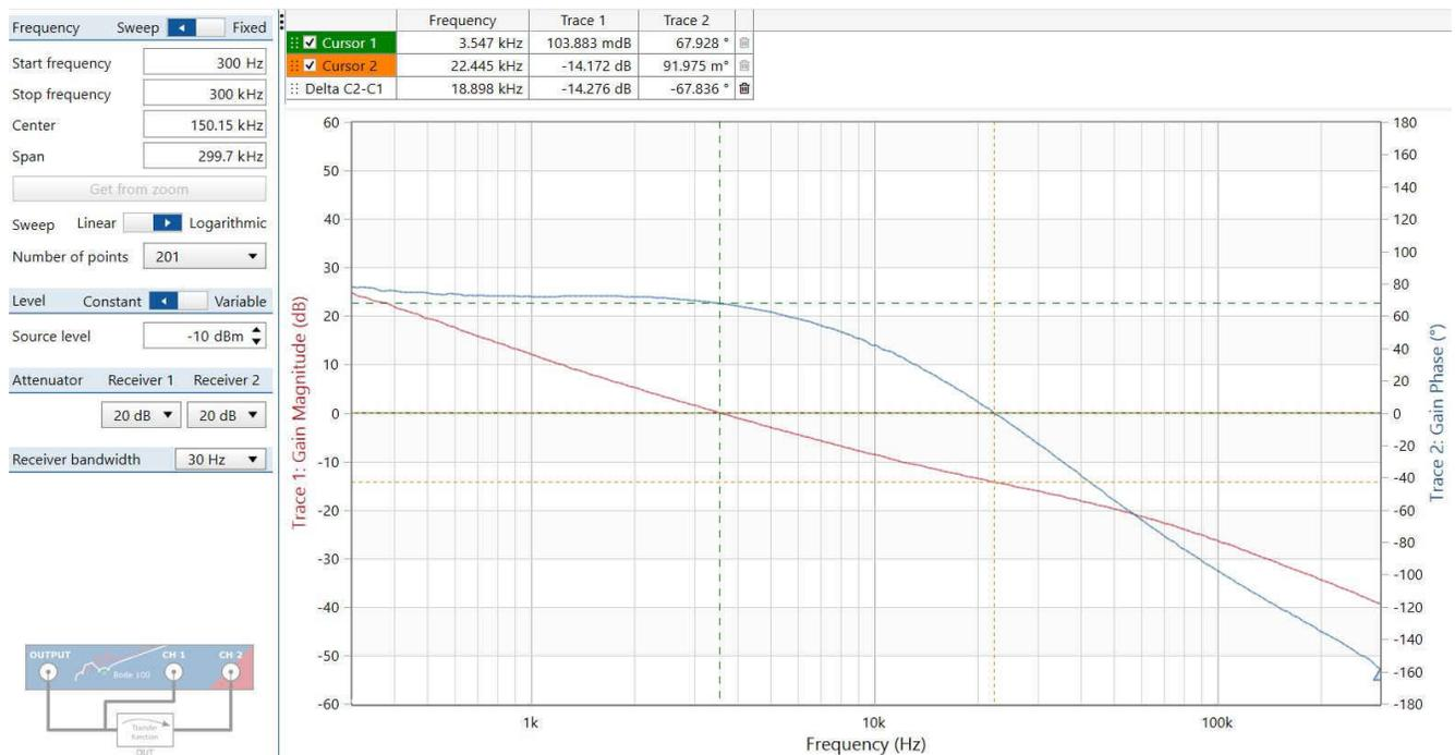
Figure 2-6. Bode Plot at 2-MHz Switching Frequency
