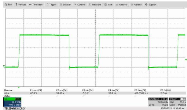
**Figure 3-4. Switching 42-V<sub>IN</sub> Q1 Drain Full Load at 445 kHz Showing Two Cycles**
