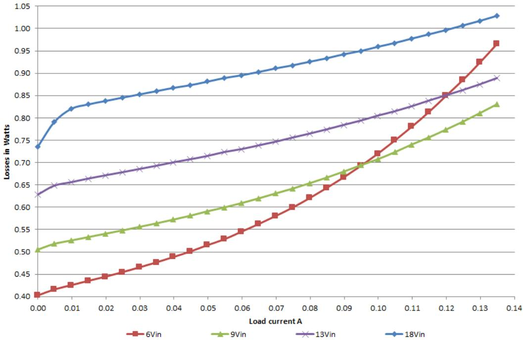
Figure 2-4. Power Loss of the PMP22817 SEPIC at 2 MHz
