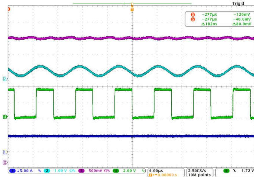
Figure 2-1. Load Current Equals 20 A (24% Load)
