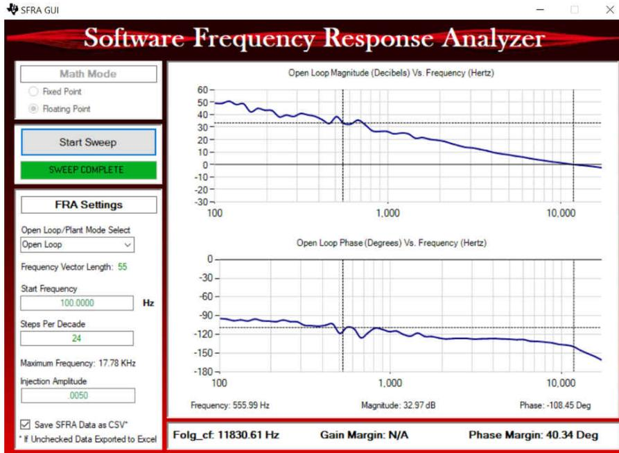
Figure 2-3. HHC Voltage Loop Bode Plot
