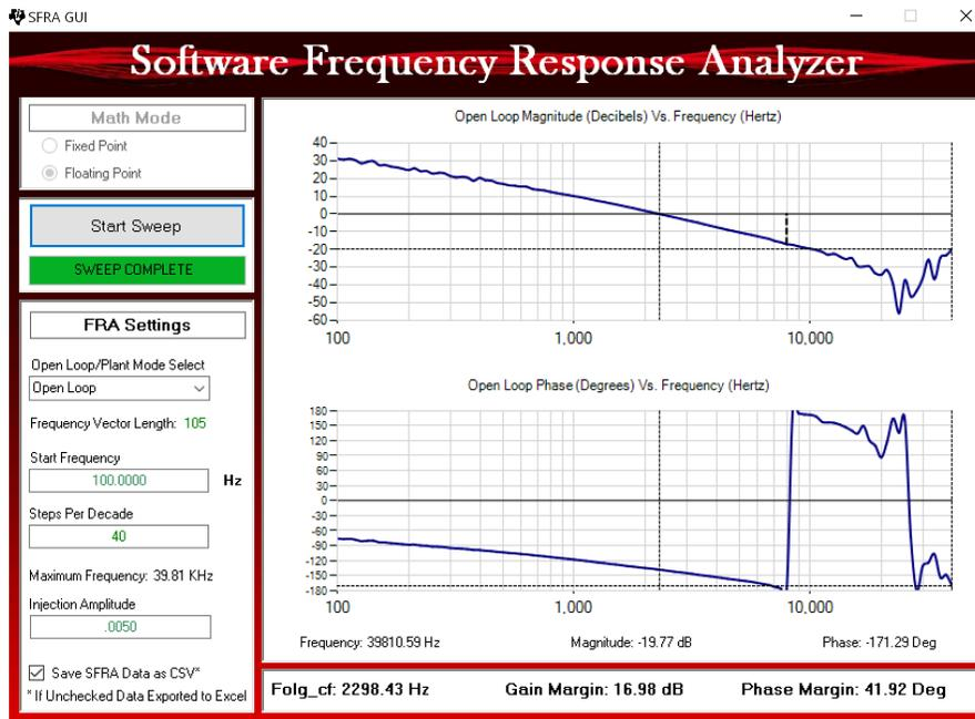
Figure 2-4. VMC Voltage Loop Bode Plot
