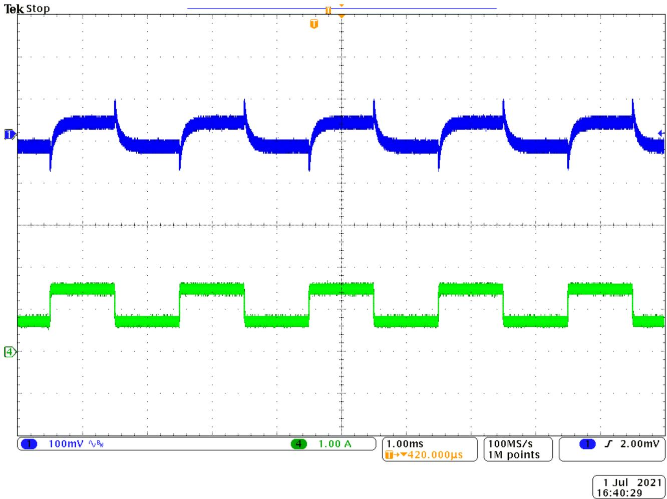
Figure 3-6. Load Transient Waveform, 12-V Input, 0.75 A to 1.5 A
