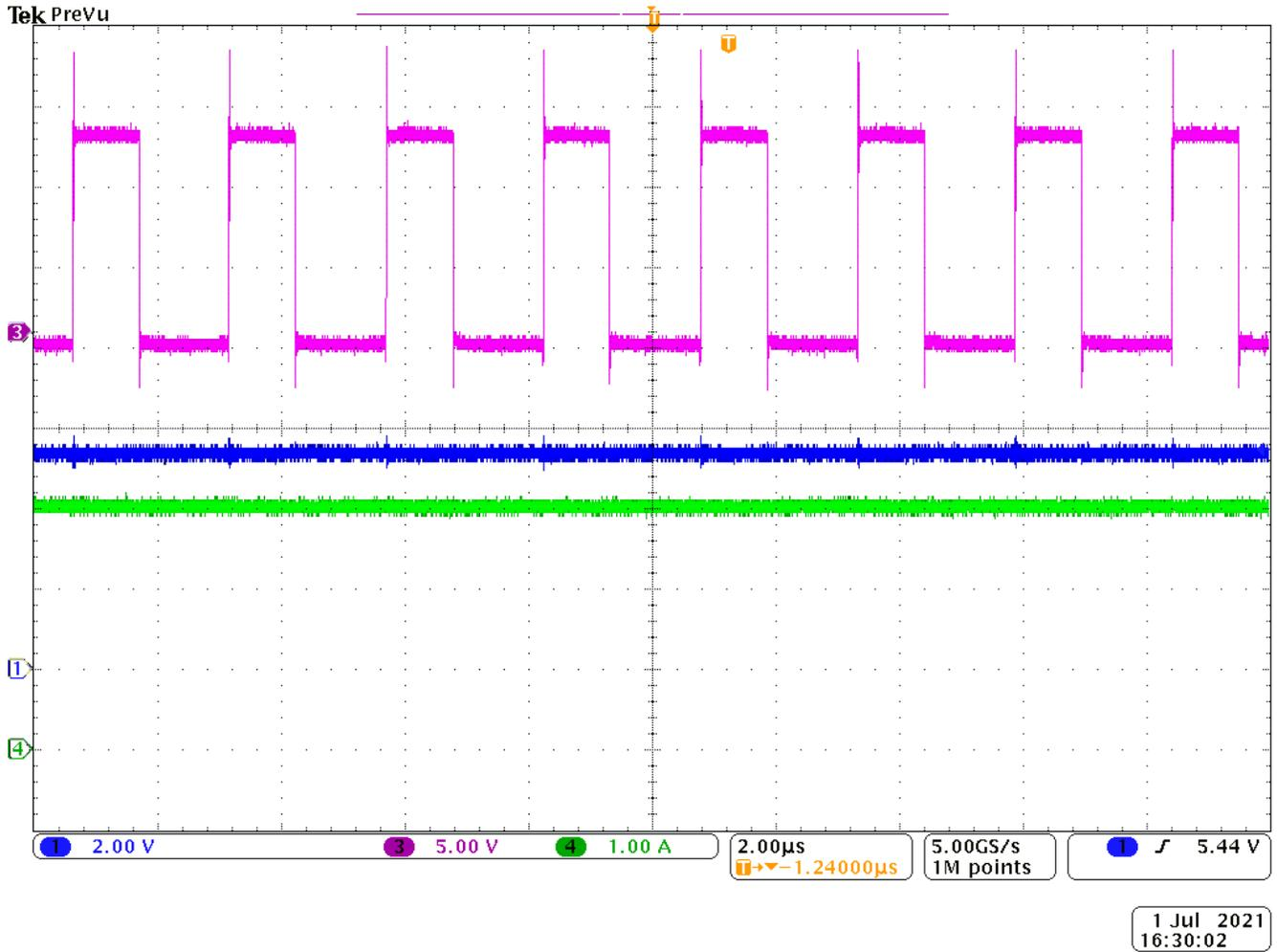
CH1:  $V_{PA\_BUS}$ , CH3:  $V_{SW}$ , CH4:  $I_{PA\_BUS}$
