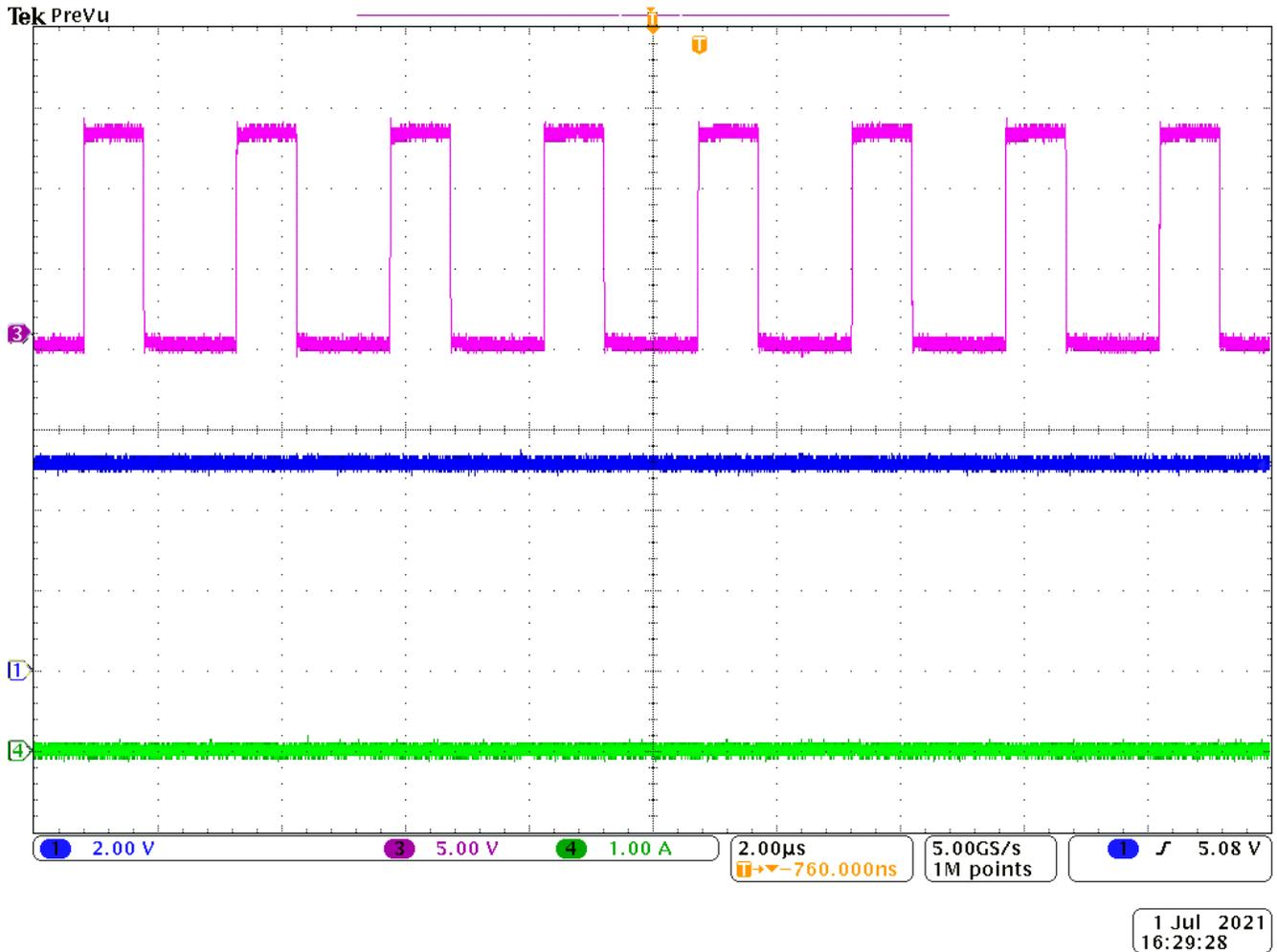
**Figure 3-1. Switching Waveform, 12-V Input, No Load**
