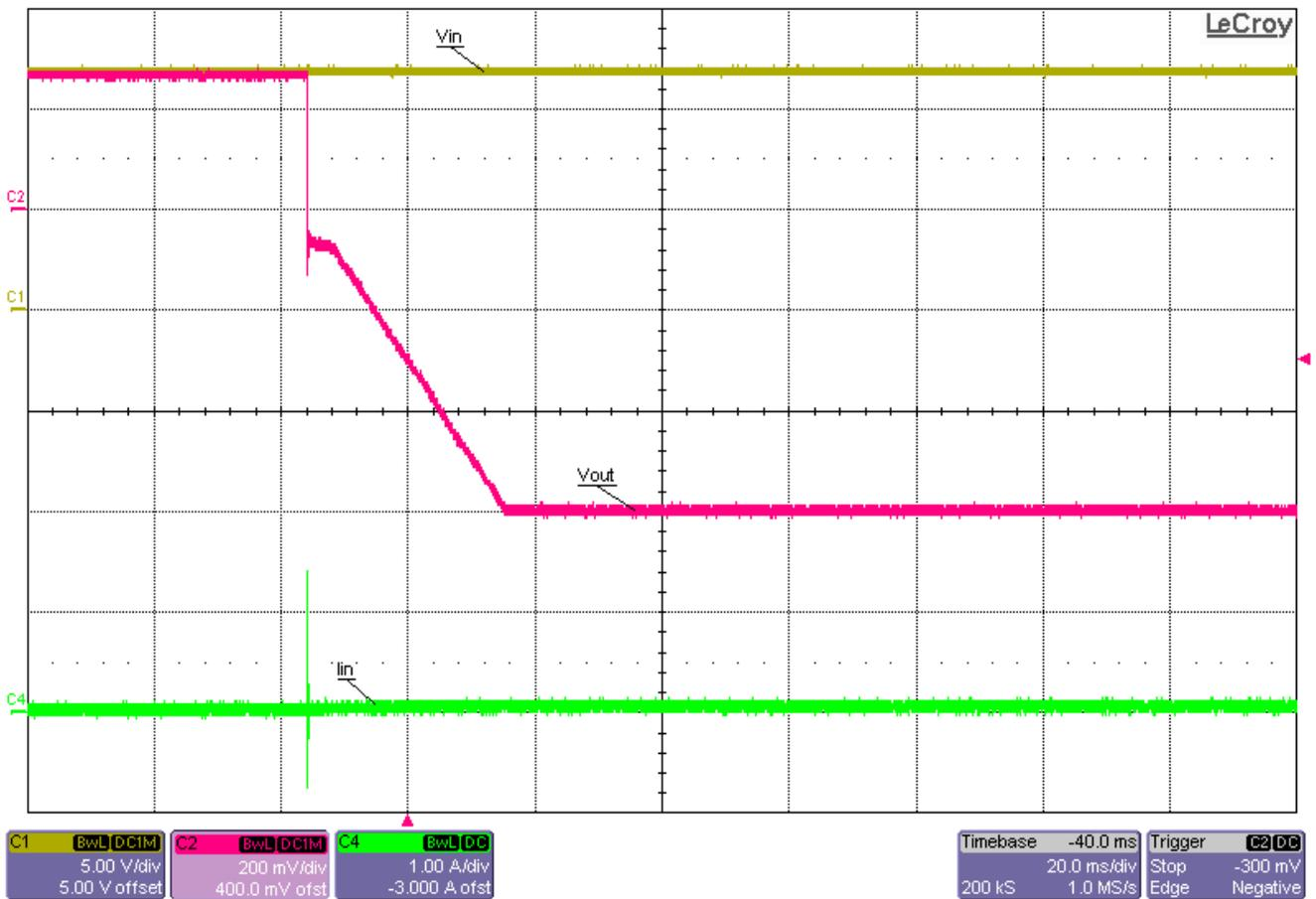
**Figure 3-15. Start-up Into No Load, 12-V Input, -0.6-V Output, Start-up Initiated via the Enable Connection (Input Supply Already Turned ON)**
