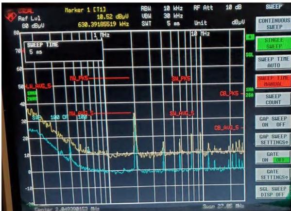
Figure 3-21. Conducted EMI Performance, 30-V Input, Low-Frequency Range
