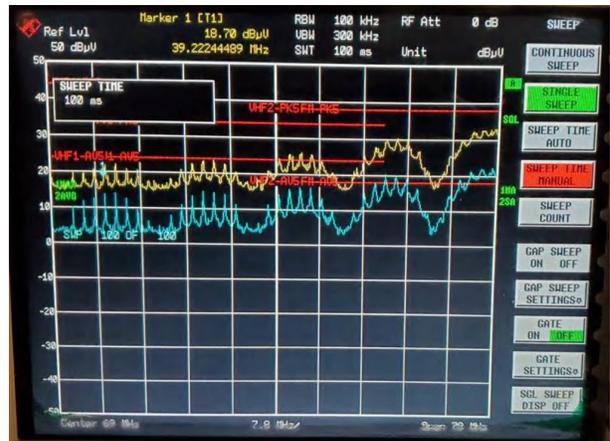
Figure 3-22. Conducted EMI Performance, 30-V Input, High-Frequency Range
