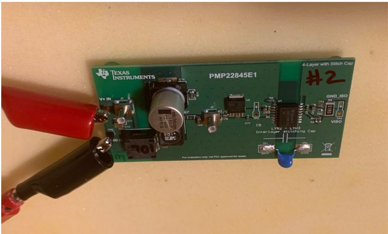
**Figure 2-3. Top Side, Through Hole Y Cap Added**
