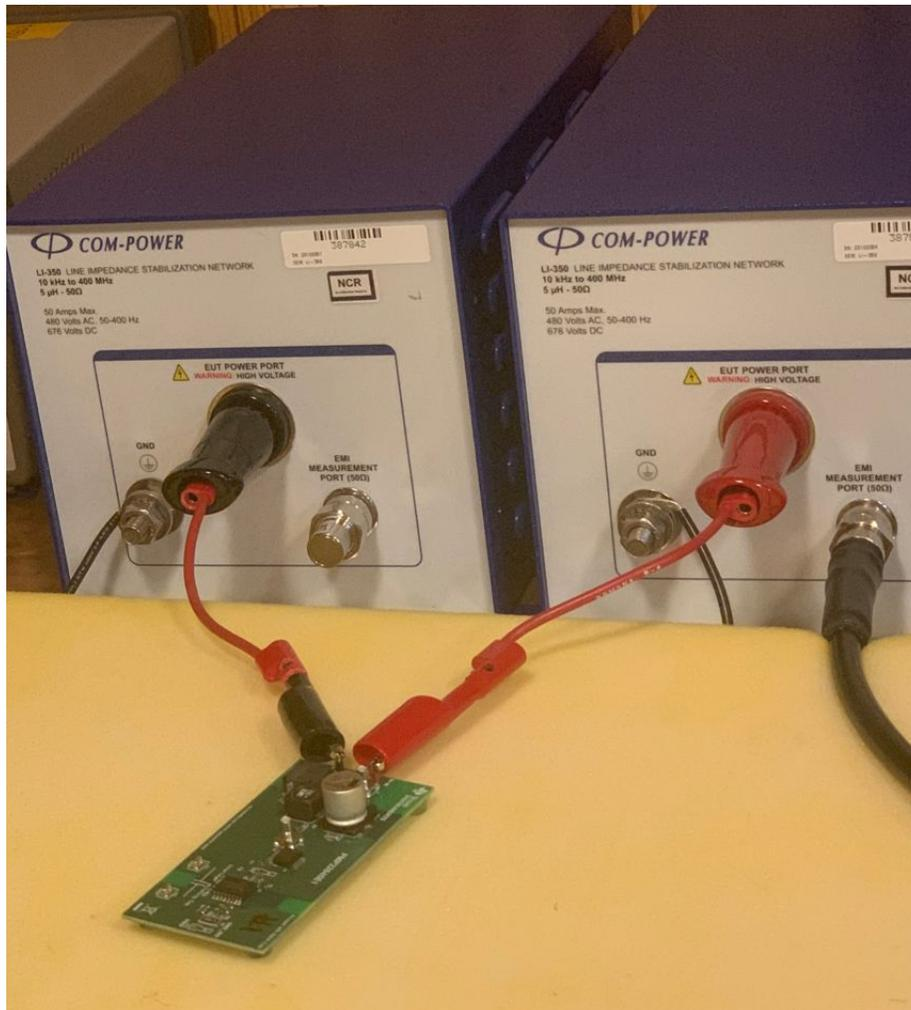
**Figure 2-1. Conducted Test Setup**
