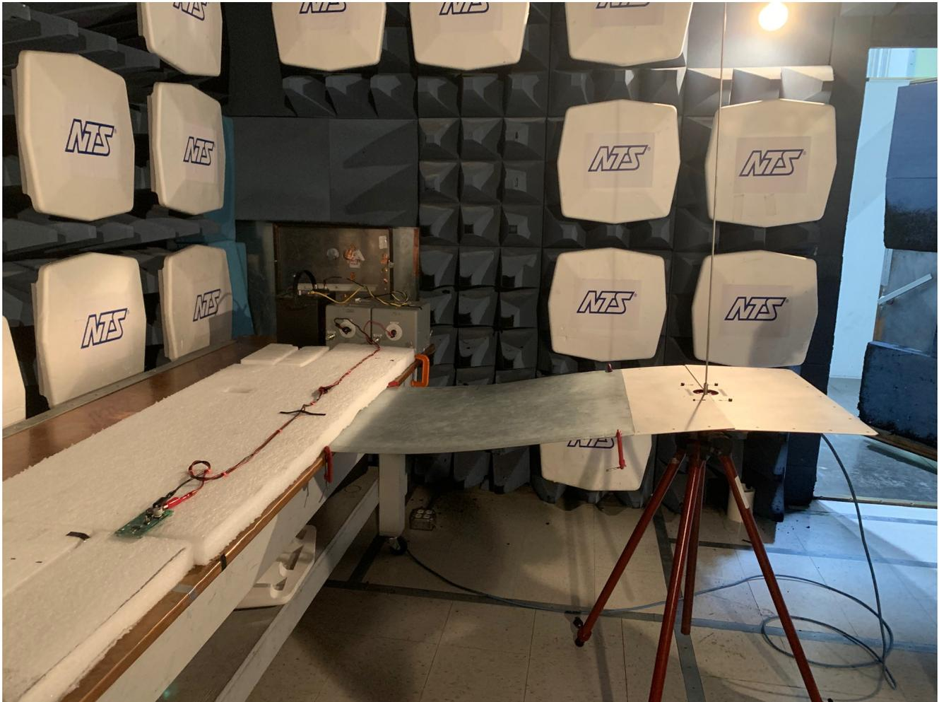
**Figure 2-4. 150 kHz–30 MHz Setup, Vertical Monopole Antenna**
