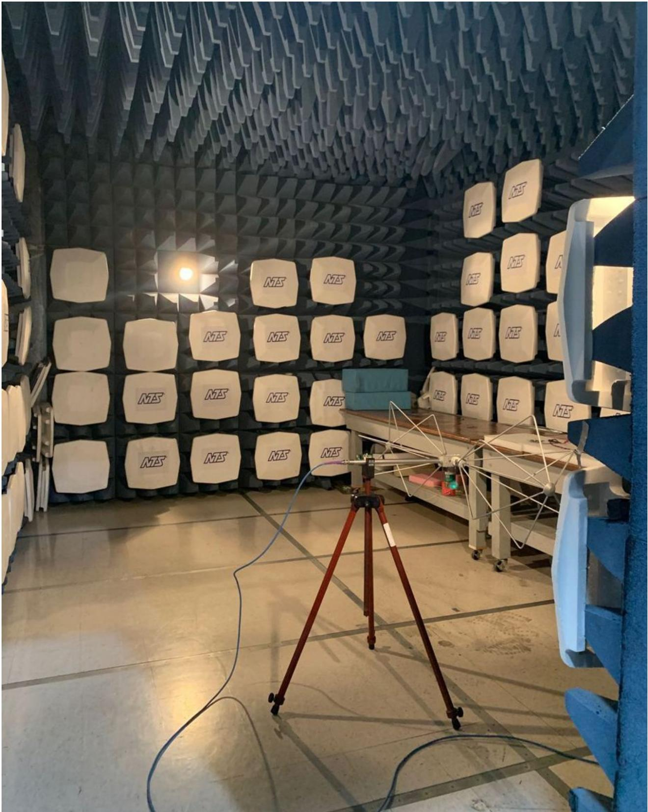
**Figure 2-6. 30 MHz –300 MHz Setup, With Biconical Antenna Horizontal**
