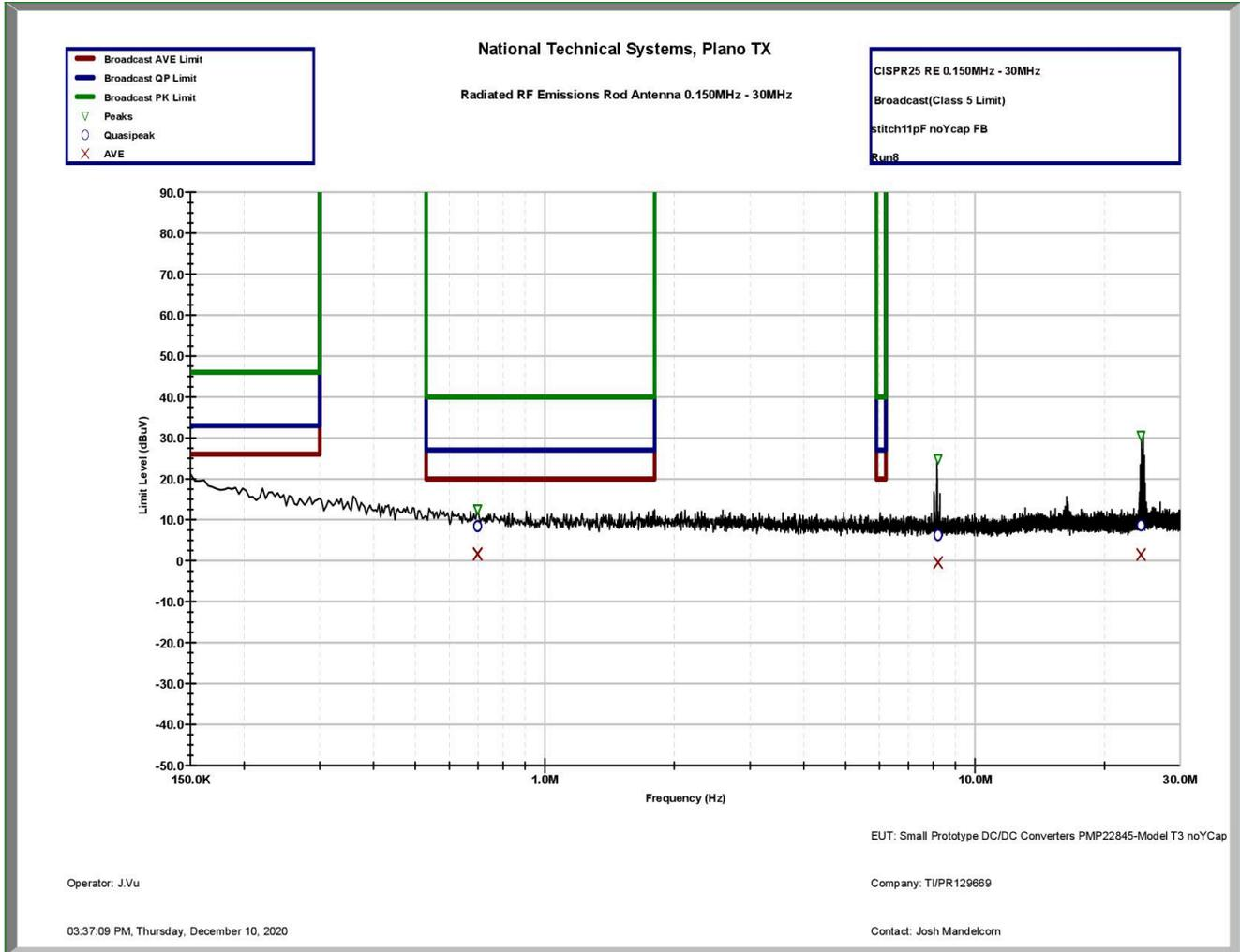
**Figure 3-6. 150 kHz–30 MHz Range With Vertical Monopole**
