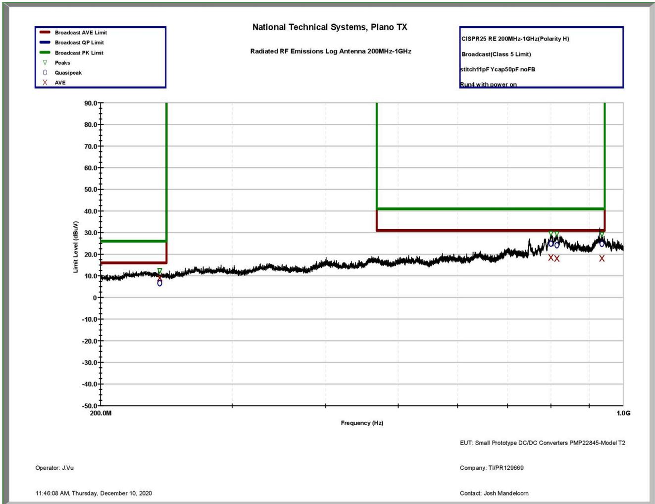
**Figure 3-11. 200 MHz – 1000 MHz Range With Horizontal Log Periodic Antenna**
