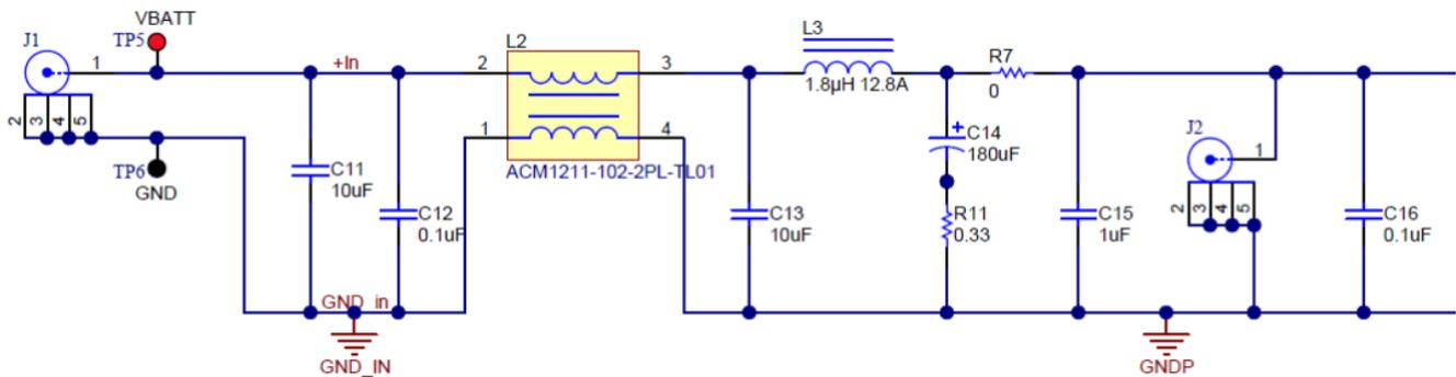
Figure 1-3. EMI Filter Schematic
