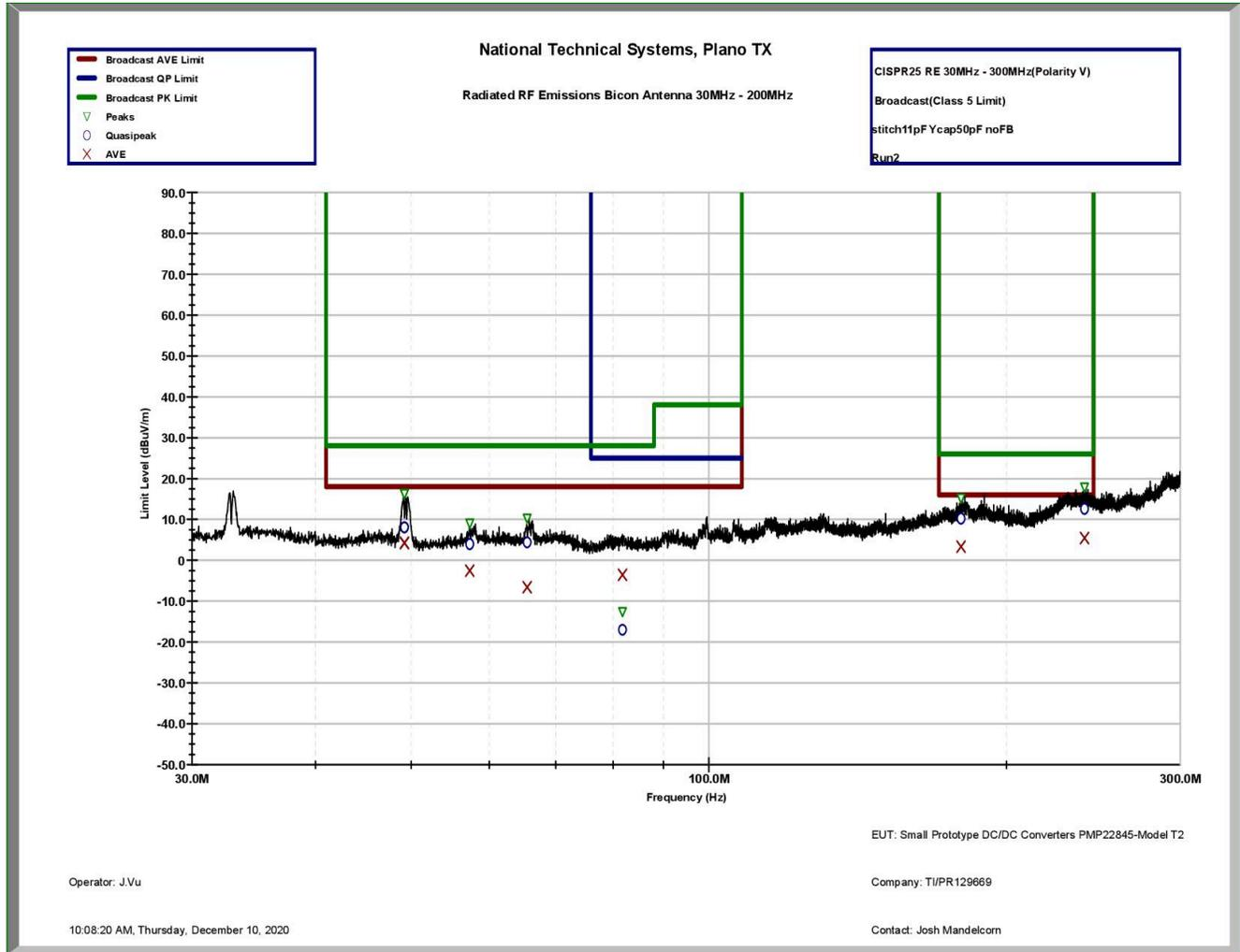
**Figure 3-9. 30 MHz – 300 MHz Range With Vertical Biconical**
