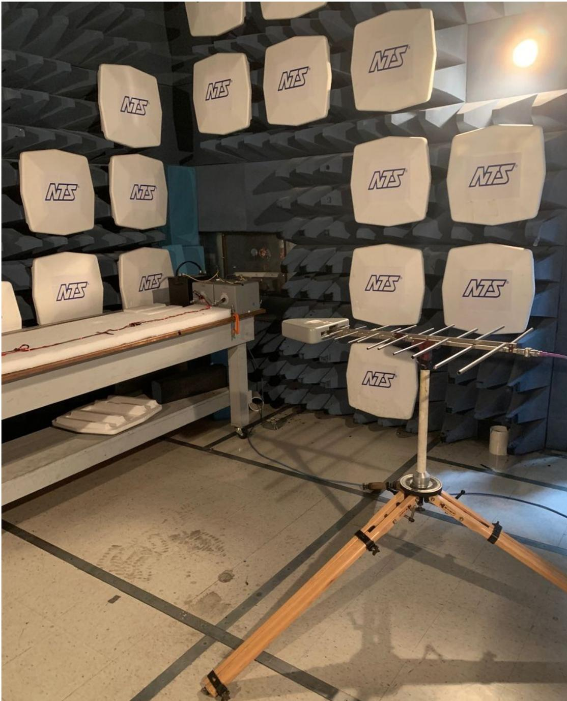
**Figure 2-5. 200 MHz –1000 MHz Setup, Horizontal Log Periodic Antenna**
