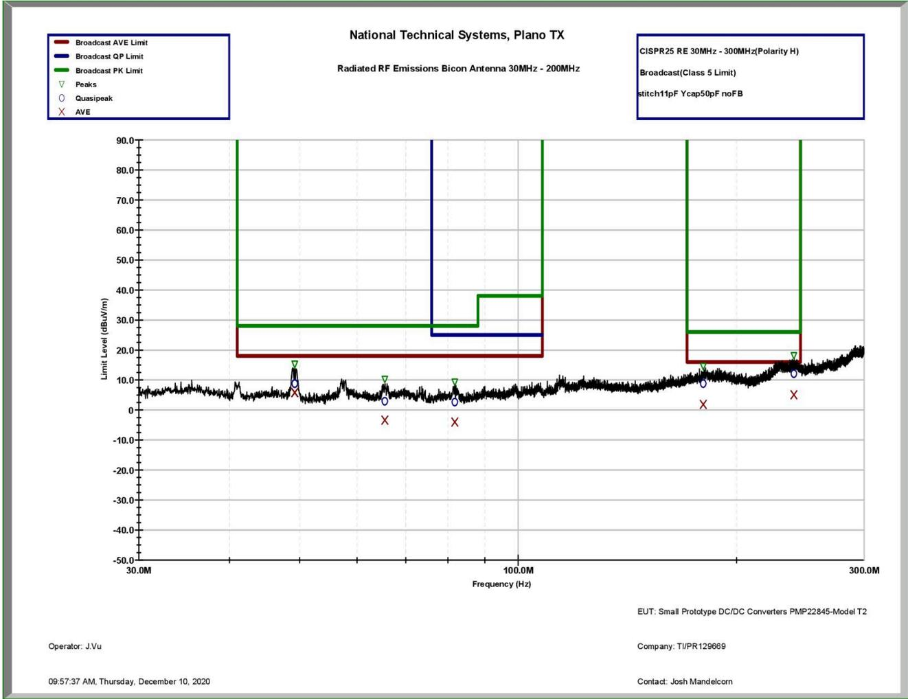
**Figure 3-7. 30 MHz – 300 MHz Range With Horizontal Biconical**
