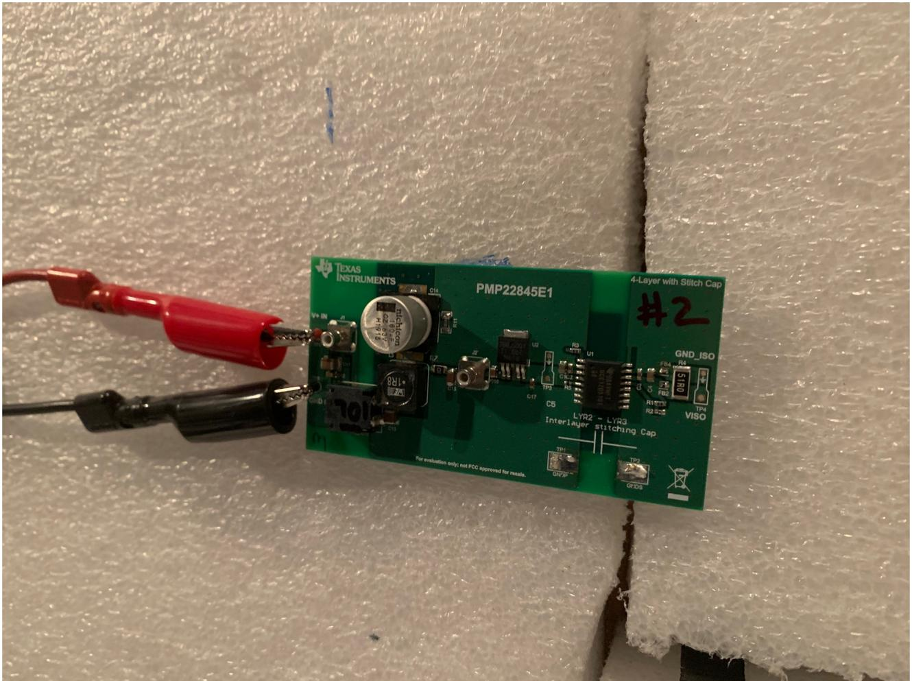
**Figure 2-7. Unit Under Test: Top Side, Version With Stitch Cap**
