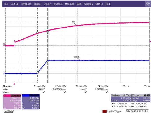
Figure 4-19. Start-up ( $V_{OUT} = 1.35\text{ V}$ )
