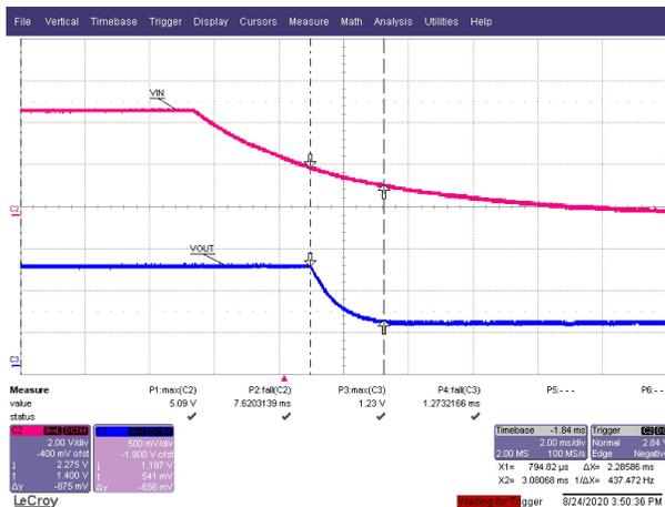
Figure 4-25. Termination ( $V_{OUT} = 1.175\text{ V}$ )
