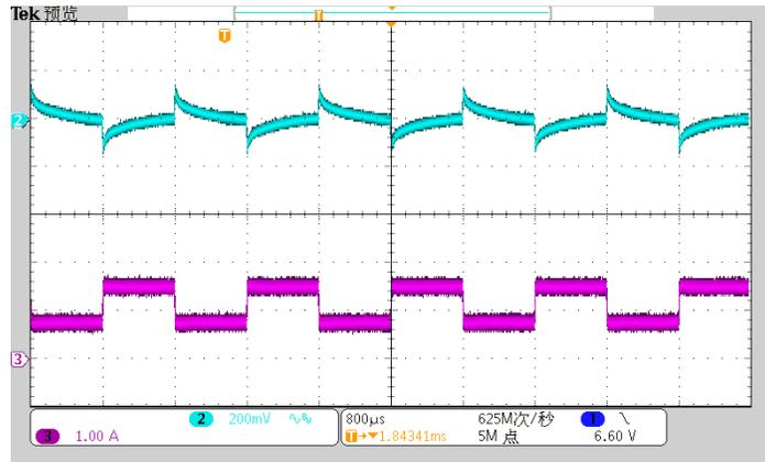
Figure 3-7. 13.5-V Input, 0.75-A to 1.5-A Output; CH2:  $V_{BUS\_AC}$ , CH3:  $I_{BUS}$
