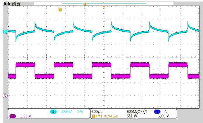
Figure 3-8. 13.5-V Input, 1.5-A to 2.4-A Output; CH2:  $V_{BUS\_AC}$ , CH3:  $I_{BUS}$
