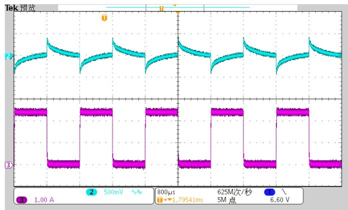
Figure 3-9. 13.5-V Input, 0-A to 2.4-A Output; CH2:  $V_{BUS\_AC}$ , CH3:  $I_{BUS}$
