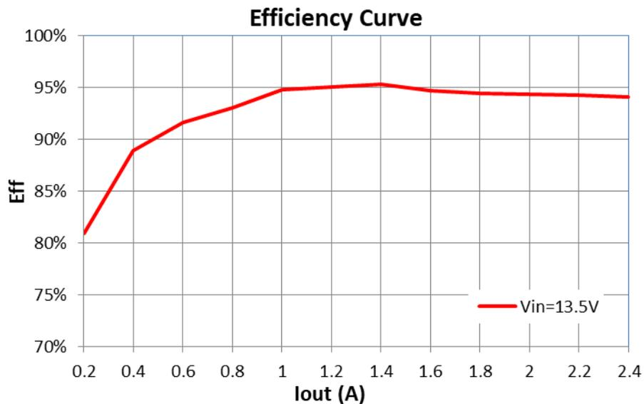
Figure 2-1. Efficiency Graph
