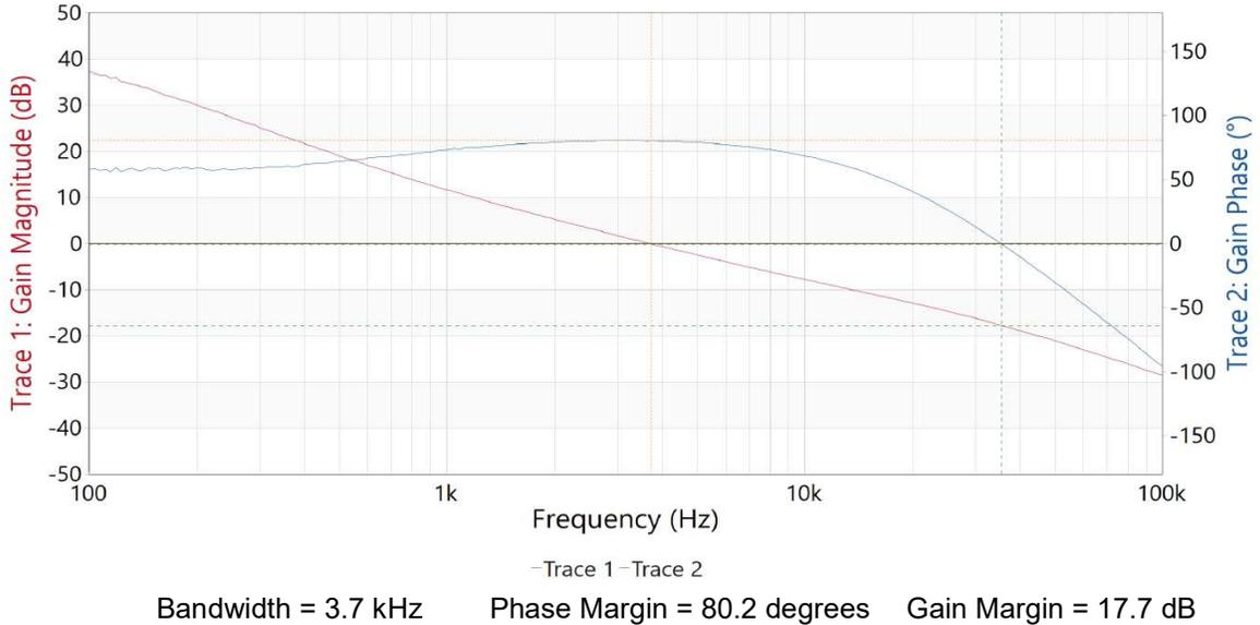
Note: Bode plots were taken in voltage regulation with a constant current load of 0.5A. This ensures the current regulation loop is not active.
