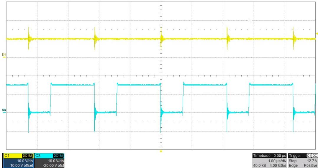
The converter is in fixed boost mode operation.
