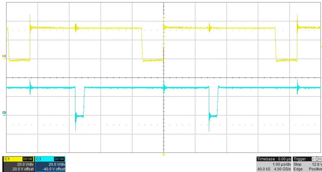
The converter is in buck-boost mode of operation.
