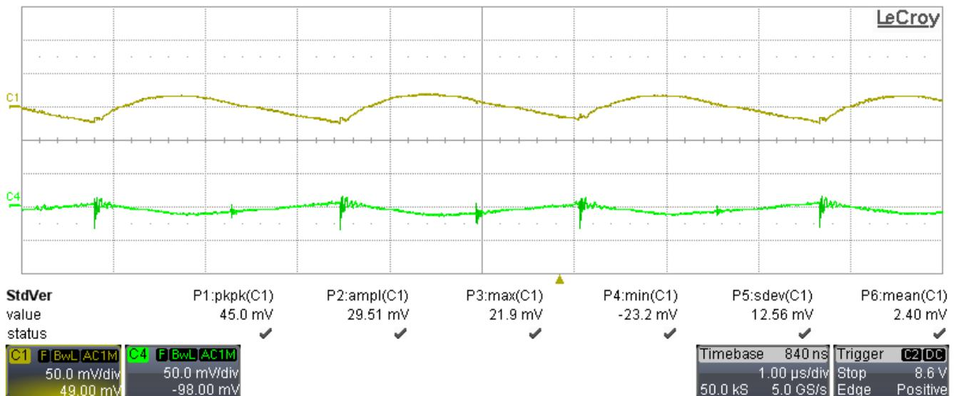
**C1: 15V Output Voltage (50 mV/div, 1 usec/div, AC coupling, 20 MHz BWL)**
