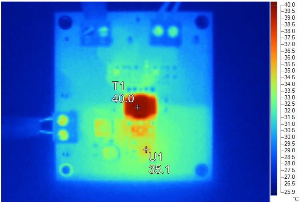
Thermal image of the PCB's top side at 12.0V in and 0.1A load current on both outputs.
