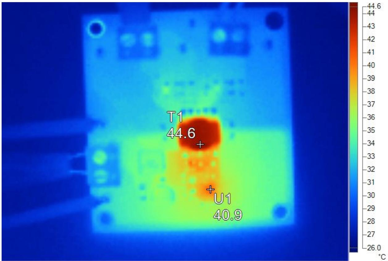
Thermal image of the PCB's top side at 8.0V in and 0.1A load current on both outputs.
