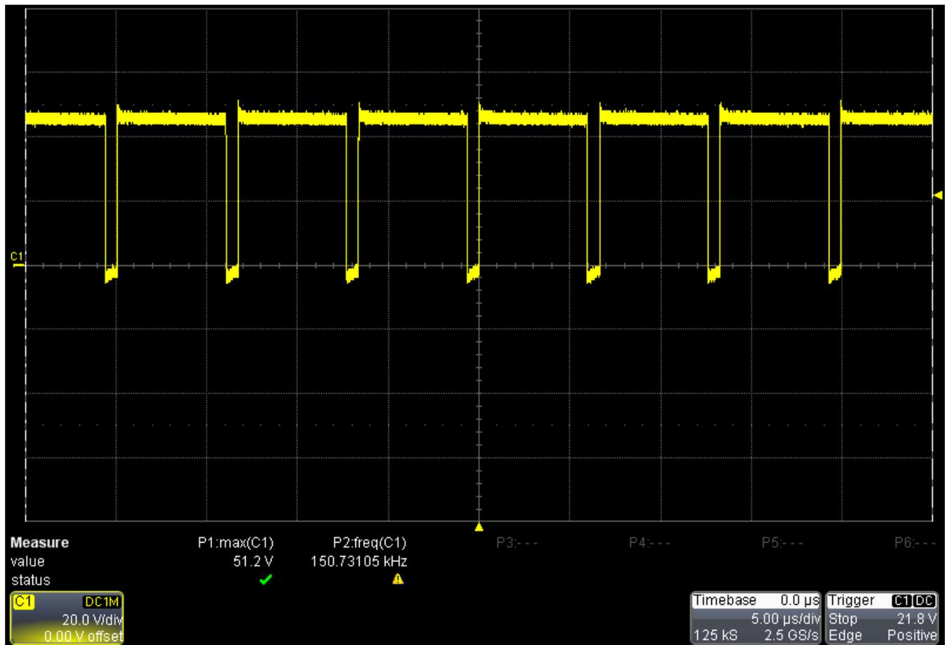
Figure 4. Primary Switching Node
