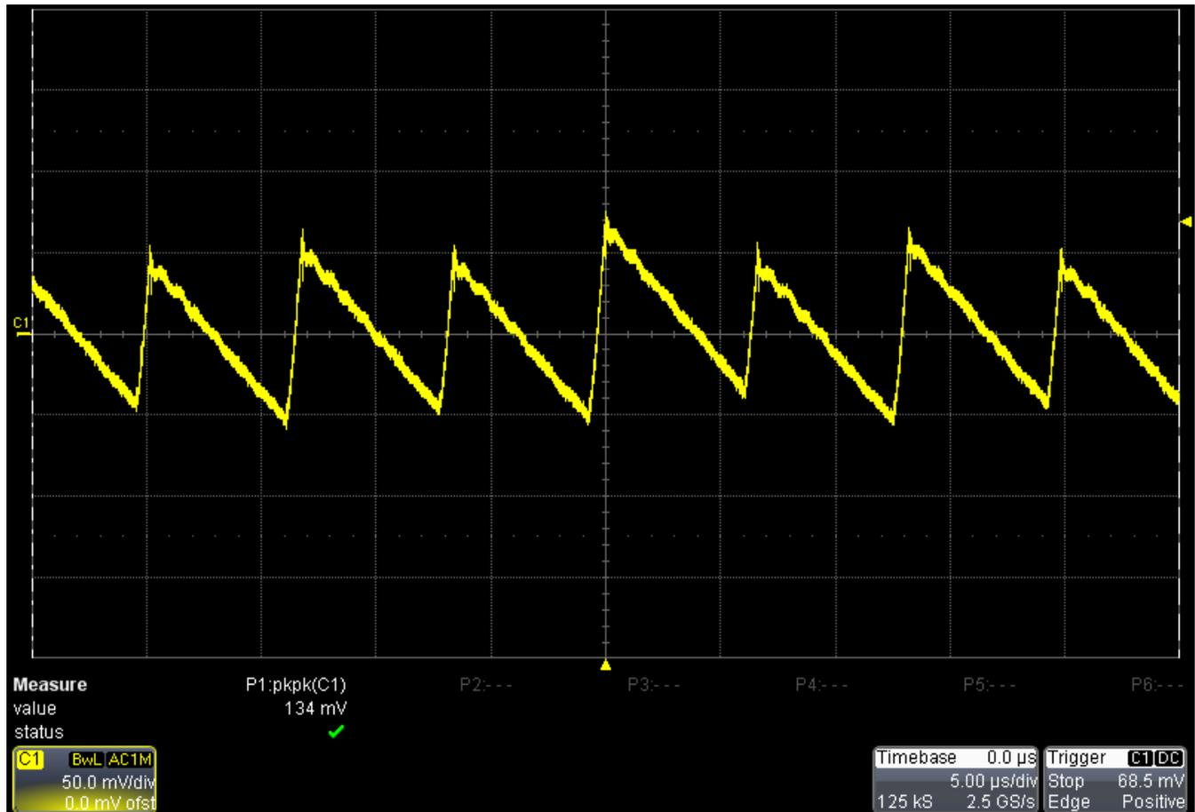
Figure 5. Output voltage ripple of the +40 V output
