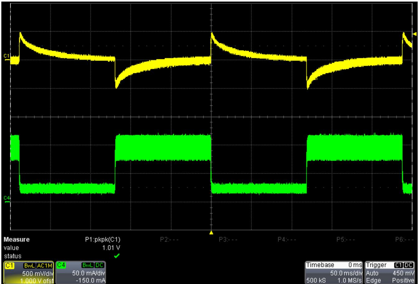
Figure 7. Load stepping Output 1 between 0.2 A and 1 A
