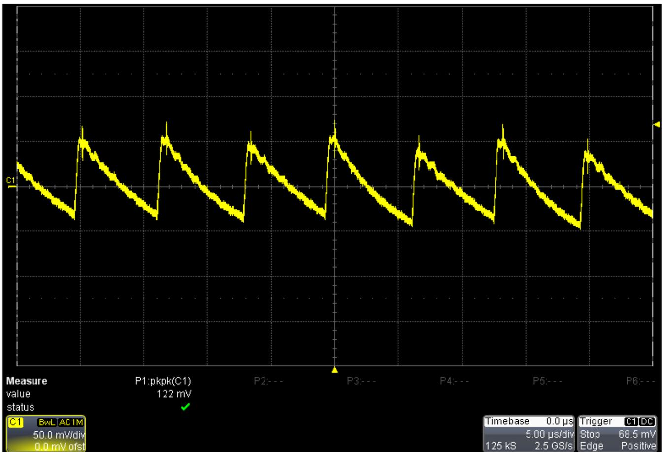
Figure 6. Output voltage ripple of the +40 V output
