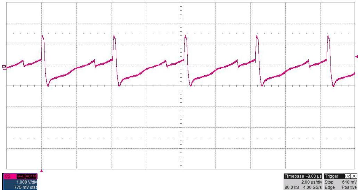
The output ripple voltage (AC coupled) is shown in the figure below. The input voltage is 12V and the -250V output is loaded to 1mA. (VOUT: 200mV/DIV, 2uS/DIV)
