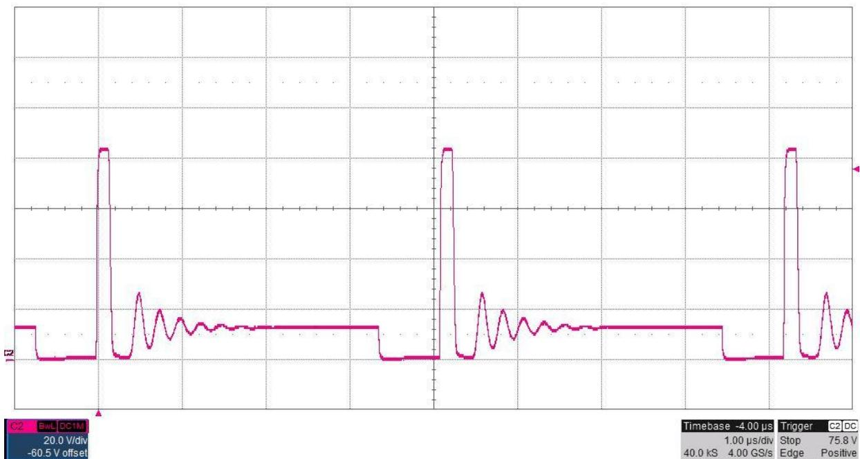
The photo below shows the FET switch node voltage at TP4. The input voltage is 40V and the -150V output is loaded to 10mA (15K ohm resistive load). (20V/DIV, 1uS/DIV)
