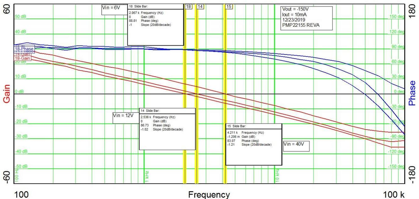
The plot below shows the converter's loop gain and phase margin when loaded to 2mA and  $V_{in} = 12V$ .
