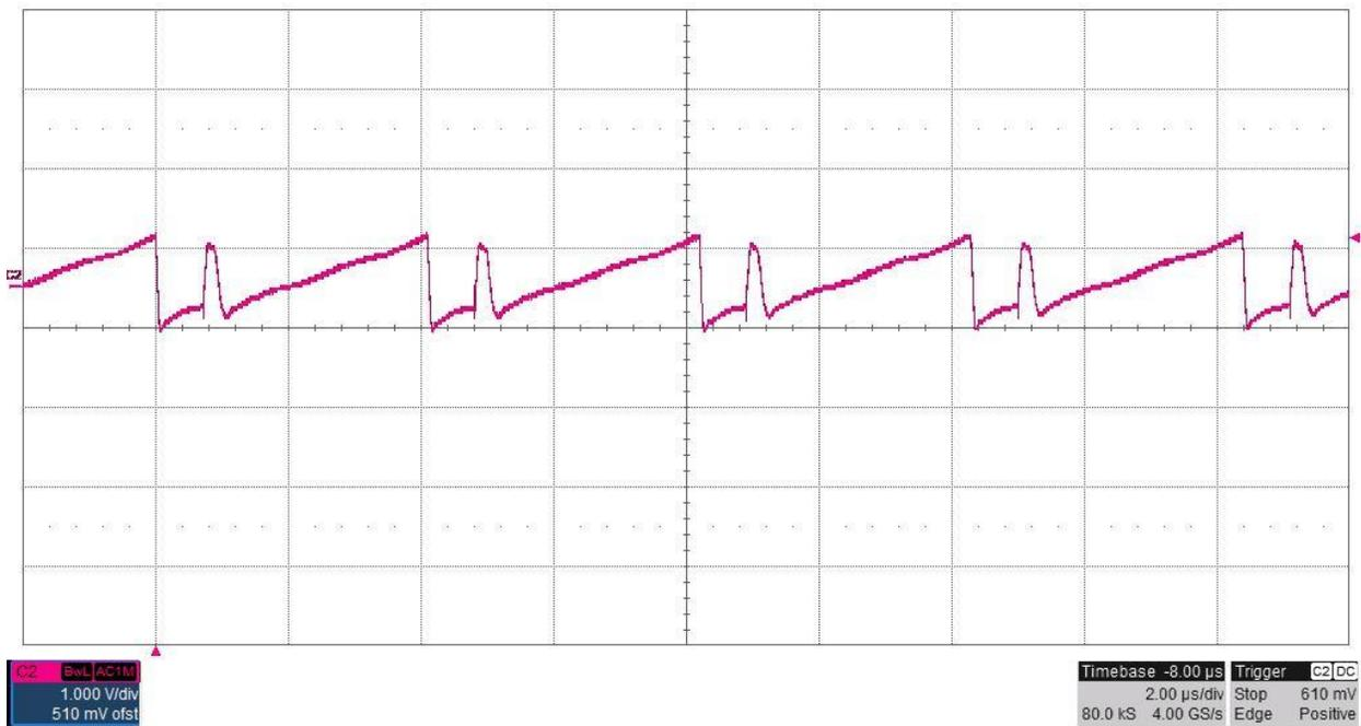
The output ripple voltage (AC coupled) is shown in the figure below. The input voltage is 12V and the -150V output is loaded to 1mA. (VOUT: 200mV/DIV, 2uS/DIV)
