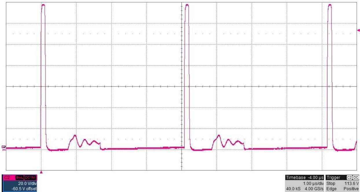
The photo below shows the FET switch node voltage at TP4. The input voltage is 12V and the -250V output is loaded to 10mA (25K ohm resistive load). (20V/DIV, 1uS/DIV)
