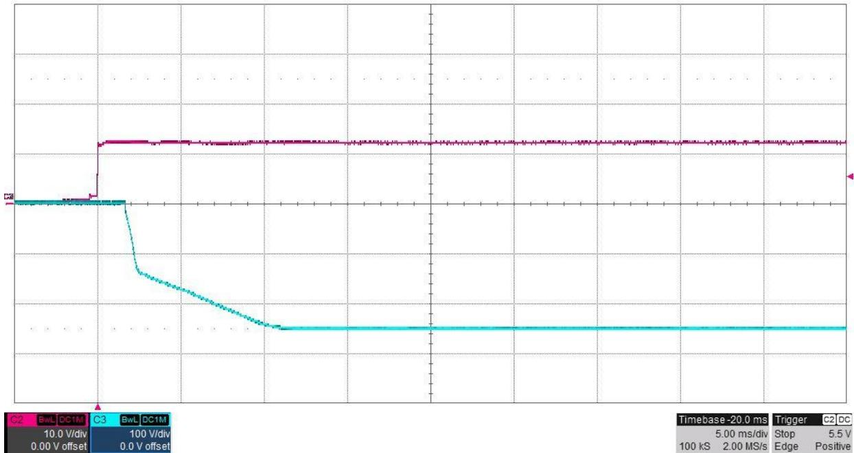
The photo below shows the output voltage startup waveform after the application of 12V input with the -250V output loaded to 10mA (25K ohm resistive load). (VOUT: 100V/DIV, 5mS/DIV), (Vin: 10V/DIV)
