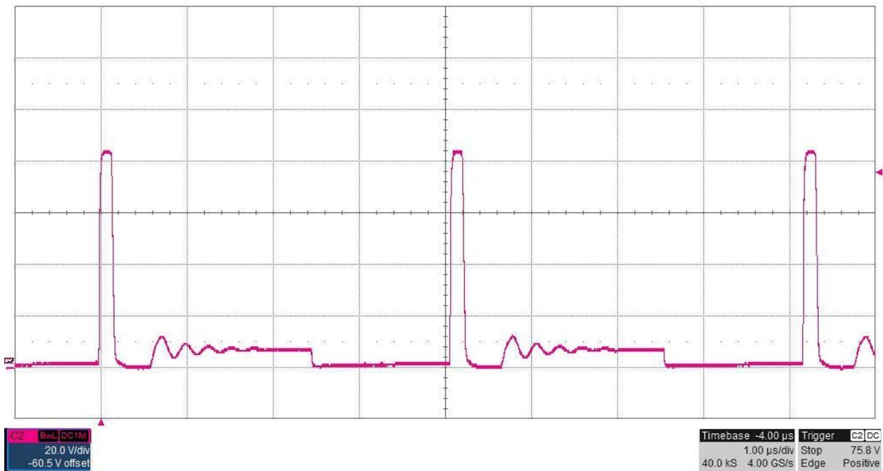
The photo below shows the FET switch node voltage at TP4. The input voltage is 12V and the -150V output is loaded to 10mA (15K ohm resistive load). (20V/DIV, 1uS/DIV)
