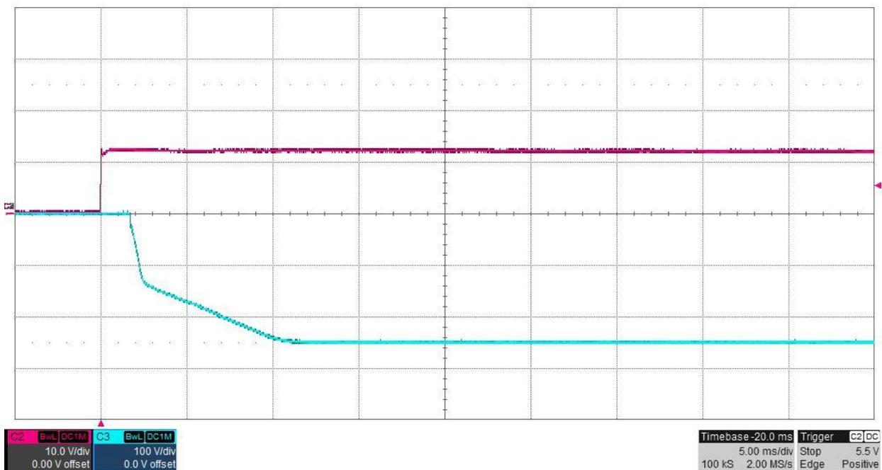
The photo below shows the output voltage startup waveform after the application of 12V input with the -150V output loaded to 0A. (VOUT: 50V/DIV, 5mS/DIV), (Vin: 10V/DIV)
