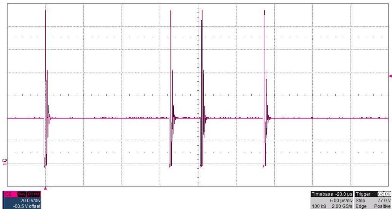
The photo below shows the FET switch node voltage at TP4. The input voltage is 6V and the -150V output is loaded to 10mA (15K ohm resistive load). (20V/DIV, 1uS/DIV)
