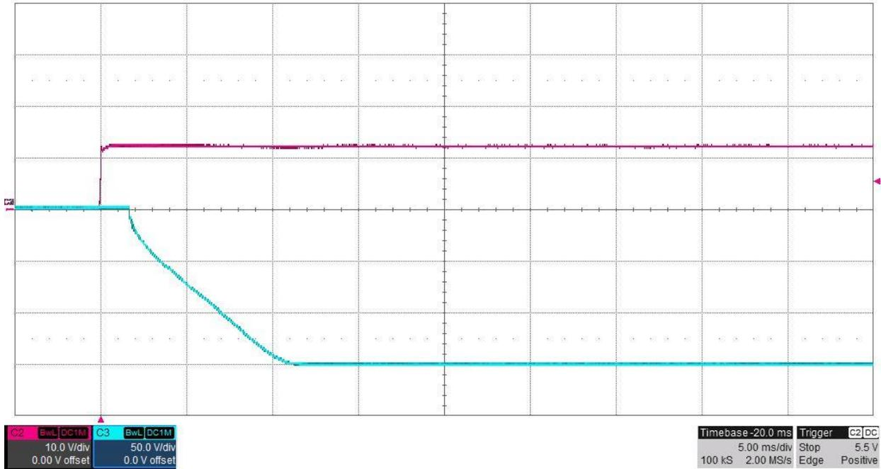
The photo below shows the output voltage startup waveform after the application of 12V input with the -150V output loaded to 10mA (15K ohm resistive load). (VOUT: 50V/DIV, 5mS/DIV), (Vin: 10V/DIV)
