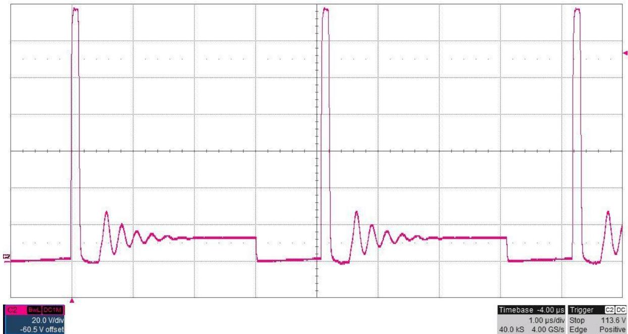
The photo below shows the FET switch node voltage at TP4. The input voltage is 40V and the -250V output is loaded to 10mA (25K ohm resistive load). (20V/DIV, 1uS/DIV)
