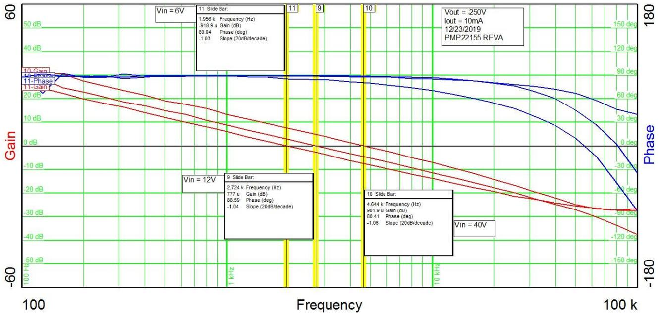
The plot below shows the converter's loop gain and phase margin when loaded to -150V @ 10mA.
