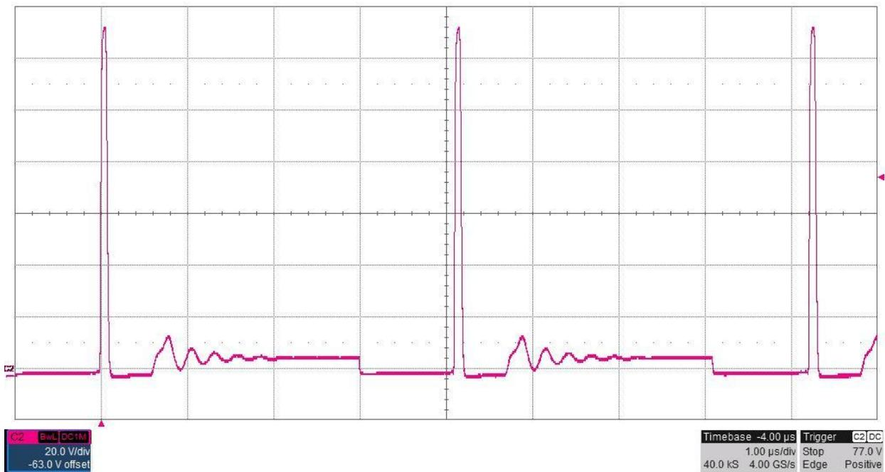
The photo below shows the FET switch node voltage at TP4. The input voltage is 12V and the -250V output is loaded to 1mA (250K ohm resistive load). (20V/DIV, 1uS/DIV)
