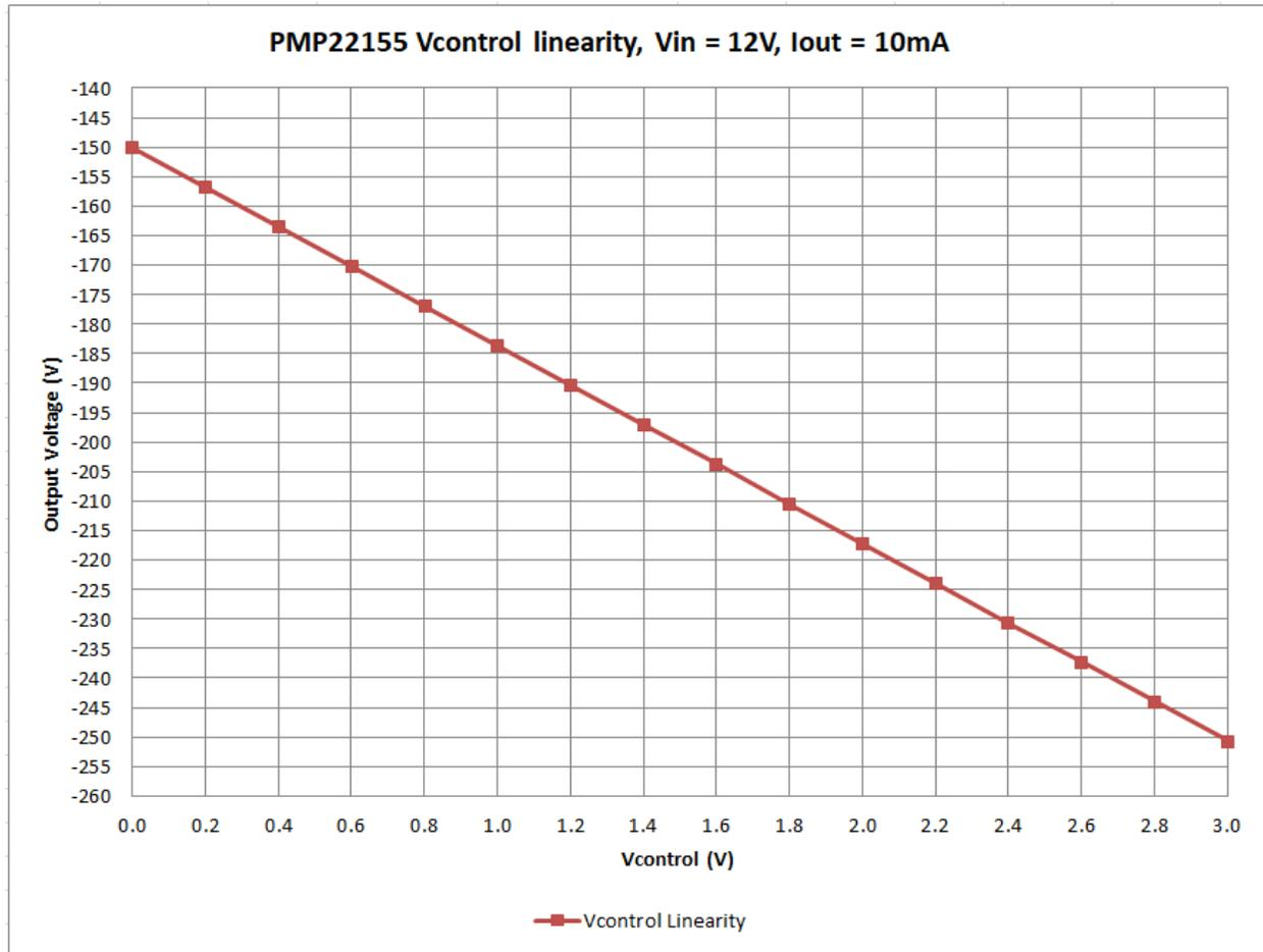
This graph displays the measured output voltage when Vcontrol is varied between 0V to 3V. The converter was set to 12V input and the output was loaded to 10mA.
