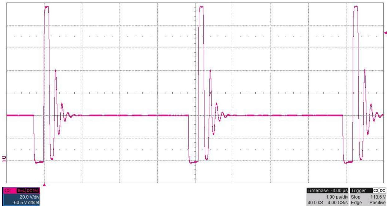
The photo below shows the FET switch node voltage at TP4. The input voltage is 6V and the -250V output is loaded to 1mA (250K ohm resistive load). (20V/DIV, 1uS/DIV)
