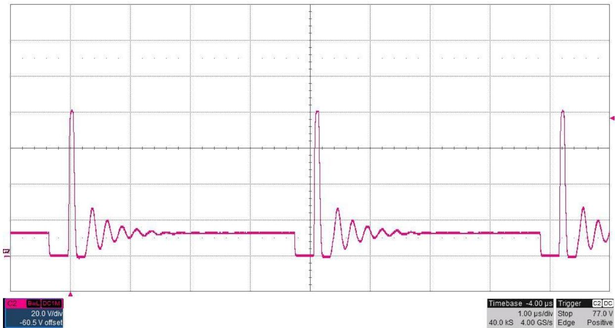
The photo below shows the FET switch node voltage at TP4. The input voltage is 40V and the -150V output is loaded to 1mA (150K ohm resistive load). Pulse skipping (20V/DIV, 5uS/DIV)
