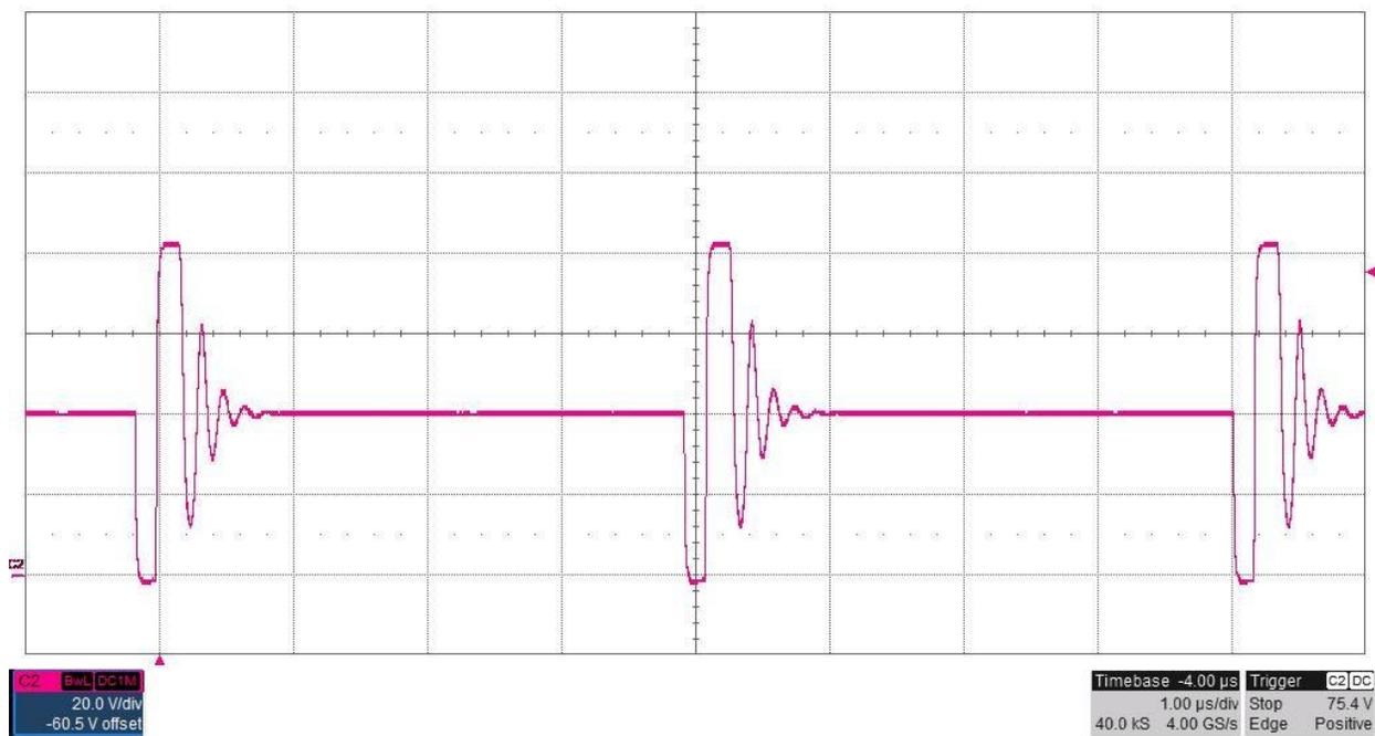
The photo below shows the FET switch node voltage at TP4. The input voltage is 6V and the -150V output is loaded to 1mA (150K ohm resistive load). (20V/DIV, 1uS/DIV)
