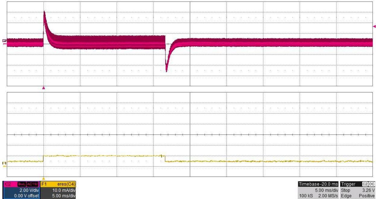
The photo below shows the -150V output voltage (AC coupled) when the load current is stepped between 5mA and 10mA.  $V_{in} = 12V$ . Current waveform digitally filtered to remove noise. (2V/DIV, 10mA/DIV, 5mS/DIV)
