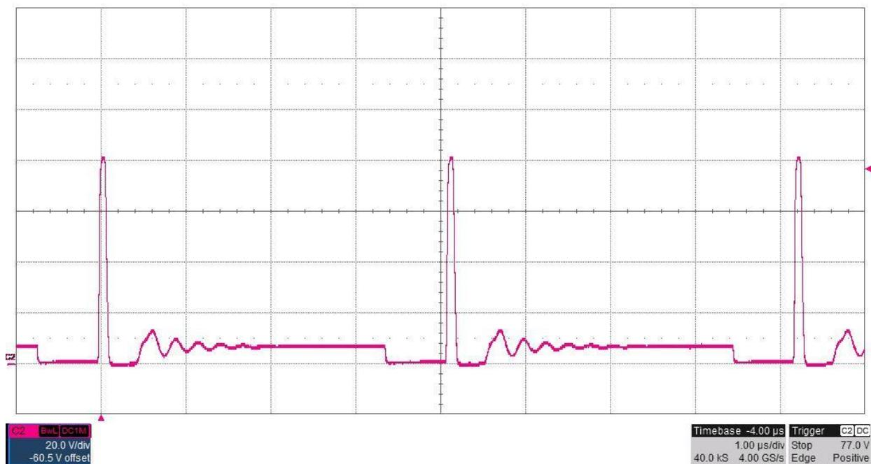
The photo below shows the FET switch node voltage at TP4. The input voltage is 12V and the -150V output is loaded to 1mA (150K ohm resistive load). (20V/DIV, 1uS/DIV)
