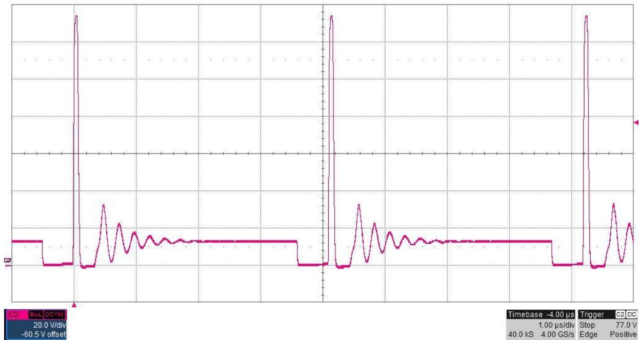
The photo below shows the FET switch node voltage at TP4. The input voltage is 40V and the -250V output is loaded to 1mA (250K ohm resistive load). Pulse skipping (20V/DIV, 5uS/DIV)
