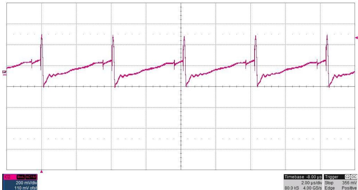
The output ripple voltage (AC coupled) is shown in the figure below. The input voltage is 12V and the -150V output is loaded to 10mA. (VOUT: 1V/DIV, 2uS/DIV)
