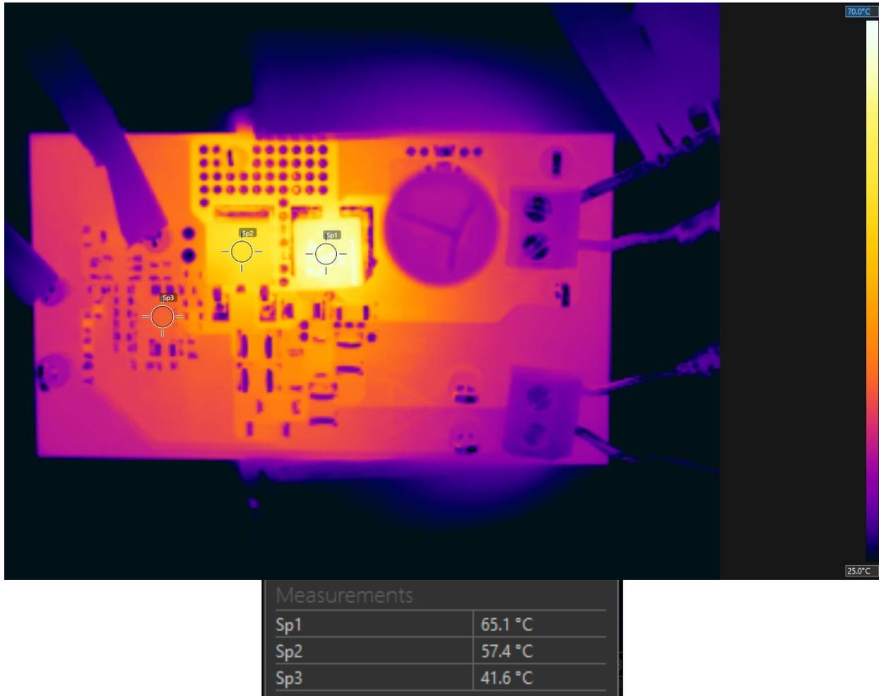
This thermal image shows the operating temperature of the board with 12V input and the output voltage set to -150V @ 10mA loads at room temperature and no air flow.
