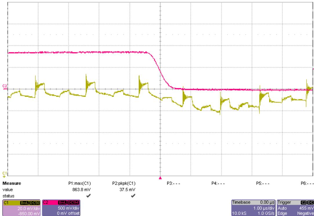
**Figure 12** Load transient used was the on-board dynamic load. Capture shows the Ramp up load transient response. Load goes between 0 A and 7.08 A.  $V_{in} = 28\text{ V}$  and  $V_{out} = 0.85\text{ V}$ .
