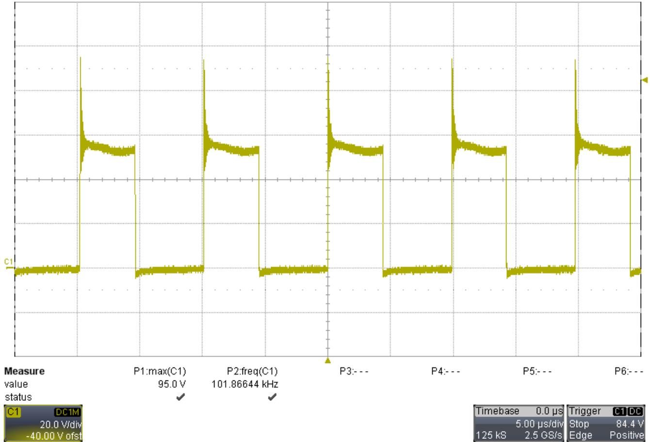
Figure 6. Primary Switching Node
