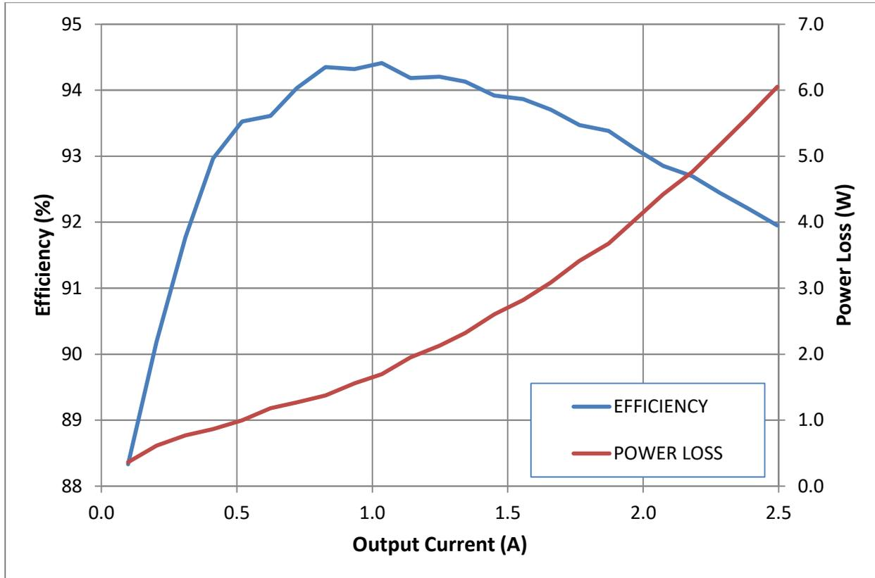
Figure 3. Efficiency with 24 Vdc Input
