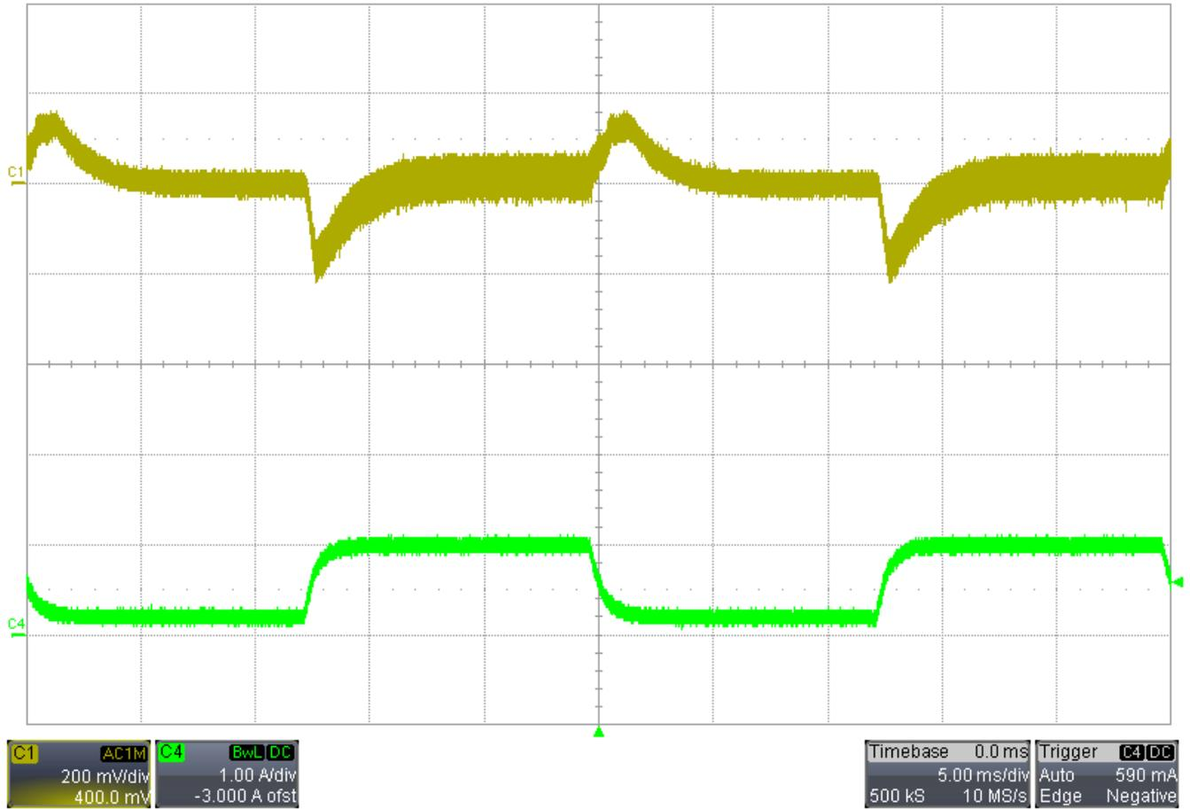
Figure 10. Load stepping between 0.2 A and 1 A
