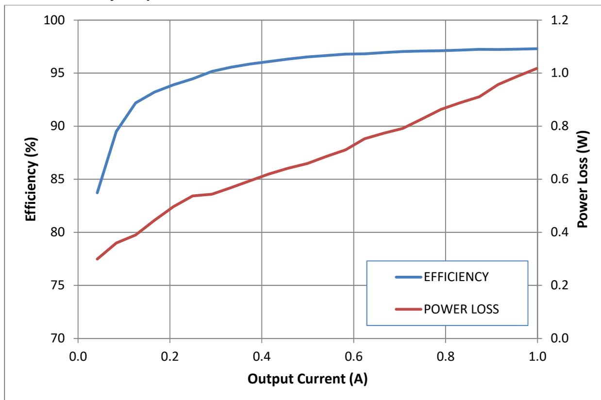
Figure 12. Efficiency with 28 Vdc Input
