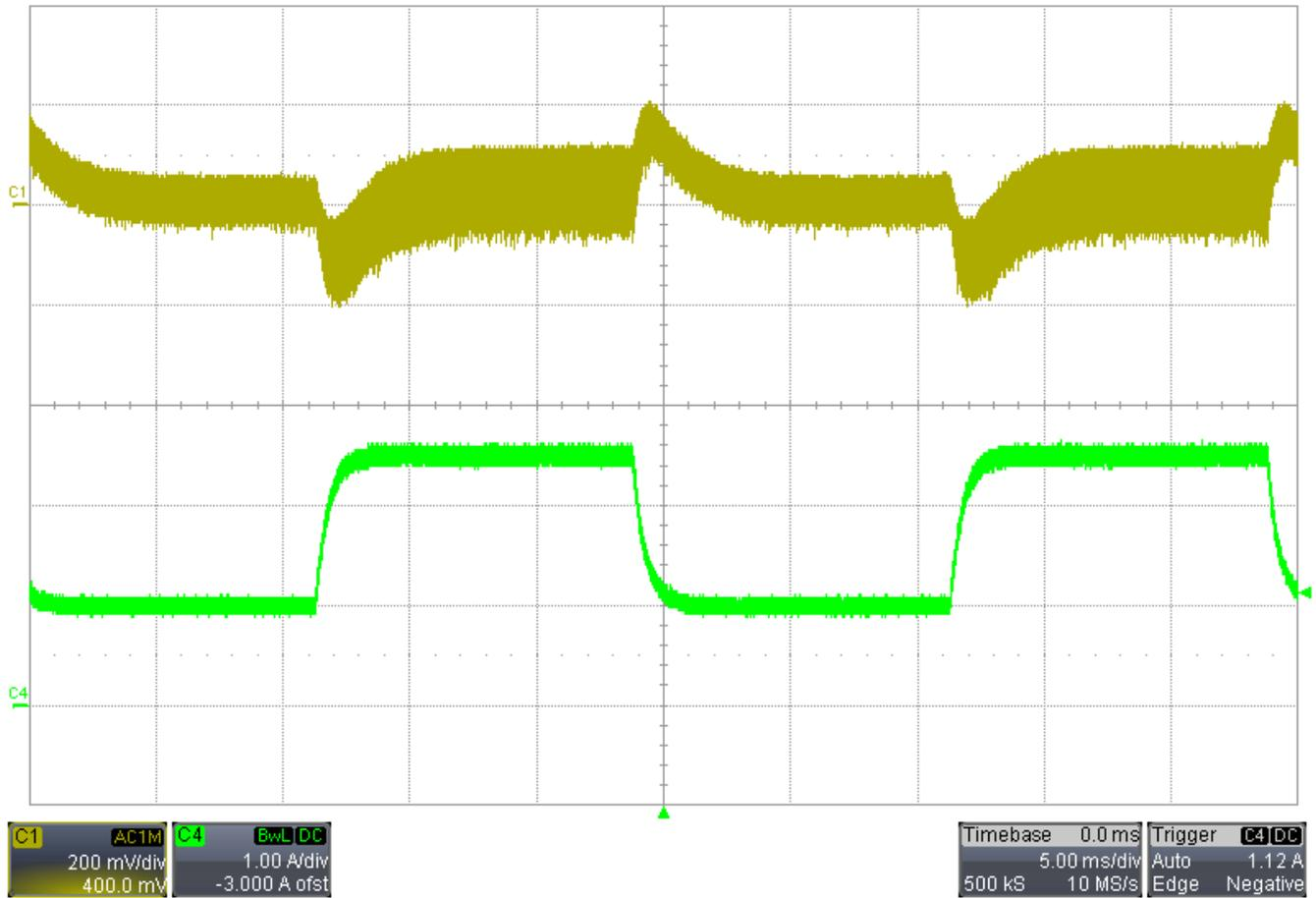
Figure 9. Load stepping between 1 A and 2.5 A
