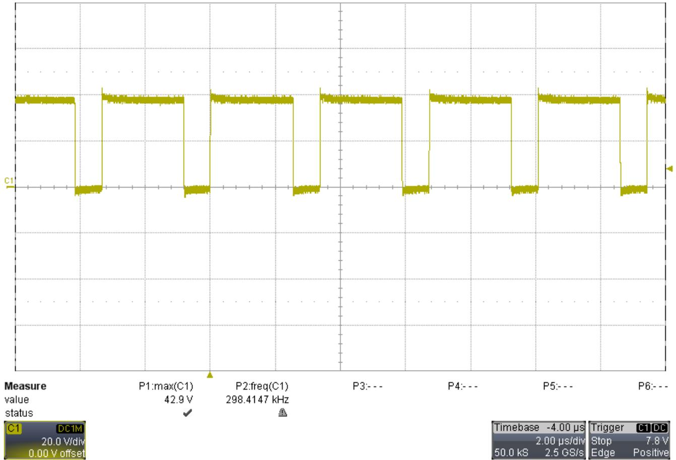
Figure 15. Primary Switching Node
