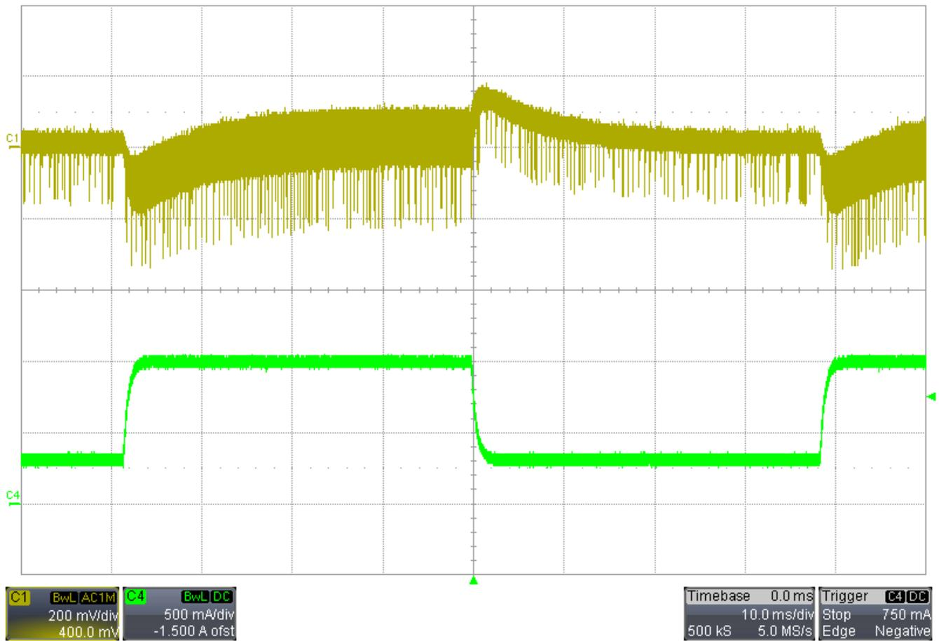
Figure 17. Load stepping between 0.3 A and 1 A
