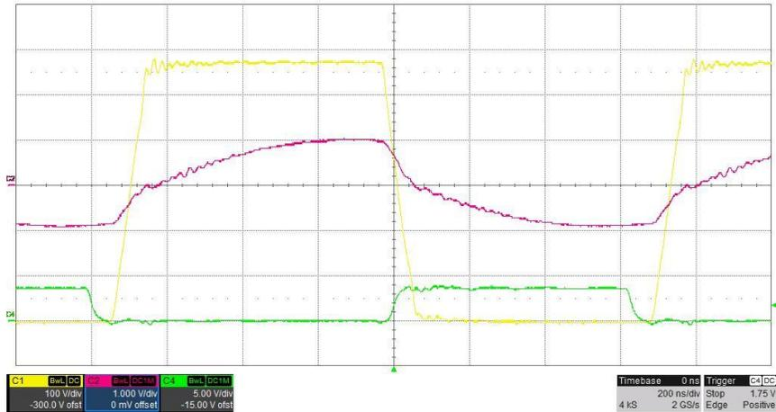
**2.4.3  $F_{sw}=300\text{kHz}$ , 3.3kW: C1: XFMR Primary Winding Current (100mV/A), CH2: XFMR Secondary Winding Current (200mV/A), CH3: SR Driving Signal (PWM3A), CH4: SR Driving Signal (PWM3B)**
