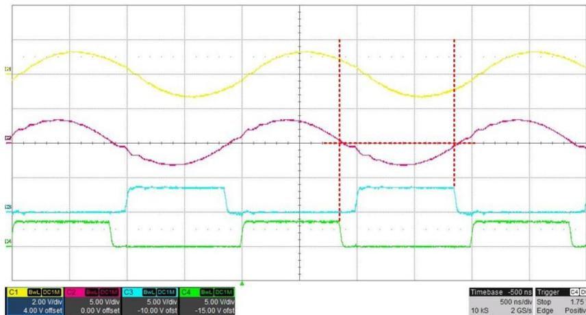
**2.4.5  $F_{sw}=700kHz$ , 2.9kW: C1: XFMR Primary Winding Current (100mV/A), CH2: XFMR Secondary Winding Current (200mV/A), CH3: SR Driving Signal (PWM3A), CH4: SR Driving Signal (PWM3B)**
