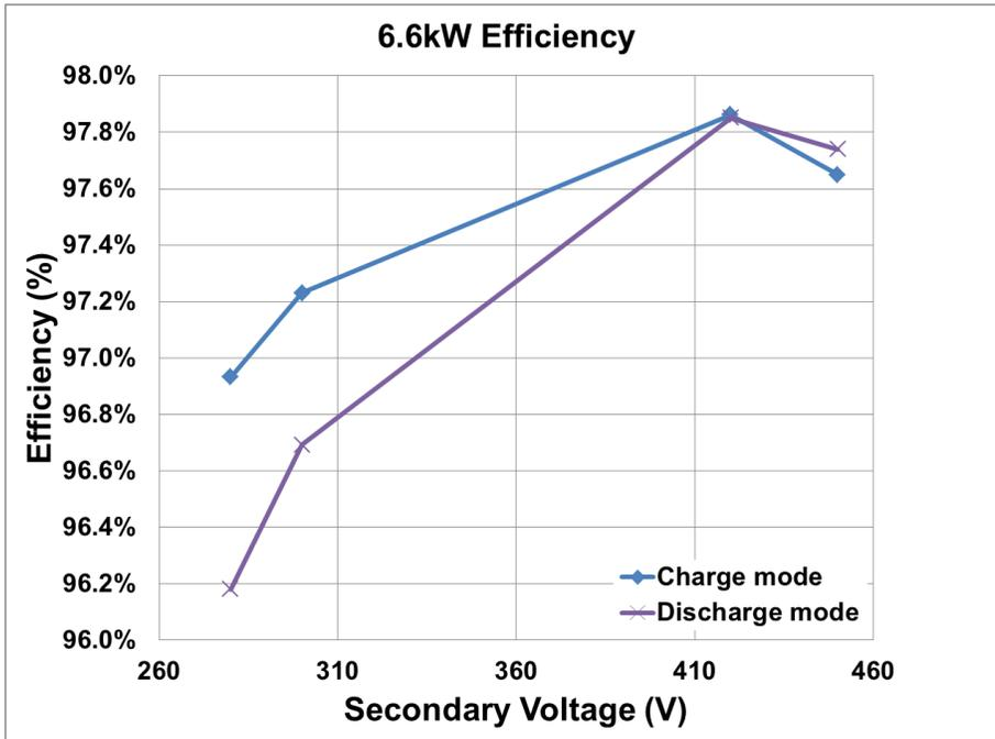
**2.2.3 Efficiency in Two Energy Flow Directions (Charge Mode: From HV to LV; Discharge Mode: From LV to HV)**
