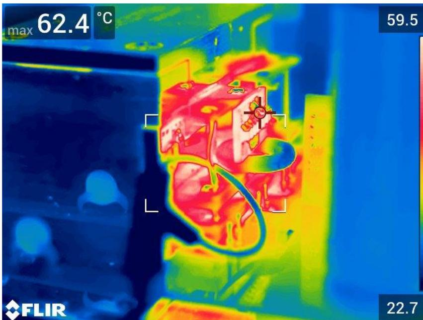
2.3.2 Charge mode: 565Vprim, 420Vsec/6.6kW, Fsw=517kHz,  $\eta=97.9\%$
