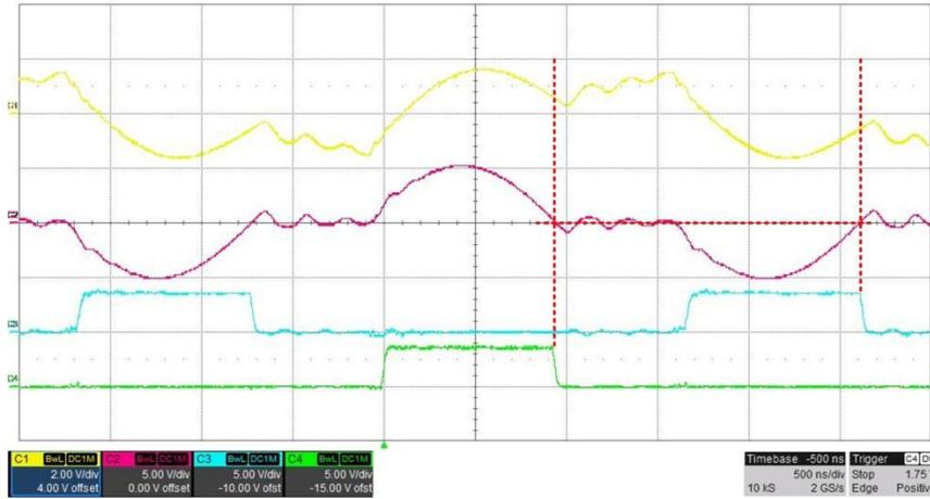
**2.4.4  $F_{sw}=500\text{kHz}$ , 3kW: C1: XFMR Primary Winding Current (100mV/A), CH2: XFMR Secondary Winding Current (200mV/A), CH3: SR Driving Signal (PWM3A), CH4: SR Driving Signal (PWM3B)**
