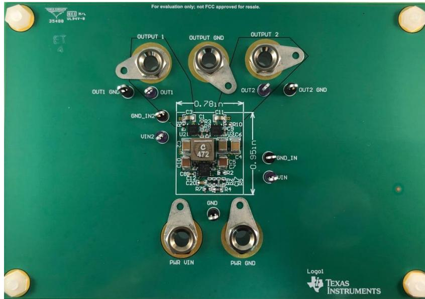
Figure 5. PMP21771 Evaluation Board
