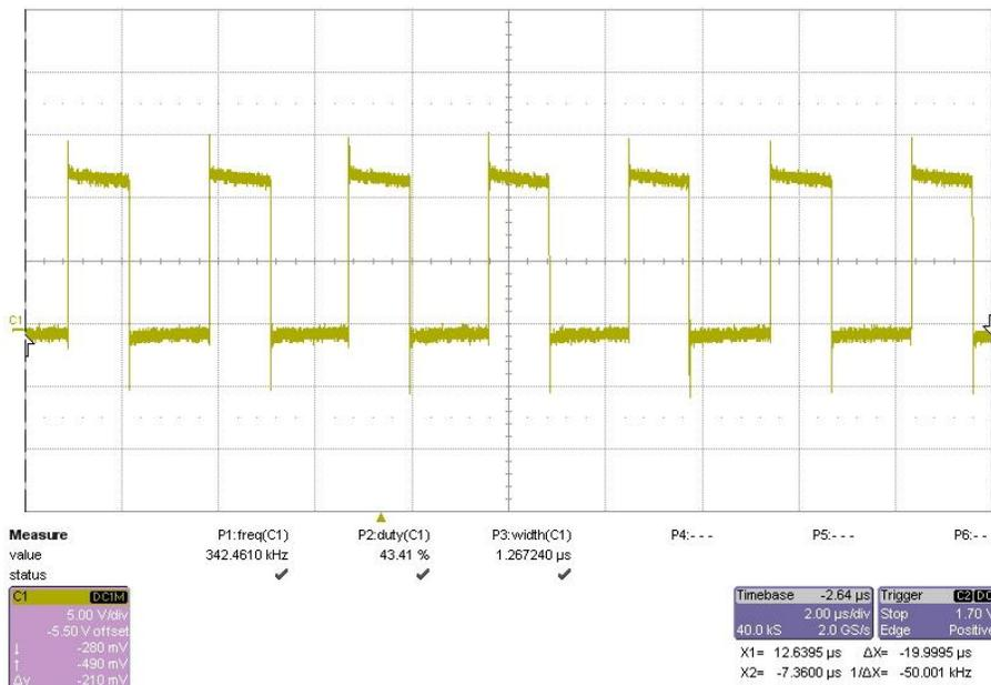
Figure 8. Switch Node Waveform (6 A Load)
