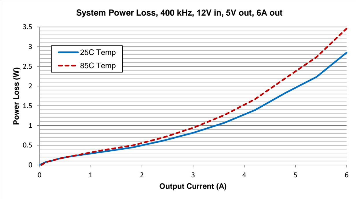
Figure 2. Power Loss vs.  $I_{OUT}$
