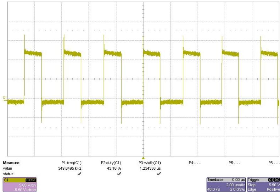
Figure 7. Switch Node Waveform (No Load)
