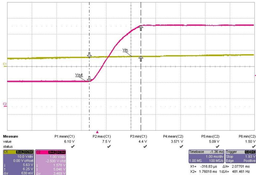
Figure 16.  $V_{IN} = 12\text{ V}$ ,  $I_{OUT} = 0\text{ A}$  (OUT2)
