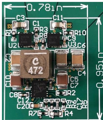
Figure 6. PMP21771 Solution Size
