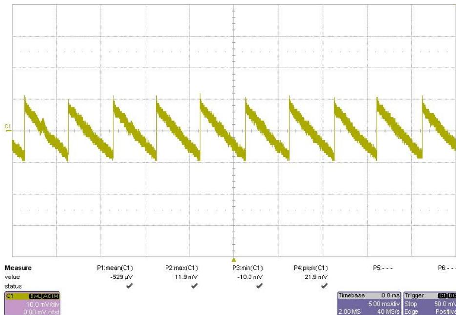
Figure 10.  $V_{IN} = 12\text{ V}$ ,  $I_{OUT} = 0\text{ A}$  (OUT2)
