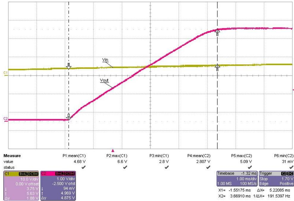
Figure 13.  $V_{IN} = 12\text{ V}$ ,  $I_{OUT} = 0\text{ A}$
