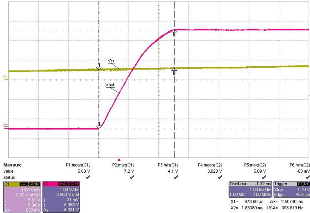
Figure 15.  $V_{IN} = 12\text{ V}$ ,  $I_{OUT} = 0\text{ A}$  (OUT1)
