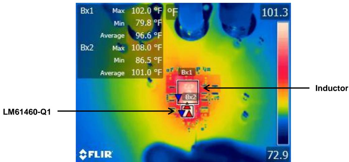
**Figure 4.  $V_{IN} = 12\text{ V}$ ,  $I_{OUT} = 6\text{ A}$**
