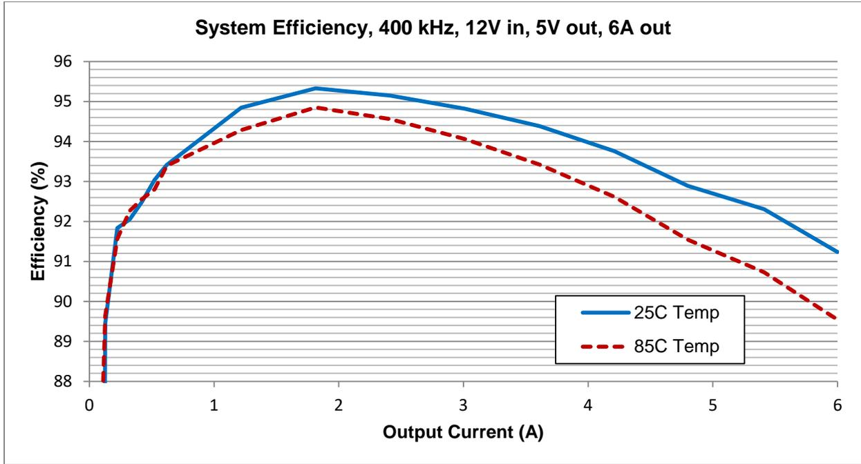
Figure 1. Efficiency vs.  $I_{OUT}$
