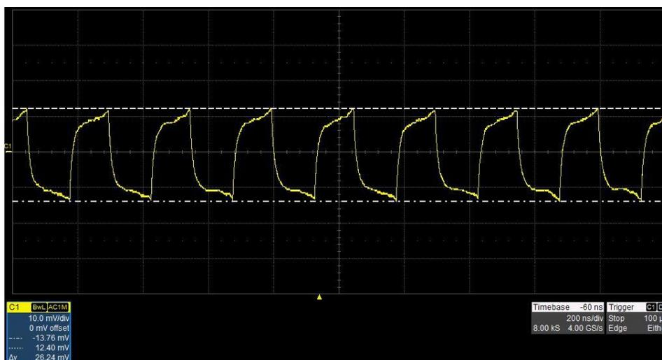
The output ripple voltage is shown in the figure below. The image was taken with the 1V8\_C output loaded to 0.3A and the input voltage VBAT set to 4.1V. (10mV/DIV, 1uS/DIV)
