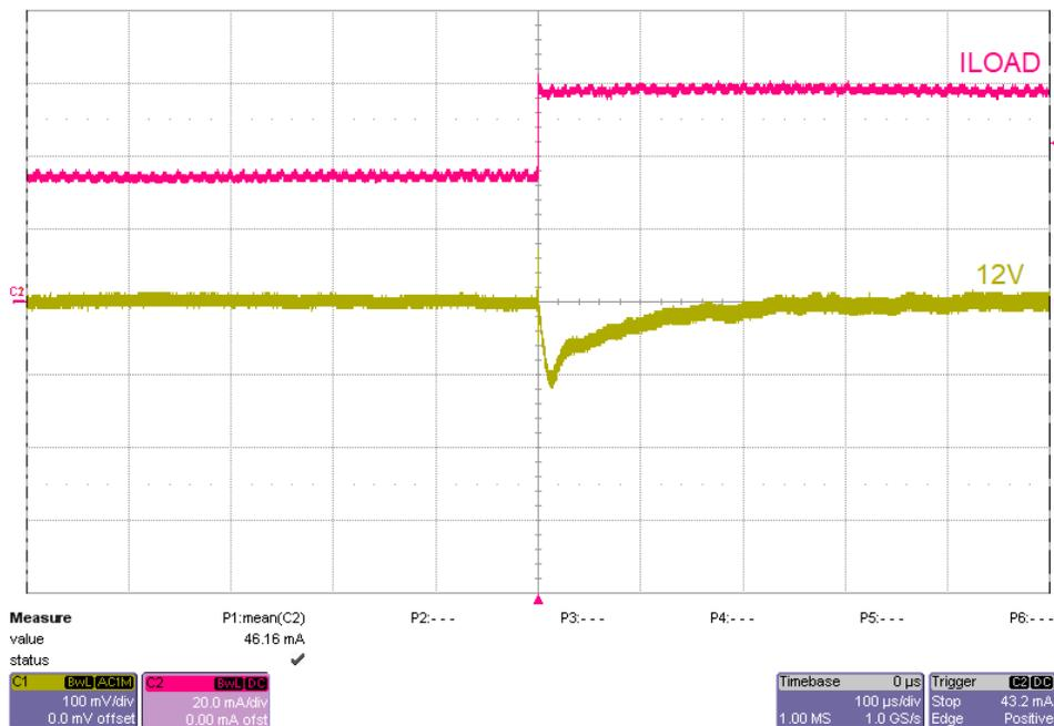
The photo below shows the 12V output voltage (ac coupled) when the load current is stepped *DOWN* between 0.036A and 0.060A ( $R_{Decade} = 333\ \Omega$ ,  $R_{Load} = 200\ \Omega$ ).  $V_{BAT} = 4.1V$ . (100mV/DIV, 20mA/DIV, 100uS/DIV)
