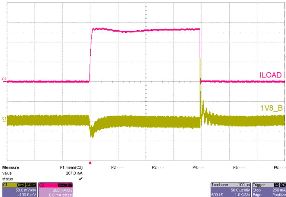
The photo below shows the 1V8\_C output voltage (ac coupled) when the load current is stepped between 0.075A and 0.345A. VBAT = 4.1V ( $R_{Decade} = 24\Omega$ ,  $R_{Load} = 6.6\Omega$ ). (50mV/DIV, 100mA/DIV, 50uS/DIV)
