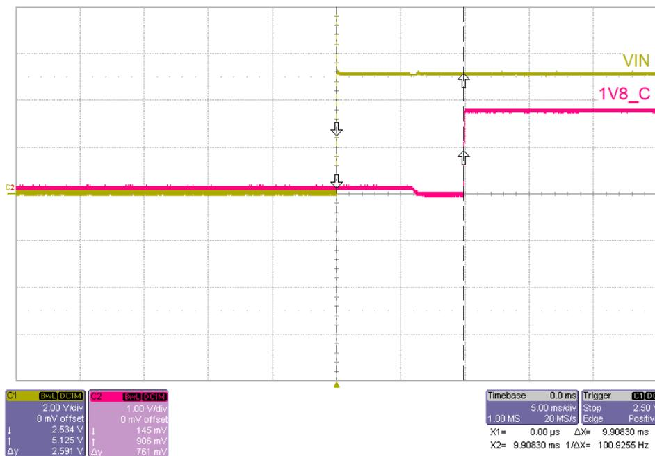
The photo below shows the output voltage startup waveform after the application of 5V in on the VIN rail with the 1V8\_D output rail loaded to 0A. (1V8\_D: 1V/DIV, 5mS/DIV), (VIN: 2V/DIV)
