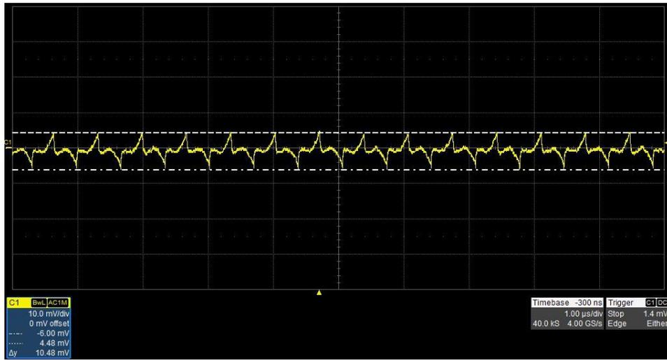
The output ripple voltage is shown in the figure below. The image was taken with the 1V8\_D output loaded to 0.1A and the input voltage VBAT set to 4.1V. (10mV/DIV, 500nS/DIV)
