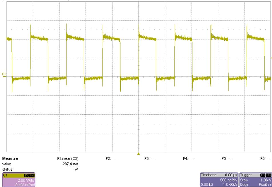
The photo below shows the switch node voltage. The input voltage VBAT is 4.1V and the 12V output is loaded to 0.06A. (5V/DIV, 500nS/DIV)
