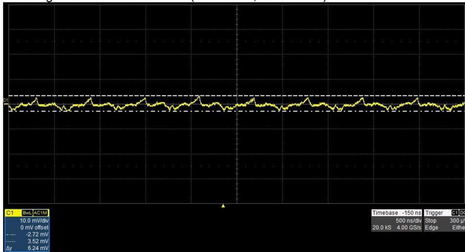
The output ripple voltage is shown in the figure below. The image was taken with the 12V output loaded to 0.06A and the input voltage VBAT set to 4.1V. (10mV/DIV, 1uS/DIV)
