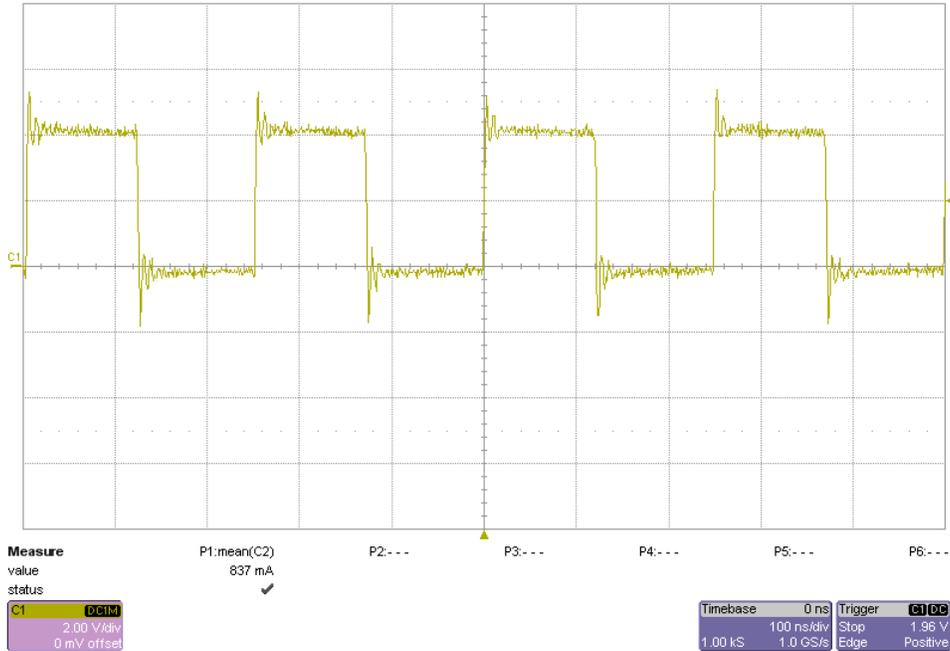
The photo below shows the switch node voltage. The input voltage VBAT is 4.1V and the 1V8\_C output is loaded to 0.3A. (2V/DIV, 500nS/DIV)
