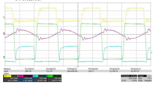
2.4.6 Soft-switching waveforms at 568.323Vin, 420.010Vout/6584.1W, 97.888%: C1: Q107\_VGS, C2: Isec measured with Rogowski Coil with 100mV/A scale, C3: Q103\_VGS, C4: Q103\_VDS.
