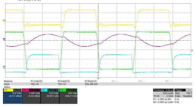
2.4.2 Soft-switching waveforms at 388.456Vin, 280.016Vout/6592.7W, Eff=96.348%: C1: Q101\_VGS, C2: Ipri measured with Rogowski Coil with 100mV/A scale, C3: Q105\_VGS, C4: Q105\_VDS.
