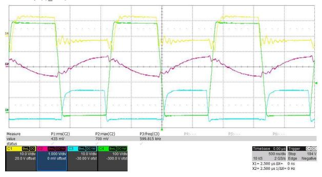
Soft-switching waveforms at 569.161Vin, 420.012Vout/6613.7W, Eff=97.696%: C1: Q101\_VGS, C2: Ipri measured with Rogowski Coil with 100mV/A scale, C3: Q105\_VGS, C4: Q105\_VDS.
