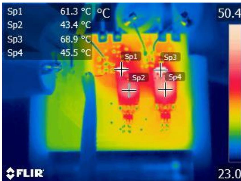
Figure 5. SN6505B Thermal Image at 120mA Load
