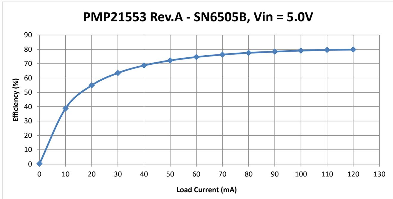
Figure 1. 19.0V Output SN6505B Efficiency with 5.0V Input
