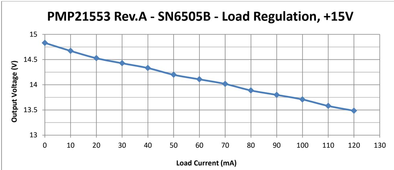
Figure 2. SN6505B Load Regulation for 5V Input, +15V Output
