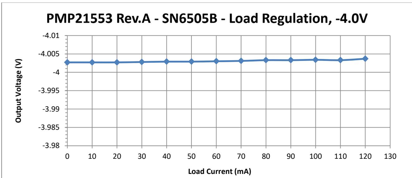
Figure 3. SN6505B Load Regulation for 5V Input, -4V Output
