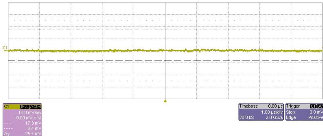
Figure 7. SN6505B Output Voltage Ripple for 5.0V Input at No Load
