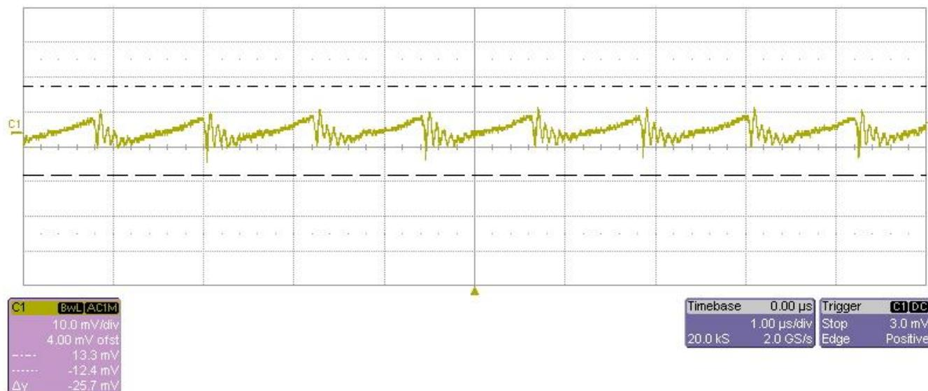
Figure 6. SN6505B Output Voltage Ripple for 5.0V Input at 120mA Load
