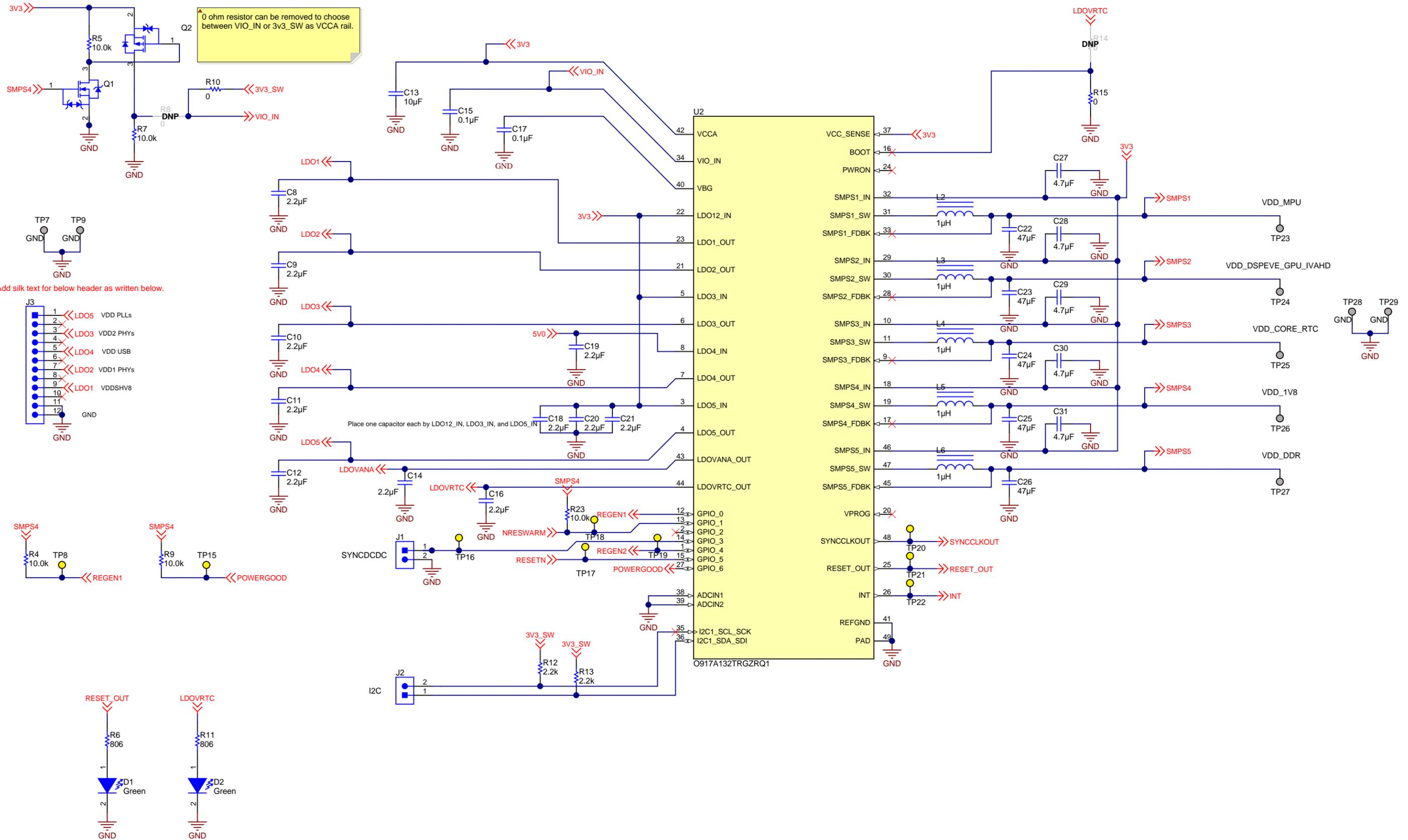
0 ohm resistor can be removed to choose between VIO\_IN or 3v3\_SW as VCCA rail.
